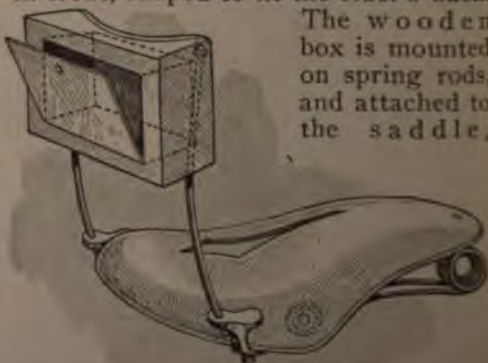
The Camera Carrier is Built in Such a Position as to Form a Back Rest for the Rider
