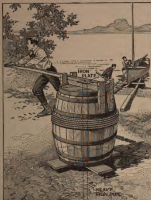
A Powerful Windlass can be Rigged Up Quickly with a Barrel as the Drum, and by Providing a Suitable Frame, the Outfit can be Made Suitable for Moving from Job to Job
