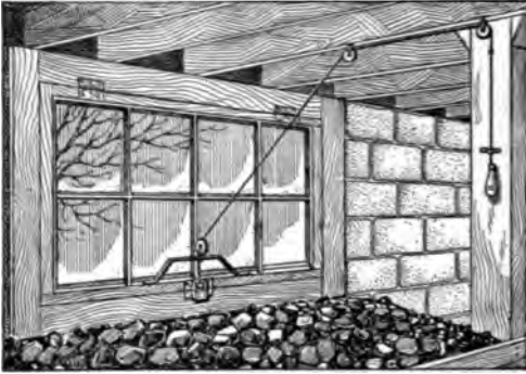
A Very Simple Arrangement for Opening and Closing the Window over the Coal Bin
