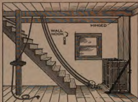
Trunks are Lifted to the Upper Floor by Placing Them on the Swinging Platform and Pulling on the Rope
