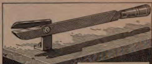
A Handy Shearing Machine for the Bench is Made from a File and a Piece of Scrap Iron
