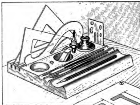
The Draftsman Who Keeps His Tools in a Rack will Have Less Trouble in Finding Them and More Room on His Table
