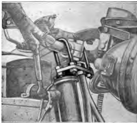
This Improved Fastening for a Pair of Motorcycle Handlebars was Made in Less Than an Hour. It Proved to Be Stronger Than the Original
