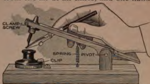
A Slight Pressure of the Hand Brings the Inking Quill into Position
