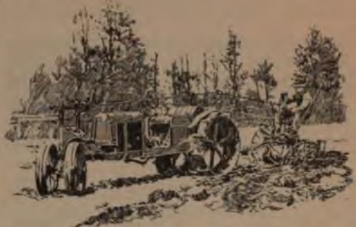
The Auxiliary Tractor Control Enables the Operator to be on the Riding Plow and to Handle Both Machines with Maximum Efficiency and Ease
