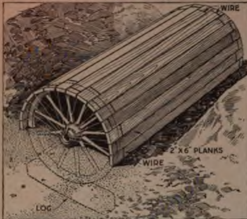
By the Use of Old Wagon Wheels Wired to the Planks Which Supported the Concrete for a Culvert, They are Easily Recovered for Further Use
