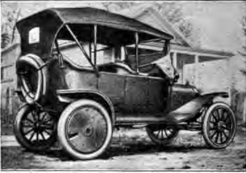
The Right Rear Wheel of This Automobile is Made from Three Wooden Disks Fitted to the Old Hub and Felloe. After the Spokes had Broken. The Car was Driven 250 Miles with It
