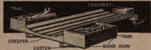
The Trays Incorporated as a Part of the Creeper Enable One to Keep All His Tools within Reach as He Moves About under a Motor Vehicle
