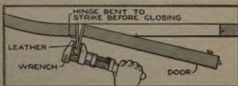
A Simple Remedy for the Rattling of Automobile Doors Is to Bend the Hinges Slightly
