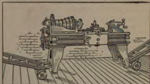
By the Use of Two Hand Trucks and a Few Minutes of Three or Four Men's Time, the Lathe can be Quickly Moved
