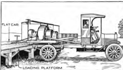
By Moving a Truck Forward and Back under Its Own Power, Heavy Machines are Unloaded from It on Rollers, and Pushed onto Flat Cars
