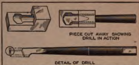
Threaded Holes are Easily and Efficiently Enlarged at the Bottom by the Use of This Simple Tool
