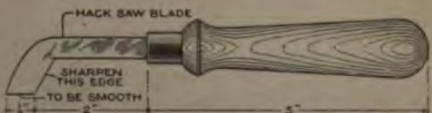
For Scraping Insulation, and for Many Other Electrical Uses, Hacksaw-Blade Knives Are Useful
