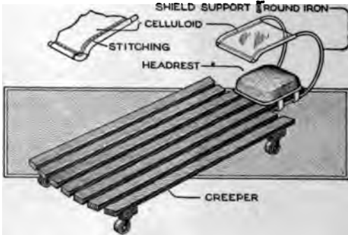
The Frame, Made by Bending an Iron Rod, Supports a Celluloid Shield above the Headrest of the Creeper
