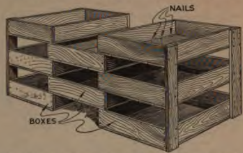
The Boxes are Arranged in Tiers to Form Handy Stock Bins. More Rows may be Added as Desired
