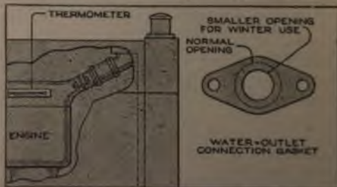
By Providing a Gasket with a Smaller Opening, the Radiator System is Operated Economically in Cold Weather
