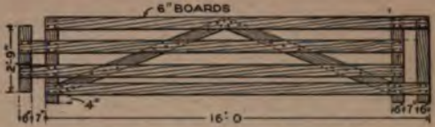
Universal Panel with Interlocking Ends Builds Portable Fence to Confine Stock to Small Feed Areas
