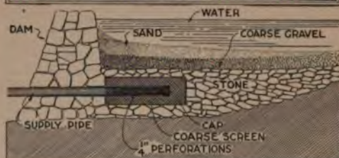
A Steady Flow of Water Free from Surface Dirt is Obtained through the Pipe
