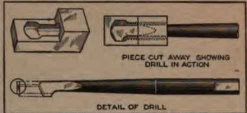
Threaded Holes are Easily and Efficiently Enlarged at the Bottom by the Use of This Simple Tool
