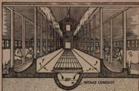
A Conduit Running the Full Length of the Dairy Barn Provides the Cattle with Fresh Air
