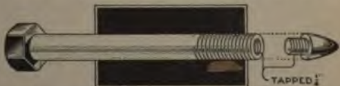
The Conical Steel Head Attached to the Engine Bolts Enables the Motorcycle Repairman to Fasten a Motor in the Frame Regardless of the Alignment of the Bolt Holes
