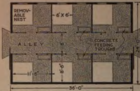
Floor Plan of the Sanitary Hog House, Showing the Arrangement of the Interior, Nests, Concrete Feeding Troughs, and Other Features: Gates may be Added to the Pens, or in the Alley, as Desired
