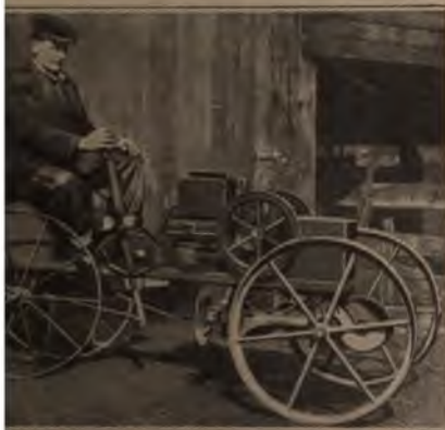
This View Shows the Mower Pitman and the Shaft Connecting It with the Engine, and Also the Steering Lever, Gripped by the Driver
