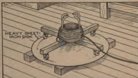
The Wire may be Drawn from the Reel Easily in Various Directions
