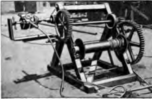
A Socket Wrench was Gripped in the Air-Motor Drill and Set on the Windlass Shaft
