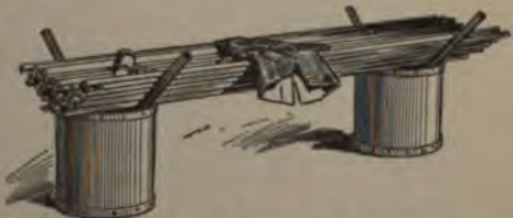
This Method of Storing Pipes or Rods Temporarily can be Adapted Widely, Using Wooden Kegs or Boxes if Necessary
