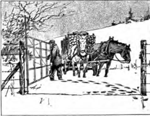
Instead of Shoveling a Path for the Gate at Its Usual Level, It is Raised and Supported on Pins Set in the Long Pipe
