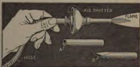
The Mantle Fixture was Quickly Converted into an Effective Bunsen Burner, with a Blowtorch Action, by Flattening the End of the Tube
