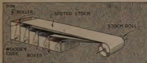
A Stock Roll of Several Layers can be Made Easily with an Arrangement of Bobbins
