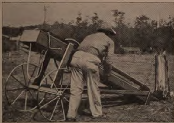
This Stump-Boring Machine of the "Day" Type Is Very Efficient for Preparing Stumps for Blasting in Clearing Land
