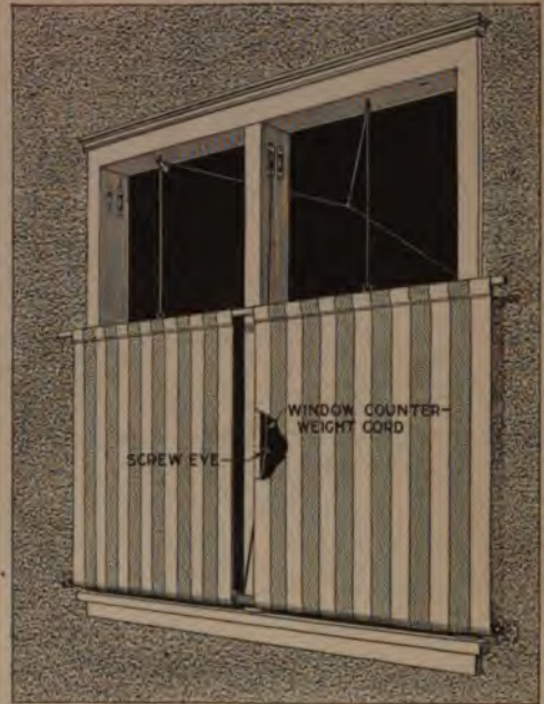
The Curtains are Held Taut and Rolled by the Center Cord Fixed to a Sash Weight
