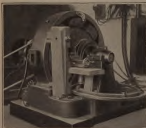
The Commutator was Turned True Quickly with This Arrangement, and the Motor was Out of Commission Only a Short Time, Because It Was Not Necessary to Take Down the Machine
