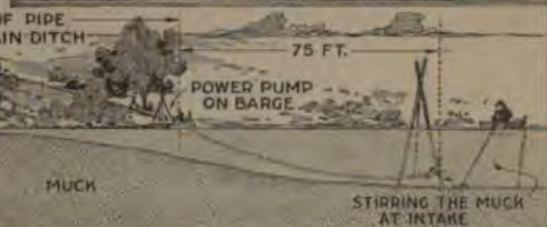
General Plan of the Muck-Pumping System, and a View of the Discharge Pipes at the Main Irrigation Ditch
