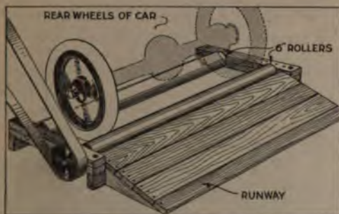
The Rear Wheels of the Automobile are Run onto the Rollers, and Transmit Power to the Drive Pulley
