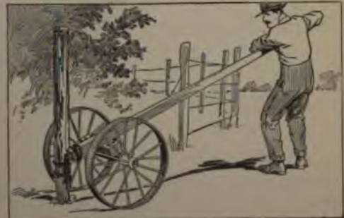
The Post is Quickly Withdrawn with Slight Effort, by Bearing Down on the End of the Lever
