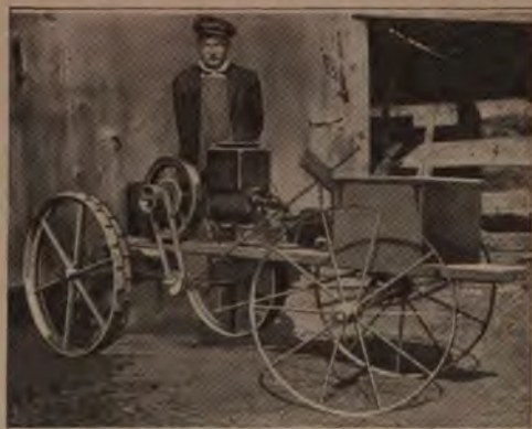
Fig. 2. The Belting of the Power from the Engine Shaft to the Lower Shaft, Which Connects with the Pitman Shaft on the Opposite Side, and the Clutch-Control Rod as Shown in This View
