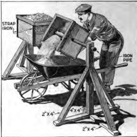
The Measuring Boxes are Used in Batteries to Make Up a Properly Proportioned Batch at a Time
