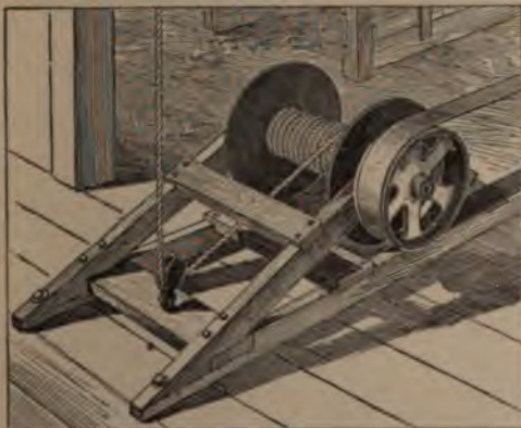
This Hoisting Arrangement was Devised on the Farm for Use with an Engine, in Putting Hay into the Mow
