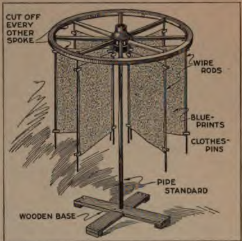
The Blueprints are Stretched from the Spokes of the Pivoted Buggy Wheel
