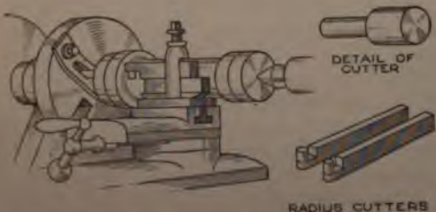
Smooth, Circular Curves were Cut in Turned Work on the Lathe by Means of Adaptable Cutters Made in Several Standard Sizes
