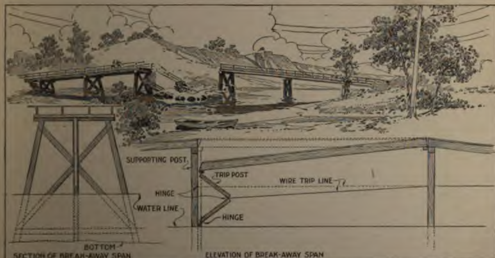
The Car Automatically Trips the Break-Away Span, Precipitating Itself into the Stream
