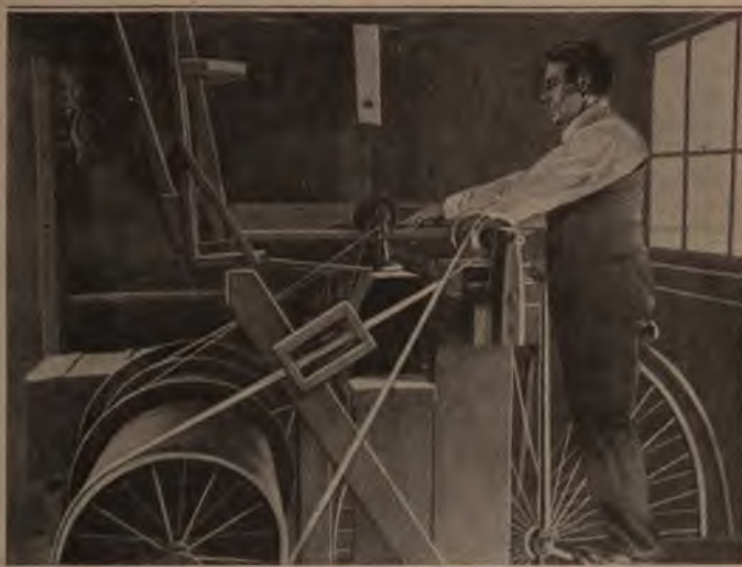
An Old-Fashioned High-Wheeler Bicycle was Rigged Up to Provide the Driving Gear for This Combination Machine; the Operator is Ripping Stock on the Circular-Saw Attachment
