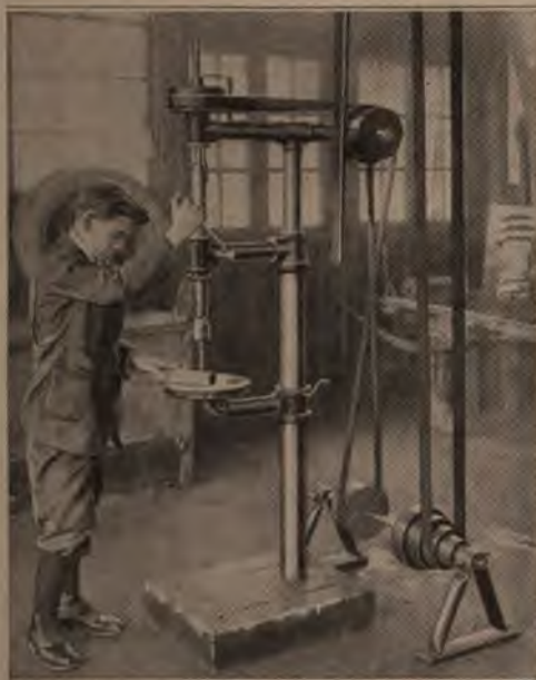
This Substantial Drill Press was Made by Boys in a School Shop, Pipes and Fittings Being the Chief Materials Used. It has Withstood Hard Wear
