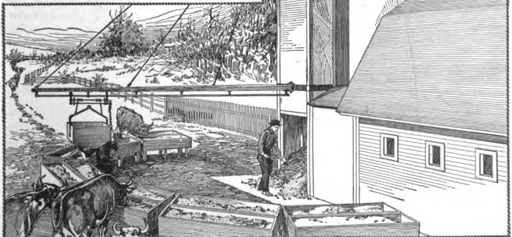
Silage is Handled Rapidly and Economically with a Minimum of Manual Labor by the Use of the Crane and Trolley Arrangement
