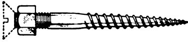
Cutting Off the Head of a Wood Screw and Threading the End Provides a Hanger Bolt
