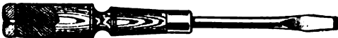
The Disk on the End of the Handle Prevents Blistering of the Palm
