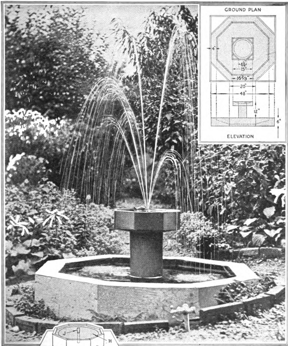
The Effectiveness of This Inexpensive Fountain for the Home Garden is Brought Out Strikingly in the Photograph Reproduced Above. The Ground Plan and the Elevation Present the General Dimensions and the Construction of the Forms for the Reservoir and the Bird Basin. The Small Sketch Shows the Use of the Forms I, for Shaping the Basin H, and the Plug J, Which Provides a Hole for the Pipe. The Sectional View Shows the Reservoir A, the Foundation B, the Post Form D, the Outlet Pipe F, and the Guide Boards M and N, for Leveling the Top Surface
