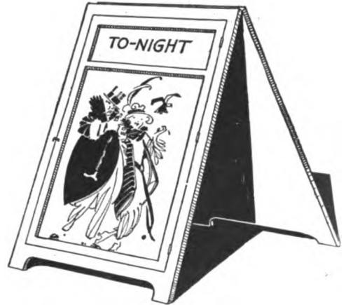
The Outer Surface of the Board Has a Hinged Skeleton Door to Hold the Poster
