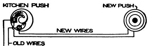
Connections for an Extra Push Button at the Front of an Apartment for the Door Latch
