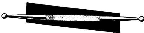
Tool Made of Steel, Highly Tempered and Polished, Then Magnetized for Taking Particles of Steel from the Eye
