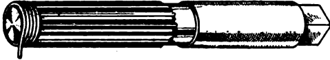
The Cutters are Ground Down and Then Wrapped with Fine Wire and Soldered
