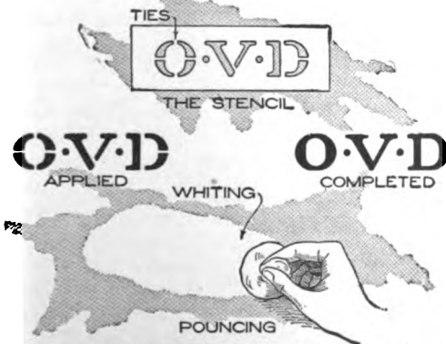
The Stencil as It is Cut; after Applying; Completed Letters; Sized and Pounced
