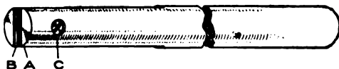
A Headless Screw Controls the Adjustment Accurately, and Holds the Parts Rigidly
