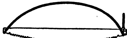
Stiffening a Cross-Cut Saw.
