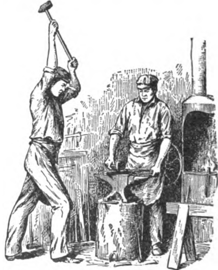
Fig. 4. The Force of the Blow Depends on How the Sledge is Grasped
