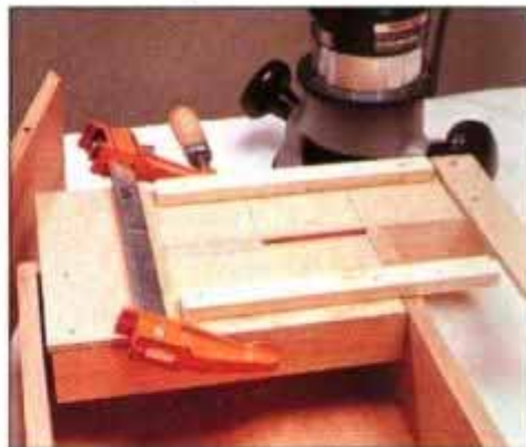
13 Cut the mortise for the lid support using a router and jig. Try the cut on a scrap piece first.
