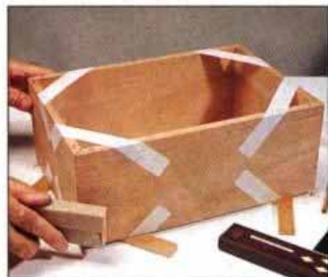
2 Test fit the sides and ends. Tape the pieces together and remove the sharp corners by hand sanding.
