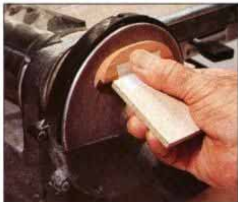
14 Cut the curve and notch in the handle pieces, then sand the taper on them, using a disc sander.
