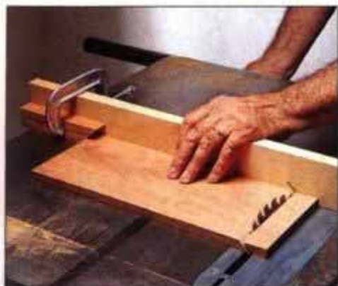
1 Cut the miters on the sides and ends, using an auxiliary fence and a 45° miter stopblock clamped in place.
