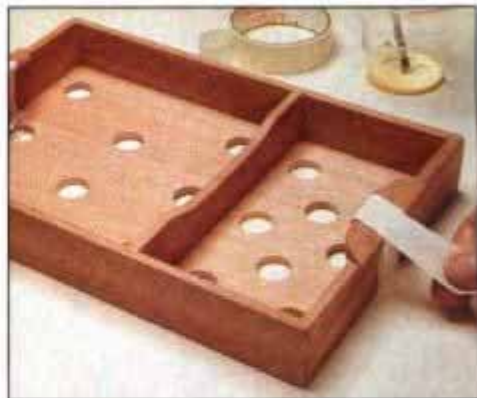
15 After the tray is sanded, apply glue on the handles and hold them in place with masking tape until the glue sets.
