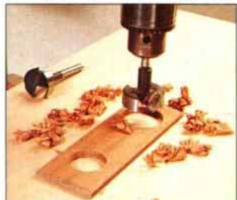
16 Bore the holes in the instrument block using a Forstner bit. Enlarge the hole for the humidifier with a drum sander.
