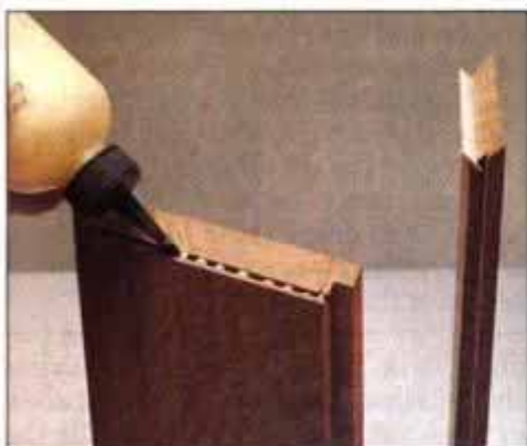
4 Apply glue sparingly and evenly in the spline slots. Use a hair-colorant squeeze bottle with a fine nozzle.
