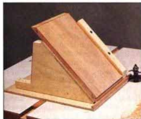
3 Use a sliding jig and slotting cutter in the router table to cut the spline slot. Make a test cut first.
