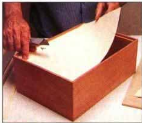
7 Make a cardboard template of the top panel. Test it in the rabbet—it should fit in the space snugly.
