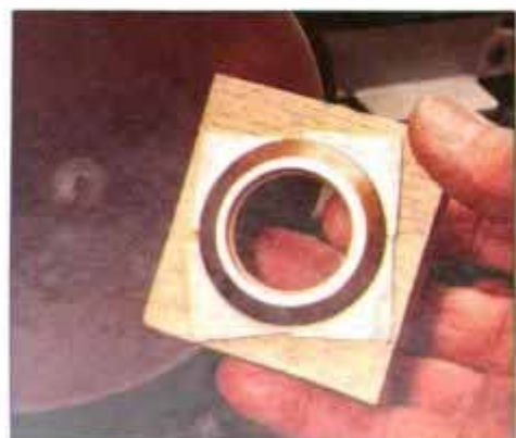
17 To sand off the center flange, the lock collar is secured to a scrap block with adhesive mounting squares.
