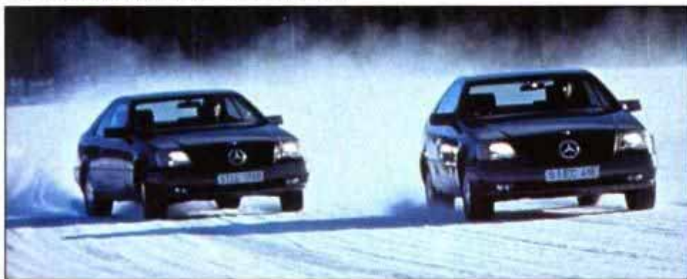
Mercedes-Benz on left has stability control switched off. Note tail-out attitude on frozen lake.
