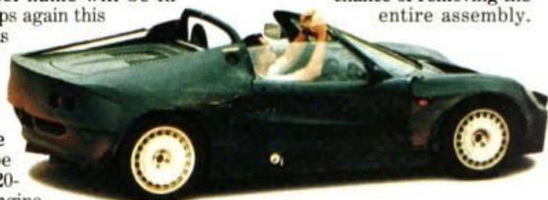
Lotus Elan has aluminum-framed, composite body.
