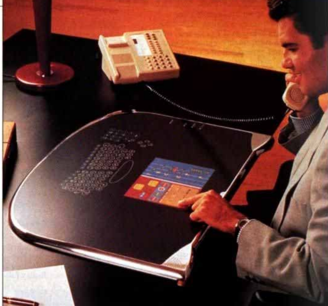
The S3500 Modula-Executive is an electronic desk blotter linked via infrared beams to your PC. The monitor is touch-sensitive so your finger works like a mouse.
