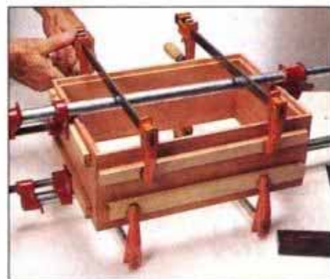
6 The waterproof glue sets quickly, so six clamps and cauls must be ready. Position the clamps and cauls as shown.
