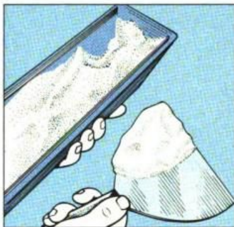
13 To reduce compound squeeze-out when working on inside corners, load only one knife corner with compound.
