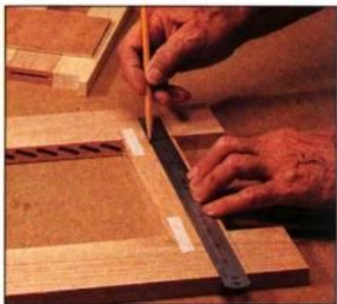
11 Align the rails with the louver slots on the stiles. After marking the work, cut the stiles to length and cut joining plate slots.
