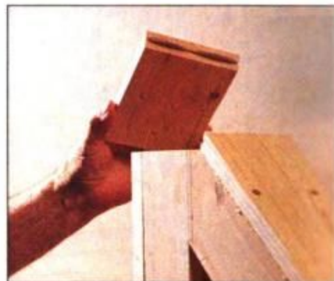
11 Use plates to join the plinth face pieces. Join the long piece to the plinth frame first, then add the short endpieces.
