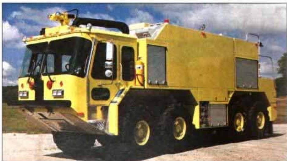
The Air Force's P-23 ARFF truck can hit 70 mph on runways and 35 mph off-road.
