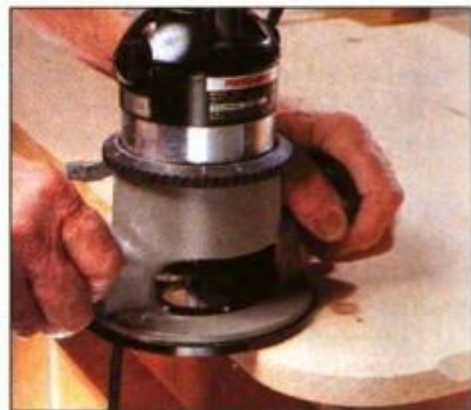
6 Use a router and piloted chamfer bit to cut the bevel around the bottom edge of the tabletop. Then, sand the top smooth.
