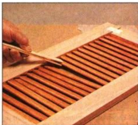
14 Assemble frame with louvers installed in one side. Draw stiles together and lift louvers into opposite slots.
