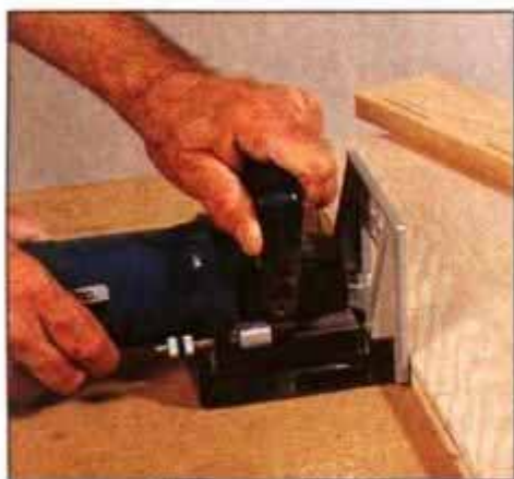
1 Place both joiner and work on a flat surface. Use a plate joiner to cut the plate slots for joining the case pieces.
