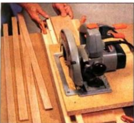
12 If you don't have a table saw, mount a circular saw on jig and pass work underneath. Have a helper at outfeed side.
