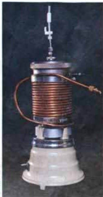
MOUTH MACHINE duplicates chewing conditions in the cause of food-flavor science.
