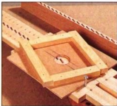
10 Clamp work between rails and butt jig against stop pin. Move pin after each slot. Reverse jig after two stiles have been cut.
