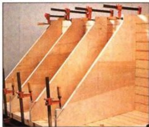
7 After cutting shelf panels, tack triangular blocks to corners and clamp panels to back assembly. Bore screw pilot holes.
