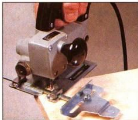
5 Cut the 3-in.-rad. rounded corners with a sabre saw and circle-cutting jig. Cut from the bottom side of the tabletop.
