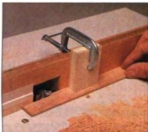
13 Use a 1/8-in.-rad. half-round bit and router table to cut louver edges. Set fence to produce finished 1-in. louver width.
