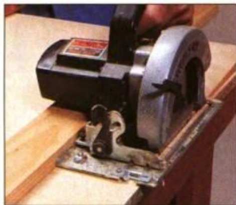
4 Use a circular saw to cut the tabletop to exact length and width. Guide the saw with a straight board clamped to the top.
