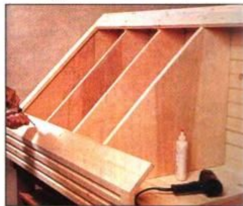
8 Join shelves to back with screws and glue. Then, apply glue and install side and stile assemblies with countersunk screws.
