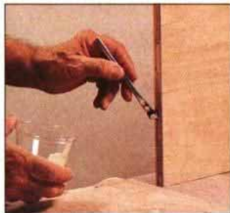
6 Apply glue to the side panel slots for joining to the floor and ledger. Use face frame to keep case square while clamped.
