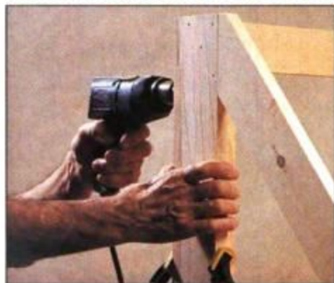
9 Use screws and glue to join the triangular lower frames to the back frames. Bore pilot holes to avoid splitting the wood.
