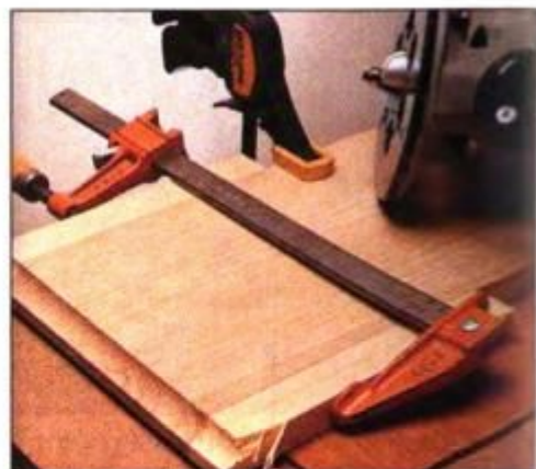
15 Use a router and 3/4-in.-rad. cove bit to trim the drawer fronts. Scrap pieces clamped to edges prevent splitting.
