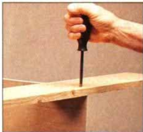
5 After the floor and divider have been joined with plates, glue and screw the pine rear ledger to the cabinet divider.
