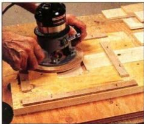
1 Rout the half lap joints with a straight bit. Hold workpiece in a jig that has guide strips to confine the cut to the lap area.
