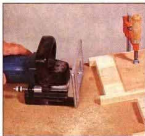
2 To cut centered slots in the face frame pieces, place the oak components in a jig that also holds the joiner in position.
