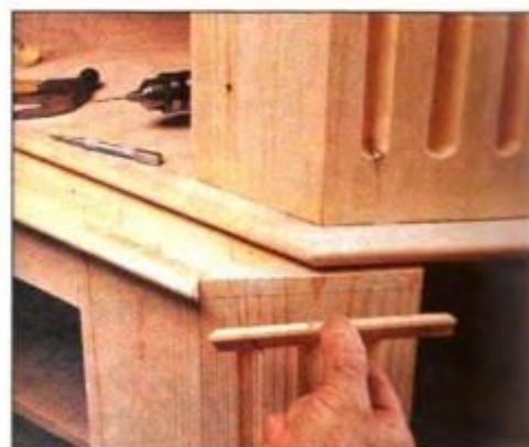
13 Miter remaining molding to length, and install each profile, long piece first. Use glue and finishing nails.
