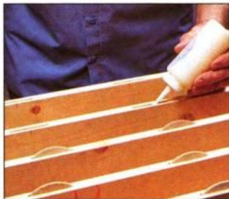
2 Apply glue to the plate slots and insert the plates. Then, apply glue along the boards' mating edges and assemble.
