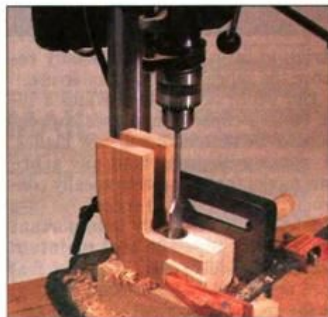
4 Use a 1\frac{1}{16} -in.-dia. spade bit ground down to 1\frac{1}{16} in. to make the hole for the \frac{3}{4} -in. plunger-assembly pipe.
