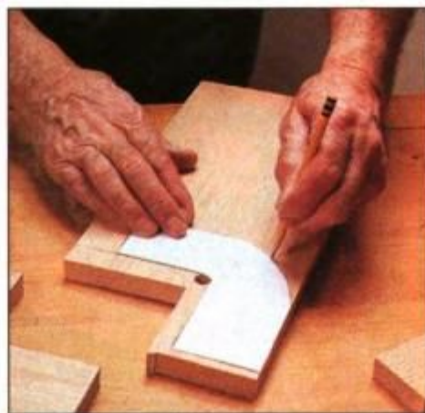
2 Make templates for contoured pieces. Trace cheek template on oak stock. Hole at corner handles inside radius cut.
