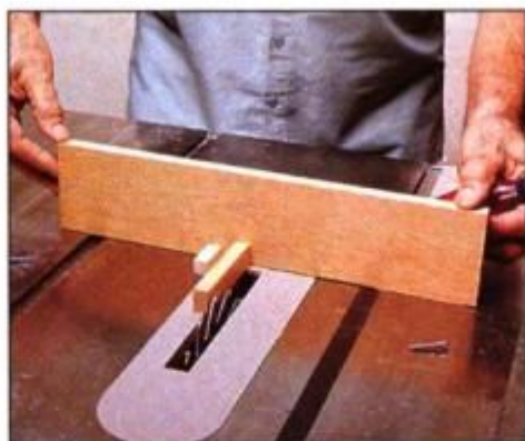
1 To position the auxiliary fence, butt the fence's guide pin against the spacer strip placed beside the dado blade.
