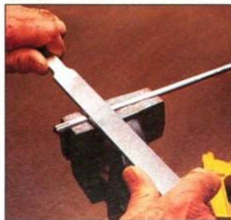
12 Use draw filing to produce flat on plunger rod. Hold file perpendicular to work. Push and pull with even pressure.
