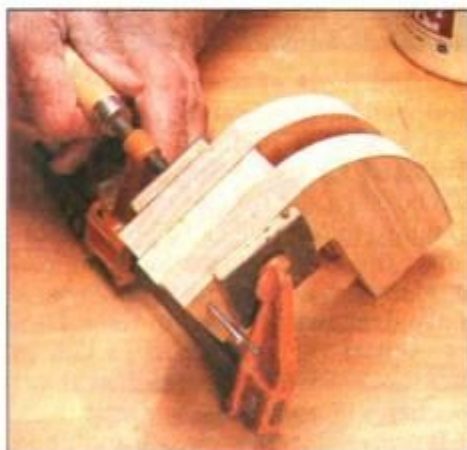
3 When gluing cheeks to spacer, use nails to maintain alignment. The spacer thickness should match the arm thickness.
