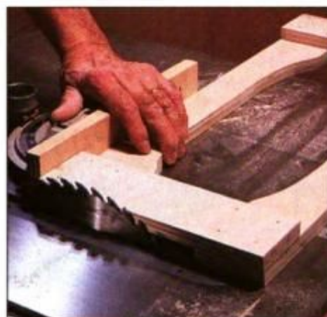
9 After assembling the side-frame components with glue and nails, trim the frame ends to a 10° bevel on the table saw.
