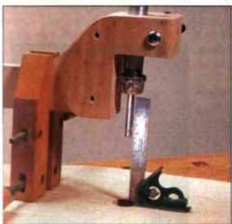
15 Clamp arm to table and use a square to align plunger rod with hole in table. Then bore pilot holes for mounting.
