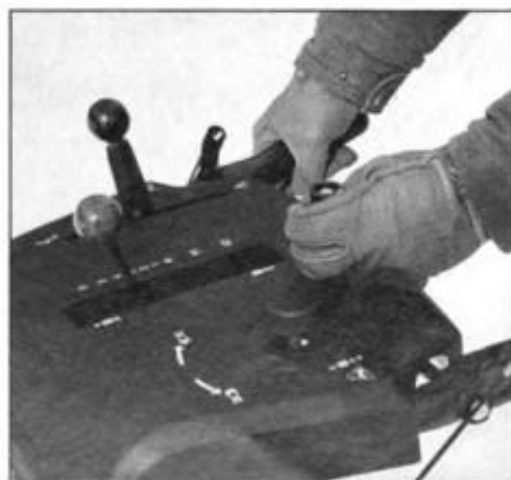
The rotating hand crank directs snow chute up to 100° right or left. Crank is linked to the chute by rod and U-joints.
