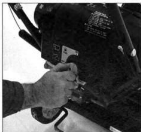
The machine features a fuel shutoff valve that must be opened before starting and then closed when finished.
