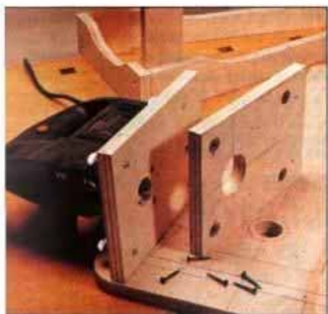
17 Make sure Teenuts are installed in upper plate before gluing to table. Lower plate holds sabre saw.
