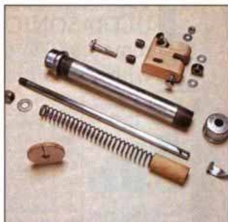
14 Completed blade holder/plunger components. Bearing block at upper right reinforces plunger rod.
