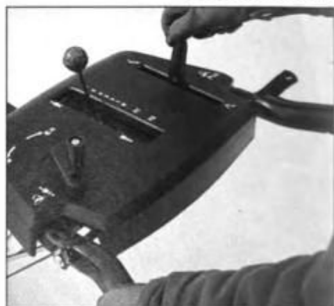
To control height and distance of blown snow, chute spout is adjusted up and down with lever on handle console.
