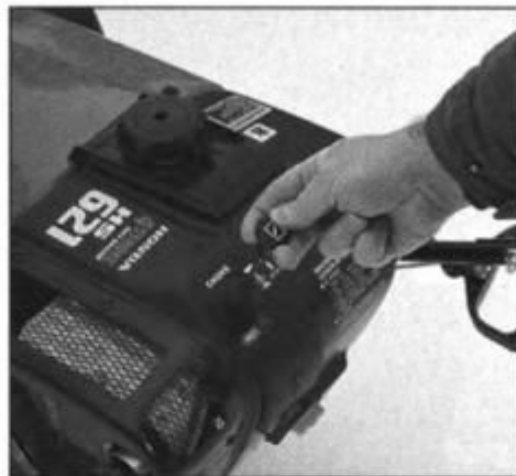
The last step before pulling the starter cord is to pull out the choke switch, located just behind the oversize fuel fill cap.
