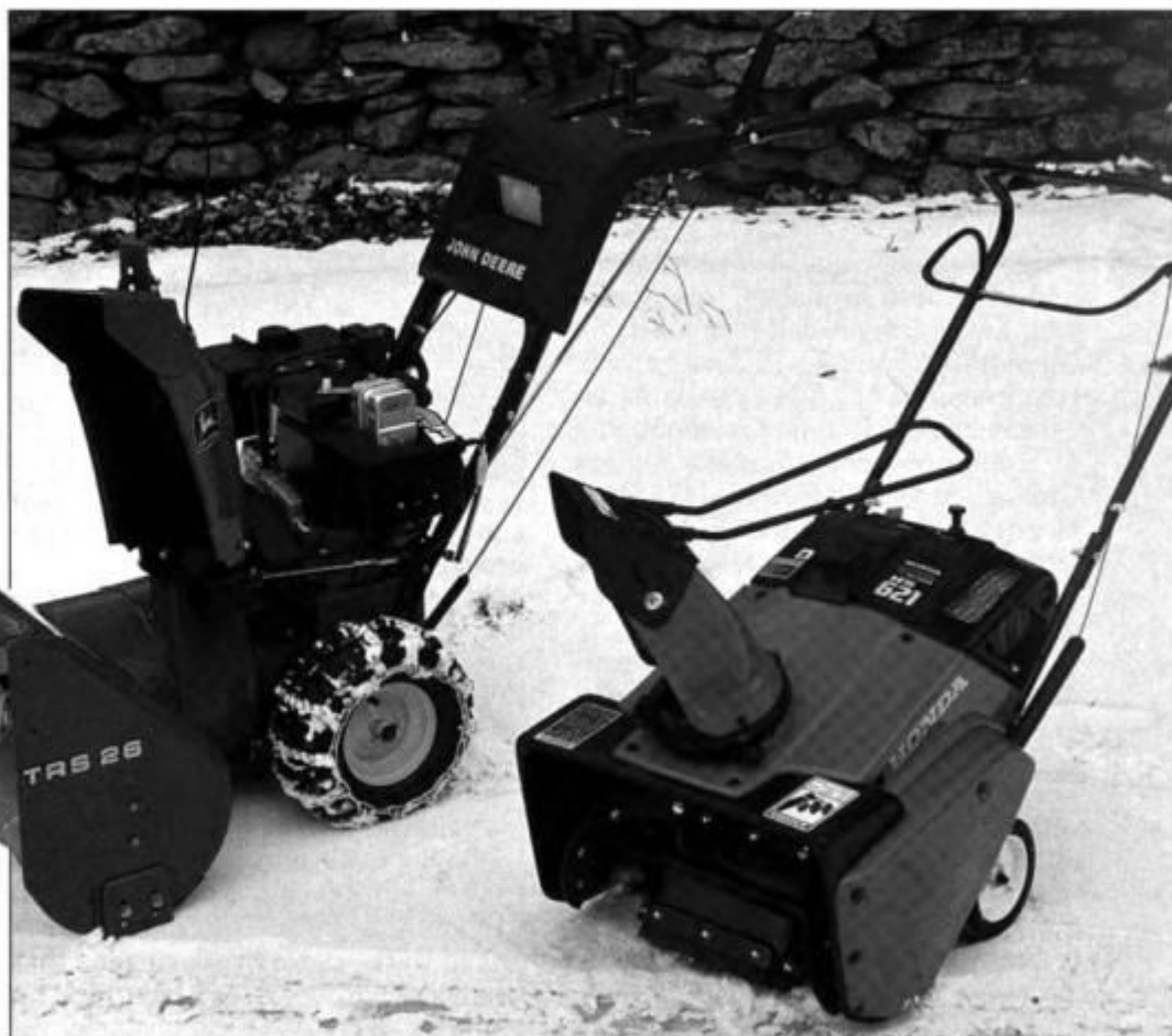
The midscale, 2-stage John Deere TRS26 (left) features an 8-horsepower engine and a 26-in.-wide x 20-in.-high auger housing. The Honda HS 621A (right) handles lighter snow accumulations with a single-stage auger, manual drive and a 5.5-hp engine.
