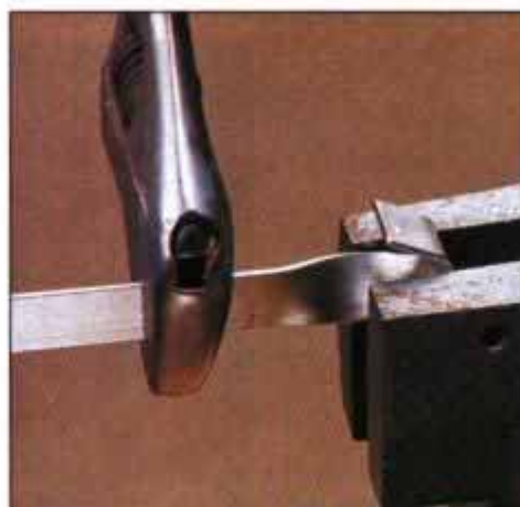
13 Bend the end of a steel strip around a bolt to form hook on lower blade holder. Use a wrench to twist shank 90°.
