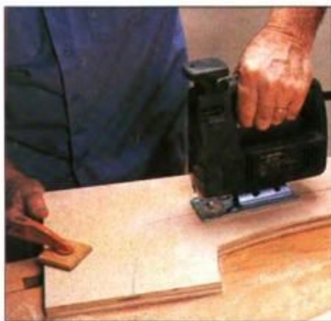
1 Mark the arm outline on \frac{3}{4} -in. plywood. Then, cut to the line with a sabre saw and sand the sawn edges smooth.
