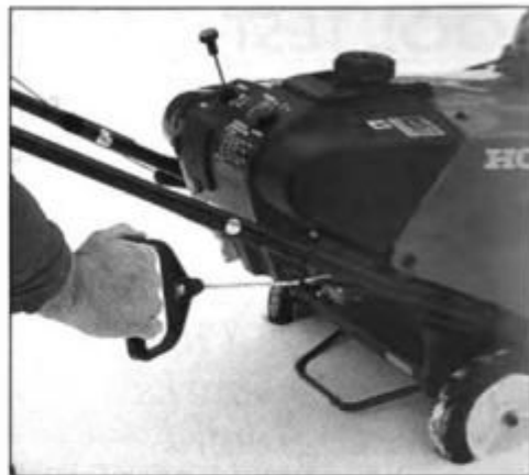
The recoil starter cord—located in a comfortable position—was easy to pull, and the engine fired on the first pull every time.
