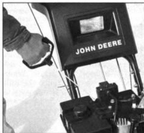
The TRS26's recoil starter features an oversize handle for winter gripping. An electric starter is available as an option.
