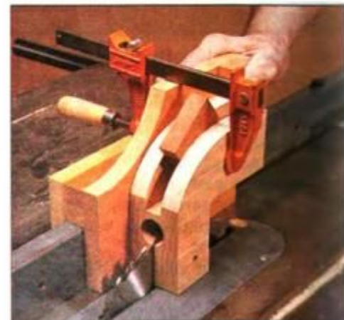
5 Use a table saw to cut the kerf in the arm head assembly. A jig that straddles the fence makes the cut safe and secure.
