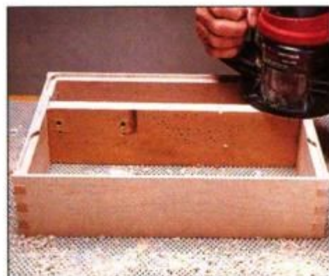
5 Place a length of scrap inside the assembly to support the router when you cut the rabbet in the sides and ends.
