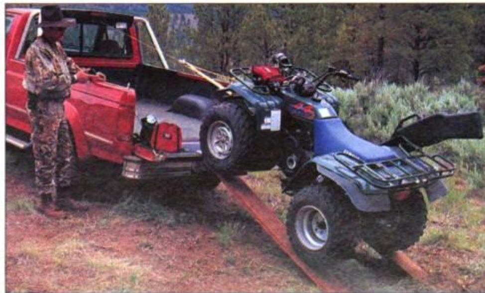
A Warn PowerBar winch safely walks a big Yamaha utility ATV up steep, narrow ramps.
