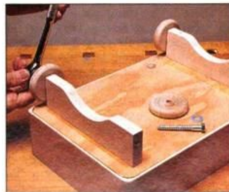
7 Attach the bottom and the wheel support blocks. Don't forget to use a washer on each side of the wheels.
