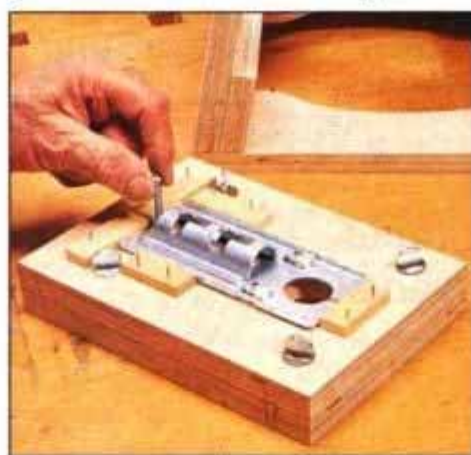
16 Remove shoe from sabre saw and place on underside of lower mounting plate. Then mark the screwholes.
