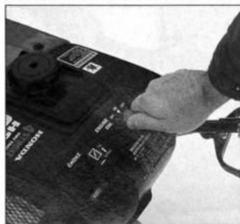
There is an ignition switch that must be turned on to start the unit. When turned off, the switch kills the engine.
