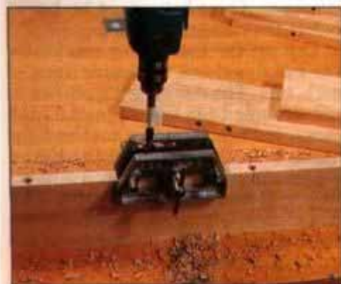
2 Bore on the dowel-location marks using a doweling jig. The tape on the drill bit serves as a depth indicator.
