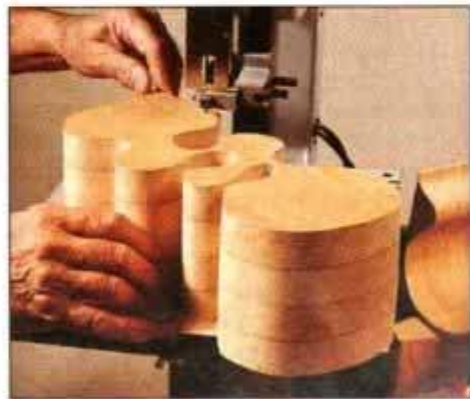
4 Tight contours with a ⅛-in.-wide blade are possible in thick stock. The blade tracks well and it produces true cuts.
