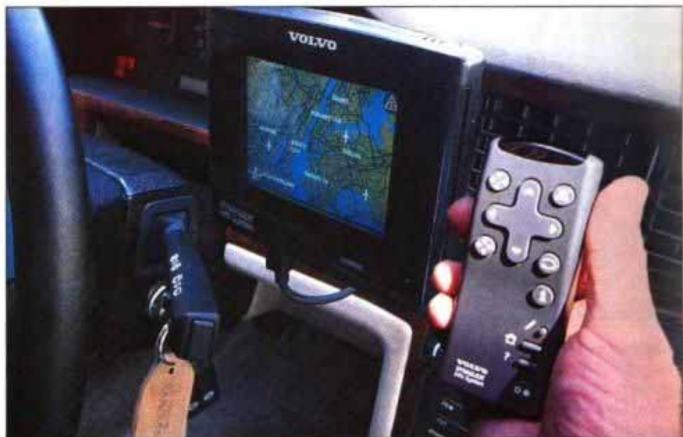
Remote control allows you to scroll around the maps on the high-resolution monitor.
