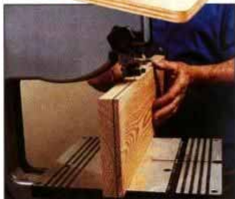
2 Resawing 6½-in.-wide fir into ⅜-in.-thick slices is well within the tool's capabilities. A ½-in.-wide blade is used here.
