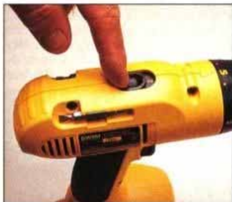
1 A sliding switch handles changing gears. The low range is for high-torque use, and the high range provides speed for drilling.
