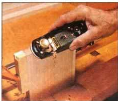
11 Cut the curved edge on a step with a block plane. The scrap blocks at both ends of the step prevent endgrain tearout.
