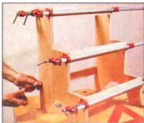
10 Assemble the stool sides and rails, then clamp them. Use one clamp at each of the five rail locations.
