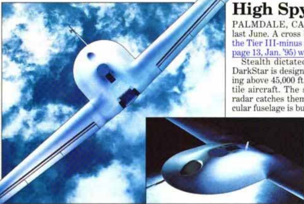
At 15 ft. long and 69 ft. across, DarkStar sports sat-com equipment on top of fuselage.
