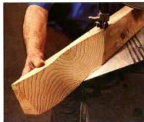
3 Contour cutting is the forte of any band saw. With a ¼-in. blade, our test tool handled beveled contour in thick stock.
