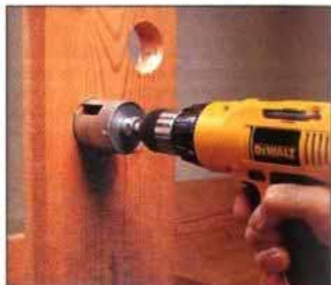
4 The driver/drill's 14.4-volt power makes many heavy-duty operations practical. Hole-sawing is well within the tool's capacity.
