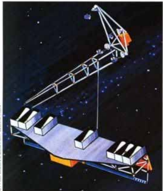
OSI would use seven 1-ft.-wide telescopes to gain three times Hubble's resolving power.
