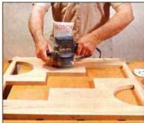
5 Clamp both of the sides and the other parts securely to the workbench and sand them before assembly.
