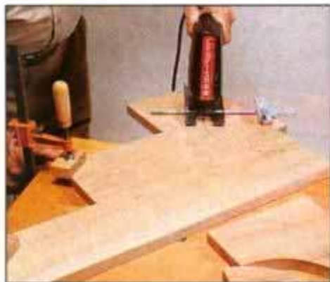
4 Using a sabre saw and pivot guide, make the base cutout in the side. An extension block supports the guide.
