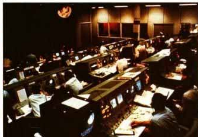
New workstation-oriented Mission Control Center (left) is replacing mainframe-based original center (above).
