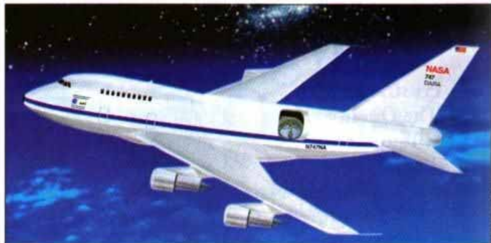
SOFIA will carry aft-mounted infrared telescope on short-fuselage, long-range 747SP.
