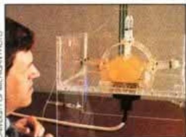
Elasticity imaging is tested on gel that simulates abdominal tissue.
