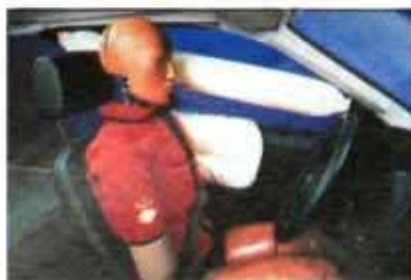
BMW's tubular airbag deploys from door upholstery to cushion head.
