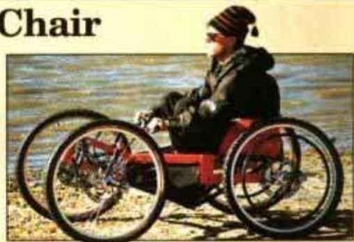
Phoenix all-terrain wheelchair conquers trails with 4-wheel suspension and hydraulic brakes.
