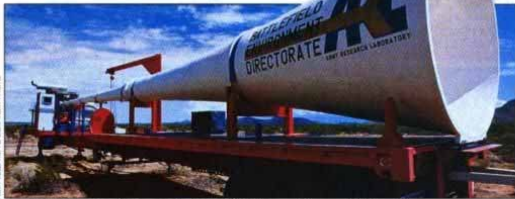
Army's Mobile Acoustic Source stretches 56 ft. long, with a mouth 8 ft. wide.
