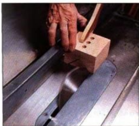
1 Set table-saw blade at 45° and align fence and blade height to produce a centered V-notch. Use pushstick for safety.
