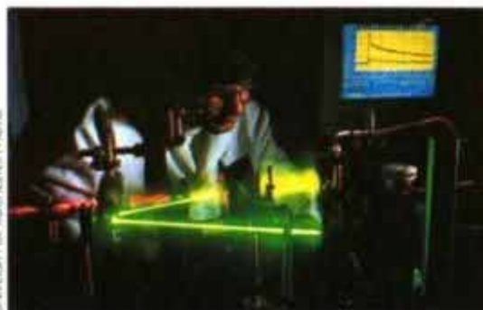
At a wavelength of 9.3 microns, pulsed laser anneals tooth enamel without zapping pulp.
