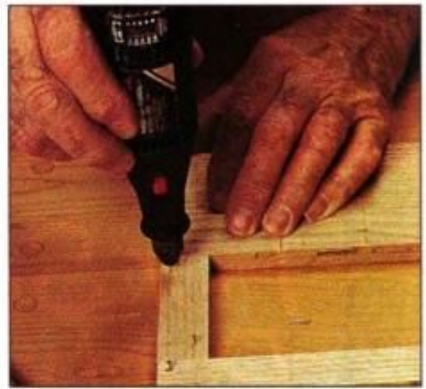
3 After applying glue, secure the upper- and lower-frame halves with nails. Bore pilot holes to avoid splitting the wood.
