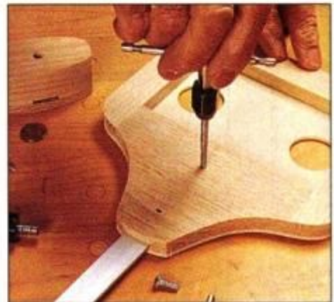
5 Attach an aluminum-strip pivot bar to the platform with screws threaded into tapped holes in aluminum and wood.
