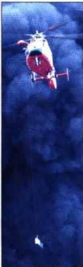
Helicopter swings airborne emissions monitor over burning oil slick during field tests.
