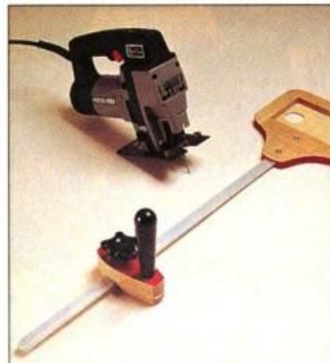
6 Twin blade holes in platform allow cutting in both directions. Locking pivot block slides on bar to adjust circle radius.
