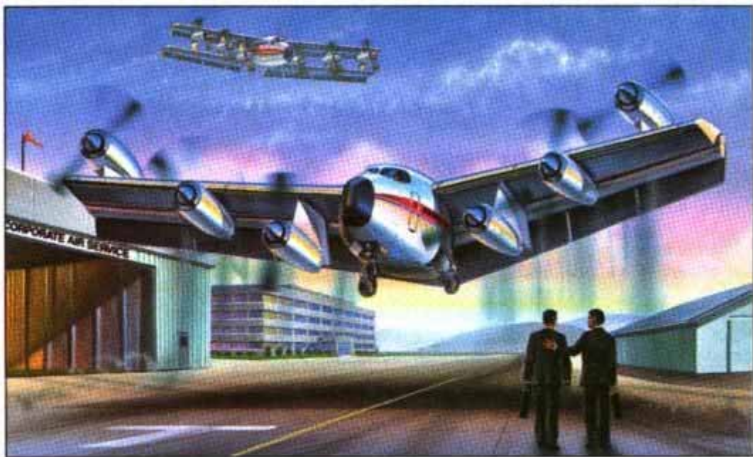
The EGR flying wing takes off vertically and can carry between four and nine passengers.
