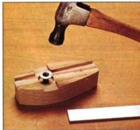
4 After cutting grooves in pivot block, bore Teenut hole and recess. Then, tap the Teenut in place with a hammer.
