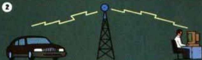
The motorist pushes the Lincoln RESCU button inside the car to initiate a cellular call. As part of the call, vehicle location and owner data are relayed to the Lincoln Security Center.
