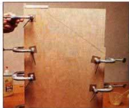
2 Glue and clamp each of the edge bands to the panels. Note that the top edge band of the end panel is just slightly long.
