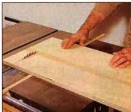
1 Tack nail a strip to the back of each panel. The strip should ride in the miter gauge groove as the panel is being cut.
