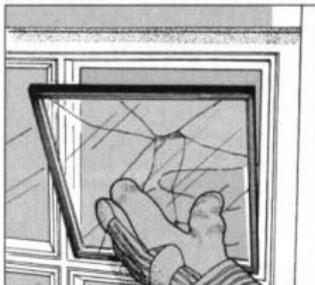
16 After cutting the seal between pane and wood, press glass away from the frame. Helper inside catches the pane.
