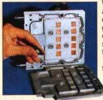
Flow boiling whisks heat from avionics modules recently designed at Purdue University.
