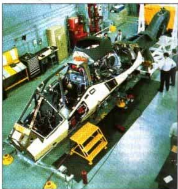
Mating of forward and aft fuselage sections means that the Comanche can accept engines and rotorblades.
