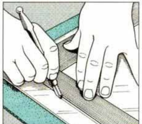
6 Use a straightedge and glasscutter to cut the glass. Lubricate the cutter wheel and score the glass with only one pass.
