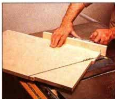
3 Using the miter gauge, cut the sloping edge on the end panels. Afterward, apply edge banding to the sawn surface.
