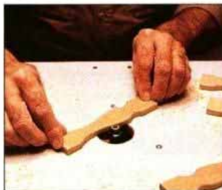
5 Since the splats are so small, it's best to round over their edges on a router table. A ball-bearing bit usually works best.
