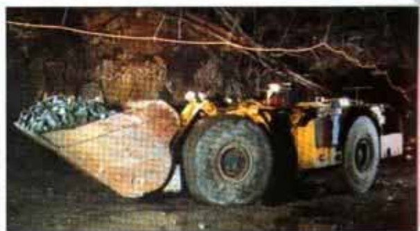
A semiautonomous robotic scoop tram ferries 12-ton loads of rock between the mine face and a crusher.
