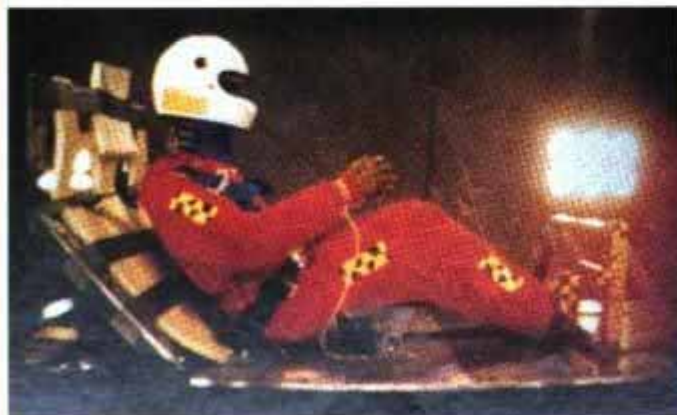
GM did crash testing, using a helmeted dummy in a mock race-car cockpit, to determine driver stress loads in a race crash.
