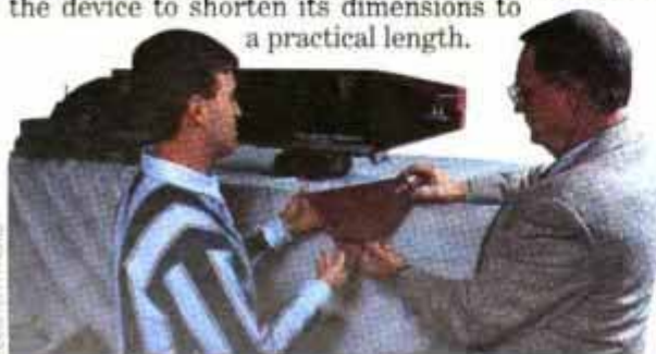
Inflatable truck boattail reduces aerodynamic drag.
