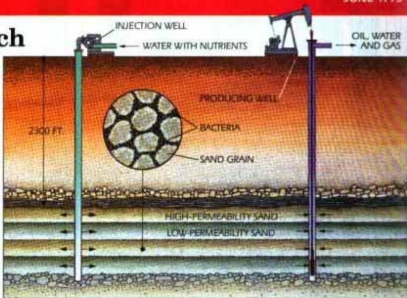
Fed nutrients, bacteria grow and divert water into low-permeability sand layers.
