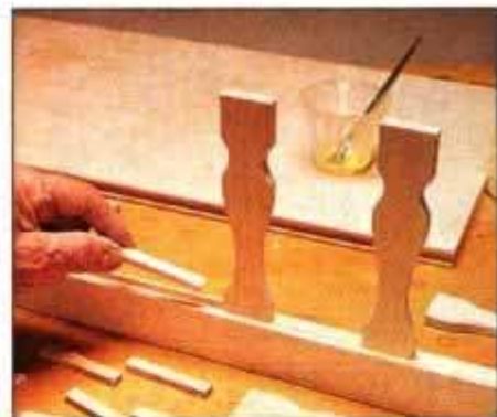
6 Insert the splats and spacer blocks in the top rail. After the glue has dried, repeat the procedure on the back panel.
