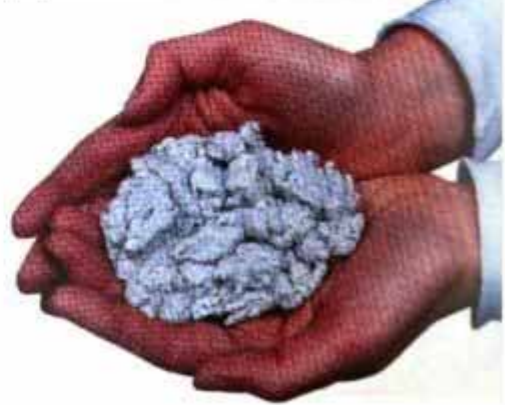
Clean pulp is ready for paper machine.
