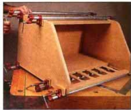
8 Clamp the chest using five bar or pipe clamps. Be sure to check the assembly for square before allowing the glue to set.
