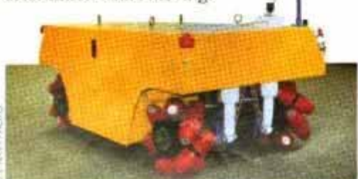
Omnidirectional robot pirouettes on wheels ringed with canted, keg-shaped rollers.
