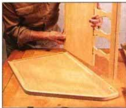
7 Begin the assembly by inserting the back into an end panel. Next, add the bottom and front, then the other end.
