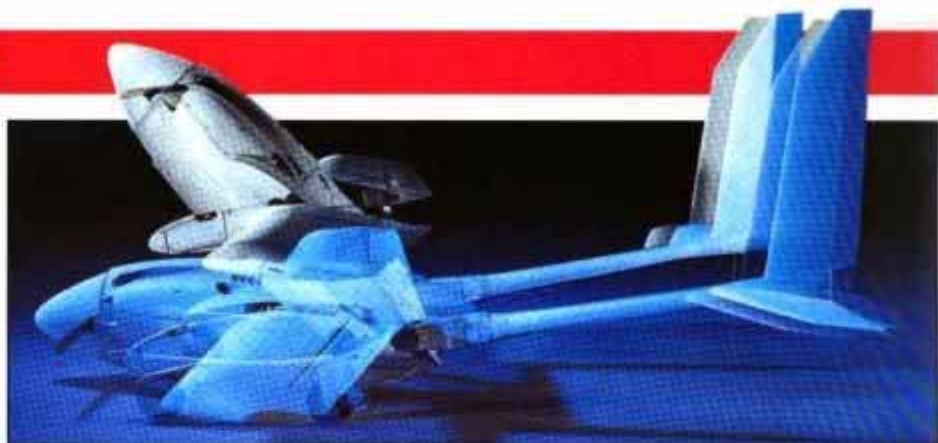
A free-wing tilt-body can cock its fuselage to vector thrust from the propeller.
