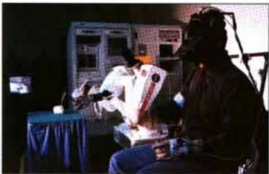
DART robot mirrors the motion of its teleoperator.
