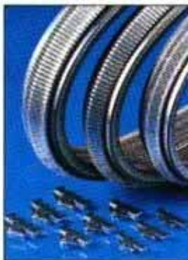
Steel belt, with elements linked by bands, enjoyed success in Canon-Williams Formula One racer.
