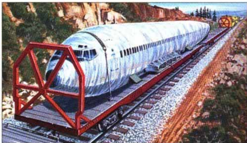
Resting on special mounts, fuselage of 737-700 will travel by rail between Boeing factories.
