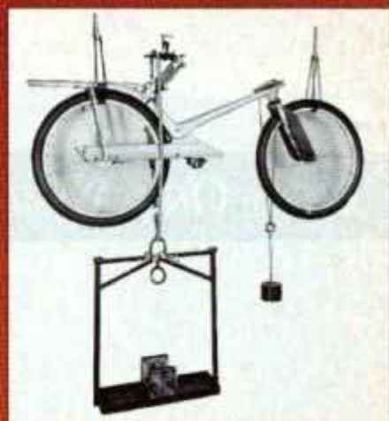
The way Aerocycle stress tests were conducted nearly 40 years ago.
