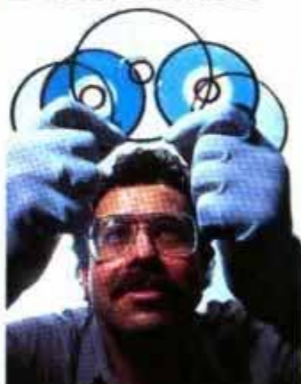
Multilayer optical disks use partially transparent storage material to boost capacity.
