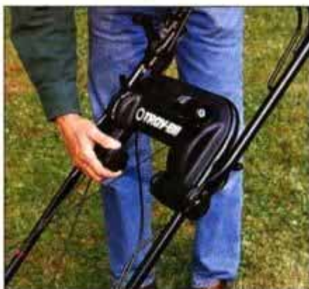
Troy-Bilt's handle turned out to be the most adjustable. It uses a rotating, geared knob assembly that's simple to change.
