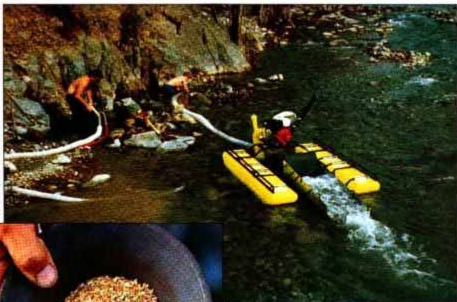
The pan still works, but mechanized gold recovery calls for gear such as this dredge on pontoons.
