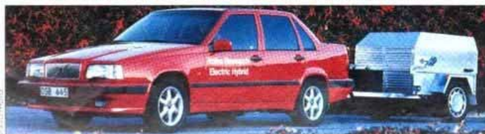
The hybrid electric Volvo 850 testbed hauls its generator in a separate trailer.
