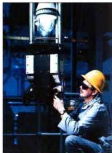
Engineers will install dual cameras in six Hanford nuclear-waste tanks.
