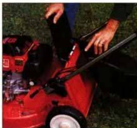
To convert the Kubota to side discharge, all you have to do is lift the back hatch and then slide in a curved discharge port.
