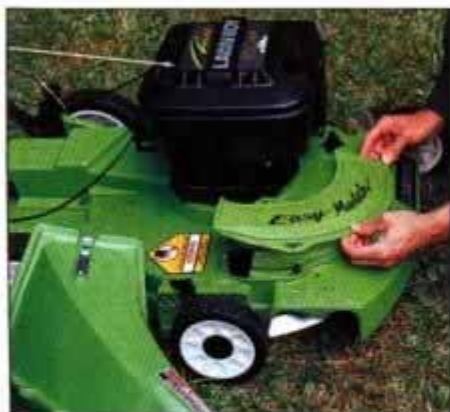
Lawn-Boy's discharge chute and mulching plate slide into place with very little effort. Parts are accessible on the mower deck.
