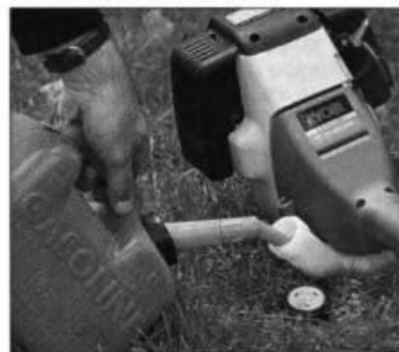
1 The 4-cycle engine takes straight gas for simplified fuelling. Fill spout is easy to access with trimmer resting on ground.
