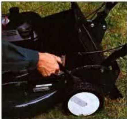
The Murray's single-lever height adjustment was the easiest to use of any of the 11 mowers that we put to the test.
