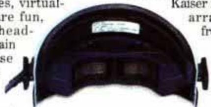
High-resolution wide-screen virtual-reality displays use three LCDs per eye.
