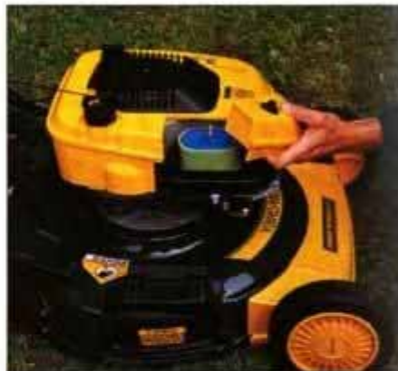
Yard-Man's air-filter cover is well located and easily removed. These design attributes make it easy to clean or replace the filter.
