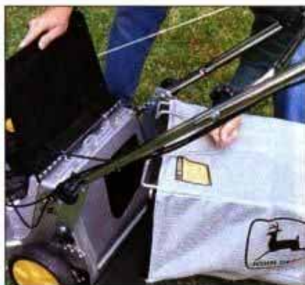
Deere's top-handled grass bag is easy to use. The bag hangs off the mower's back, right under the spring-loaded hatch.
