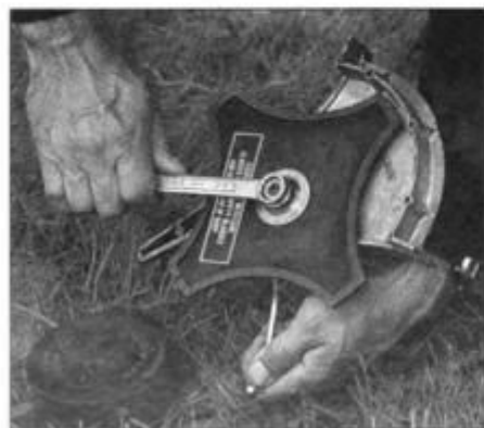
2 To switch from trimming to brush cutting, simply remove the shroud and replace the trimmer head with the brush blade.
