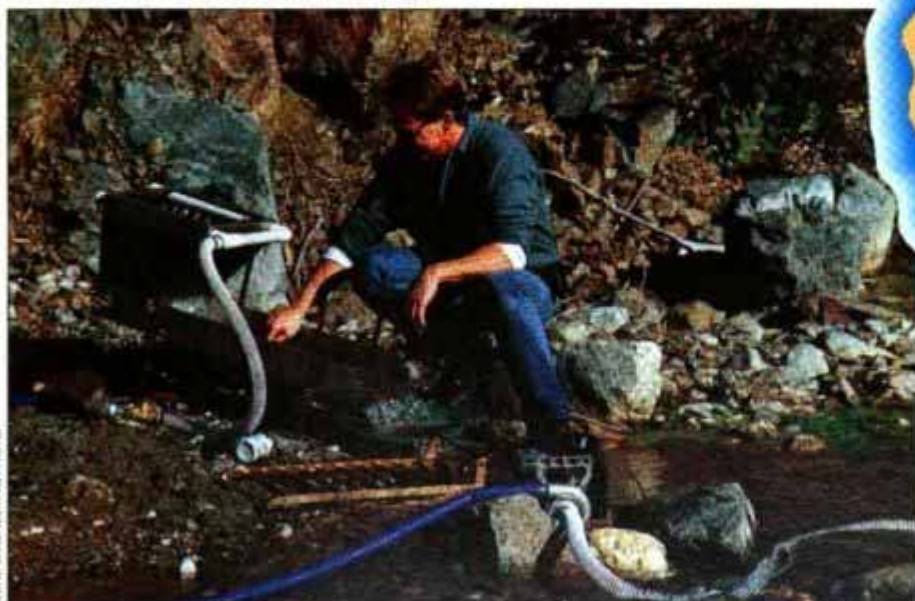
Magnetite deposits, or black sands, are dredged and passed through a sluice box.
