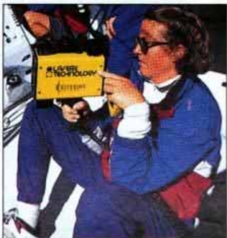
Laser/GPS gun gives speed/position data.
