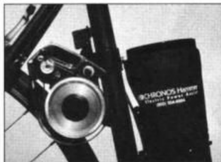
The compact Chronos Hammer delivers electric power to bikes.
