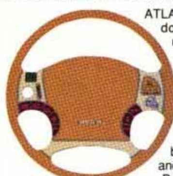
Alcohol-monitoring steering wheel sets off car alarm if driver is drunk.
