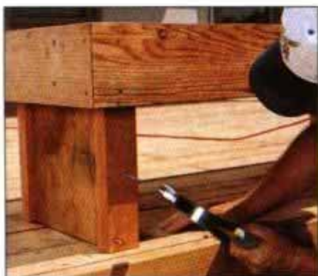
16 Finish the legs with 2 × 3 vertical trimpieces. These pieces hide the leg screws and give a more substantial feel.
