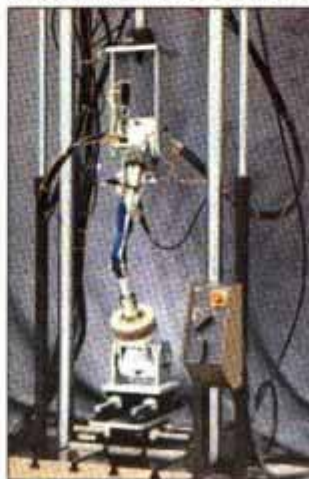
Knee simulator (above) and lower-jaw loader (right) measure durability.
