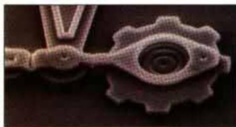
Linkages move up and down and left and right to spin minute gear at 500,000 rpm.
