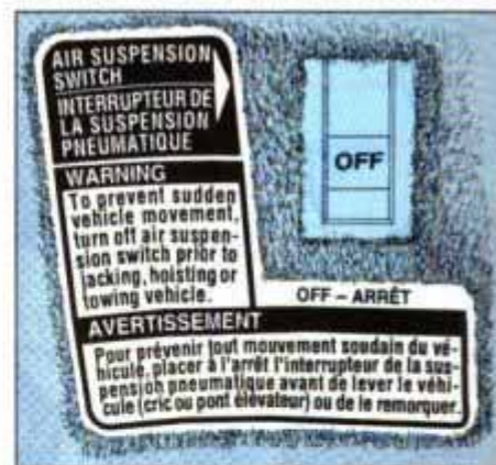
Air suspension must be off before jacking up Lincoln Town Cars or Mark VII/VIIIs.
