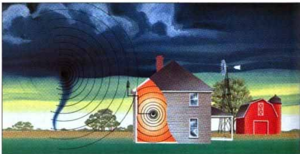
Tornado alert recognizes trait frequencies of approaching storm and triggers high-decibel alarm.
