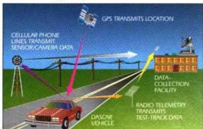
DASCAR will try to prove that a car's position and distance from other cars can be recorded, for future crash-avoidance systems.
