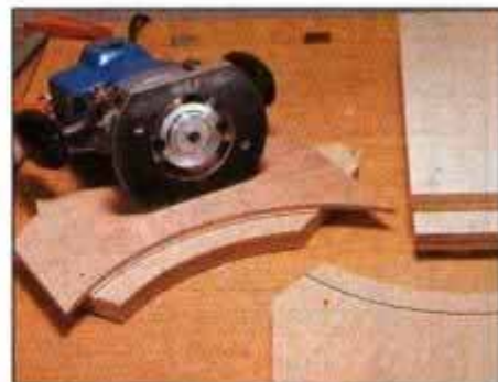
8 Use a router, guide bushing, template and veining bit to cut strip clearance grooves in retainer pieces and turntable.
