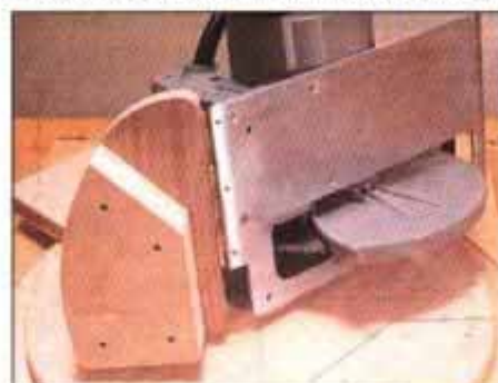
11 After securing hinge to saw mounting block, refasten it to saw base. Angled mounting block provides workpiece clearance.
