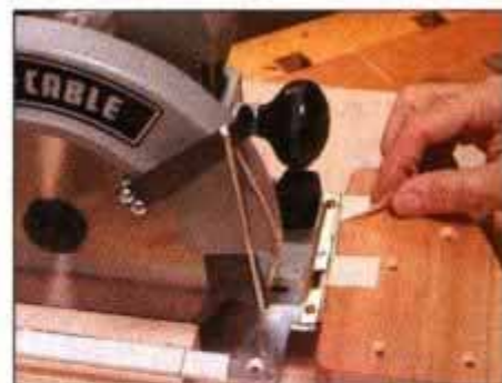
10 After placing saw and gauge block on turntable centerlines, tape free leaf of hinge to saw support. Remove hinge from saw.
