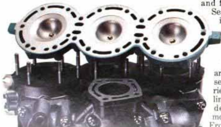
The 900 ZXi's triple has machined combustion chambers.
