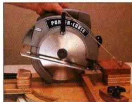
18 Tie string from screweye to guard lever. Adjust it so blade guard retracts properly as the saw is lowered.
