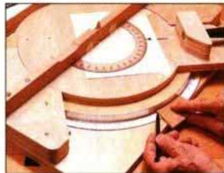
14 Tape protractor to fence. Mark on paper shows turntable angle. Align marks on scale with index scribed on aluminum.
