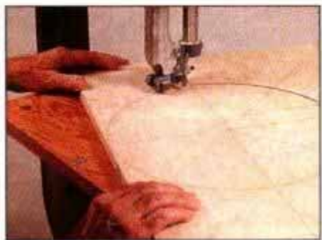
3 Cut circular pieces with a bandsaw or sabre saw and circle-cutting jig.
