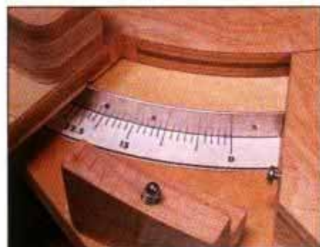
17 After enlarging detents with ¼-in. bit, enlarge click-stop block guide hole to accept spring and ¼-in.-dia. steel ball.
