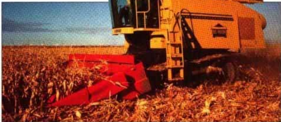
Bi-Rotor's compact thresher means the grain tank can be twice as big as normal.
