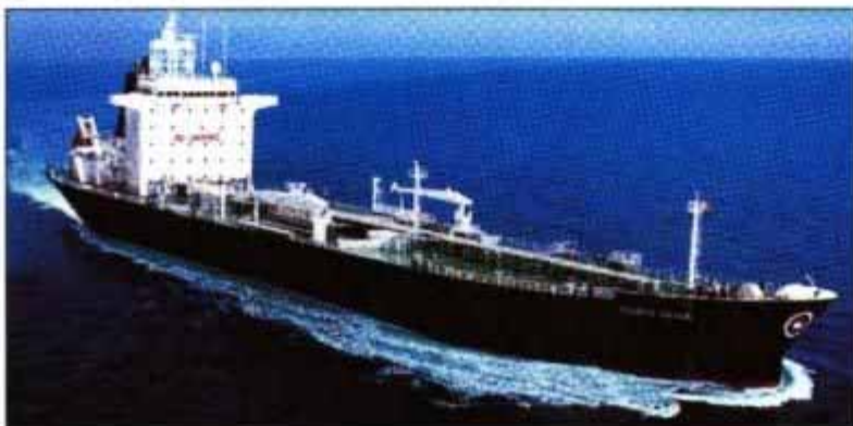
Double Eagle tanker carries up to 56,000 cu. meters of oil.
