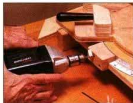
16 Use ⅛-in. hole in click-stop block to guide drill in starting detents. Place a detent at common miter settings.
