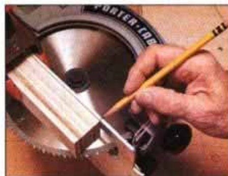
9 With saw blade extended, align corner of 1 3/16-in.-thick gauge block with blade edge. Then, mark block position on base.
