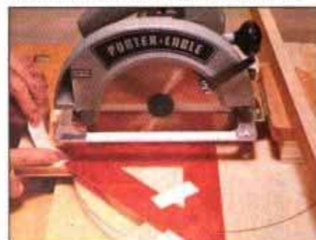
12 Secure mounting block and check that blade is square to centerline. Butt fence against square and install.
