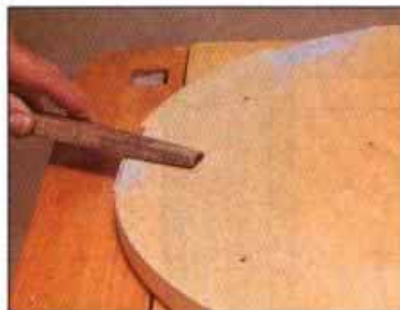
7 Width of aluminum strip is slightly greater than plywood thickness. Use a file to trim flush to surface in setback areas.
