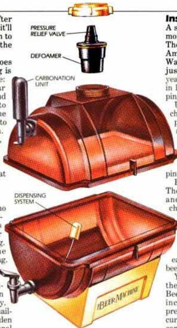
The 2.6-gallon Beer Machine is easily assembled. Note the CO 2 dispenser, which lets you vary the amount of carbonation.
