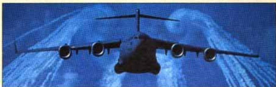
C-17 launches flares designed to camouflage plane from heatseeking missiles.
