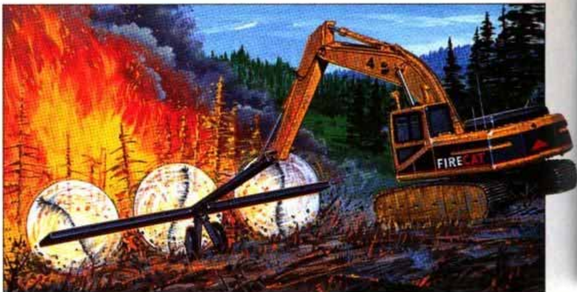
Firecat shreds burning debris, halting spread of flames by disrupting combustion.
