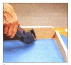
Sanding to a corner between wood and plastic laminate leaves the laminate unmarred while smoothing the wood.
