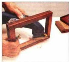
4 Dried glue on inside corner of frame is quickly removed. Small 1/16-in. orbit action produces swirl-free surface.
