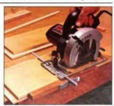
14 Use a rip fence accessory to guide portable circular saw when making rabbet shoulder cuts parallel to the grain.
