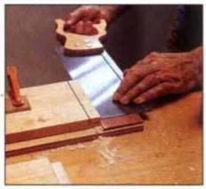
3 To cut a rabbet, first make the shoulder cut. Then, rest the saw horizontally on a quide block and saw away waste area.
