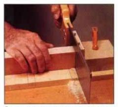
1 Cut dado shoulders with a backsaw. Use a block to keep the saw aligned. A second block acts as depth stop.
