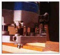
15 For fast rabbeting along straight and contoured surfaces, use a router and a rabbeting bit with ball-bearing pilot.
