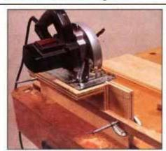
13 Build an L-shaped jig and attach it to saw base to give extra support when making rabbet cuts from stock edge.
