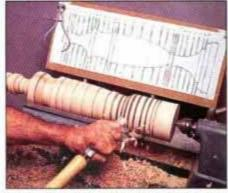
7 The gouge quickly removes waste between the sizing grooves. Once the waste is removed, the turning is roughly formed.
