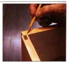
18 Use the grooved piece to lay out narrow dado in second mating piece. Align inside of groove with end of mating piece.
