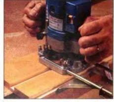
Rout grooves parallel to the grain with a router fence. Where a fence won't reach, clamp a guide strip to the work.
