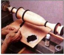
11 Run the lathe at low speed, and use a foam brush to apply acrylic paint on the beads. Steady the brush with both hands.
