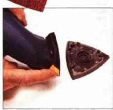
2 To rotate pad, press button at front, remove pad, turn and reinstall. Rotating pad distributes wear on sanding sheet.
