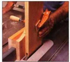
17 Begin combination joint by cutting grooves in end of the first workpiece. Clamp work to Jig that straddles saw fence.
