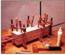
2 Push a ramrod down the center of the turning blank. This pushes out the glue that has squeezed into the hole.
