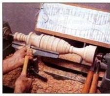
Use the round-nose chisel to dress concave curves. Move the chisel in an arc by pivoting it against your thumb.
