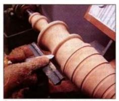
9 The diamond-point chisel forms smallradius beads. The convex curves can be formed with this tool or a skew chisel.
