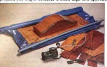
utilizes a heavyduty  $54 \times 54$ -in. vinyl bag and pump to apply 1700 pounds of uniform pressure. It's especially useful on curved substrates. The Vacu-Press costs about \$325 from The Woodworkers' Store. 21801 Industrial Blvd., Rogers, MN 55374.
