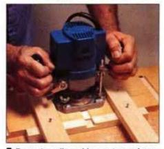
5 Frame-type jig guides router and constrains dado width. Initial cut through jig crosspiece helps in aligning jig.
