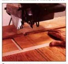
S Install dado blade in radial-arm saw and make initial cut through new fence. Use resultant notch to align work.
