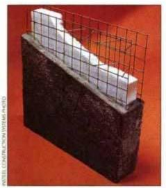
5 These polystyrene panels have built-in reinforcing mesh. A sprayable concrete is applied to both sides of the forms.
