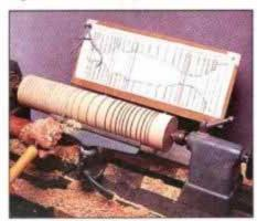
6 A parting tool can get quite hot when cutting deep sizing grooves. Widen these grooves to avoid overheating the tool.
