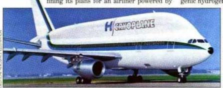
hydrogen (see "The Hydrogen Age," page 21, Sept. '90). Together with other German aerospace firms and Tupolev and TRUD of Russia, the planemaker has conceived Cryoplane, so called because it would carry cryogenic hydrogen as fuel. The concept poses challenges. Not
