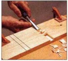
2 After cutting the shoulders, remove the waste with a chisel. Work from the ends toward the center to avoid splintering.
