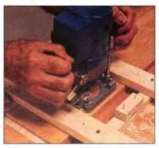
6 To rout a stopped dado, tack a stopblock to the frame Jig crosspiece. After cutting dado, square blind end with a chisel.
