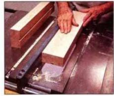
1 Use a dado blade in the table saw to cut the groove in the center of each half of the turning blank.
