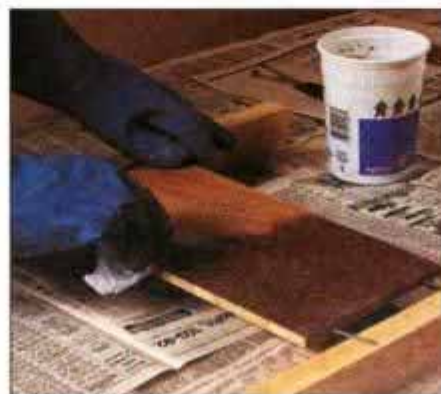
13 Apply warm water to raise grain, let dry and sand. Then color the panels with aniline dye according to the instructions.
