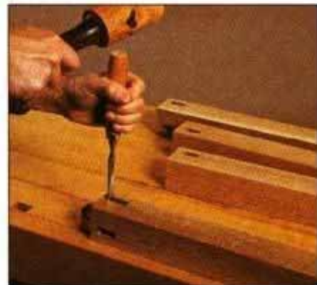
4 After the mortises have been routed, use a sharp chisel to square the mortise ends so the rail tenons will fit snugly.
