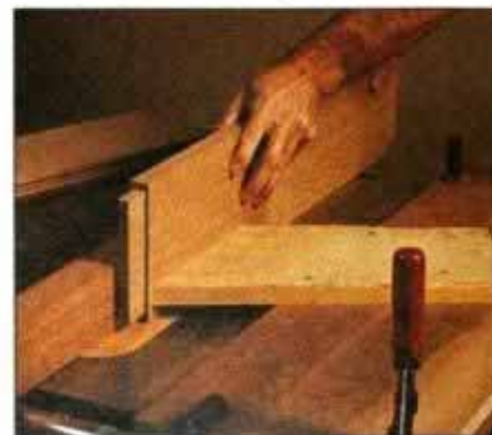
7 Reset the dado blade, and cut the grooves for the panels and the stiles. Use a featherboard to hold work against fence.
