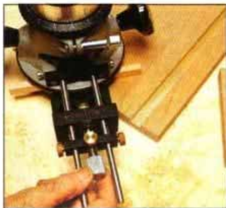
1 The fence excels at guiding groove cuts to fit plywood parts. These parts are often thinner than their nominal dimension.
