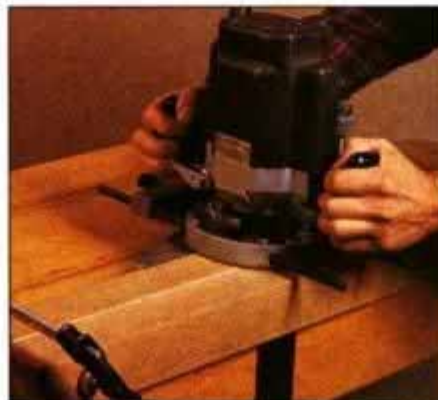
3 Use a plunge router and edge guide to cut the leg mortises. Spare leg clamped to side of workpiece helps support router.
