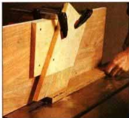
1 Rip the mitered leg sides on a table saw. A featherboard clamped to the fence holds stock for a smoother, more accurate cut.
