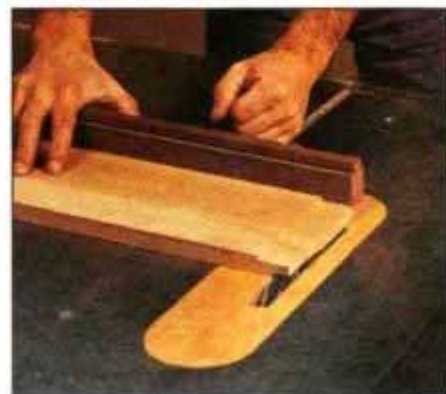
5 Use a dado blade to cut the tenon faces on the rail ends. A stopblock clamped to the table ensures consistent tenon length.
