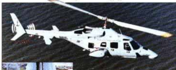
Bell turned Model 230 into a naval chopper sporting nose-mounted radar.
