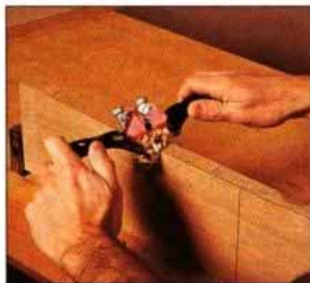
10 Smooth the curves to the layout line with a spokeshave. Cut down the curve from each end to avoid tearing the wood.
