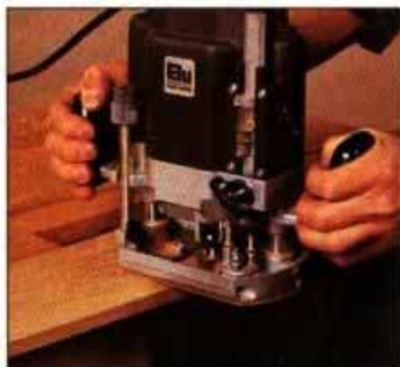
11 Rout a chamfer along the top front edge of the front rail. Use a 30° chamfer bit with a ball-bearing pilot for the job.
