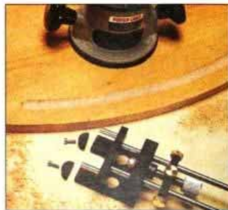
3 To do routing along curved edges, use the half-round plastic inserts. These are attached with screws to the main fence.
