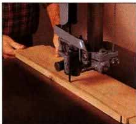
9 Use a band saw or sabre saw to cut the curve on the lower rails. Stay just to the waste side of the layout line.
