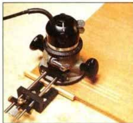
2 The Micro-Fence guide is a boon for cutting accurately spaced grooves, and its low-profile fence helps on thin stock.
