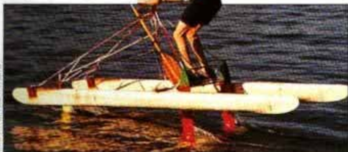
Pogo Foil can hit 11 mph driven by flapping of submerged wing. Smaller front foil allows turns.
