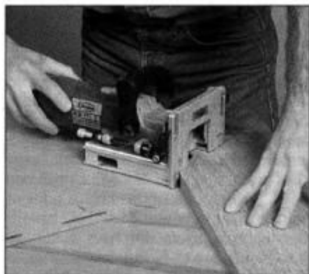
16 After mitering the arm pieces, use a plate joiner to cut the slots for joining the components with plates (biscuits).
