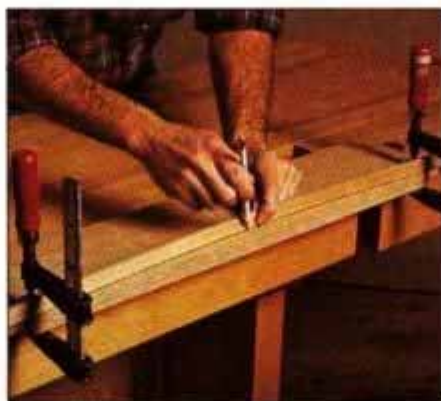
8 Bend a thin strip over the lower rail pieces to lay out a smooth curve. Clamp the strip at ends and trace curve with a pencil.
