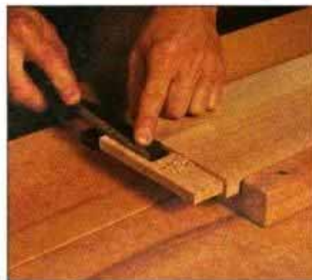
6 After cutting tenons slightly oversize, use a chisel to pare them for a snug fit. Paring also removes dado blade marks.
