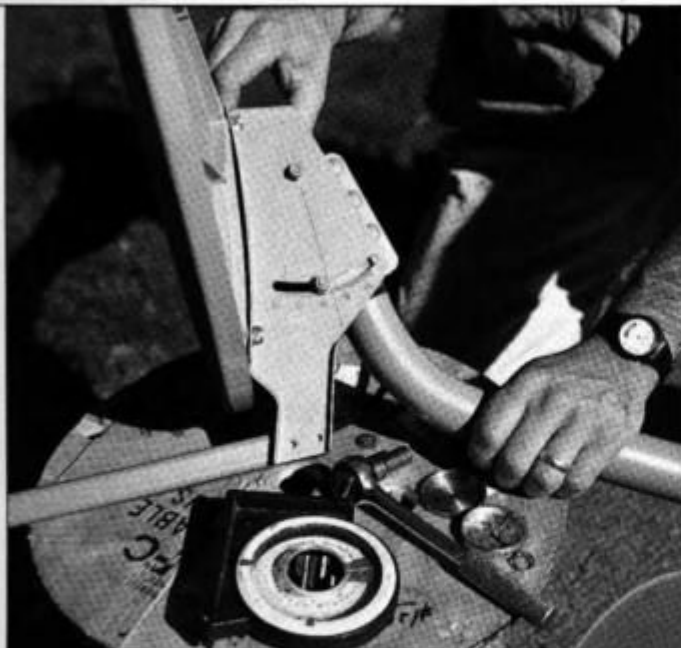
Indicator scale on LNB support arm has tick marks in degrees to set the angle of elevation correctly.
