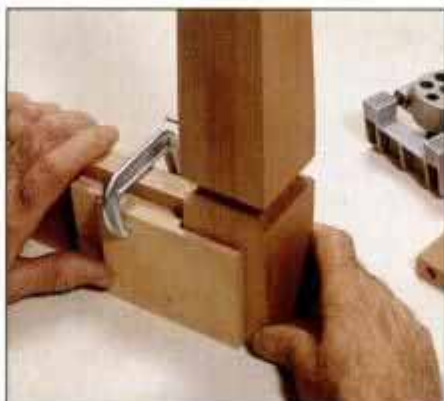
8 Press mating pieces together to mark holes with dowel centers. Shims clamped to work sides control alignment offset.
