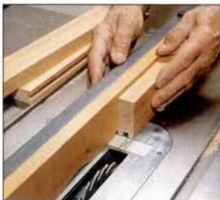
10 Use a dado blade for tongue-and-groove joints. First cut makes groove. Making the tongue requires two cuts.
