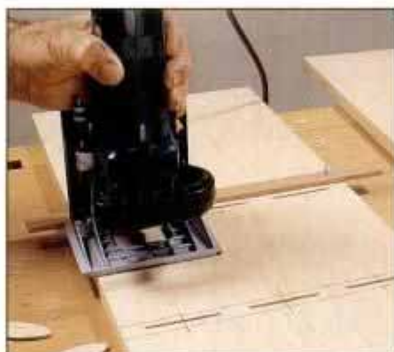
20 Use a plate joiner for fast assembly of shelves and side panels. First cut slots in sides, then matching slots in shelf ends.
