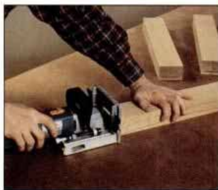
10 Mark the curve on the backrest slats, and mark the biscuit location. Cut the biscuit slots using a plate joiner.
