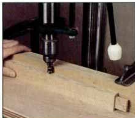
17 Bore and counterbore pilot holes for attaching the ottoman's slip seat. Use the drill press or a doweling guide to do this.
