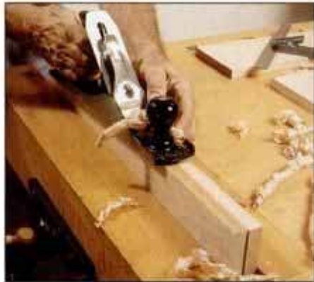
1 Fold workfaces together and plane the edges. Planing angle doesn't affect parallel alignment of faces when boards are joined.
