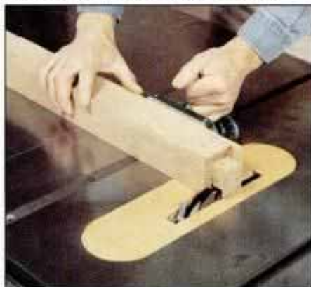
3 Using a miter gauge, cut the tenon on the leg with a dado blade in the table saw. Bevel the tenon end with a chisel.
