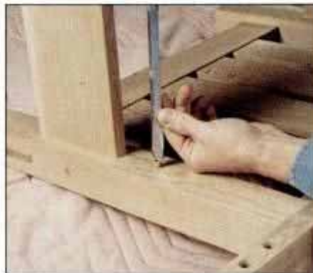
15 Bore holes, and install the threaded inserts in the rear legs. Lubricate the inserts with wax before installing them.
