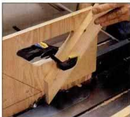
18 Use a jig to support workpiece when cutting spline slots parallel to face in end of miter joint. Use two splines per joint.
