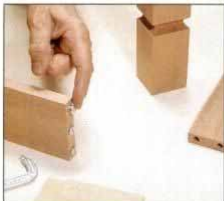
7 For unaligned dowel joints, place dowel centers in dowel holes in preparation for marking adjoining hole positions.
