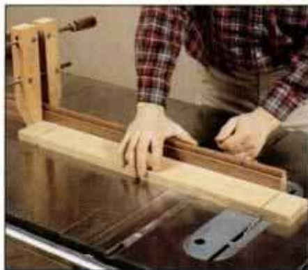
5 Attach an extension fence with a stop to the miter gauge, and cut the tenon shoulders on the front and back rails.
