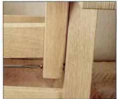
16 Drive a machine screw through the backrest side and into the insert. Use three washers between the leg and side.
