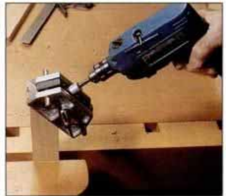
6 Use a doweling jig to bore holes for miter joints. Use a depth stop or masking tape around bit to gauge hole depth.
