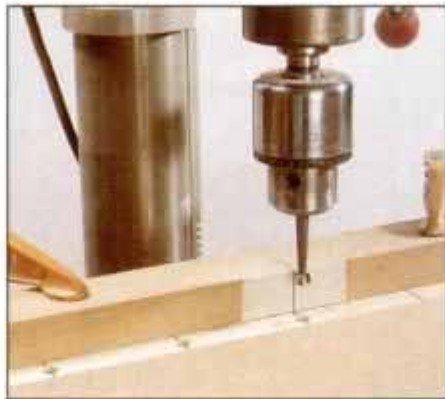
5 To bore dowel holes on a drill press, set up fence and position for centered hole. Align holes with index mark on fence.
