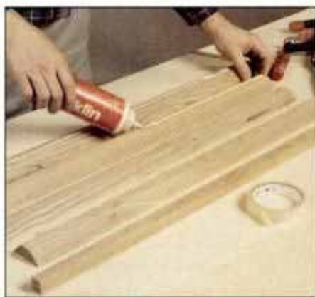
1 Each leg is an assembly of four beveled pieces glued to a core. Spread a thin film of glue on each bevel and each core.
