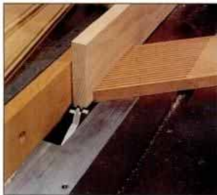
13 Use a featherboard to hold workpiece against wooden auxiliary fence when using molding head. Glue-joint cutter shown.
