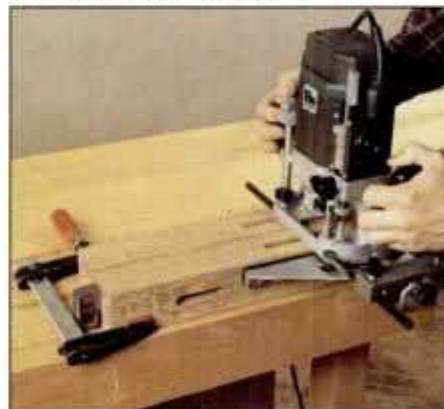
4 Cut the leg mortises with a plunge router. To provide adequate support for the router, clamp two legs together.
