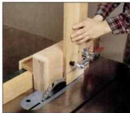
6 Next, attach an auxiliary fence to the table saw's rip fence, and use a tenoning jig to cut the tenon cheeks.
