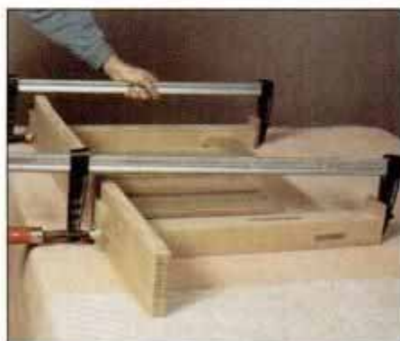
12 Glue and clamp armrests to the side assemblies. Use blocks to prevent marring and to spread clamp pressure.
