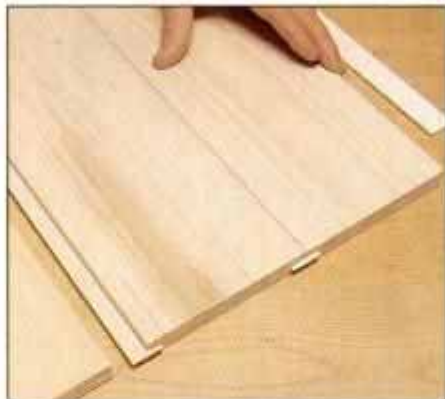
15 Referencing slot with same face of each board ensures alignment. Cut splines slightly narrower than double slot depth.
