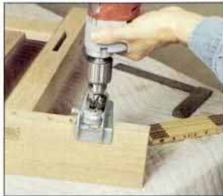
13 After the side-arm assembly is complete, use a doweling jig to bore holes for the backrest peg in each arm.
