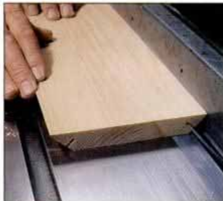
16 Use a table saw to cut kerf-width slots. Cut slots in miters with blade tilted to miter angle and slightly below center.
