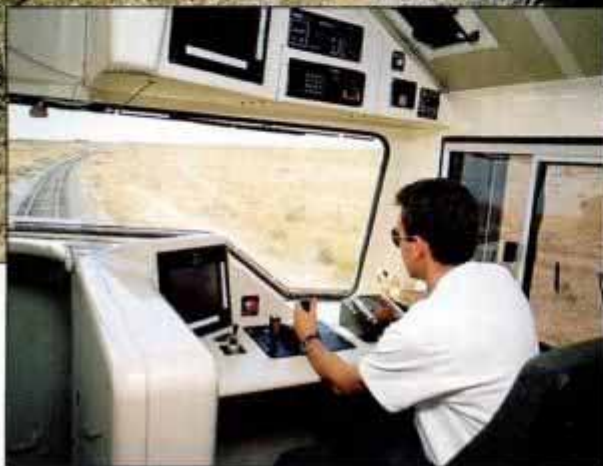
Throttle lies at engineer's left, while automatic and independent brakes are at right. Dynamic braking occurs when reverser key and throttle handle are shifted back.
