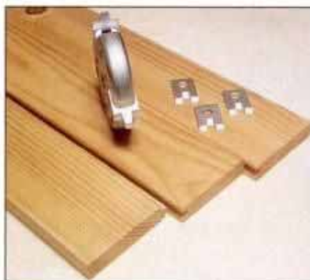
11 To make tongue-and-groove joints in two passes on a table saw, use a molding head with tongue-and-groove cutters.
