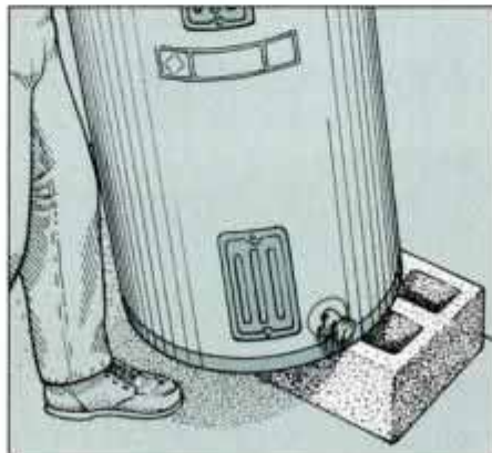
2 Slide the tank onto the blocks and center it. Align the drain toward the front and make sure the tank doesn't rock.
