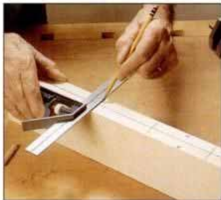
3 Place adjoining boards face to face, and use a square to mark dowel hole centerlines across both edges at once.
