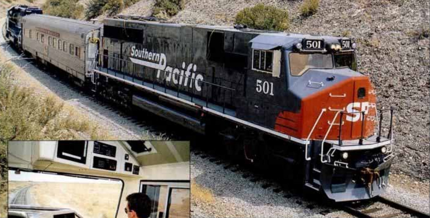
Throttle lies at engineer's left, while automatic and independent brakes are at right. Dynamic braking occurs when reverser key and throttle handle are shifted back.
