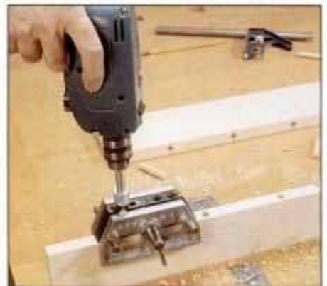
4 Align index mark on doweling jig with centerlines on stock edge and bore holes. Self-centering jig aligns hole across edge.
