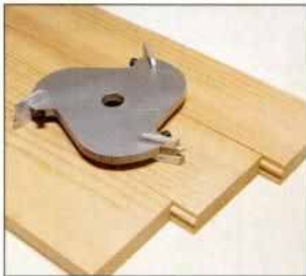
12 Glue-joint cutter in molding head shapes both sides of joint. Shaped glue joint increases glue surface area.
