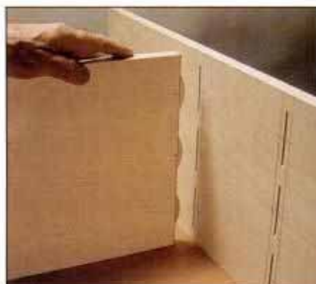
21 Apply glue to plate joint slots and install plates in shelf ends. Then, assemble components, adjust alignment and clamp.
