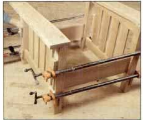
14 Glue and clamp the side assemblies with the front and back rails. Use two clamps at the front and back.
