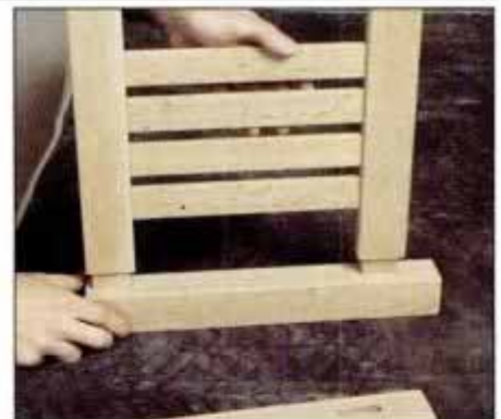
18 Begin the ottoman assembly by gluing and clamping the side rails to the slats. Then glue and clamp this to the legs.
