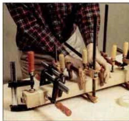
2 Tape the leg assembly together, then position closely spaced clamps around the assembly and let the glue set.
