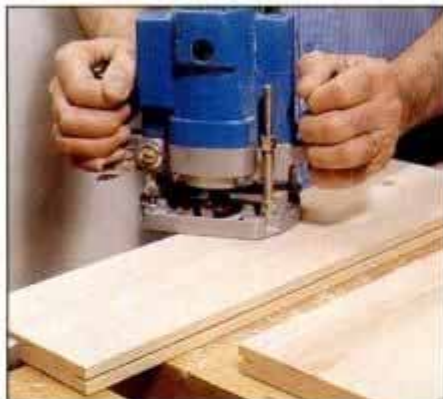
14 Use a router equipped with a winged slot cutter to make spline slots. Stop cut short of end for blind spline joints.
