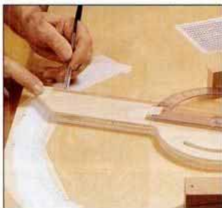
7 Install the fence and use it to mark the graduations in the recess. Use a protractor clamped to the fence to measure angles.
