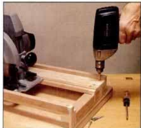
3 Use your saw to position right guide rail accurately. Then, bore pilot holes and attach right rail assembly with screws.
