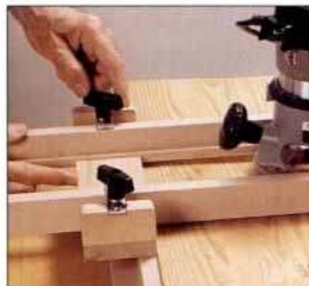
4 Position router carriage over L-shaped tracks and lock sliding joiner. Then adjust bit depth for shallow cut.
