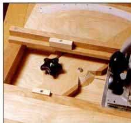
9 Install stops to limit forward travel of saw. Make blade-clearance cut in fence by repeating cuts through fence pivot range.
