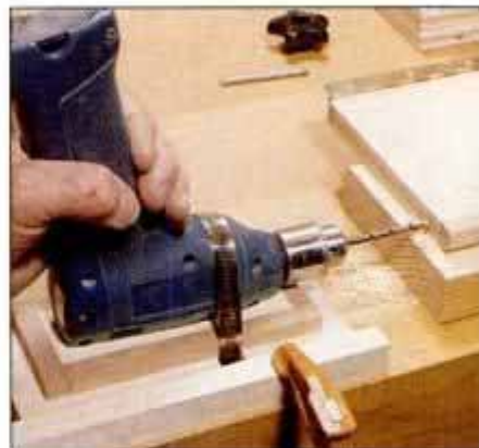
9 Use the drill carriage to bore accurate holes in the platform support piece. Guide carriage against strip clamped to bench.
