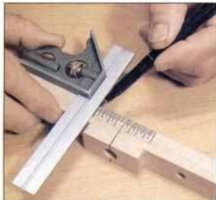
1 Use a black fine-point pen to mark the graduations. Make sure the graduations on each side are aligned accurately.
