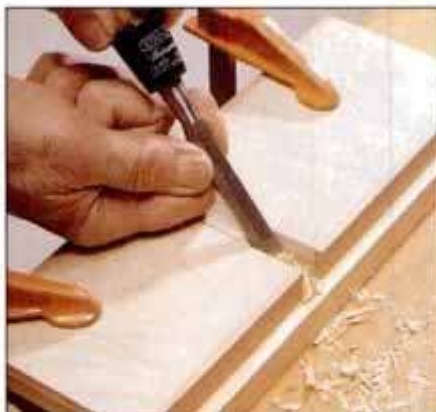
8 After sawing edges of hose clamp recess, use a chisel to remove the rest of the waste on the bottom of the drill carriage.
