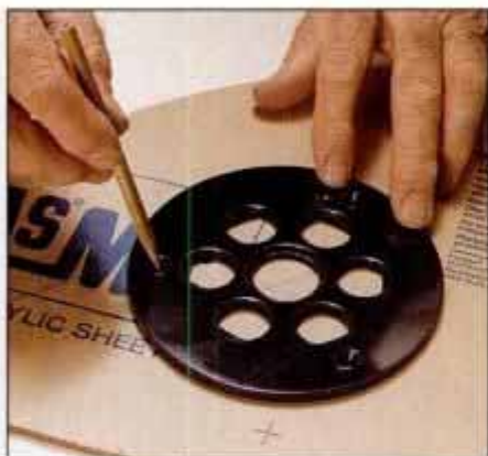
1 Remove the base from the router and use it to mark the screwholes and the router-bit hole on the acrylic sheet.
