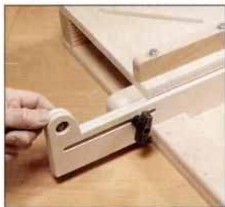
16 After making sliding support, install and check action. Curved edge supports platform pin at shallow height settings.
