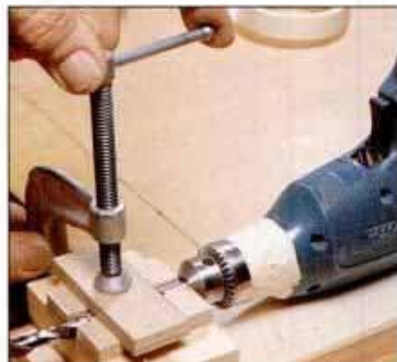
2 Install bit in drill and tape chuck so it won't turn. Then, clamp bit to support block to suspend drill housing over base.
