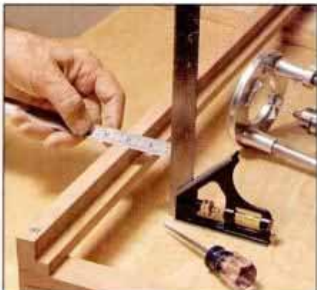
2 Mark kerf by measuring saw blade-to-base edge distance from left guide. Place pivot on kerf, 8 in. up from base edge.
