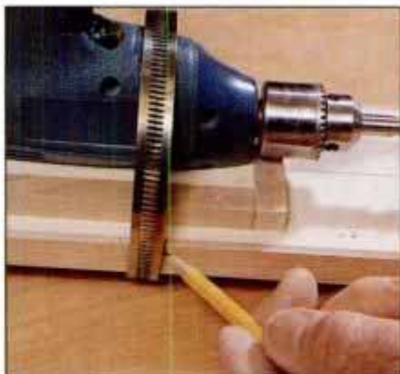
7 Align hose clamp with the section of the housing that affords the best grip. Then, mark the base for the clamp notches.
