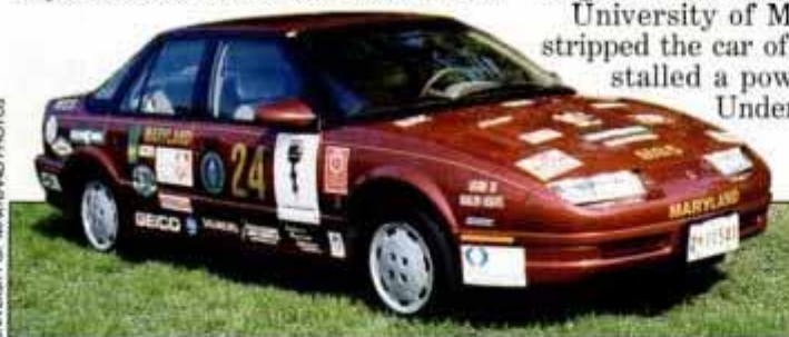
Hybrid Saturn uses a Geo engine to recharge batteries for its power-assisting electric motor.
