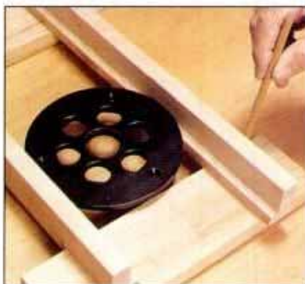
1 Make the carriage tracks and place them on the track joiners. Adjust spacing and then mark for joiner dadoes.
