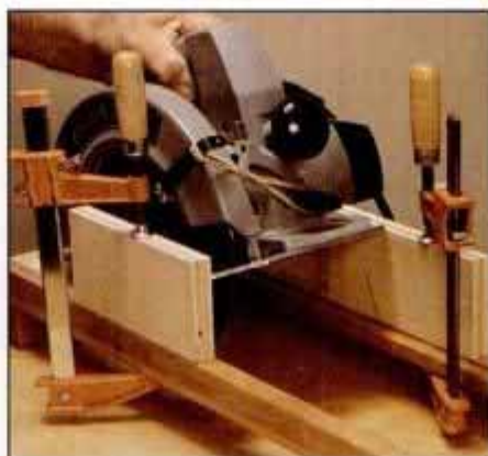
8 To make the kerf in the base, first clamp two temporary support walls to the rails. Lower the saw and move it along the rails.
