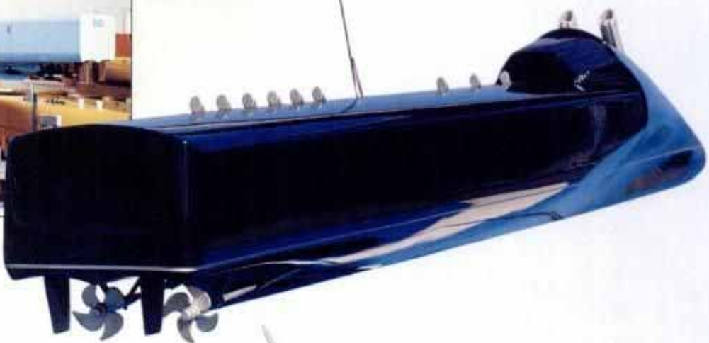
A 1/40-scale model Euro Express underwent development in a test tank to determine power requirements and seakeeping ability, or how the ship behaved in simulated rough-sea conditions.
