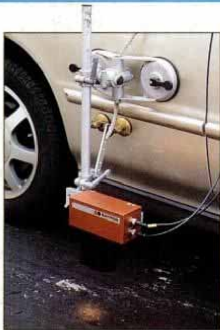
Datron Corevit optical sensor reads the texture of the road surface. The unit is more cumbersome than the radar gun.
