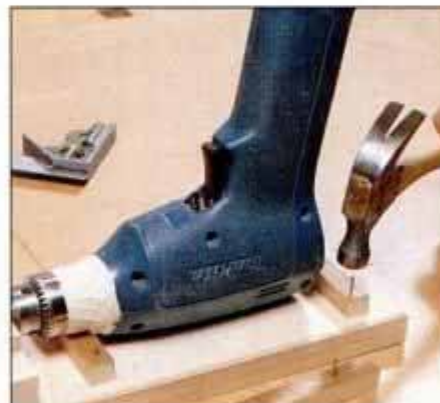
3 With bit clamped and drill handle vertical, nail enclosure strips around drill housing to contain filler that will support drill.
