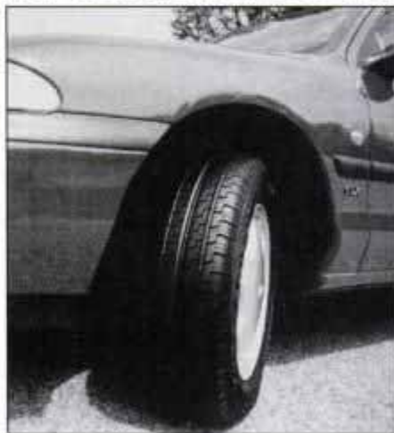
Blocky tread with wide grooves defines the new Pirelli P400 Aquamile rain tire.
