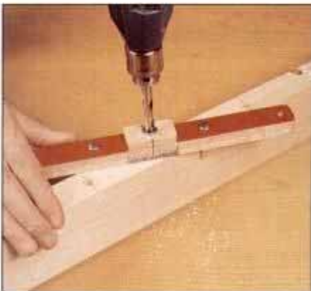
3 To use jig, install steel bushing to suit bit. Place jig over the work and bring the pins in contact with the workfaces.
