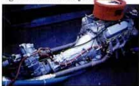
Ford truck engine, transmission and transfer case comprise the powertrain.
