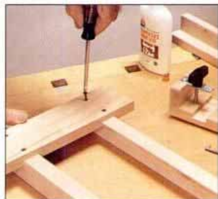
2 After the dadoes have been cut in the joiners, secure one joiner with glue and screws. Opposite joiner is adjustable.
