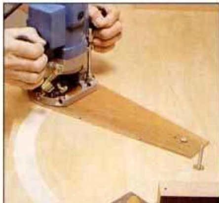
5 Use a shopmade guide to rout the recess for the miter scale. Guide has two pivot centers to rout recess in two passes.
