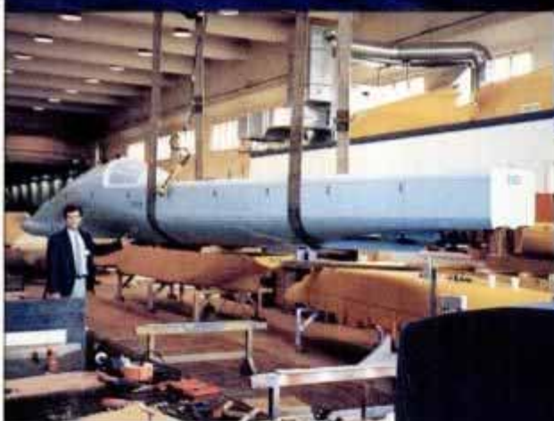
A 1/40-scale model Euro Express underwent development in a test tank to determine power requirements and seakeeping ability, or how the ship behaved in simulated rough-sea conditions.
