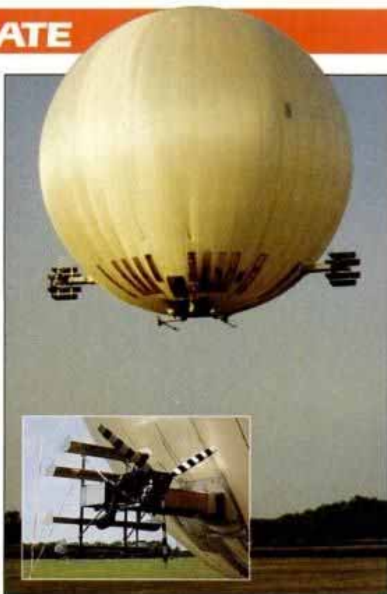
Stubwing-mounted engines and vanes allow blimp to assume spherical shape. Gondola is carried inside.
