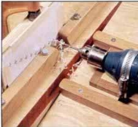
1 We used the horizontal boring jig to make this spacing jig. Change the hole diameter and spacing to suit application.
