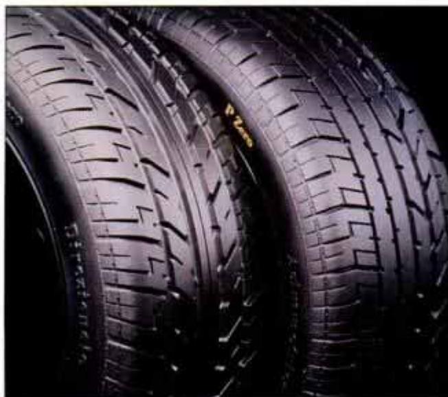
Tread is different on Direzionale (left) and Asimmetrico (right).
