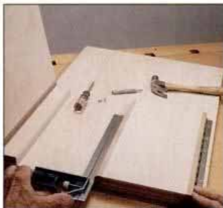
10 Secure platform support hinge with one screw. Check alignment with base and tilting platform. Install remaining screws.
