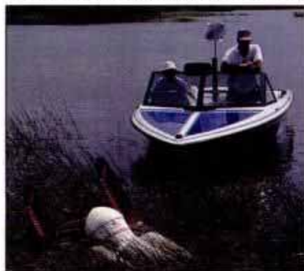
Fiberglass drone simulates a 165- to 170-pound slalom skier. Metal target in boat improves reading of radar signal.
