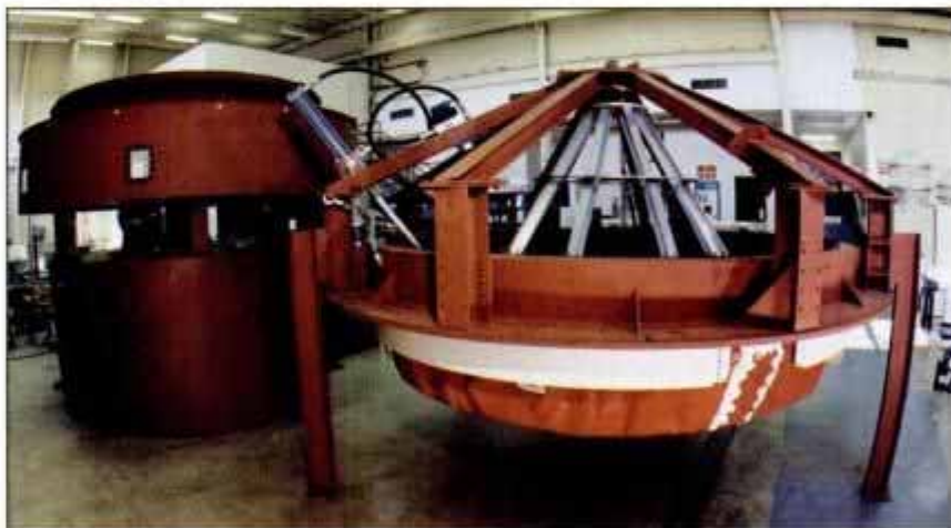
Heat shield peeks from under rig that simulates business end of a Titan IV booster.
