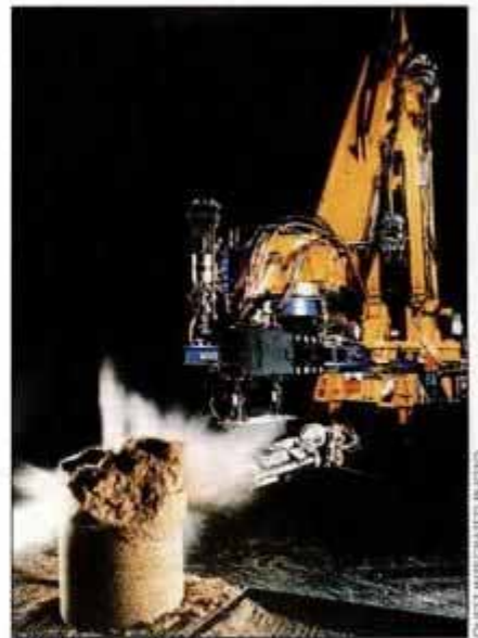
Hydraulic pulse generator shows how it could fragment rock-hard materials.
