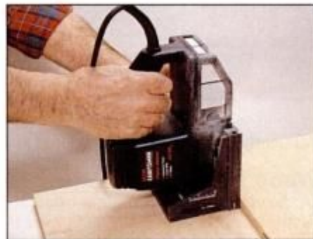
2 Remove the adjustable fence to cut plate joint slots that fall in the middle of a panel, such as in bookshelves or cabinets.
