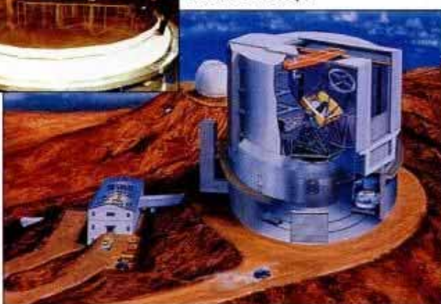
Sprawling mirror, only 9 in. thick, will reflect starlight in Japan's Subaru telescope.
