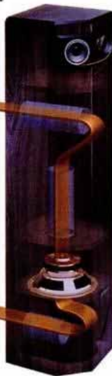
Both sides of the Bose 501's woofer (left and above) are used to generate more bass from a smaller space. The B&W Nautilus (top left) minimizes standing sound wave problems.
