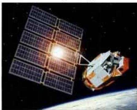
TRW's Lewis Smallsat will explore Earth with hyperspectral imaging.
