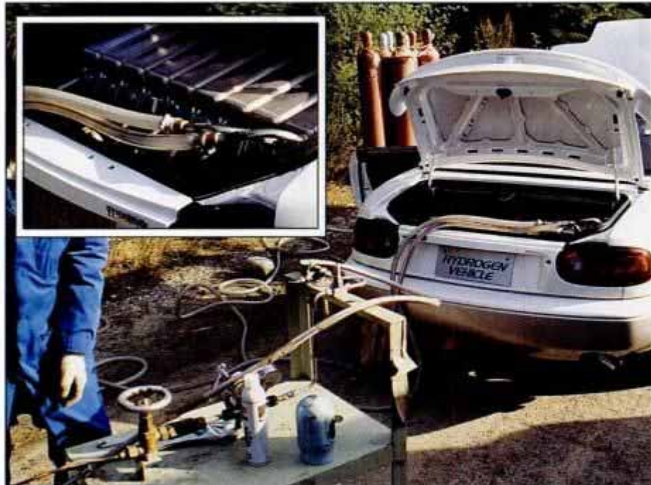
Metal-hydride fuel is stored in a suitcase-size tank (inset) that consumes the Miata's trunk. The refueling process is a slow one, and requires special equipment.
