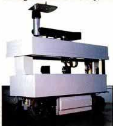
Tessellator will wheel beneath shuttle, expanding and contracting, to eye the spacecraft's underbelly.
