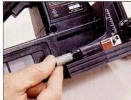
4 A knob on the side of the base controls cutting depth. Depth can be set at three preset positions for standard plate sizes.
