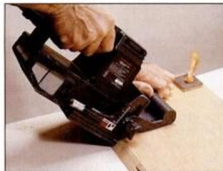
1 To cut plate slots in a miter joint, set fence at matching angle. Fence tilts up and down to cover a wide range of angles.
