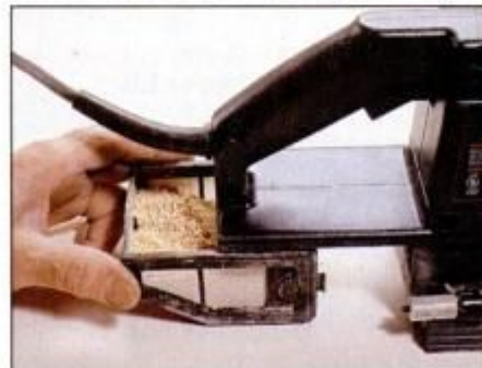
3 The Sears plate joiner has a dust-collection box mounted under the handle. To remove it, simply slide it back.
