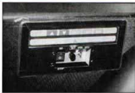
Peak Power controller and panel manage power from solar array and batteries.
