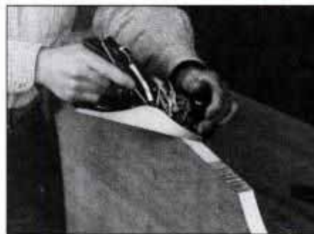
9 Saw the headboard to shape. Smooth away saw marks and refine the shape using a smooth plane and spokeshave.
