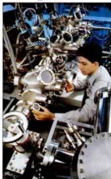
Molecular-beam epitaxy machine, which lays down one atomic layer at a time, makes zone laser.
