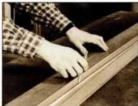
1 Rip and crosscut the post blanks, and use a long straightedge to mark the taper. Also mark the mortise positions.
