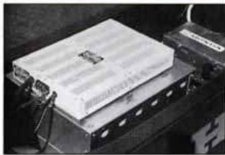
Peak Power controller and panel manage power from solar array and batteries.
