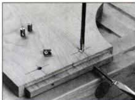
13 Bore 10mm holes for cross dowels in the back of the headboard. Turn the dowel to align its hole with the screw.
