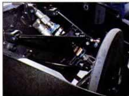
Ultra-lightweight suspension is faired in top and bottom to reduce aerodynamic losses.
