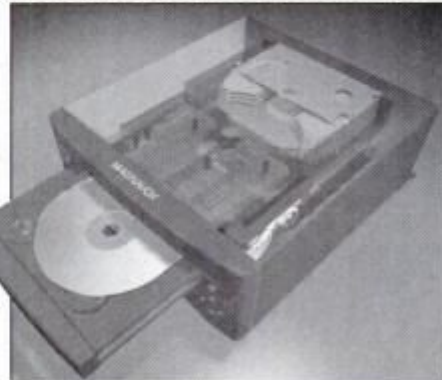
The elevator mechanism (below right) in Magnavox's micro FW14MX37 7-disc changer.
