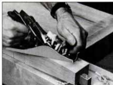
5 Smooth the sawed surfaces and refine the taper with a hand plane. Set the plane to take a fine shaving.
