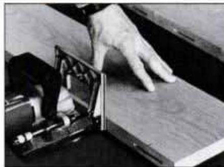
7 Rip and crosscut the headboard stock oversize. Cut joining plate slots in the stock, then glue and clamp the stock.
