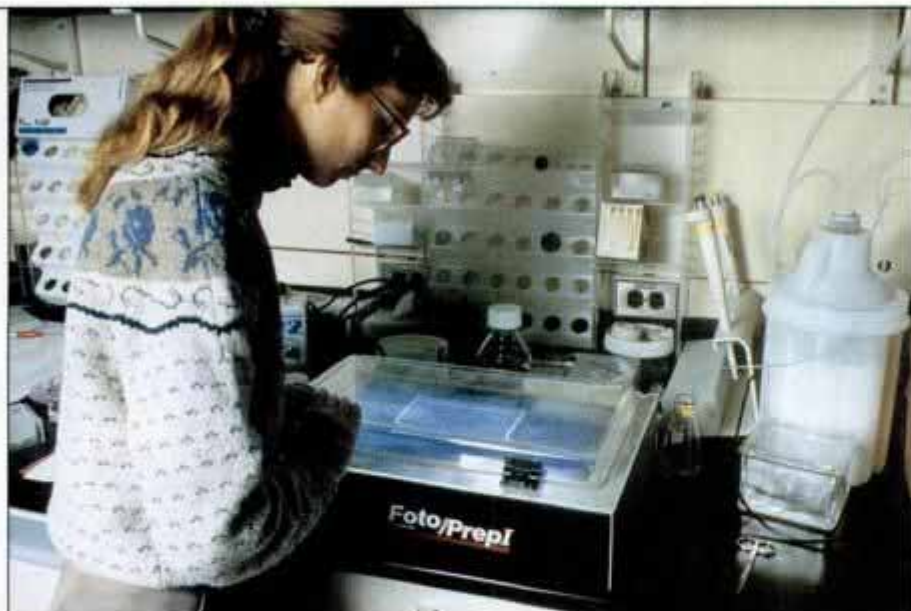
Transilluminator used in DNA identification emits UV light, which makes dyed DNA glow.
