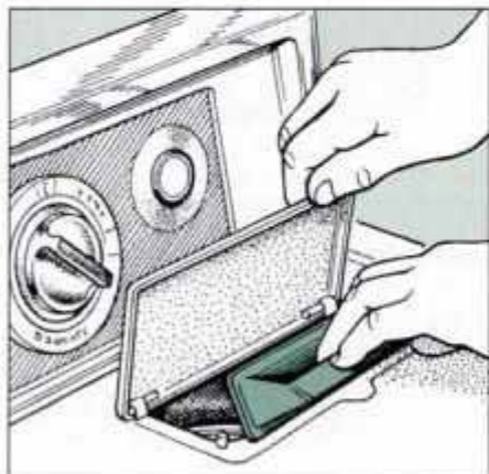
1 Prepare for replacing the dryer belt by lifting the lint-screen cover on the top of the dryer. Then remove the lint screen.
