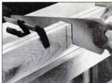
14 Clamp the end support rails firmly together, and cut the cross support notches in them using a handsaw.
