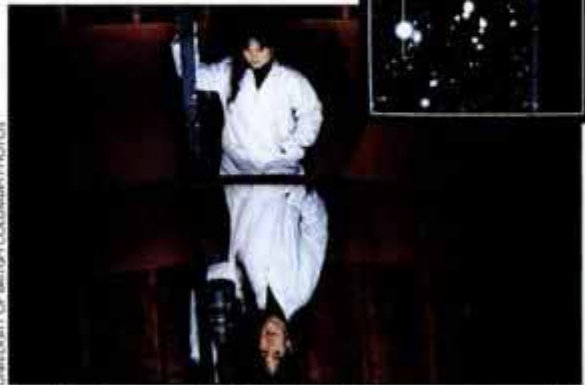
Liquid mirror, made of highly reflective mercury, provides quality images at a tenth the cost of glass equivalent.
