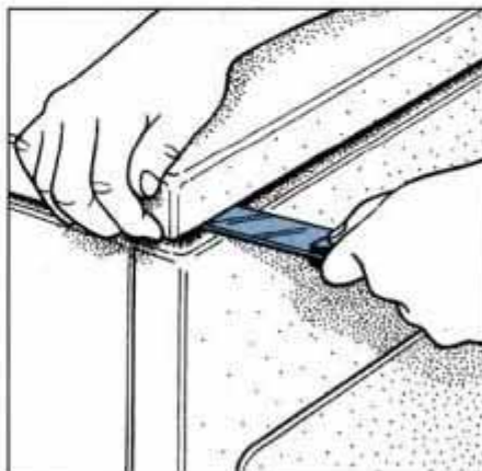
3 Slide a putty knife between the front panel and the top near a corner. Lift the corner and repeat on the other side.
