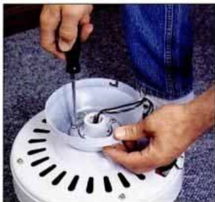
10 With the fan components on the floor, attach the motor cowling to the fan canopy with the screws provided.
