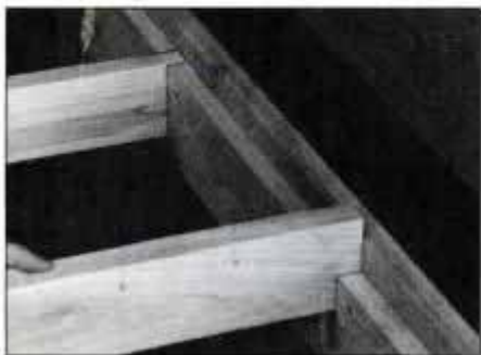
17 Prepare for installing the slats by fitting the cross supports into the notches that are cut in the end support rails.
