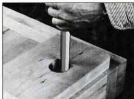
12 Use a chisel to cut a flat surface into the hole on the side rails. The bed bolt nut bears on the flat surface.
