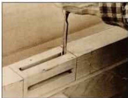
3 Clamp the posts firmly to the bench, and chop the ends of the post mortises square using a sharp chisel.
