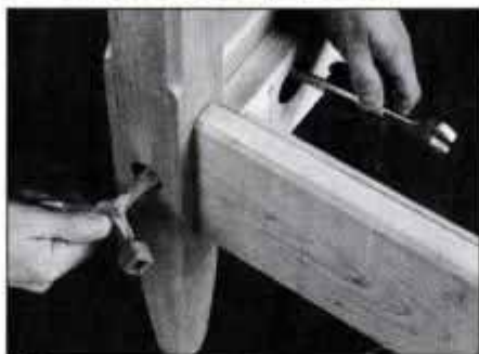
16 Use a bed bolt wrench and an open-end wrench to tighten the connection between the rails and posts.
