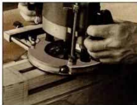
2 Cut the post mortises before sawing the tapers. Use a plunge router or bore out the mortises on the drill press.
