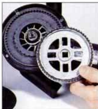
The Bosch 1370DEVS has a reversible drive plate. Geared position fixes disc speed for aggressive sanding.
