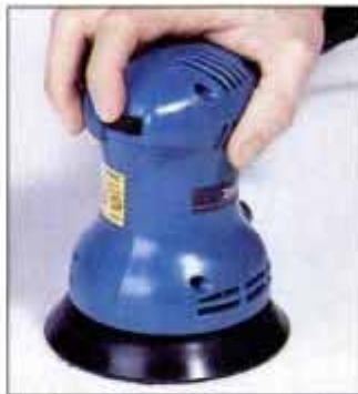
Single-speed palm-grip sanders have a rocker-type switch. The tool is held on top, or around the narrow waist.
