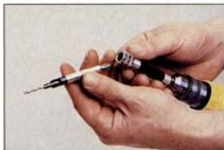
1 After boring a pilot hole with the drill bit, slide forward the collar and flip the cartridge around to access the driving bit.
