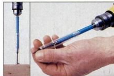
2 To use the Vision Finder/Driver, first load the screw in the clear plastic tube. The tube retracts as the screw is driven.
