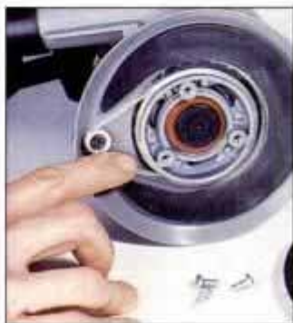
To control disc speed, the P-C 333 uses a plastic belt. Other tools use varying designs to slow down free-spinning disc.
