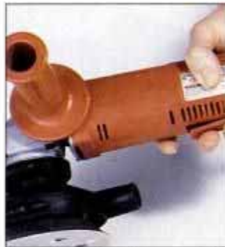
The Milwaukee has a paddle switch. The other right-angle designs have a sliding switch that can be locked.
