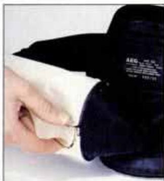
Most tools have a dustbag that's spring clamped to a dust port. The bags are fairly effective in containing dust.
