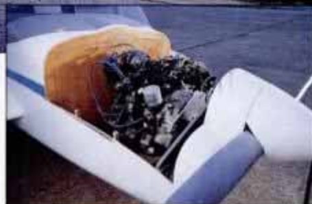
Mockup reveals 180-hp Mazda rotary in proof-of-concept version. Cockpit includes both air and road instrumentation, dual-mode steering yoke and automobile-style pedals.
