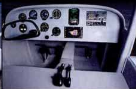
Mockup reveals 180-hp Mazda rotary in proof-of-concept version. Cockpit includes both air and road instrumentation, dual-mode steering yoke and automobile-style pedals.
