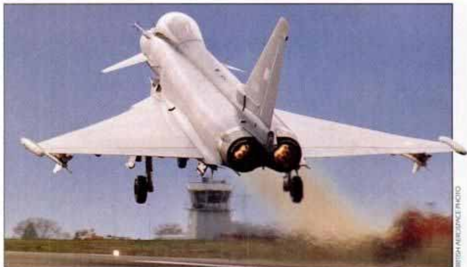
The Eurofighter 2000 boasts a thrust-to-weight ratio greater than 1:1.
