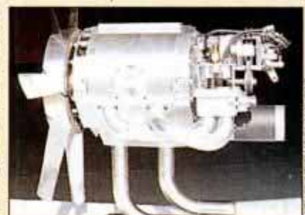
Moller's single-rotor 530-cc engine, finally complete, will power his volantor.
