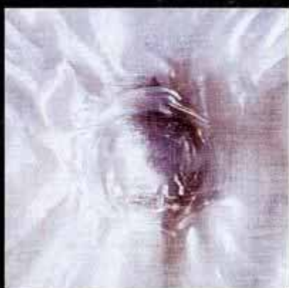
Energy dispersion of Spectra Shield covers a wide rounded area, flattening the bullet by sending energy across the surface at super-high speeds.
