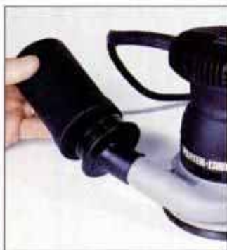
The P-C 333 uses a permeable rigid canister to collect dust. A vacuum can be connected to the dust port, as well.
