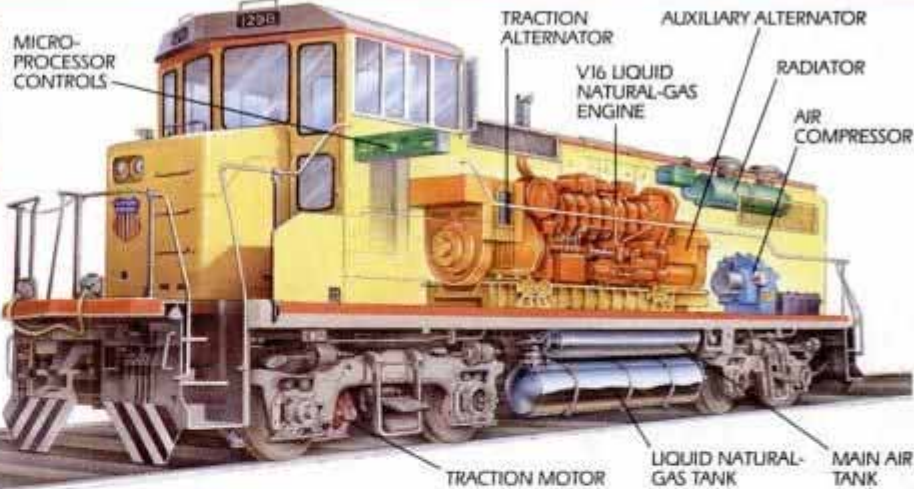
MK1200G switcher locomotive burns natural gas carried in cryogenic storage tanks.
