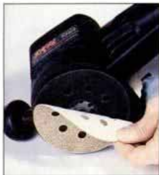
Most sanders use the hook-and-loop system for securing the disc. The holes in the disc and pad carry dust away.
