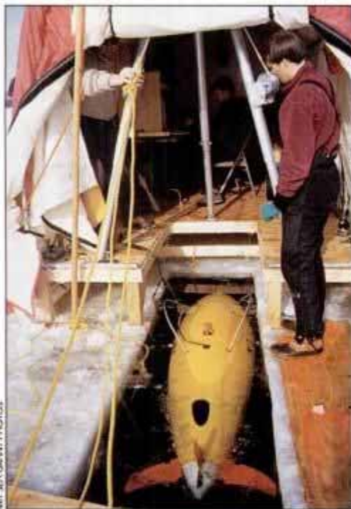
Odyssey II , shown here during initial trials in New Hampshire, later mapped hidden underside of Arctic ice pack off Prudhoe Bay, Alaska.
