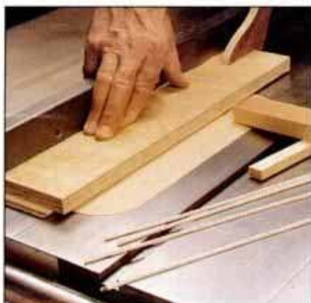
11 Tape triple veneer under board with 1 in. extending past end. Reference T-guide against extension to cut \frac{1}{16} -in. strips.
