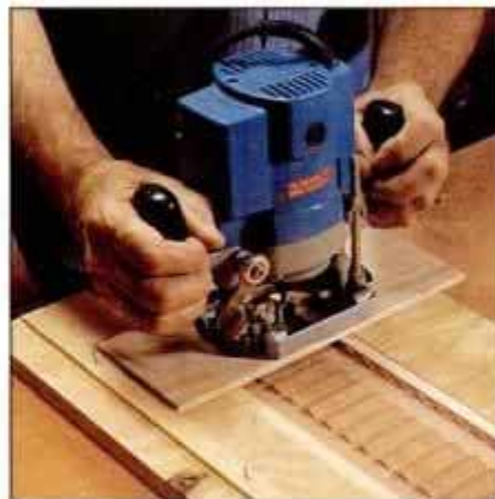
3 Tack strips to both edges of assembly and place between guide boards. Install a wide base on router and trim faces flat.
