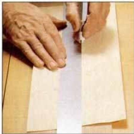
4 To add stripes to each side of the diamond pattern, cut maple and mahogany veneer to the size of the diamond blank.
