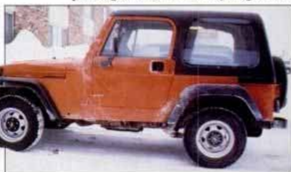
Nothing but coil springs hold up the new Wrangler.
