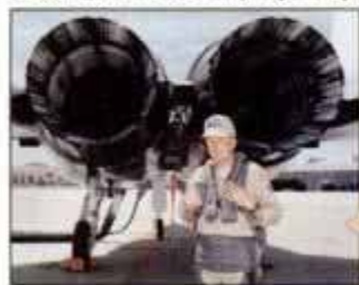
Engines become steering mechanism in flight-control system that uses thumbwheels for input.
