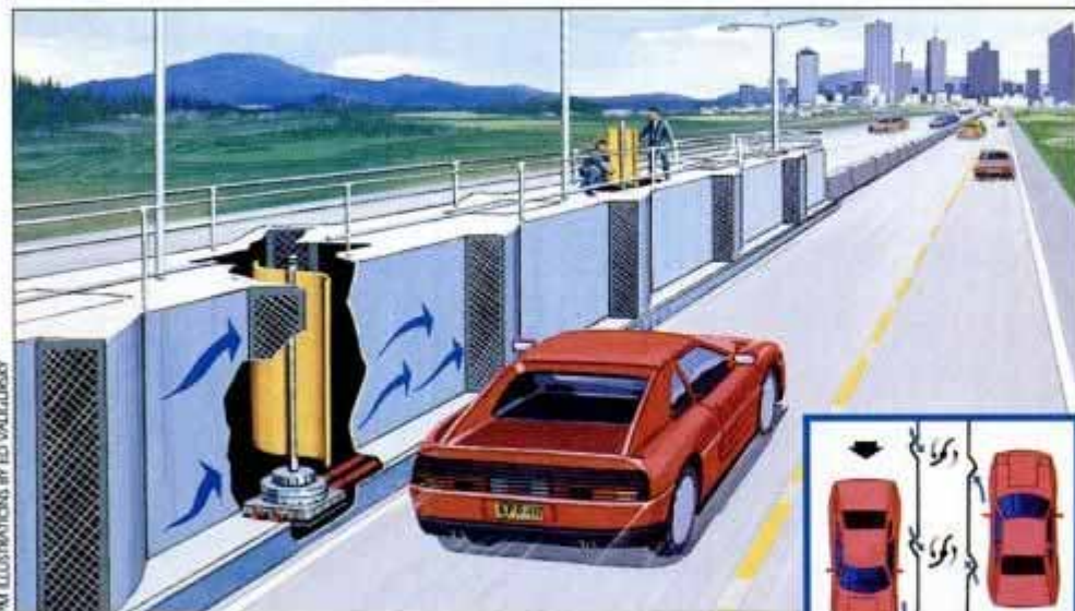
Wind would rush through slots on each side of the crash barrier, spinning blades counterclockwise to generate electricity.
