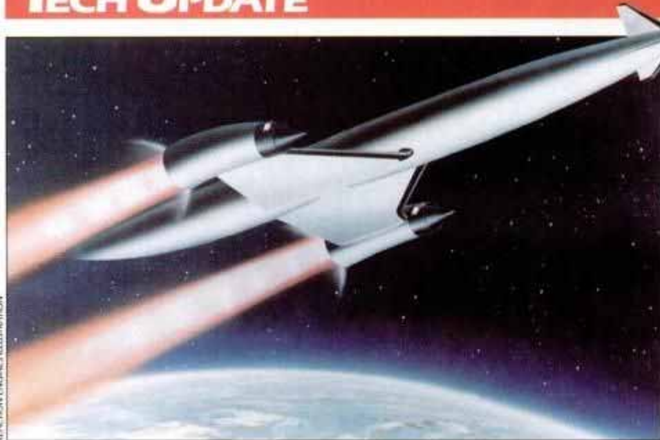
Unmanned Skylon, 270 ft. long, would fly at a speed of Mach 5 before converting to rocket mode.
