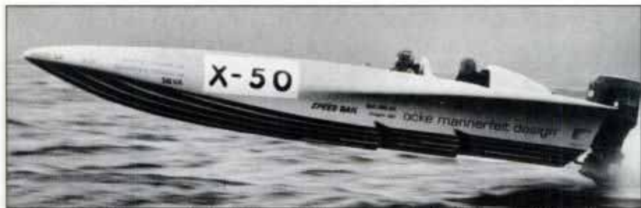
Steps cut laterally across the hull. Speed Rails run along the hull's longitudinal axis.
