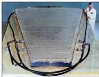
A mere ½ in. thick, giant mirror segment rests on corrective actuators.
