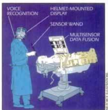
CAMIS borrows target recognition and helmet-mounted display from the cockpit.
