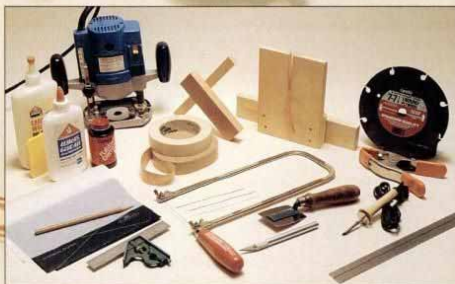
To make our banding inlays, you need a router with guide bushing, masking tape, spring clamps, shopmade T-guide, veneer saw, knife and glue. To lay out and inlay a marquetry insert, use carbon and tracing paper, a hard pencil, rule, rubber cement, gummed veneer tape, a fret saw and a shopmade birds-mouth (cutting support).
