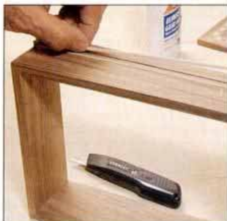
12 Cut triple-stripe recess with a fine-cutting thin-kerf blade. Then glue stripes in place, using butt joints at corners.
