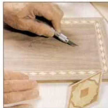
16 Use a sharp knife to trim round corners left by router. Apply glue and clamp marquetry assembly. Sand flush when dry.
