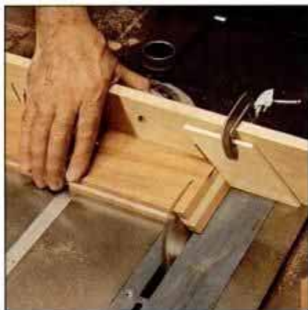
1 With the saw blade tilted at 45°, cut the lamination into 1/4-in. slices. Clamp a stop-block to a miter gauge fence for uniformity.
