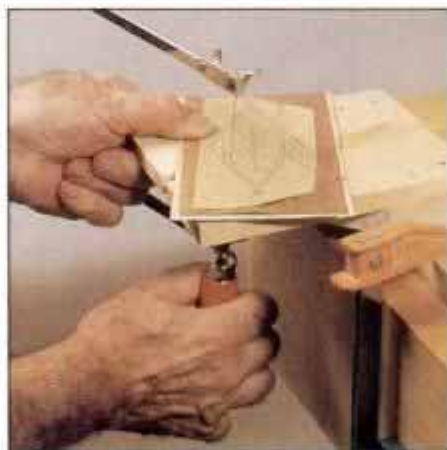
13 Support veneer on birds-mouth, and use fret saw to cut shapes. A pushpin makes holes that start each internal cut.
