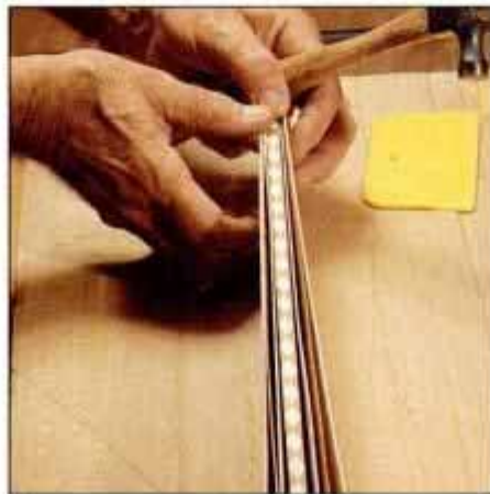
5 Laminate a stack of maple, mahogany and maple veneer to each side of the diamond blank. Clamp until glue sets.
