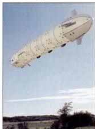
Scale model demonstrates concept for articulating cargo blimp nearly twice the length of the Hindenburg.
