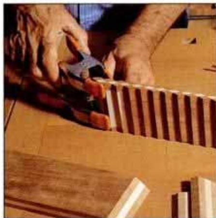
2 Reassemble the slices so each maple section abuts a mahogany piece. Use tape and spring clamps to hold pieces in place.
