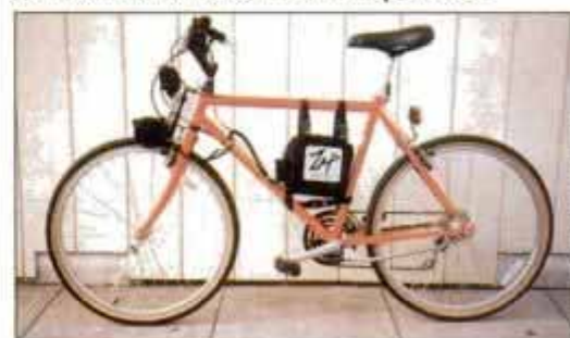
ZAP Power System uses front-wheel rollers to lend electric power to pedaling efforts.
