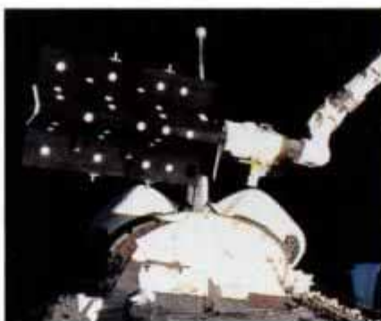
Dot-based system was tested on '92 shuttle flight for future use during space-station assembly.
