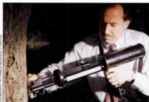
Decay-detection drill maps inner condition of wood by monitoring resistance as it penetrates.
