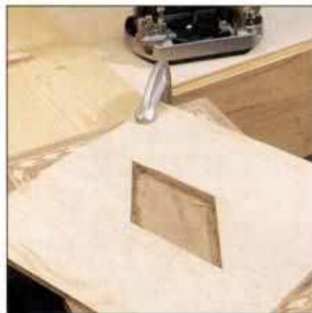
15 Use a template, guide bushing and straight bit to rout marquetry recess. Bushing and bit size determine template size.
