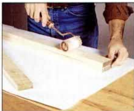
1 Begin each leg by gluing three \frac{3}{4} \times 2\frac{1}{4} -in. boards together. Use waterproof glue, and trim each blank to 2 \times 2 \times 20 in.
