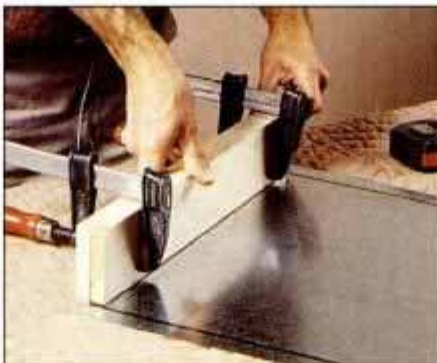
12 To bend sheetmetal neatly, clamp hardwood strips at bend line. Then, use strips to bend metal to a 90° turn.
