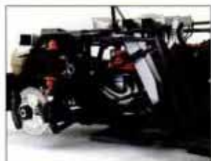
Left: The rear independent suspension system complete with operating Koni shock absorbers, brake disc and brake calipers— all faithfully reproduced in 1:8 scale. (The item just to the right of center is the oil reservoir tank.)
