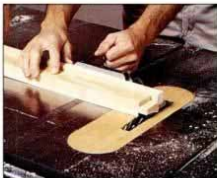
3 Cut the rail tenons with a dado blade. A stopblock clamped to a miter gauge extension ensures accurate repetitive cuts.
