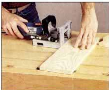
5 Make the side panels by gluing the narrower stock together. Use a plate joiner to ensure good alignment.
