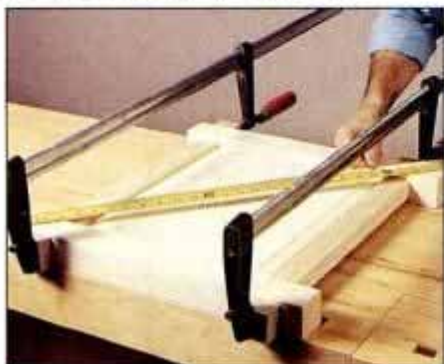
8 Check that the assembly is square by measuring opposite diagonals. If necessary, loosen the clamps and adjust.
