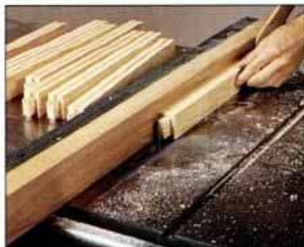
4 Reset the dado blade and make the \frac{1}{4} -in.-wide \times \frac{1}{2} -in.-deep grooves in each rail. Use a push block to move work safely.
