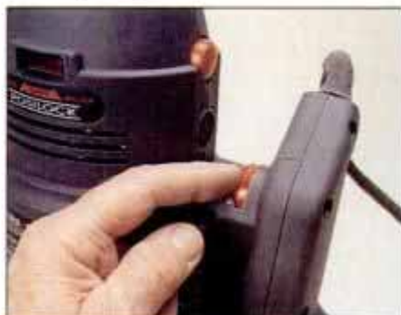
Variable-speed dial is located near right handle. The right hand also works the ON/OFF trigger and power-lock button.
