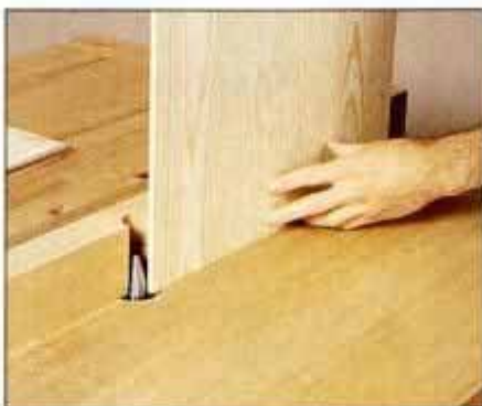
6 After trimming the panel to exact size, cut the raised panel profile on a router table with a vertical panel-raising bit.
