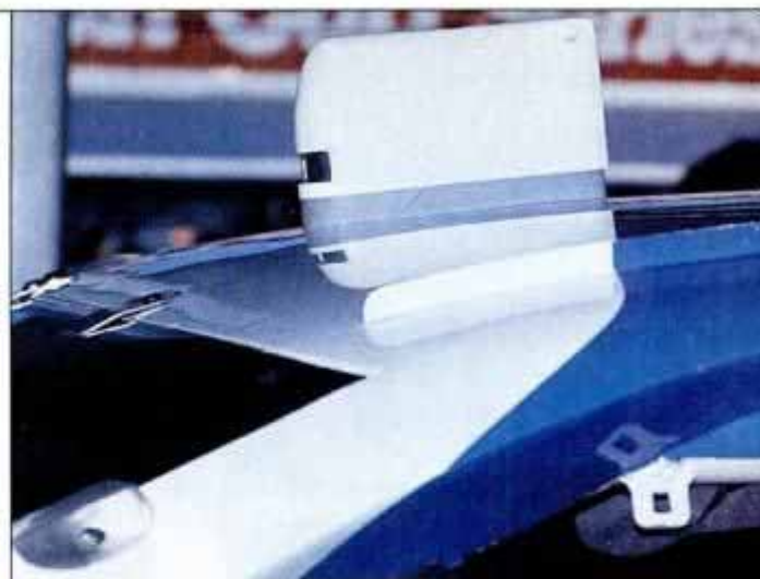
Extra padded steering wheel and aero roofcam are recent intros to NASCAR racing.
