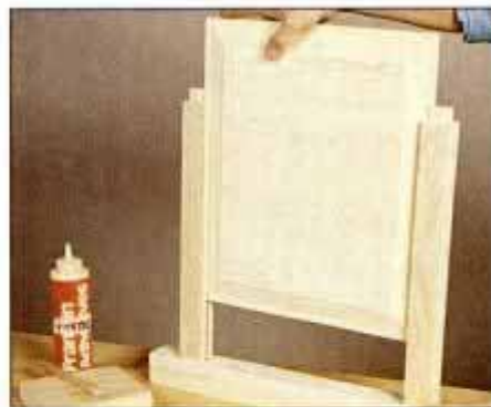
7 Begin assembly by gluing two rails to one post. Then, slide panel into grooves, add opposite post and clamp joints tight.
