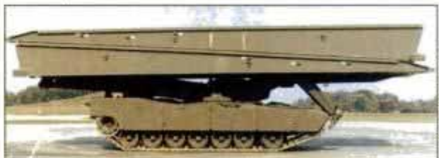
Hydraulic arms extend the twin leaves of the Heavy Assault Bridge from the roof of an M1 chassis.
