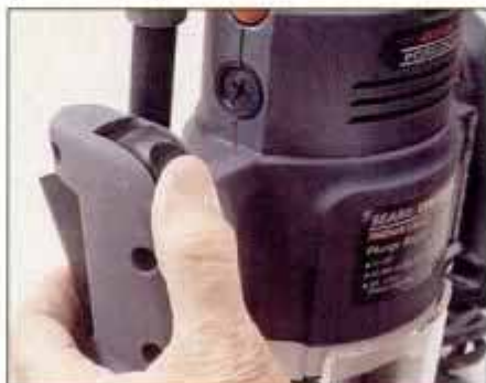
Comfortable handles contain router controls. Left handle incorporates plunge-lock lever and release button (under thumb).
