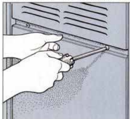
1 Use a screwdriver to release the retaining clips that hold the furnace access door in place. Then, remove the door.
