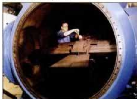
Pratt & Whitney scramjet delivered thrust at Mach 14 (9500 mph) in shock tunnel.
