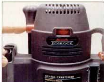
Engage spindle lock by pressing button on housing top. Red light at center indicates locked spindle, and tool will not start.
