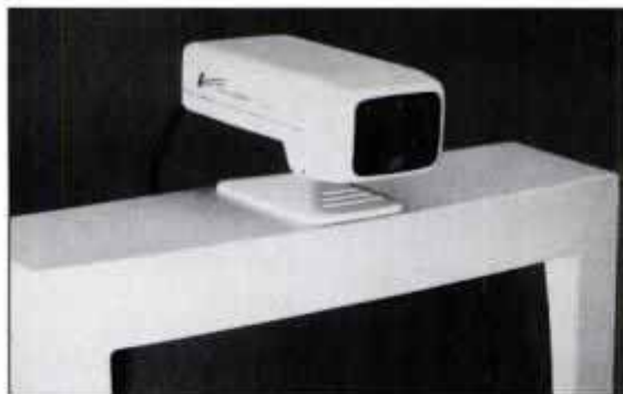
This tiny video camera mounts atop a computer monitor for face-to-face conferencing.
