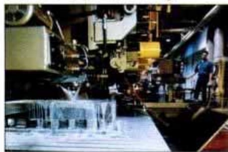
Five-axis milling machine works over component of first flying F-22 fighter.
