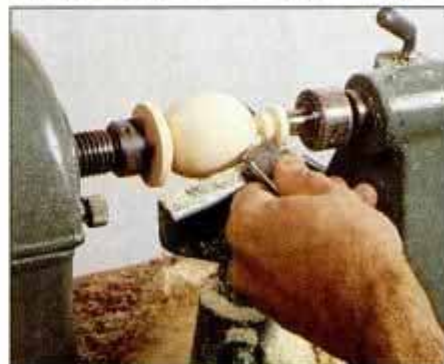
10 Use a template as a guide to shape finials. Leave a stub at top end and sand while in lathe. Then, sand stub smooth.
