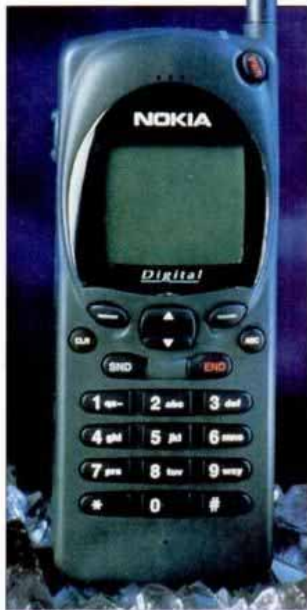
NOKIA The 2120 features a 30-character display and a continuous diagnostic readout.
