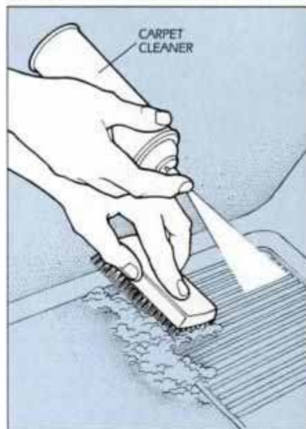
Stubborn grease or salt stains on floor carpeting can be removed with a foam-type carpet cleaner and a scrub brush.
