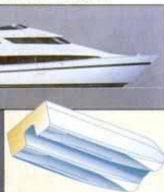
As ferry or yacht, SeaCoaster offers air-blown twin-hull with wave-slicing bows.
