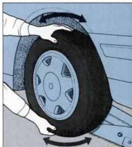
Check nondriving wheel bearings by trying to rock the raised wheel in and out at the 12 and 6 o'clock positions.
