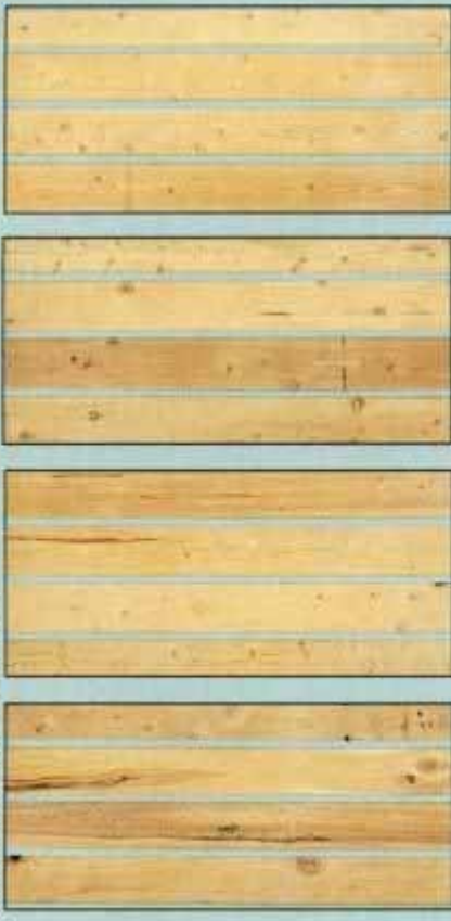
Structural joists and planks are more than 5 in. wide. Shown (from top to bottom) are select structural and Nos. 1, 2 and 3.
