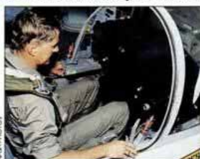
On needle-nose aircraft like this F104 Starfighter, periscope relays a runway view to pilot during take-off or landing.
