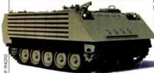
Enhanced Applique Armor Kit swaddles M113 in steel-composite sandwich.
