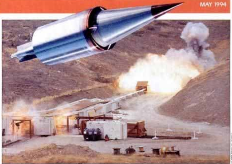
Scale model of axisymmetric scramjet (inset), with built-in hydrogen propulsion system, roars out of 2-stage gas gun. Compressed hydrogen in gun boosted engine to Mach 8.
