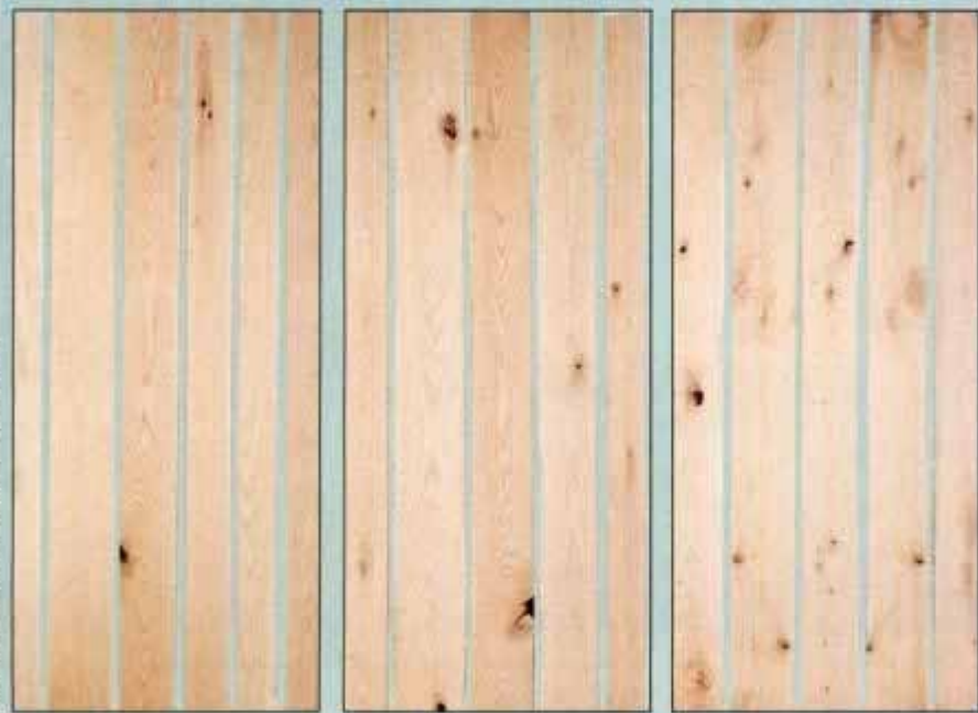
Hardwood lumber is typically graded from the poorer side. Oak samples shown (from left to right) represent FAS (firsts and seconds), No. 1 and No. 2.
