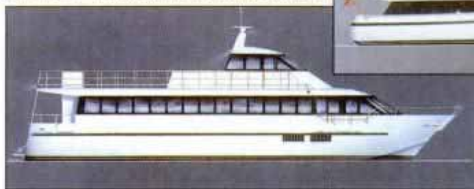
As ferry or yacht, SeaCoaster offers air-blown twin-hull with wave-slicing bows.
