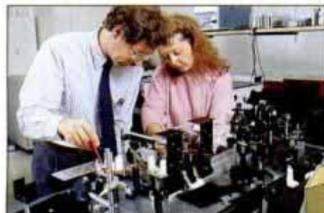
Laser pulses stimulate photosynthesis, then gauge speed of electron transfer in microbes.
