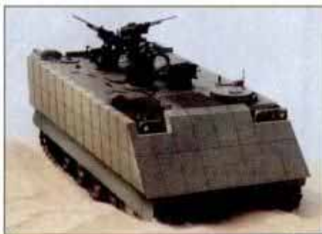
Reactive-hybrid package shields vehicle from brunt of exploding armor panels.
