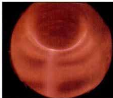
Inside tokamak, donut-shaped torus vessel (left) confines deuterium-tritium plasma (above), which glows at 600 million° F.
