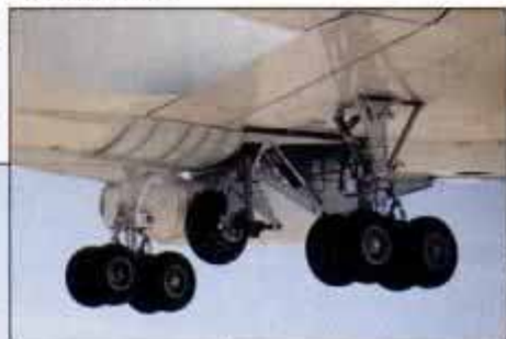
As NASA's Convair 990 lands, shuttle gear emerges from cavity in fuselage to simulate aborted-mission touchdown.
