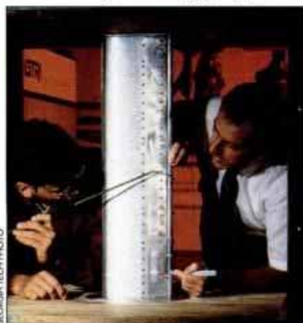
Circulation-control wing releases air through flaps to boost lift by decreasing pressure on wing's upper surface.
