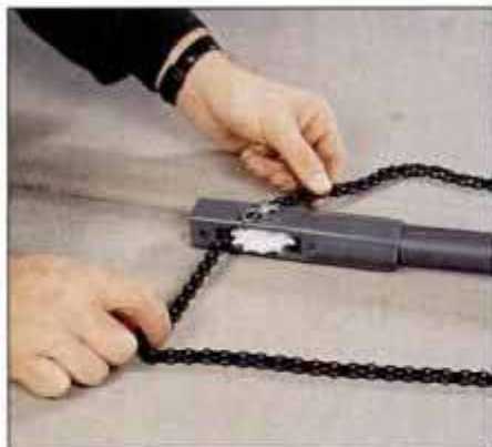
7 At the idler assembly, remove all remaining chain from the spool and feed it through the return sprocket.
