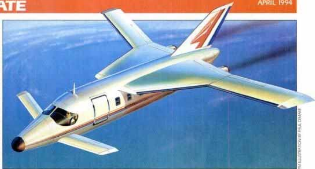
Canards distinguish Contender, which could serve as a commuter, cargo or executive jet.
