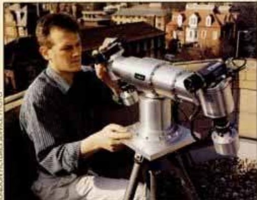
Computer-guided motors allow Yorick to follow objects even if they take unpredictable turns.
