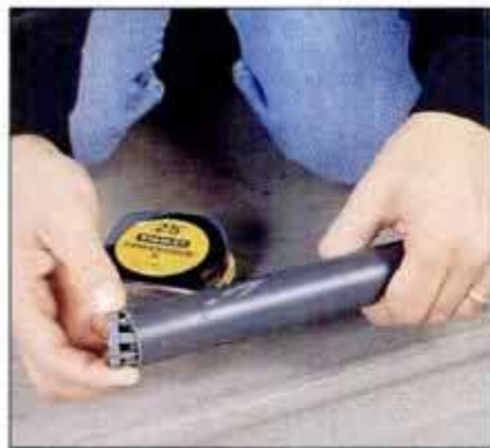
1 Lay out all parts on the floor, then slide the cap onto the power-unit end of the tube until it hits the retaining flange.
