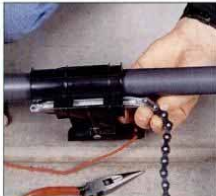
5 Attach the drive chain to the traveler with a repair link supplied in the kit. The retainer clip must face up.
