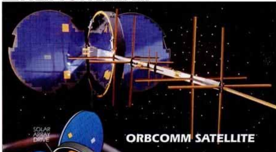
The ORBCOMM paging satellite (left) relays a signal to one of four strategically placed gateways (above) that act as switching centers.
