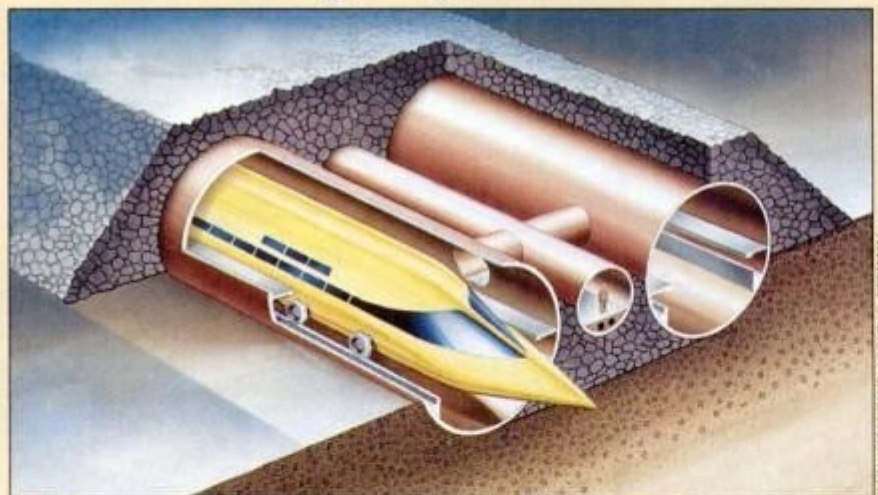
Trains race through WorldLink tunnel made from prefab double-tube segments.
