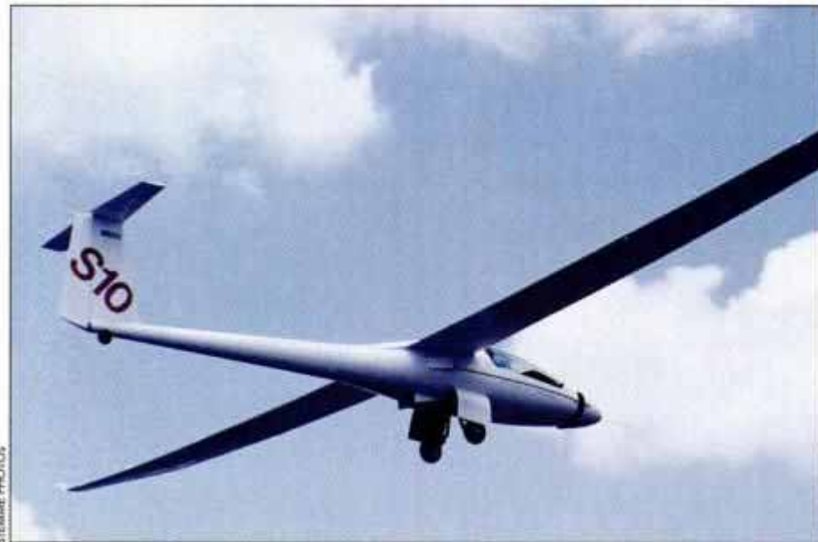
Highlights of the high-flying Stemme S10: retractable folding propellers, all-composite construction, high-performance wingspan and panoramic views.
