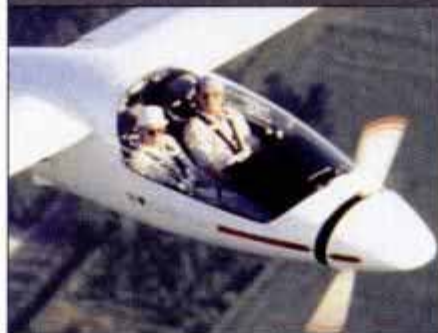
Highlights of the high-flying Stemme S10: retractable folding propellers, all-composite construction, high-performance wingspan and panoramic views.
