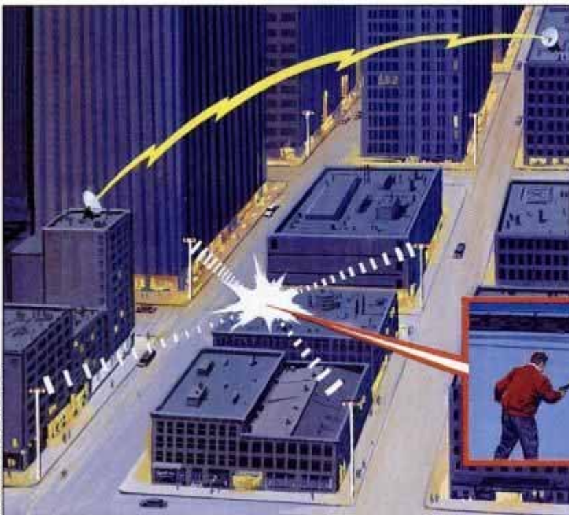
Acoustic sensors detect and pinpoint gunfire, then relay data via digital radio to command post, which dispatches emergency services.
