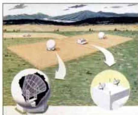
The ORBCOMM paging satellite (left) relays a signal to one of four strategically placed gateways (above) that act as switching centers.
