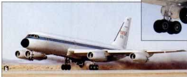
As NASA's Convair 990 lands, shuttle gear emerges from cavity in fuselage to simulate aborted-mission touchdown.
