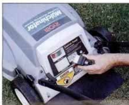
2 After removing extension cord, slide door over recharging port to insert ignition key. Key also acts as a circuit breaker.
