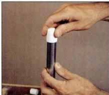
21 Press the tubing caps on the handle and leg. Soften them, if necessary, in hot water or use a heat gun or blow dryer.
