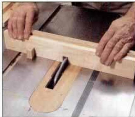
9 When cutting evenly spaced notches, use guide block secured to fence. Place last cut over guide block to position next cut.
