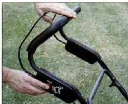
3 To start motor, press button at side and move up control bar. Mower stops running as soon as control bar is released.
