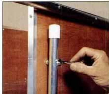
22 Use three washers between the leg and the sides. Cut off the excess screw shaft, and file it smooth.
