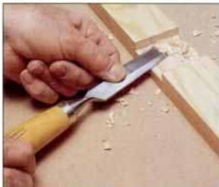
4 After prying out the waste with a chisel, pare the notch bottom flat and smooth. Then test fit and adjust if necessary.
