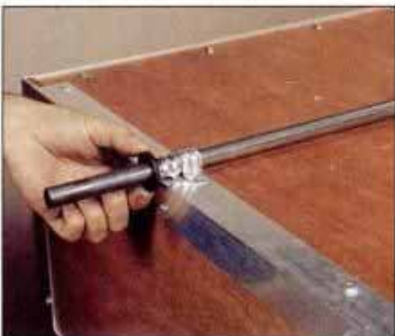
15 Slide a washer onto the axle. The washer acts as a bearing surface between the wheel hub and cart.
