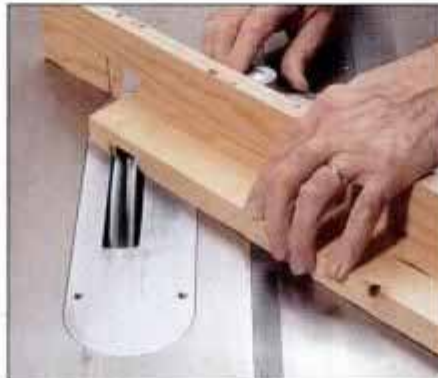
11 Begin mitered half lap by making a mitered notch on the end of square-cut stock. Align shoulder cut with corner.
