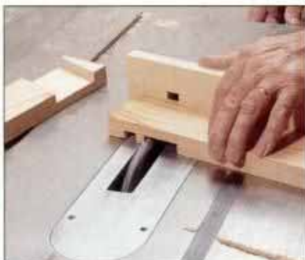
7 Cut angled end lap near end of stock—trim overhang after assembly. Notch in fence helps position shoulder cut.
