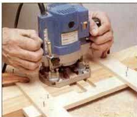
5 Use a guide frame to cut half-lap joints with router. Place both pieces edge to edge and cut at the same time.
