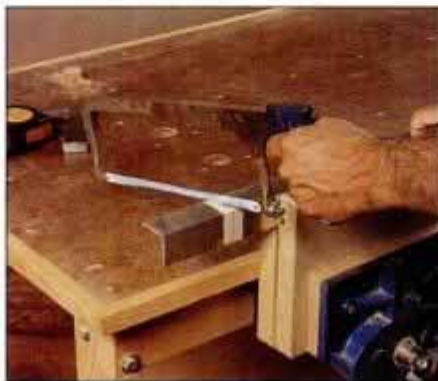
3 Apply tape to the angle stock, and mark the cutline on the tape. Clamp the angle stock firmly while cutting it.
