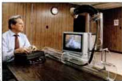
For turns, two body hoses are vacuumed while the third is pressurized.
