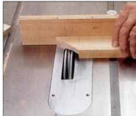
12 Set miter gauge to 90° and cut notch on end of mitered stock. Align the shoulder cut with the obtuse corner of miter.
