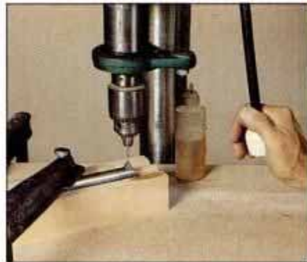
18 Clamp the axle and support block to the drill-press table. Use cutting oil when drilling the cotter pin hole.
