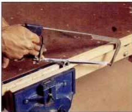
16 Clamp the nut in a vise and then saw it in half. Clean up the saw marks with a fine file or a sanding block.
