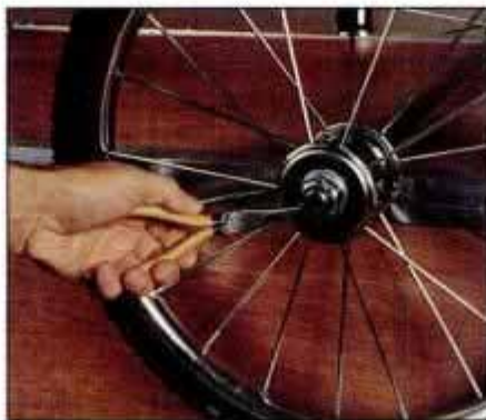
19 Clean off the burrs on the axle made from drilling the cotter pin hole. Install the axle, washer, wheel, nut and pin.
