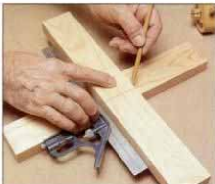
1 Lay out width of half-lap notch by scribing against mating piece with a sharp pencil or knife. Use a square to hold stock at 90°.
