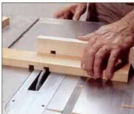
6 To cut joint on table saw, install dado blade and set height to half the stock thickness. Notch in fence indicates cutline.
