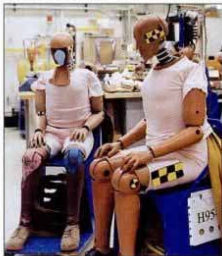
Instrumented crash-test dummies are now sartorially and anatomically correct.
