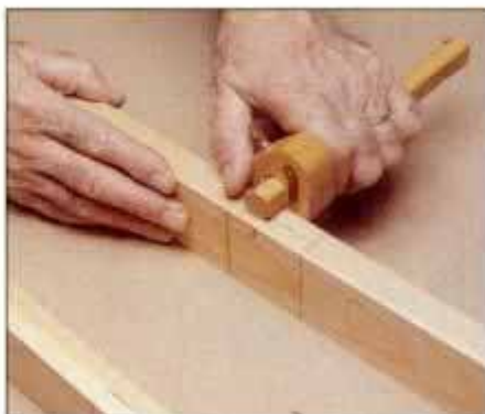
2 After extending lines across edges, use a marking gauge to lay out notch depth. Set gauge at one-half the stock thickness.
