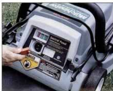
1 To charge battery, connect mower to the nearest outlet with an extension cord. A full recharge takes about 16 hours.
