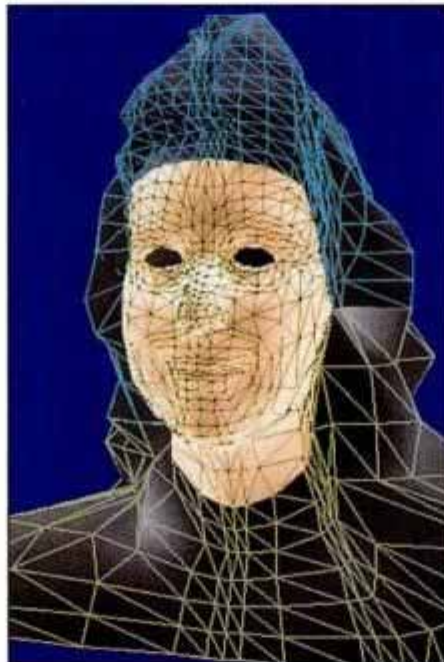
The collage at top shows a digitized scan of a person's face and the computer model, later manipulated to show various emotions. Remove the texture mapping (bottom left) and you see the 3D triangulated surface mesh. A closeup (bottom right) reveals the amount of detail in the computer construct.
