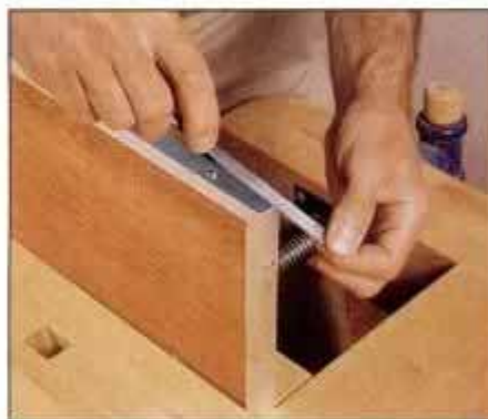
8 File a small bevel on the miter corners where channels meet. If you lack a fine file, use a sanding block.
