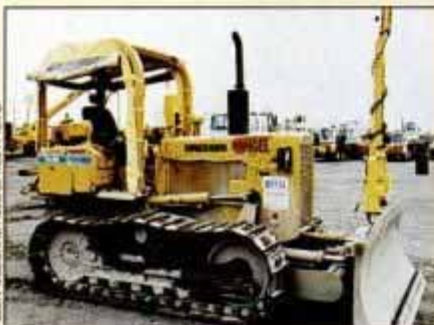
Ohio State's Center For Mapping is testing precision control of earthmover blades.
