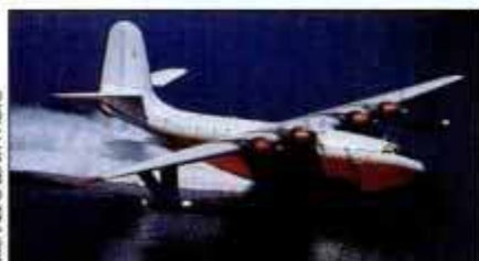
Big fires call for big bombers. Clockwise from top left, Lockheed C-130 Hercules swamps blazes with modular tank system, Consolidated PB4Y Privateer sprays mud or water, Douglas DC-6 delivers retardant and Martin Mars flying boat scoops up 24 tons of water.
