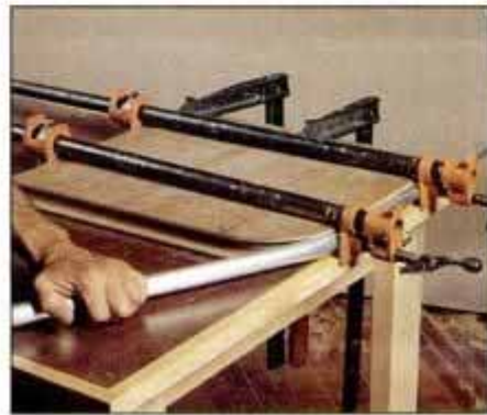
20 Align the marks on the tubing with those on the jig, and clamp the bending jig securely to the workbench.
