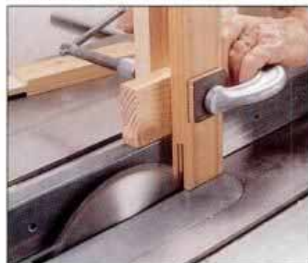
14 To cut slot, clamp work with scrap blocks to straddle fence. Make cuts with blade height at width of mating piece.
