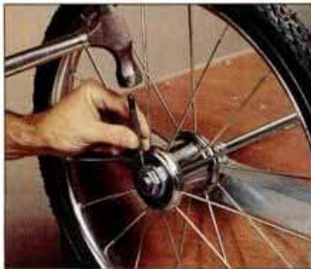
17 Temporarily install the wheels and nuts. Dimple the axle using a centerpunch to mark the cotter pin hole.
