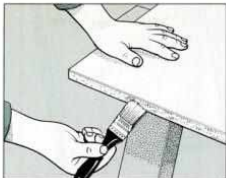
11 Use a brush to apply two coats of contact cement to the edges. Then, coat 1-in. strips, let cement dry and install on edges.
