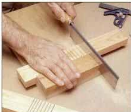
3 Use a backsaw to make shoulder cuts with stock held on bench hook. Then make a series of kerfs in waste area.
