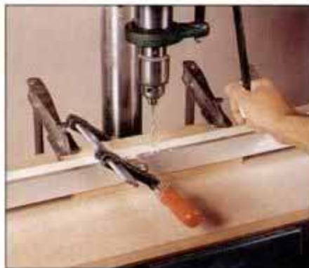
4 Clamp a fence to the drill-press table. Clamp the angle stock to the fence to support the stock while drilling.
