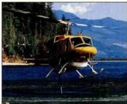
Versatile Bell 212 can deploy probe to draw water out of source as shallow as a foot deep or dump 360 gallons of foam.
