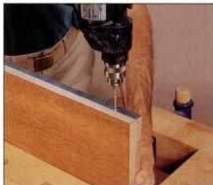
6 Place the channels on the panel edges. Bore the pilot holes for the screws that hold the channels in place.
