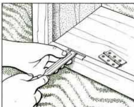
20 Lay out the mortises for the butt hinges on the inside of the cabinet face frame. Remove the waste with a razor-sharp chisel.
