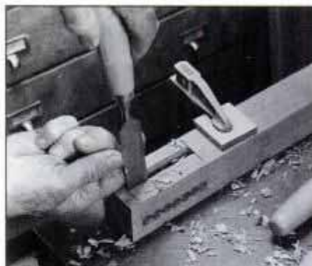
2 Clamp the legs to the bench. Using a razor-sharp chisel, pare the sides of the mortise parallel and the ends square.
