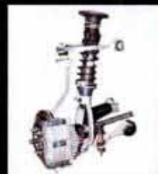
Short/long-arm front suspension reduces ride harshness.
