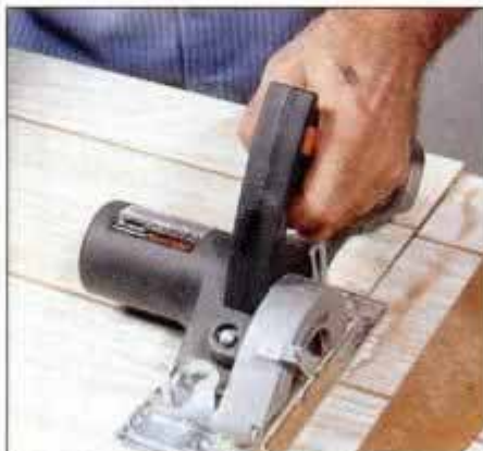
Light plywood and panel cutting are typical chores for this cordless tool. A rip fence accessory is available.
