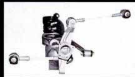
Five-link rear suspension is first to use fiberglass links mated to aluminum alloy ends for strength and light weight.
