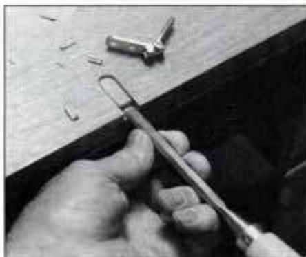
16 Cut a notch for the hinge knuckle at the rear of the mortise. Each half of the mortise is notched to receive a knuckle.
