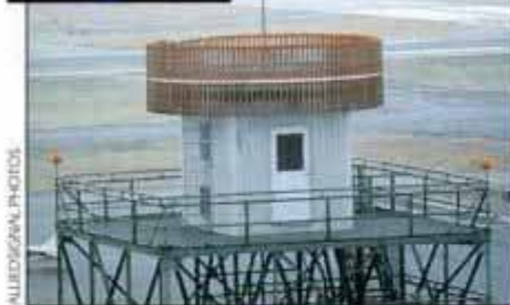
PRM allows tighter spacing on runways, thanks to phased-array antenna.
