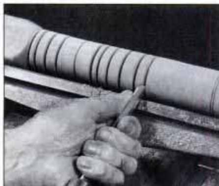
6 Using the parting tool, make each of the depth cuts. Back off from the parting tool occasionally to let it cool.
