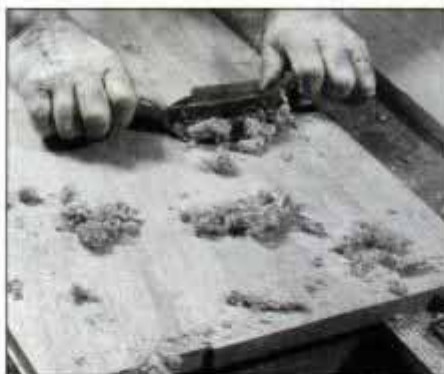
14 Push a cabinet scraper over the panels to remove the dried glue at the joints and to level the panels.
