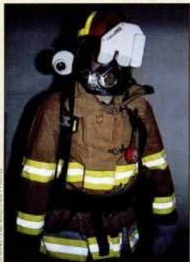
CairnsIRIS infrared camera alerts firefighter to trapped people, hidden hot spots and flashovers.
