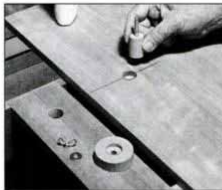
21 Dry assemble the pivot, then position the top on the base to check for movement. Mark the pivot stop position.
