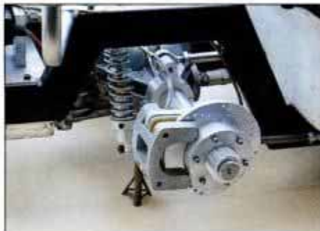
Cobra front A-arm suspension features adjustable shocks. Aluminum brake calliper grips with fiberglass pads (upper left). Rear suspension is 4-link setup. Rear disc brakes also are hydraulically activated (lower left). Cobra chassis shows fuel filler and dual master cylinders on rear platform (above).
