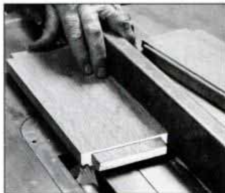
19 After the tenons are cut, shape the bead on the aprons with a molding head installed in the table saw.
