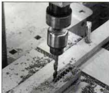
1 Lay out the mortises in the legs. Remove the bulk of the mortise waste by boring holes with a drill press.
