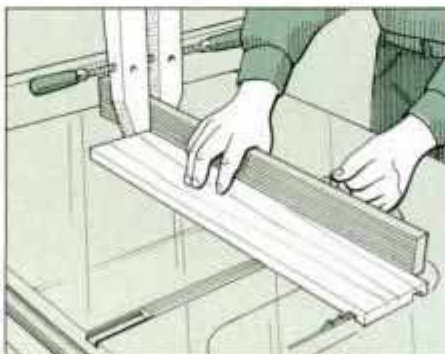
22 Use a table saw and dado blade to cut the grooves, dadoes and rabbets in the drawer sides, front and back.
