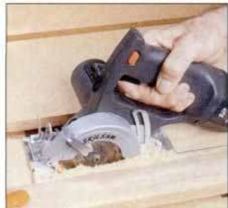
With a maximum cutting depth of 1 5 / 16 in. at 90°, the 4.5-pound saw easily handles 3/4-in.-thick particleboard.
