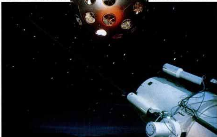
Laser measures changes in Stella's orbital path caused by gravitational blips.
