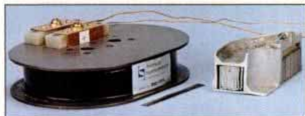
Acoustic transducer (top) and generator coil (above) feature new superconducting materials.
