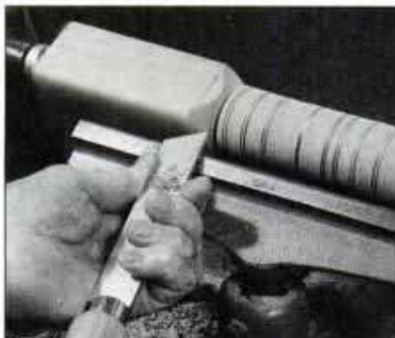
5 Use the skew chisel to turn the round shoulder on the leg. The nick cut made earlier prevents splintering.
