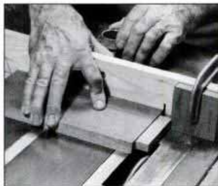
18 Cut the apron tenons on the table saw using a dado head. Butt the apron against the stopblock to make the cut.
