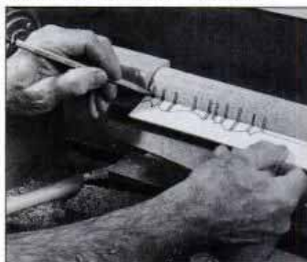
4 Use the half pattern of the leg to mark out the depth cuts that establish the diameters at key points.
