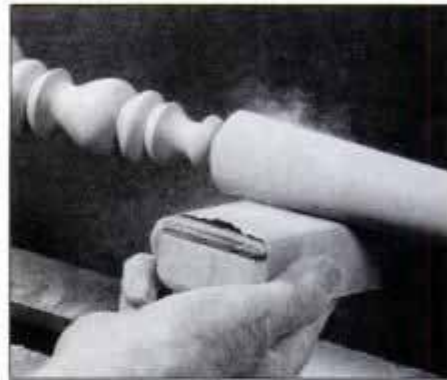
11 Use a felt-pad sanding block and 220-grit paper to smooth the long, tapered portion of the turning.
