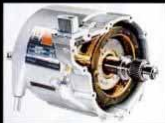
AC induction motor spins at 20,000 rpm to eliminate the need for a transmission.
