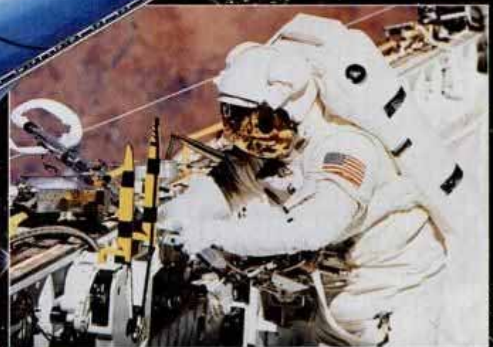
Astronaut Carl Walz tested NASA's Power Ratchet Tool, a key instrument in the Hubble repair mission, during a Shuttle flight last summer. The computer-controlled tool will be a Jack of all trades.
