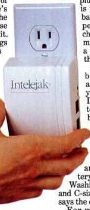
Phonex Corp.'s Intelejack uses a house's existing electrical wiring to extend the reach of telephones.
