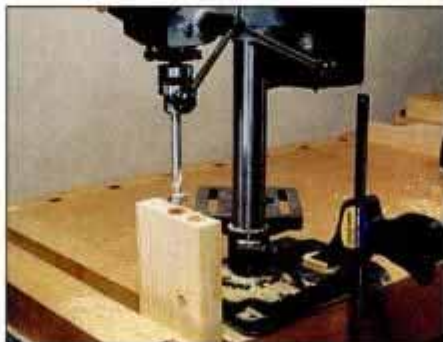
To increase capacity, the head can be rotated. Here, the tool is clamped to a workbench while the work is held in the vise.
