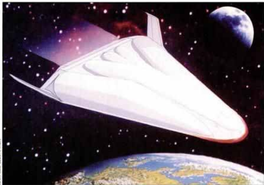
Aeroballistic rocket combines plug-nozzle engines with lifting-body silhouette.
