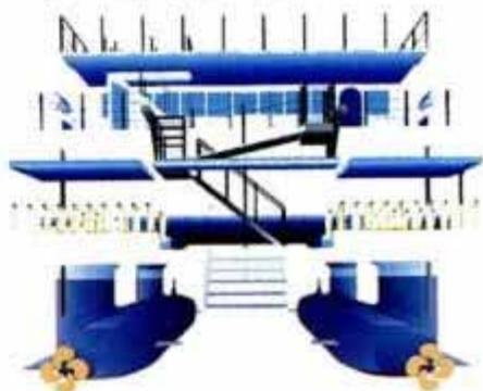
Nekton allows divers to take the plunge from hydraulically lowered stern platform.
