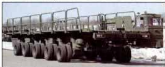
New loader raises conveyor bed on hydraulic jacks and is air-transportable itself.
