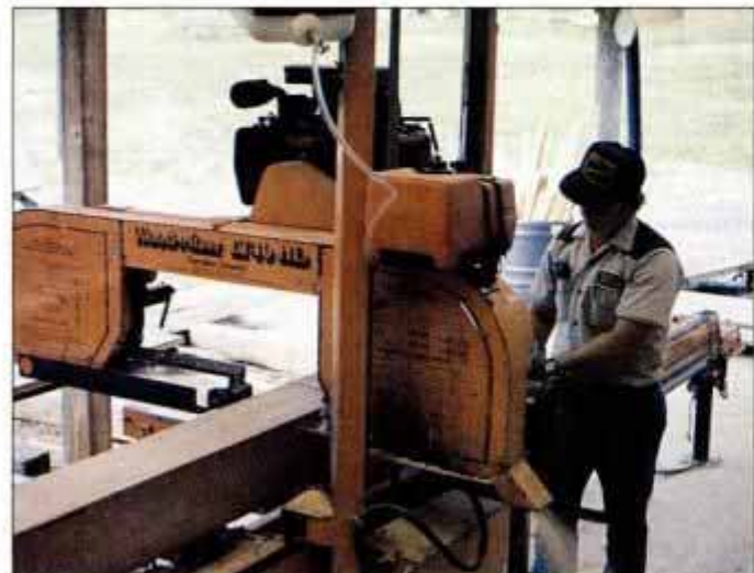
Once a log has four sawn surfaces, it is called a cant. At this point, the cant can be easily sawn into smooth, straight boards.
