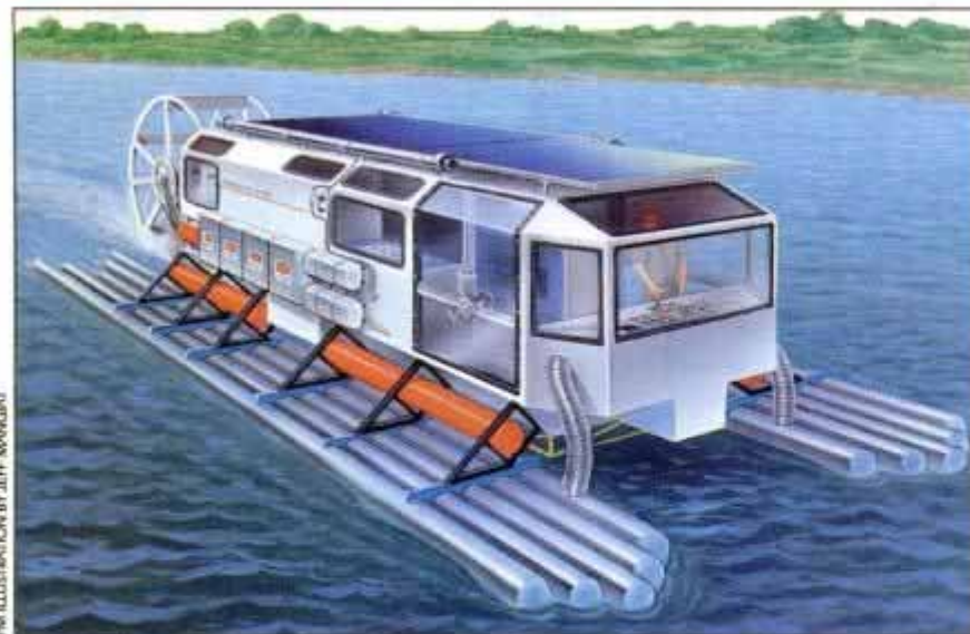
Homebuilt riverboat combines all-electric drive with high-flotation pontoons.
