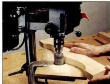
For drum sanding, clamp board with a hole to the table. Then raise the table until the work meets the drum.
