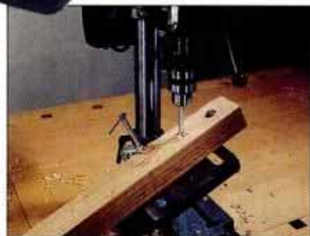
The table tilts to the right or left for angle drilling. The table and the base feature clamp access slots for securing your work.
