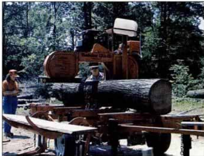
The saw has been trailered to a pile of logs outside, and away from the saw shed. One face of the log has been sawn.
