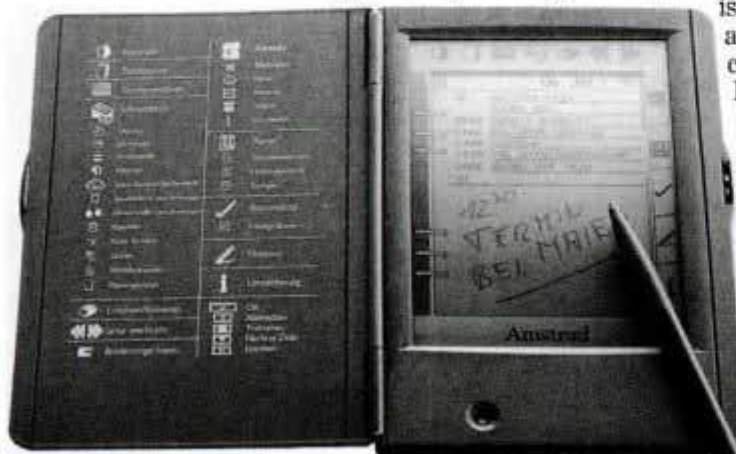
The display screen for Amstrad's PenPad looks like a notebook. You flip through the electronic pages by touching the arrows.
