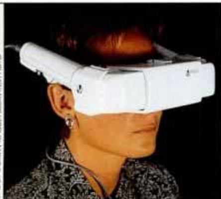
Miniature cameras in this headset give virtual-reality-like viewing to persons with low visual acuity.
