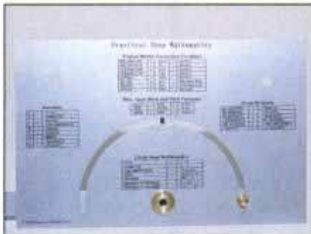
1 Etched into the protractor's back is a variety of handy shop information that relates to working with angles.
