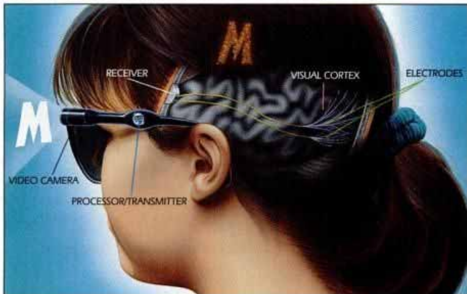
Virtual-reality technology mated to a GPS receiver are the keys to a future guidance system for the blind (above). Aural technology makes sounds emanate from particular points in space (Inset). Another device (below) uses data from a camera to stimulate microelectrodes implanted in the brain, producing the sensation of light.
