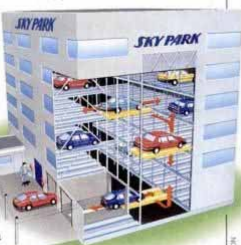
Robotic Sky Park uses robotic trolley to pigeonhole cars automatically.
