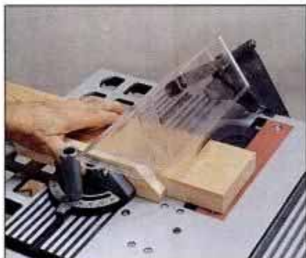
3 With a maximum capacity of 2 1 / 2 in. when the blade is at 45°, bevel cutting nominal 2-in. lumber is no problem.
