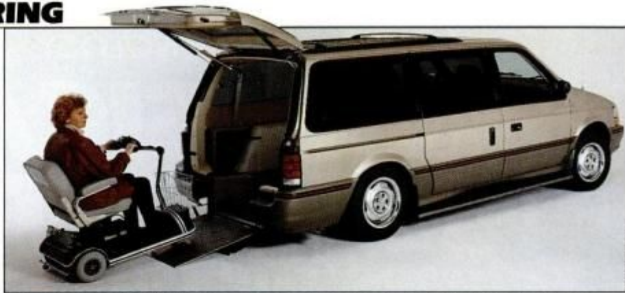
Van conversion lets driver open gate, drop ramp and hydraulically lower suspension.
