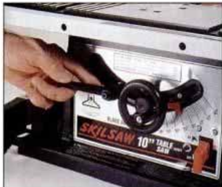
1 A crankwheel controls blade height. To adjust angle, loosen locking lever and pivot the arbor assembly manually.
