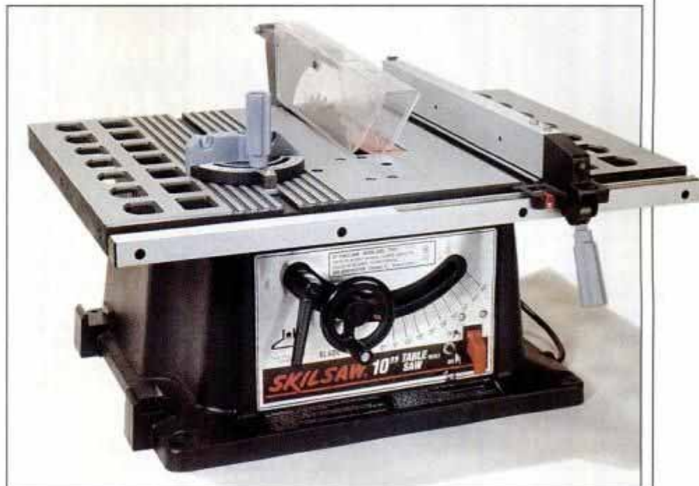
The 40-pound Skil Model 4300 benchtop table saw is designed for small shops and portability. It features a 10-in. blade, a 13-amp motor and a die-cast aluminum top.
