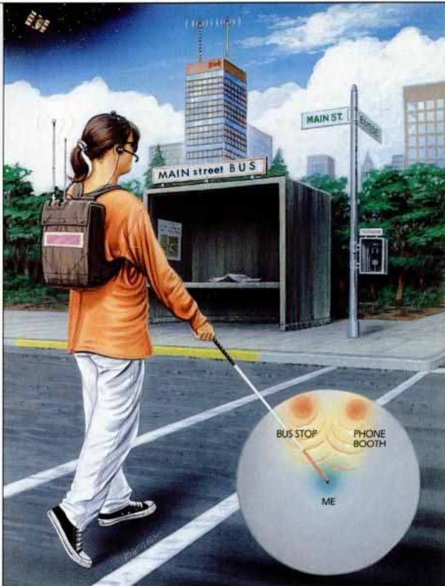
Virtual-reality technology mated to a GPS receiver are the keys to a future guidance system for the blind (above). Aural technology makes sounds emanate from particular points in space (Inset). Another device (below) uses data from a camera to stimulate microelectrodes implanted in the brain, producing the sensation of light.
