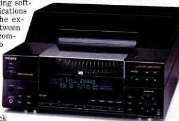
One hundred CDs are stored on a carousel inside this Sony player.
