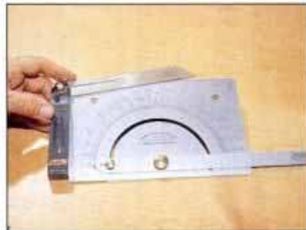
5 Using the protractor's ruled edges or the face icons, you can quickly set the angle for hand-cutting dovetails.
