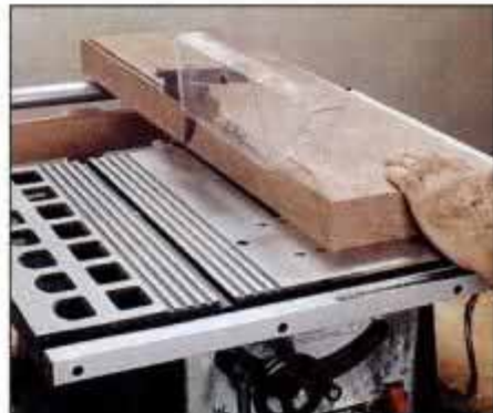
2 Blade guard with splitter and accurate fence make ripping safe and precise. The saw easily handles 2 1 / 2 -in. hardwood.
