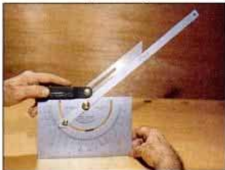
4 You can set the desired angle on a sliding T-bevel using the protractor for cases where a smaller tool is handler.
