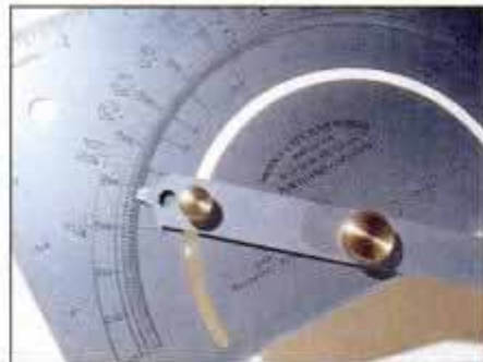
2 There is no discrepancy in setting the hairline on an angle, since the end of the indicator arm is beveled.
