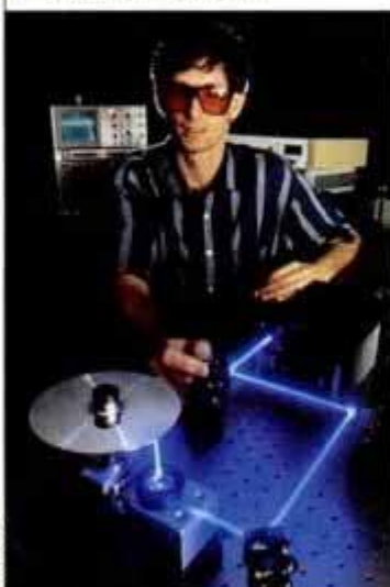
Blue laser can focus on a spot a quarter of the area of a standard infrared disk-writing laser.
