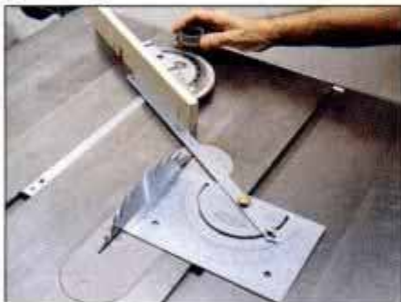
3 The sides of the protractor are ground square, allowing the tool to be used in setting up shop machinery.
