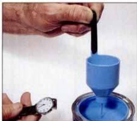
3 To determine proper finish consistency, measure the time it takes material to flow through viscosity cup. Thin if necessary.
