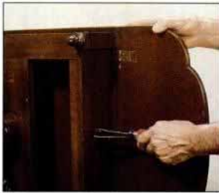
1 First, disassemble the piece and remove all hardware and metal components. Separate pieces are easier to strip and finish.
