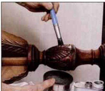
8 After the stripper has been removed, rinse away residue with recommended solvent. Don't use water on veneered work.
