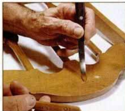
Use the burn-in method with a shellac stick to fill deep scratches, dents and gouges. Practice first on scrap stock.
