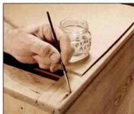
14 Where iron in nails have discolored wood, bleach the area with oxalic acid. Wash off residue when bleach has dried.
