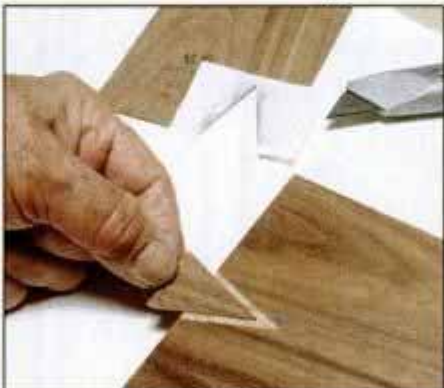
Repair chipped veneer with a patch veneer of the same species. Cut patch to fit trimmed area and stain to match.
