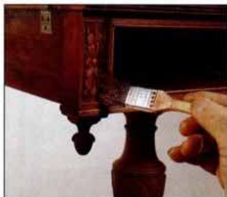
10 Use a small brush to reach crevices when staining detailed carvings and moldings. Blot up any excess with a cloth.
