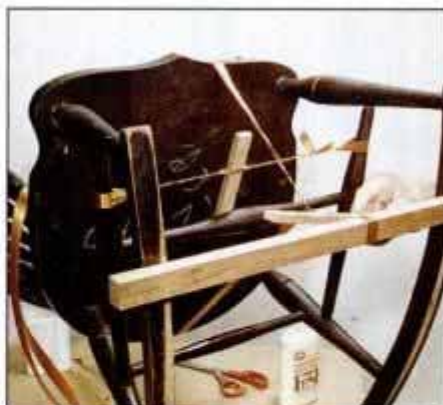
2 Apply glue to the joints and reassemble. Use a shopmade tourniquet clamp or band clamp to hold components together.
