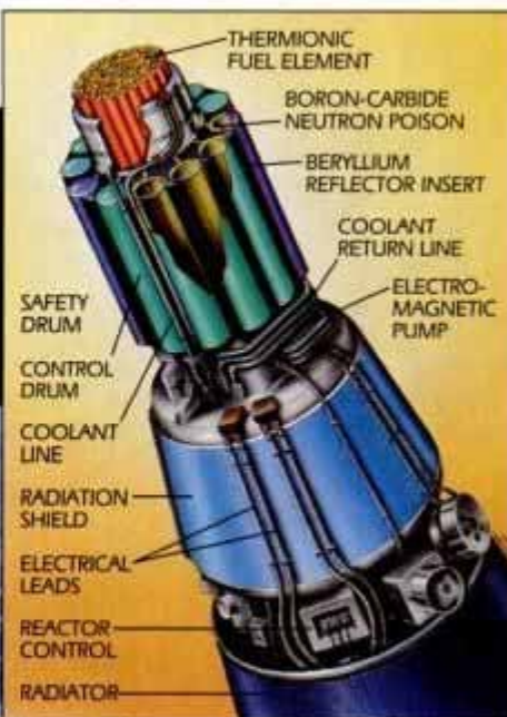
Topaz II reactor (right) will telescope out of Nuclear Electric Propulsion Space Test Program (NEPSTP) spacecraft (below).
