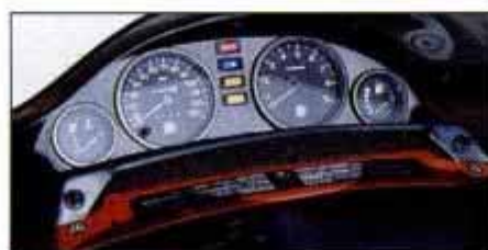
Dash panel has instruments with large numerals that are easy to read at speed.
