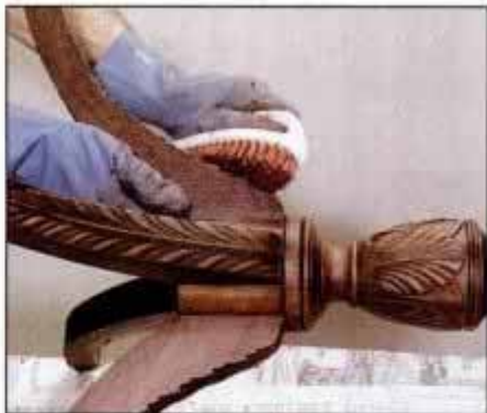
6 On larger carved areas, remove the stripper waste with a large plastic-bristle brush. Be sure to reach all crevices.
