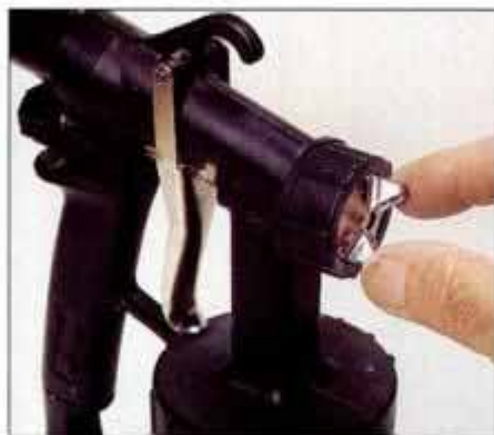
1 Adjust cap diagonally for a round spray pattern. Vertical and horizontal spray-cap positions produce elongated fan patterns.
