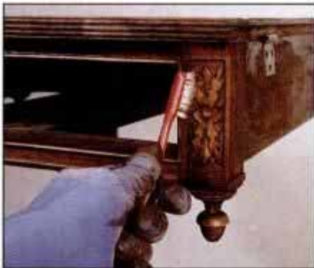
5 At small carvings and details, use an old toothbrush or small plastic-bristle brush to remove the stripper and finish.
