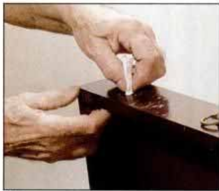
2 Use paper to plug holes left after removing hardware. This prevents stripper and finish products from dripping through holes.
