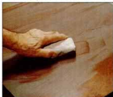
19 Begin the final rubbing with rottenstone and water. Use a soft cloth to smooth the surface, checking progress frequently.
