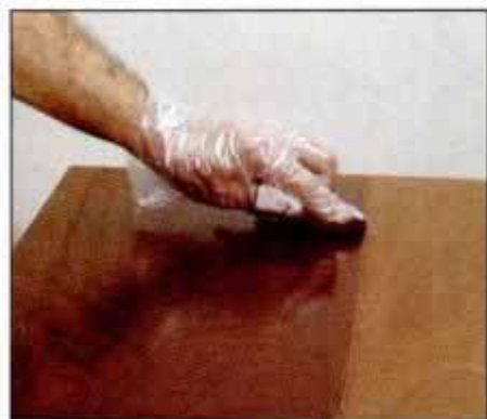
9 To color wood with aniline dye, first mix with retarder to eliminate lap marks. Apply with a soft cloth in grain direction.
