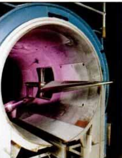
Wind-tunnel tests computer-conceived model to verify fluid-dynamics program.
