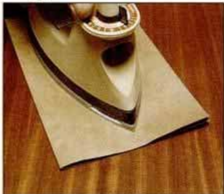
Use a clothes iron with kraft paper underneath to flatten blistered veneer. Keep the iron on medium heat.
