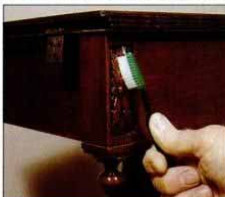
20 Use a small plastic-bristle brush to apply rottenstone to carved details. Then, clean the entire piece and let dry.
