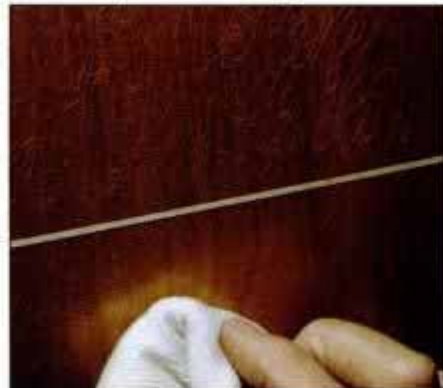
Restore alligatored lacquer by wiping with a lacquer-thinner dampened cloth. Small artist's brush handles fine scratches.
