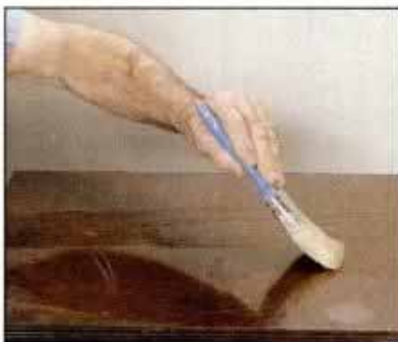
3 Use a brush to apply stripper. Non-water-base stripper is best for veneered work where water may delaminate veneer.
