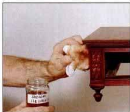
11 After the staining is done, apply a thin coat of shellac to act as a sealer and form a good base for the paste wood filler.
