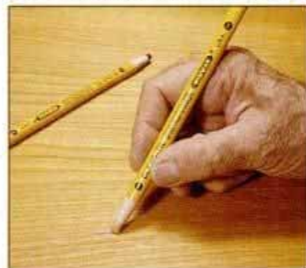
Small scratches and holes can also be filled with a wax pencil. These are available in a range of wood colors.
