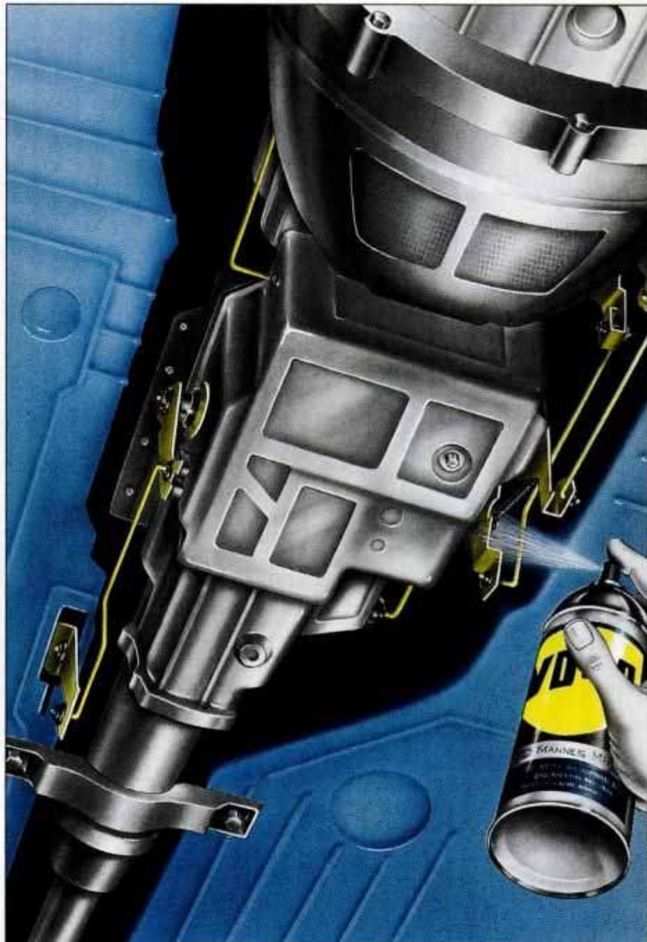
Check the operation of the various shift linkages of your automatic or manual transmission. Lubricate the pivots with a water-resistant, light lubricant.
