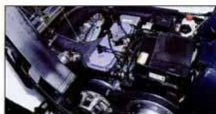
Lightweight 3-cylinder block is fitted with three 34mm Mikuni carbs.
