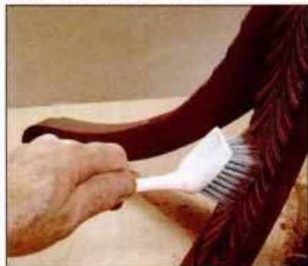
14 To remove the excess paste wood filler from crevices in carved details, use a stiff plastic-bristle brush.
