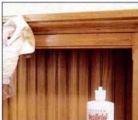
21 Apply two coats of gel clear finish with a cloth. Wipe-on finishes eliminate dust problems and visible brush strokes.
