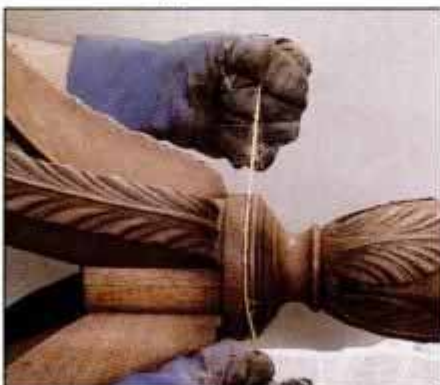
7 For detailed turnings, use coarse twine to remove the waste. Wrap twine around the turning, and pull back and forth.
