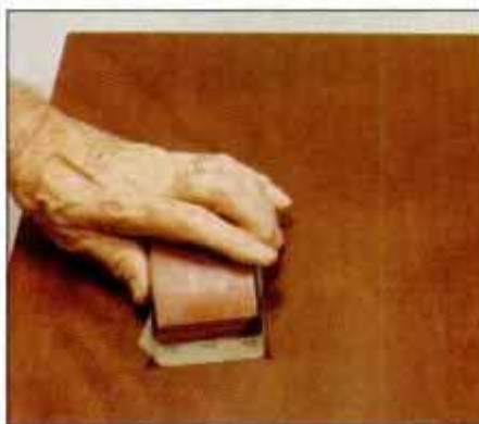
17 After the first two coats, dry-sand with 320-grit paper. Use a rubber sanding block to maintain a flat uniform surface.
