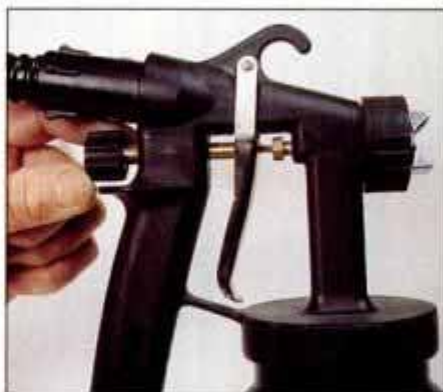
2 Control the amount being sprayed by adjusting knob at the back of handle to suit spray pattern and distance from work.
