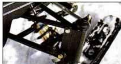
Front suspension features a double A-arm with coil spring and gas shocks.
