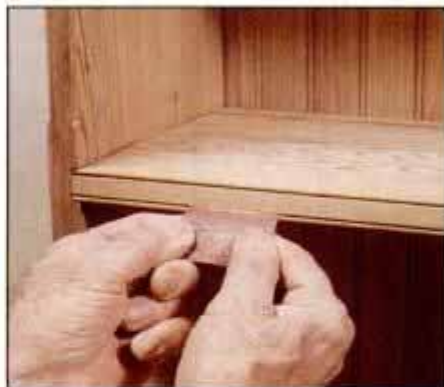
16 Hand sand tight crevices with folded sandpaper. Use a sanding block on narrow flat surfaces to avoid rounding corners.
