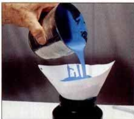
4 After checking viscosity, pour finish in spray gun cup through a strainer. This removes lumps that may clog the spray gun.
