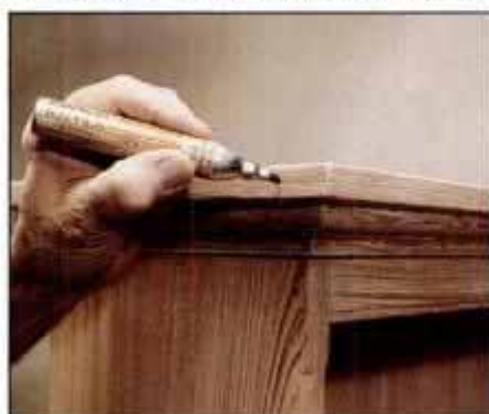
13 If wood filler color doesn't correspond to wood, use a wood-colored marker to tone filled areas so they match.
