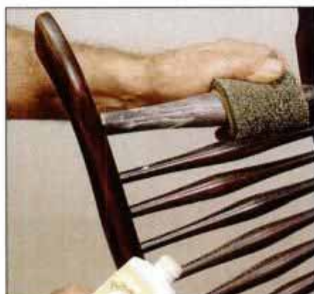
5 To clean up the chair spindles, wrap the cloth or applicator pad around them and polish along their length.
