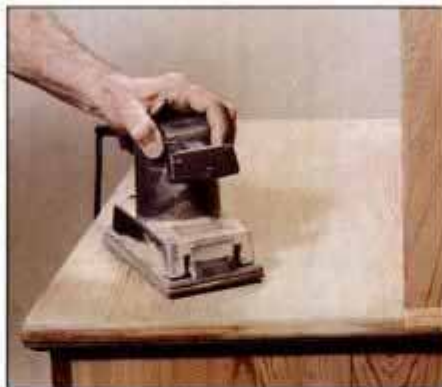
15 Use an orbital sander to speed smoothing of broad areas. Finish by hand sanding with the grain to remove any swirl marks.
