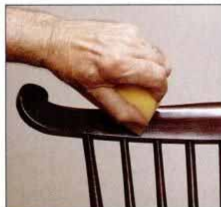
6 Apply Face Lift Finish with the felt-faced applicator pad. Wipe on the finish in thin, even coats.
