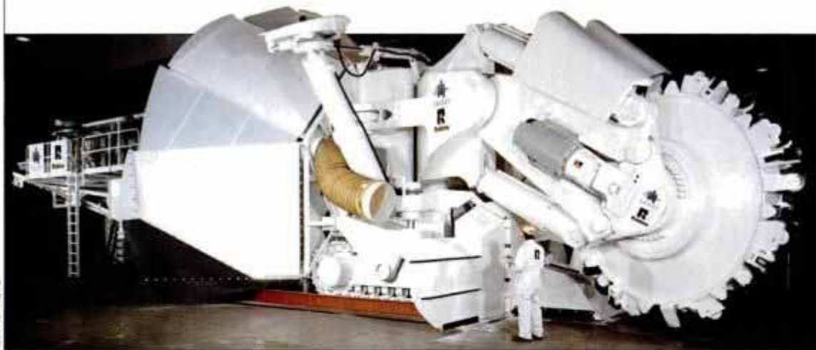
Boom-mounted cutting wheel buzz-saws out the perimeter of an arched roadway tunnel.
