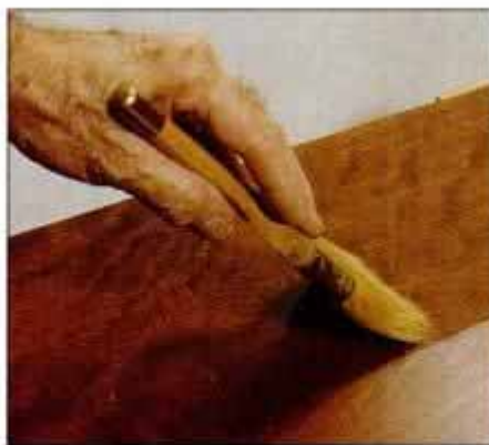
15 Fill half the bristle length with varnish and wipe excess on wire affixed to can. Flow on across grain, and then with grain.
