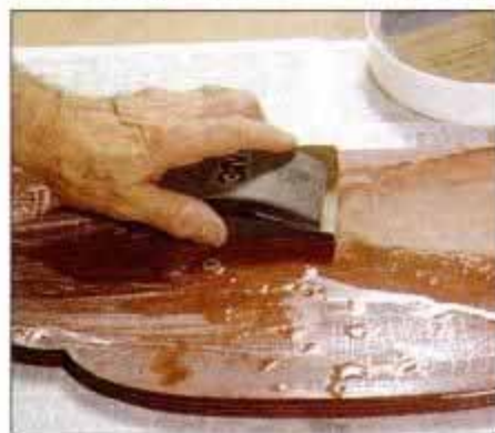
18 After the third coat, wet-sand with 400-grit paper and water. Move to 600-grit paper to wet-sand the final fourth coat.
