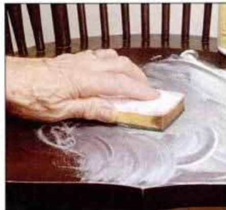
4 To remove minor surface scratches and blemishes, use a polishing compound. Rub each area for several minutes.
