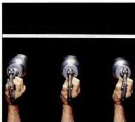
5 Always move spray gun parallel to the worksurface. Practice moving gun in a straight line to uniformly cover flat surfaces.
