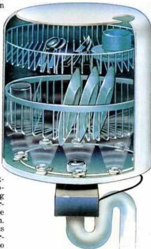
Ultrasonic dishwasher fills with water, vibrates food from dishes, then passes water through recycling loop where reverse-osmosis filter provides high-speed cleansing of contents.
