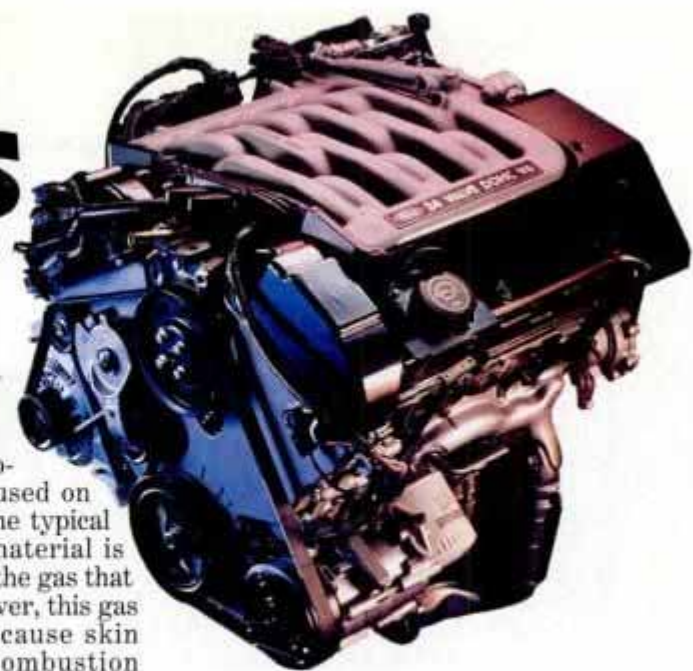
FORD'S MODULAR V6 Compact and lightweight, the dohc 24-valve modular is derived from the 4.6 V8.
