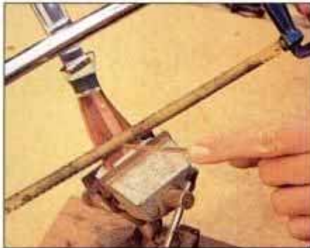
14 Insert the brass pin bar in each hole in the handle. Cut so that the pins extend \frac{1}{8} in. This enables the pins to be flared.
