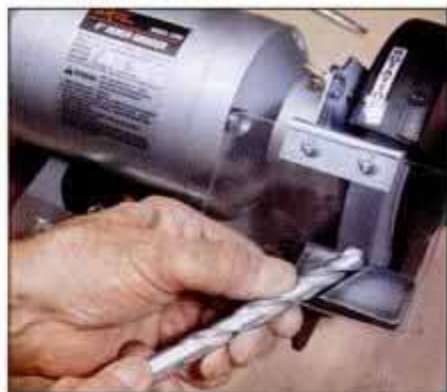
3 Use the grooved toolrest for grinding drill bits. Lift the bit and twist it to correctly shape the point.
