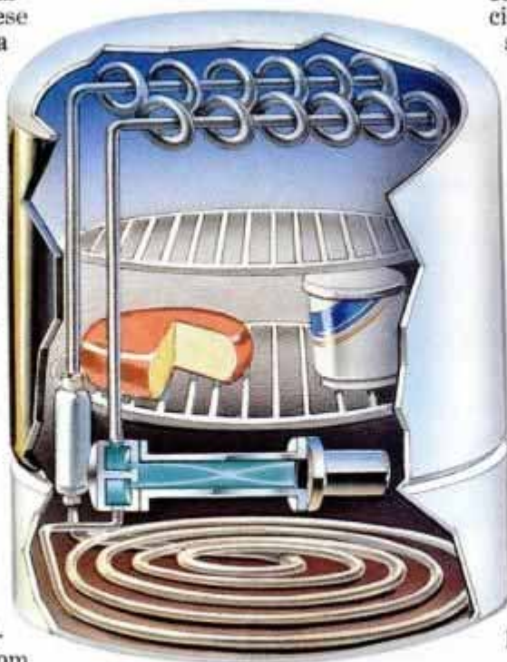
Compact refrigerator runs on a sonic compressor, which liquifies a nonchlorofluorocarbon refrigerant and opens and shuts flapper valves to distribute cooling.
