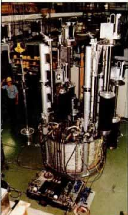
Electrorefiner (left) extracts transuranics, used to make ingot (above) for new fuel.
