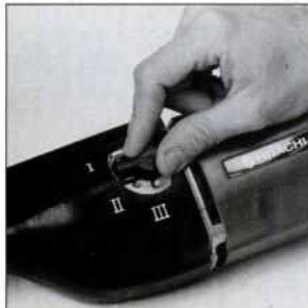
Bosch, AEG, P-C and Hitachi tools tested have orbital action plus straight cutting. Orbital action speeds cutting in wood.
