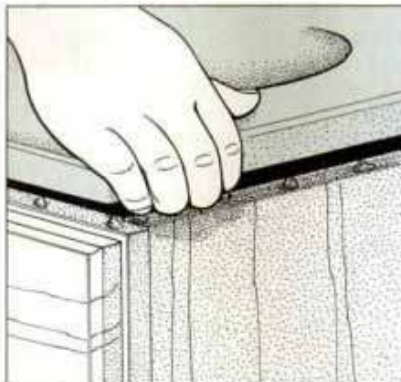
13 Place the vanity top on the base, and push it against the wall. Wipe off any adhesive that oozes from under the top.
