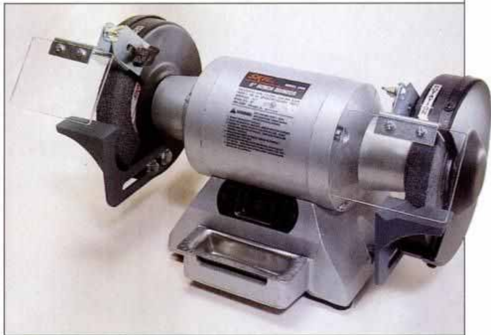
The Skil Model 3396 bench grinder performed well in a series of tests that included removing metal and grinding a cutting edge on hand tools.
