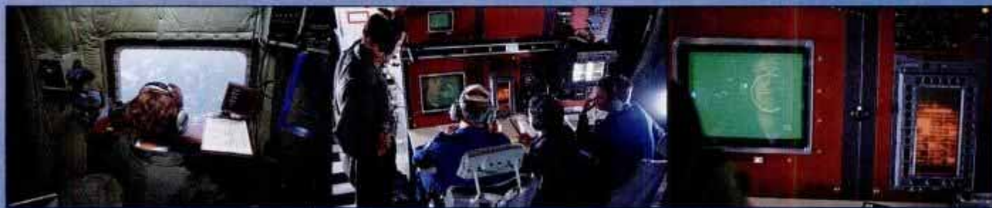
Aboard the C-130, icepicks make visual sightings (left), and radar operators man console with FLAR on left and SLAR on right.
