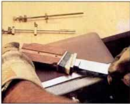
10 With all but the brass pins in place, use a belt sander to smooth the sides of the handle. Gloves and a sure grip are required.
