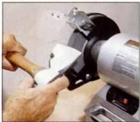
1 The grinder comes with coarse- and medium-grit grinding wheels—a perfect combination for large sharpening jobs.
