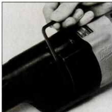
Saws require an Allen wrench to install blade. Milwaukee and AEG store wrench in housing. Others store wrench on cord.
