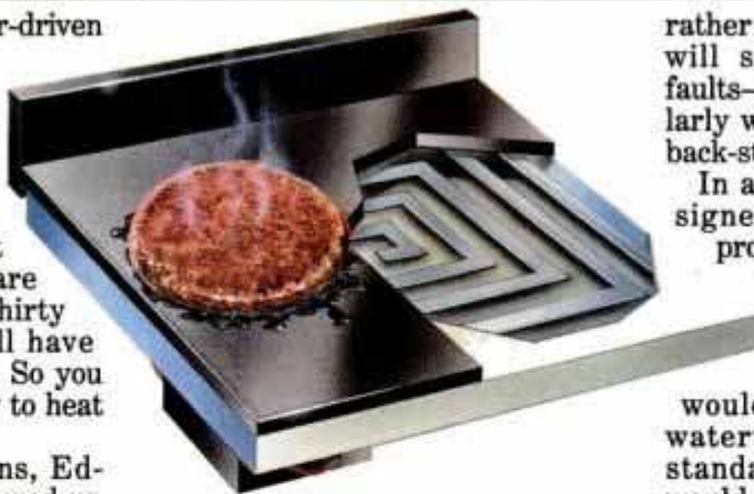
MetCal grill heats up through electromagnetic induction, provided via coil. Cooking temperature stays even because the surface's magnetic properties fade if temperature rises too high.
