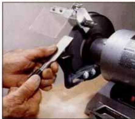
2 The machine's toolrests do not pivot. You have to learn to use a rest as a fulcrum while grinding edge tools.
