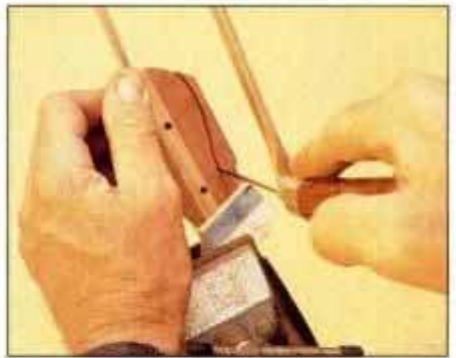
12 Carefully cut along the pencil line with a coping saw to create the rough shape of the handle. Only fine work remains.
