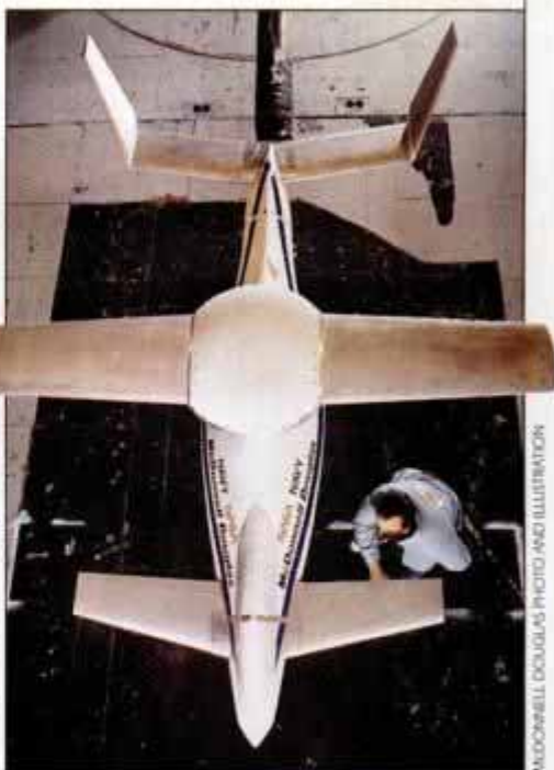
Canard rotor/wing 75%-scale model (right) undergoes testing in NASA-Langley's wind tunnel.
