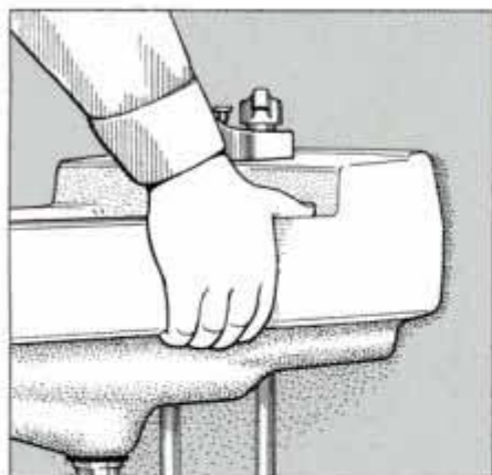
4 With all the plumbing connections undone, lift the sink from its sides and pull it clear of its wall bracket.
