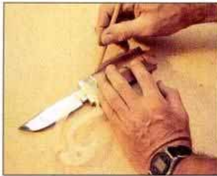
11 Draw a profile of the handle using a template based on the photos in this story, or create one by using a French curve.
