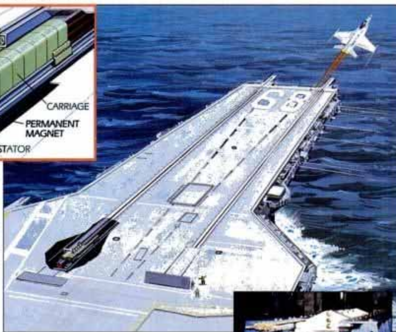
Electromagnetic catapult system minimizes on-deck equipment.
