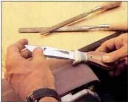
13 Use a belt sander to round out the shape of the handle. Always use gloves. This shot was done just for the camera.
