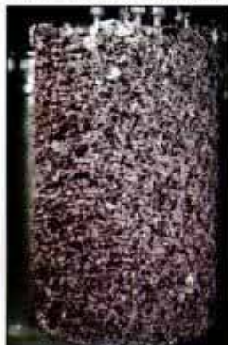
Electrorefiner (left) extracts transuranics, used to make ingot (above) for new fuel.
