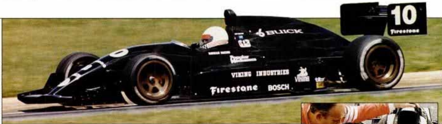
New Lola T93/20 chassis will carry Firestone Indy Lights racers through the '95 season. Race-prepared stock-block Buick V6 engine produces 425 horsepower.
