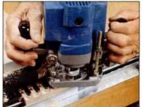
11 With dovetail bit and guide bushing in router, follow the dovetail template. Both pieces are cut in one operation.
