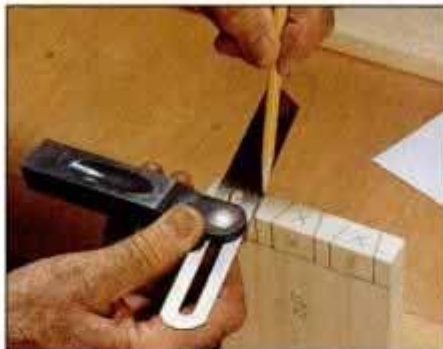
1 After laying out the pin spacing on the face of the stock, use a sliding bevel gauge to mark the dovetail angles.
