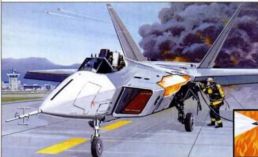
Drill punctures composite skin and snuffs fire without exposing flames to more air.
