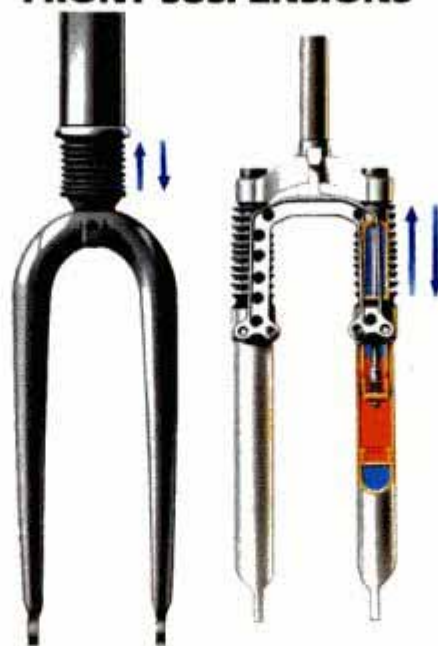
The modern era of suspended bikes was born with telescoping forks (right). New is Cannondale's single shock above the crown.
