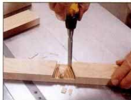
15 Cut the adjoining half lap by making successive passes at the dovetail angle from each side. Clean up with a chisel.
