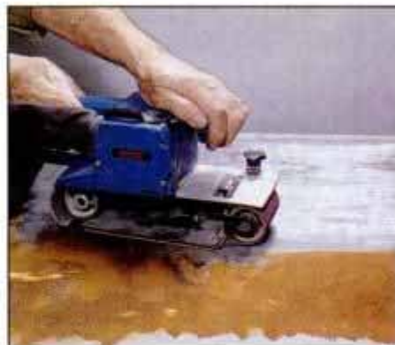
5 A belt sander is an effective rust stripping tool, especially on large flat workpieces clamped to a bench.
