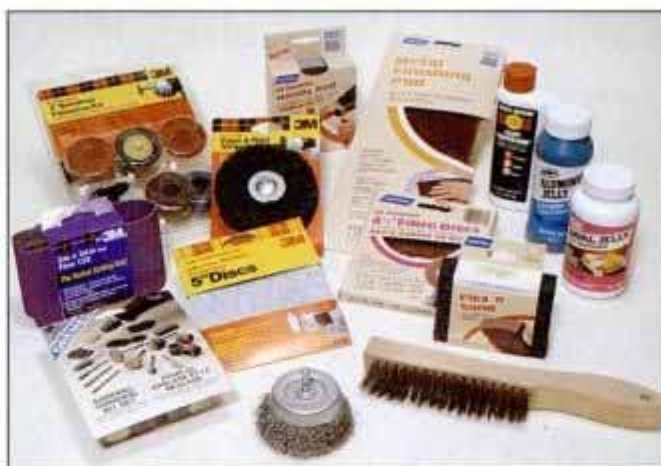
1 A survey of rust-removal products (clockwise from left): abrasive stones in various shapes and abrasive sanding sleeves that chuck into a Dremel motor tool, sander belts, discs that chuck into a hand drill, abrasive strips and pads that you use by hand, wire brushes and chemical corrosion treatments. Don't forget to wear eye protection when using these tools.
