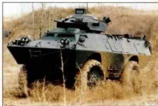
Versatile V-150 runs on diesel V8 and features unitized body of steel plate.
