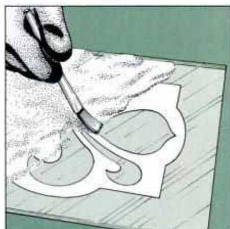
6 With newspaper or a plastic sheet under the work, apply acid cream to the glass and let it stand for 10 minutes.
