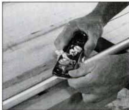
20 The seat support rails are made from birch dowels. Clamp a rail to the bench and plane a flat on one face.
