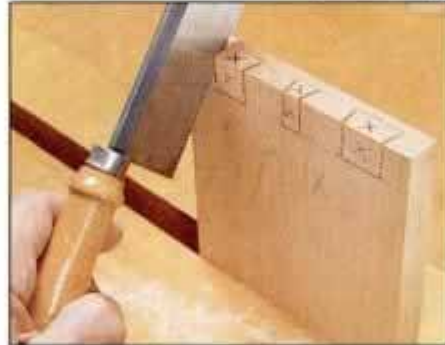
8 With pin layout lines in place, hold the backsaw at an angle and follow angled end lines and parallel face lines.
