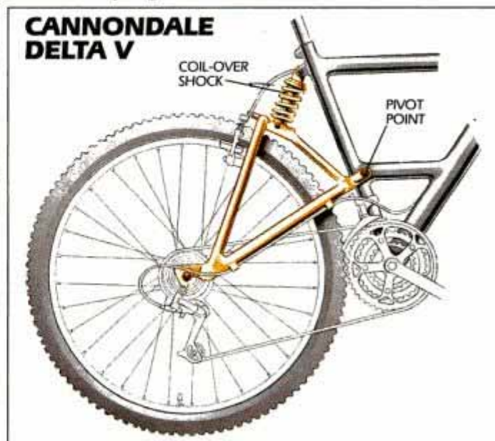
The Delta V's triangulated swing arm has a single pivot point on the seat tube above the crank spindle.
