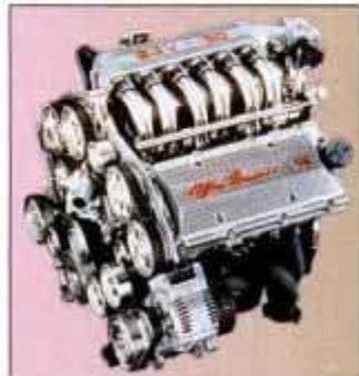
New dohc 24-valve cylinder heads give Alfa's 3.0-liter alloy V6 a 15% boost in horsepower.
