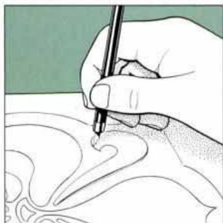
4 Use a sharp razor knife to cut the stencil. A swivel-blade knife is best for patterns that have many curved lines.
