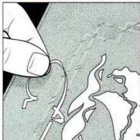
14 When you're satisfied with the results, remove the remaining stencil material and clean the glass surface.
