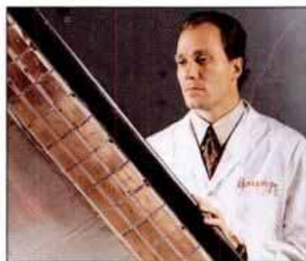
Boeing tested a 1/5-scale model of the EX's conformal radar (above). Three-view (below) shows how the joined wing provides unobstructed radar vision.
