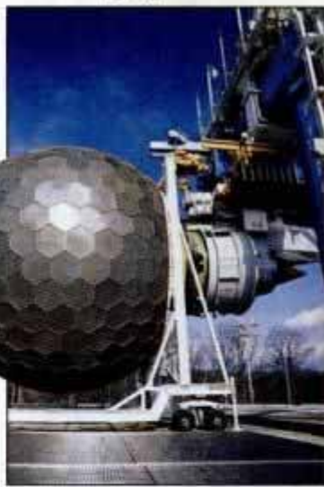
Giant golfball structure smooths out airflow during intake tests of GE90 turbofan.
