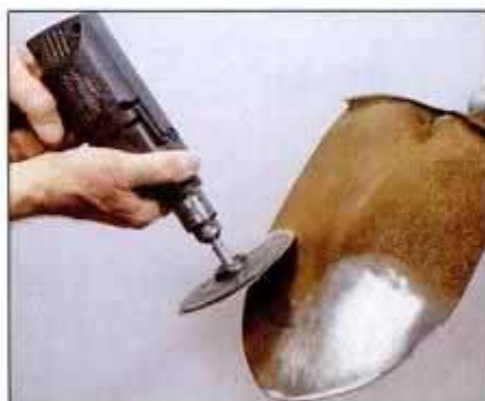
3 Use the upper third of a disc sanding attachment when using an electric drill to strip rust on curved surfaces.
