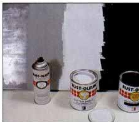
6 To stop saponification, use a specialty coating, like Gutter Shield, between the zinc primer and the topcoat.
