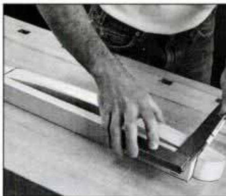
17 Prior to boring postholes, mark the posts' positions on the rockers, using a square and a square.
