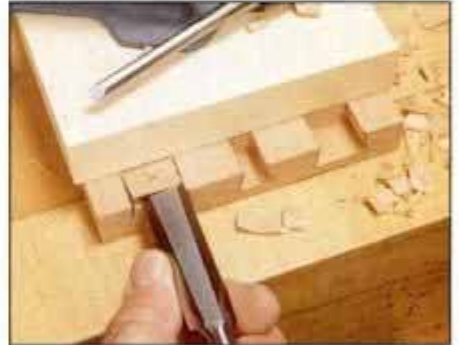
9 Remove waste from pin sockets with a chisel. Make alternating cuts—first across the grain and then with the grain.
