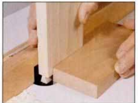
13 Shape mating piece by routing both sides of work with a dovetail bit. Test fence position on scrap stock first.
