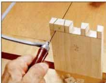
3 After the pin sides are finished, remove most of the waste with a coping saw. Cut almost to the baseline.
