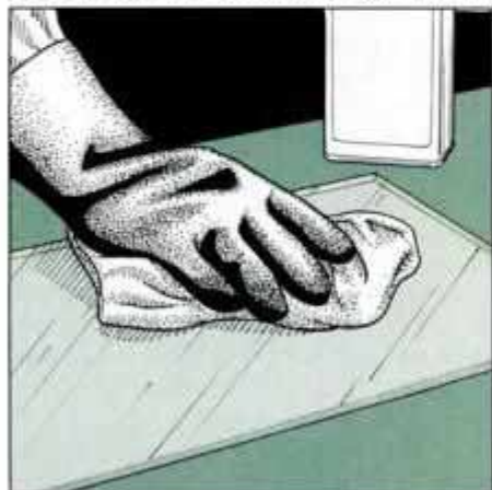
1 To prepare for acid etching, first remove oil and dust from glass by wiping with alcohol. Then, allow to dry.
