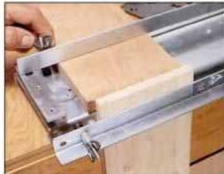
10 A typical dovetailing jig cuts half-blind and through dovetail joints. Clamp stock in jig with pieces offset.
