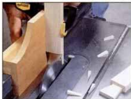
14 After the half lap is cut, angle blade and cut dovetail sides. Use a tenoning jig to safely hold workpiece vertically.
