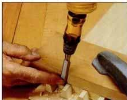
4 Clamp a guide board at the baseline and use a chisel to trim the sockets. Trim halfway down, then reverse the work.
