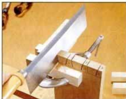
6 Cut to the waste side of the dovetail lines with a backsaw. Remove waste with a coping saw and trim with a chisel.
