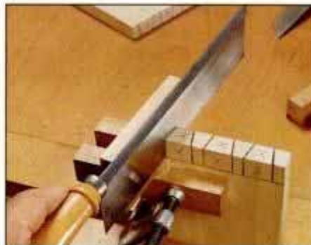
2 Use a backsaw to begin cutting the pins. Stay to the waste side of the line. A shopmade guide block helps accuracy.
