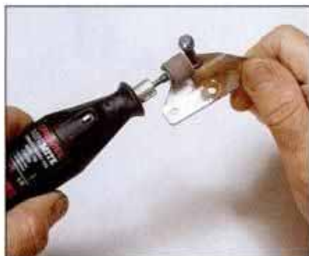
2 A Dremel tool can strip rust with a drum and an abrasive sleeve. Small parts can be held while the rust is removed.
