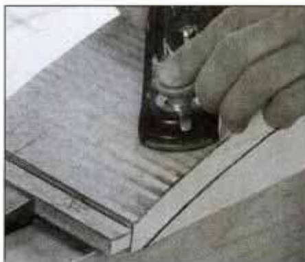
12 Remove the saw marks from the outside of the backrest using a block plane and a scraper.
