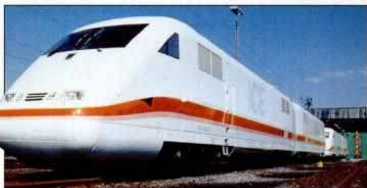
Extruded aluminum panels give ICE its unique seamless profile.
