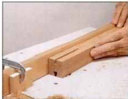
12 After preliminary groove is cut with a straight bit, use a dovetail bit to rout dovetail channel for a sliding dovetail.
