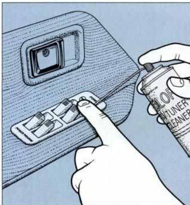
Electrical contact cleaner can remove current-blocking dirt and corrosion from contacts with the switch in place.
