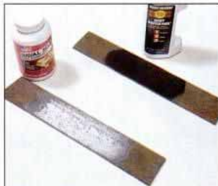
10 Naval Jelly dissolves rust so it can be stripped (left), while rust converters change it into a paintable oxide.
