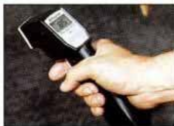
Teams strip engines to bare componentry between rounds of racing. Critical adjustments will be made to the multidisc clutch that has replaced the transmission (left) while handheld noncontact thermometers are used to check track and tire prior to racing.
