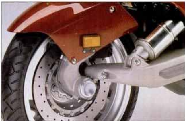
Stripped of bodywork, GTS1000A clearly shows its compact design with weight low and centered between the wheels for stable handling (above). Hub-ster front suspension incorporates anti-dive geometry and mounts front disc brake on wheel centerline for straightahead stopping (left). Six-piston front brake caliper provides unbelievable stopping power (below).
