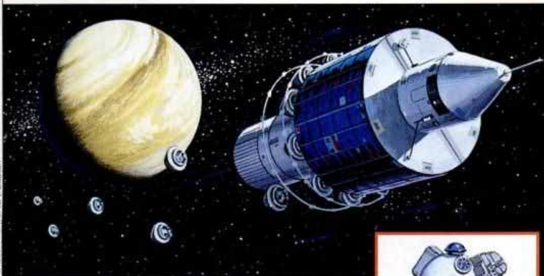
Venus Multiprobe Mission will scatter aerobrake-shielded probes into the planet's caustic atmosphere.
