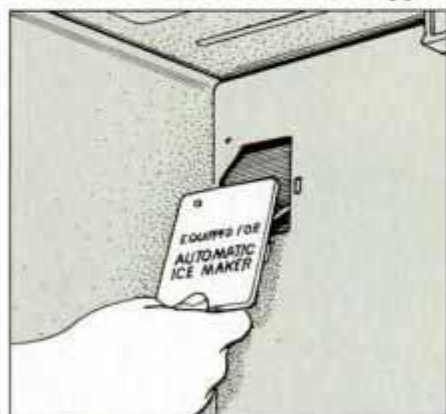
1 Begin by removing the cover plate inside the freezer. Back out the fastening screw, and remove the plate.
