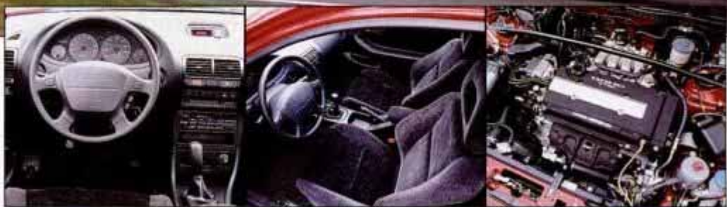
New dashboard, seats and 170-hp 1.8-liter dohc 16-valve VTEC distinguish new Integra GS-R.
