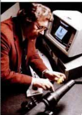
Zero-expansion composite body houses ultra-precise X-ray microscope.
