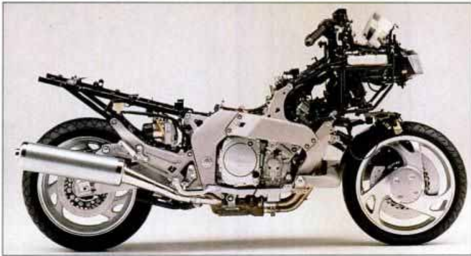
Stripped of bodywork, GTS1000A clearly shows its compact design with weight low and centered between the wheels for stable handling (above). Hub-ster front suspension incorporates anti-dive geometry and mounts front disc brake on wheel centerline for straightahead stopping (left). Six-piston front brake caliper provides unbelievable stopping power (below).
