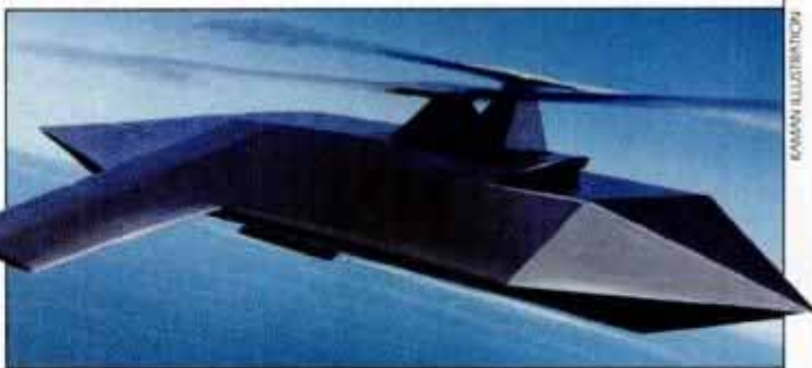
An all-electric unmanned rotorcraft, Spyglass could carry out stealthy reconnaissance missions using intermeshing rotors.
