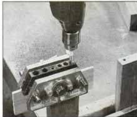
1 Bore the dowel holes in the top rail. Offset a self-centering doweling jig using a thin piece of wood.
