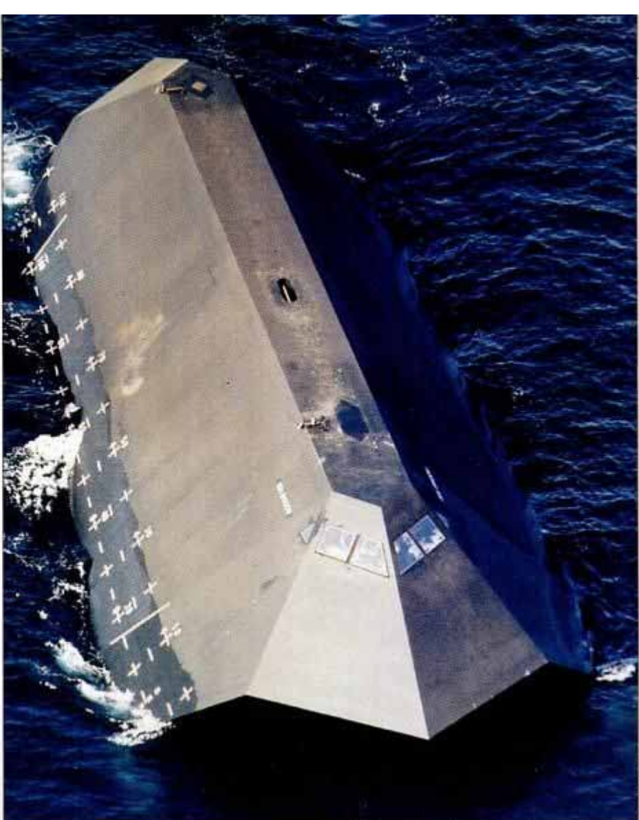
From above, hexagonal hatches are visible at each end of the Sea Shadow's weather deck, with what may be an air intake between. Front hatch aids docking operations, such as entering the Hughes Mining Barge (below).
