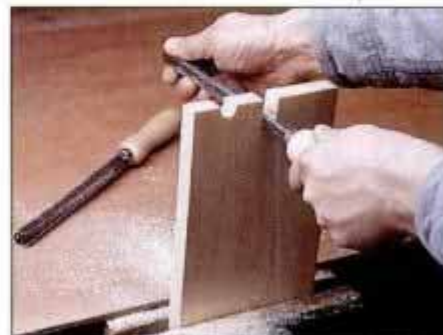
Handled rasps are either round or square. Aggressive cutting removes stock at the rate of 1/4 in. on each pass.
