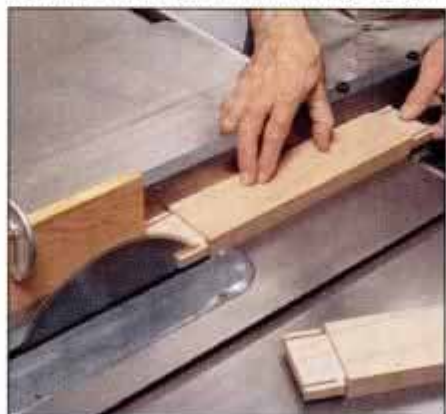
9 Cut narrow cheeks by ripping toward the shoulder. Stop the kerf short of the shoulder and remove waste with a chisel.
