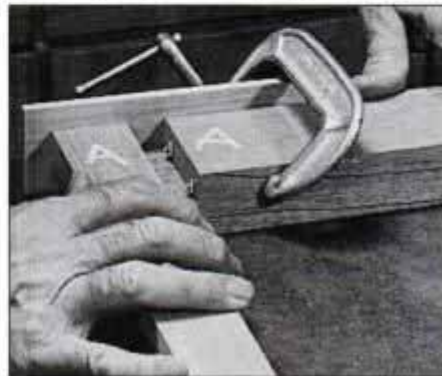
4 To mark the dowel holes in the legs, insert dowel centers in the top rail and press the rail against the leg.
