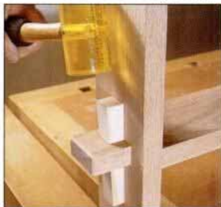
14 Make a pin to fit tapered mortise and tap it in place with a mallet. Here, joint secures trestle table leg to stretcher.
