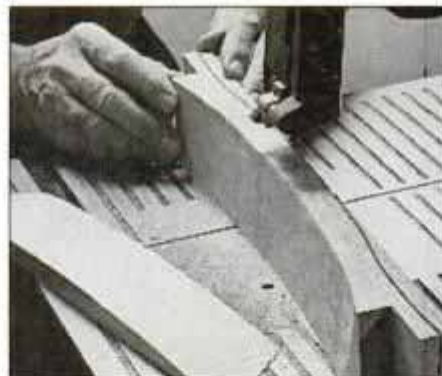
5 Tip the band-saw table to 7°. Cut just to the waste side of the line and save the cutoff pieces.
