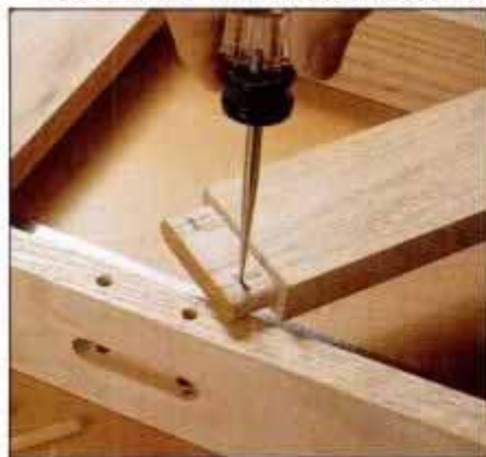
11 Use dowel pins to lock the tenon in place. Bore holes in the tenon slightly closer to shoulder to draw the joint tight.
