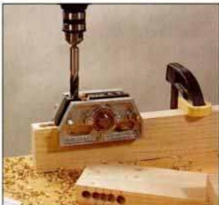
3 If you don't have a drill press, use a doweling jig and brad point bit to remove most of the mortise waste.
