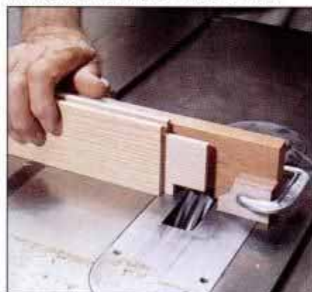
10 Use a stop clamped to an auxiliary fence to position tenon for cuts with dado blade. Here, a haunched tenon is cut.
