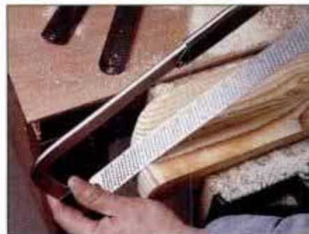
The flat, flexible rasp excels at shaping convex curves in wood. A second flat rasp is rigid for handling straight cuts.
