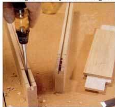
12 When cutting mortises in grooved stiles, use groove as a guide. Haunched tenon fills the gap left by the groove.
