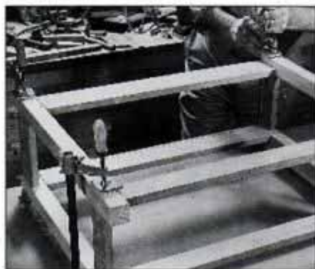
20 Glue and clamp the legs to the long aprons. Then glue and clamp these subassemblies to the short aprons.
