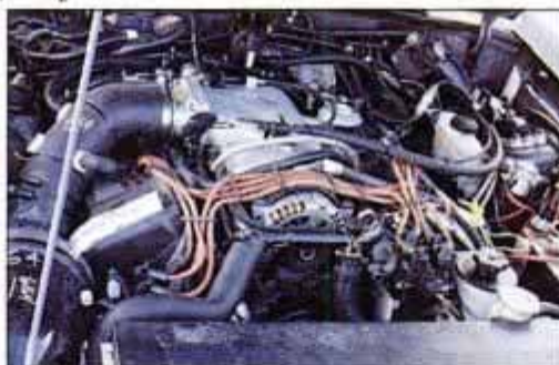
Ford's 4.6-liter V8 makes for a crowded Mustang engine bay.
