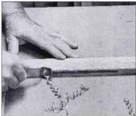
11 Round the corners on the legs, except where they meet the rails. This is done quickly with a cornering tool.
