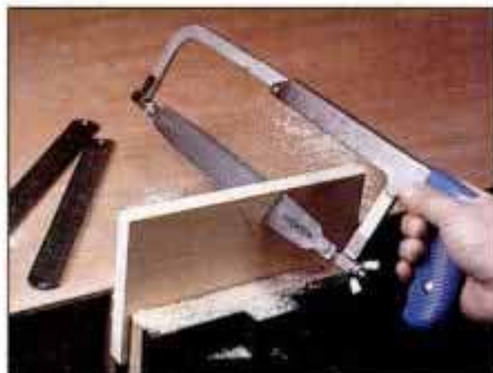
The double-edge, thin-kerf saw blade has a curved profile for fast cutting. One edge is coarse and the other, fine.
