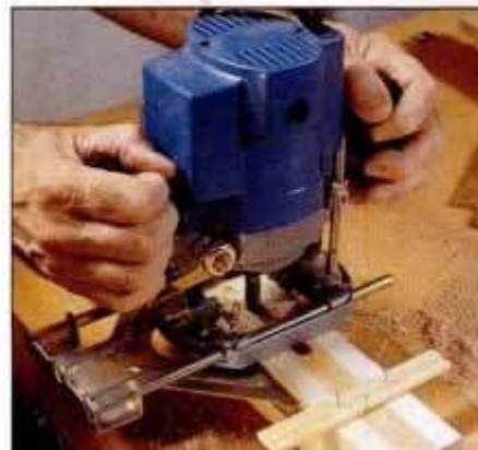
5 Set plunge router fence to align the bit and use stops to limit router travel. Make several passes to remove waste.
