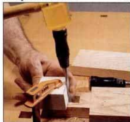
13 To make a tapered mortise for a keyed tenon, use an angled block to guide the chisel after mortise is first cut square.
