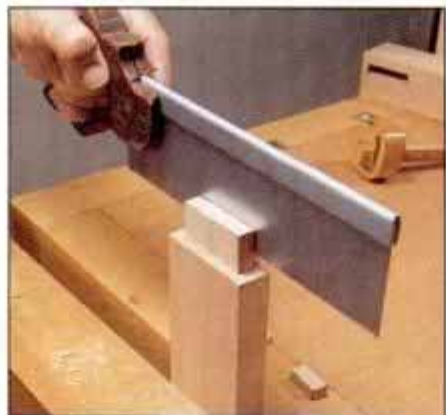
6 To cut a tenon by hand, first cut the shoulders. Then cut to cheek lines and trim shoulders square with a sharp chisel.
