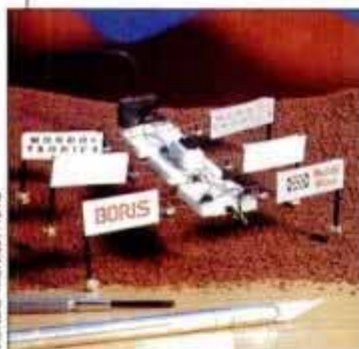
Boris the spider, choreographed by a microprocessor, walks with muscle wires.
