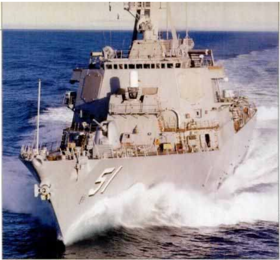
The Navy says experience from the Sea Shadow was used in sculpting the Arleigh Burke's low observable shape (top) and in designing the TAGOS-19's SWATH hull (below).
