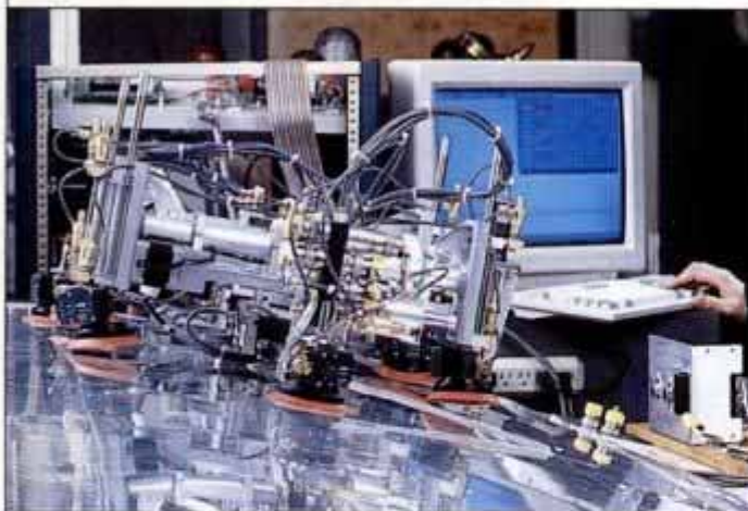
Automated skin-panel inspector inches its way along aircraft seeking cracks and corrosion.
