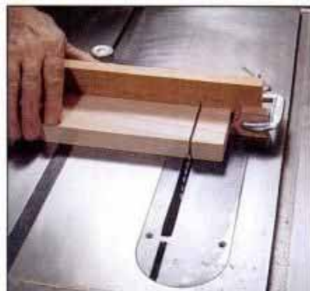
7 With a standard blade in table saw, first cut tenon shoulders. A stop on auxiliary miter-gauge fence positions the work.
