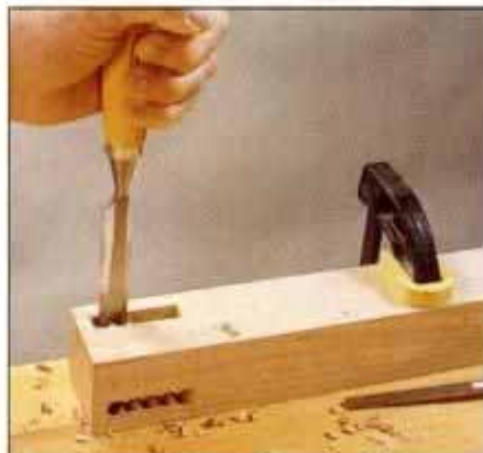
4 Trim roughed-out mortise to guidelines with a sharp chisel. Keep the sides parallel and square to the stock face.
