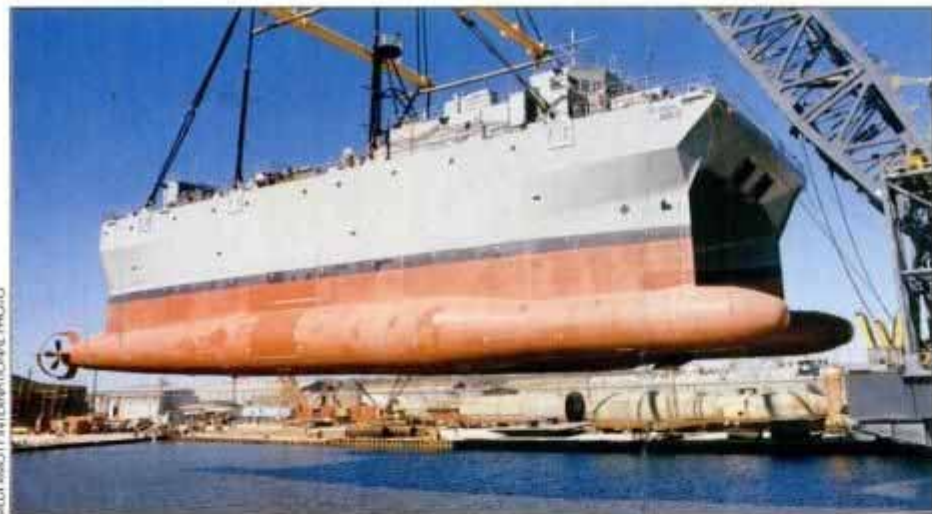
The Navy says experience from the Sea Shadow was used in sculpting the Arleigh Burke's low observable shape (top) and in designing the TAGOS-19's SWATH hull (below).
