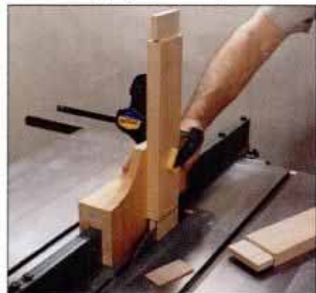
8 Use a table saw tenoning jig to cut broad tenon cheeks. Align the work so waste falls away from the saw blade.
