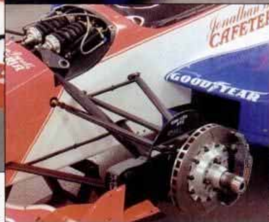
The POPULAR MECHANICS/Dick Simon Racing Lola driven by Scott Brayton is standard, state-of-the-art Indycar weaponry. Built to the '93 rules, the Lola chassis has a carefully contoured aero bottom tub (top right), plumbing work tucked under the side pods (center right) and massive outboard front disc brakes (bottom right).
