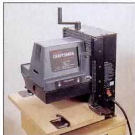
3 Sears planer also accepts molding knives. Open-side design permits molding the edges of a wide board.
