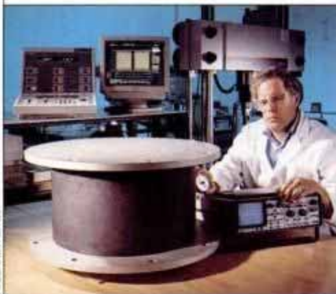
Seismic isolation bearings display extraordinary shear strength.
