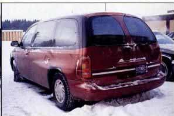
New front-wheel-drive Ford Windstar will use the Taurus drivetrain, eventually replacing the current rear-wheel-drive Aerostar minivan.
