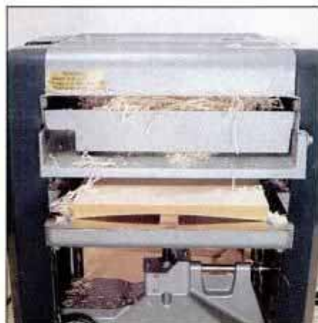
7 The shim supports the center of cupped stock and eliminates any bending caused by feed-roller pressure.
