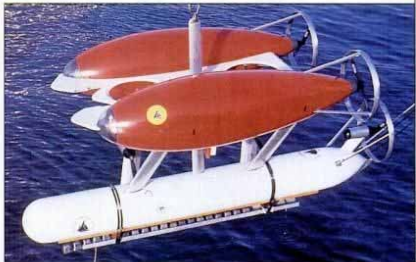
Struts connect twin buoyancy tanks, each containing three glass spheres, with ABE's 8-ft.-long instrument housing, for a stable triangular configuration.
