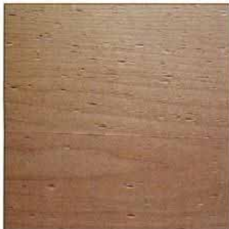
17 Chips of wood that adhere to the feed rollers cause pockmarks in a planed surface. Clean rollers with alcohol.
