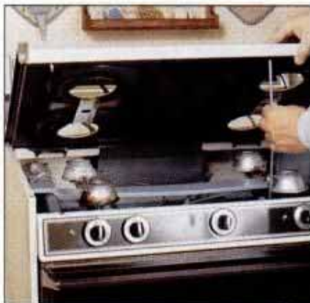
4 To inspect the burners and pilot light on a gas-fired range, lift its top and prop it up with a rod.
