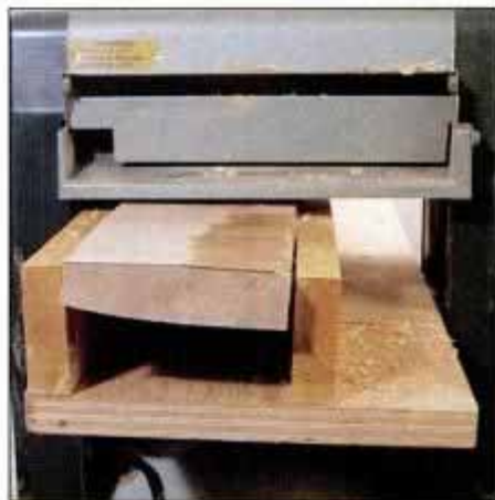
11 Make successive passes to flatten twisted surface. Initial passes may have to be hand fed due to irregular worksurface.
