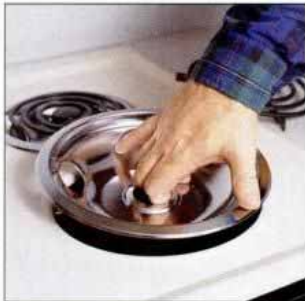
9 After removing the heating elements, lift out and clean the reflecting pan and the surface below the pan.
