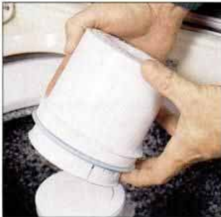
18 The reservoir should lift free of the agitator shaft. Clean the reservoir in the sink using warm water.
