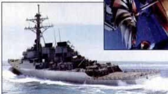
Future Arleigh Burke-class destroyers may be first vessels to feature the WR21, based on RB211 (above right).
