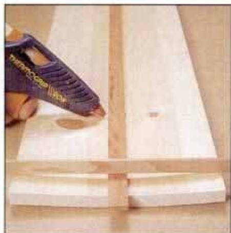
6 To flatten cupped work on a thickness planer, secure a shim on the concave side. Shim height lines up with stock edges.
