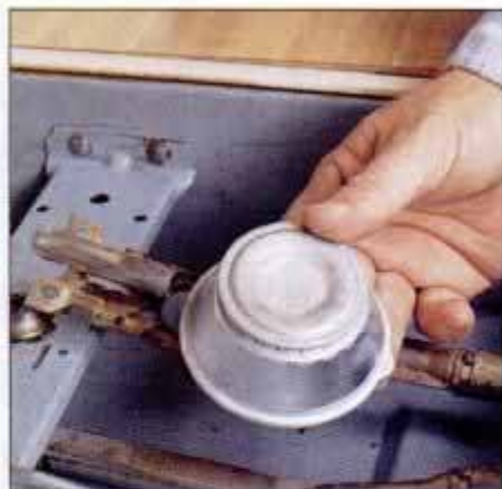
7 Gas burners are not held in place with fasteners. Lift them out to inspect and clean them.
