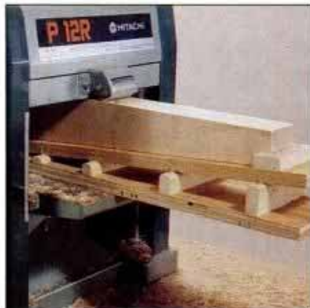
23 Plane long tapers with a jig that holds stock at the correct angle. This jig is hinged at one end for a range of tapers.
