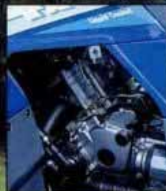
KAWASAKI BAYOU 400 The Kawle's big engine (left) is liquid cooled and has a cold-start carburetor primer pump. Note the steel external oil lines to prevent leaks.
