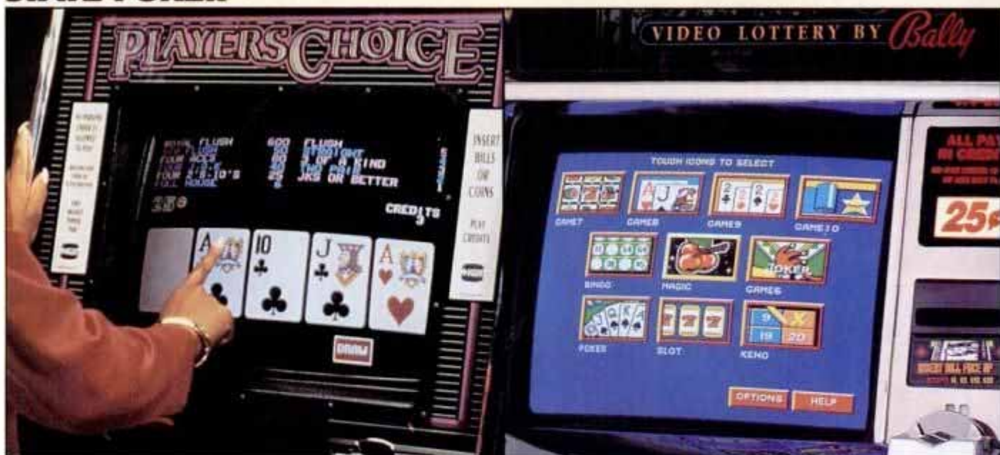
The cornerstone of video lottery is a touch-sensitive screen that allows a player to make choices quickly. Since the number of machines installed at each location is limited, one machine offers a multitude of games. Bally's V7000 machine (above right) offers 10 games.
