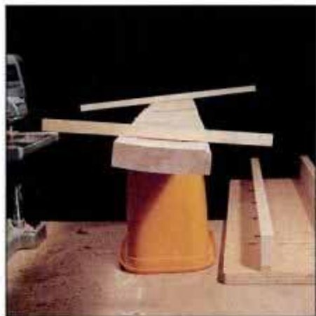
9 To check for twist, lay a straight stick at each end of the work. If the sticks aren't parallel, the board is twisted.
