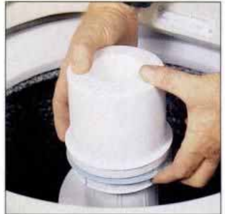
17 To release a soiled and sticky fabric-softener reservoir, lift up on the friction ring (in blue).
