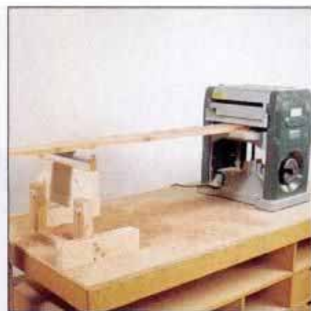
5 Long or heavy stock requires the extra support of adjustable roller stands at infeed and outfeed sides of planer.
