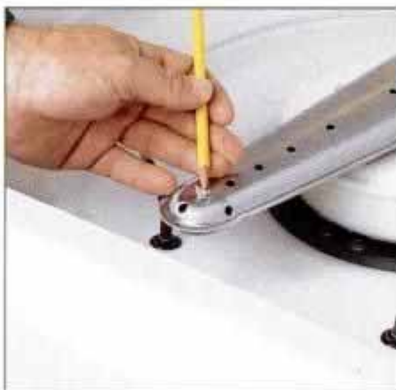
14 Check the holes in the spray arm to be sure none are clogged. Here, a small piece of shredded plastic blocks a hole.
