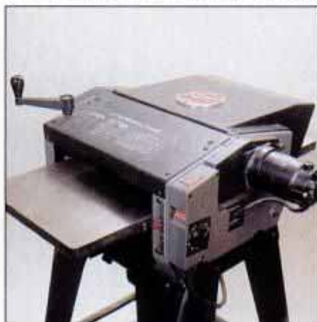
2 Shopsmith thickness planer features separate motors that drive the cutterhead and feed rollers so feed rate is variable.
