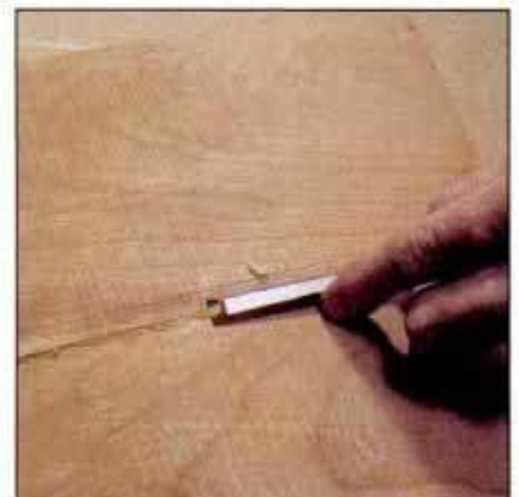
19 In addition to nails and other particles, glue lines can wear nicks in knives. Remove excess glue before planing.
