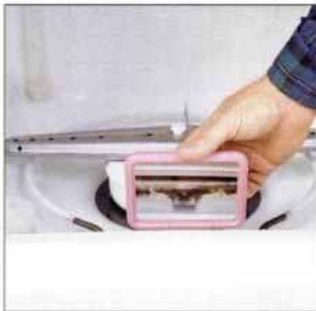
12 Use a hand mirror to check for a slimy accumulation along the bottom door gasket on a dishwasher.
