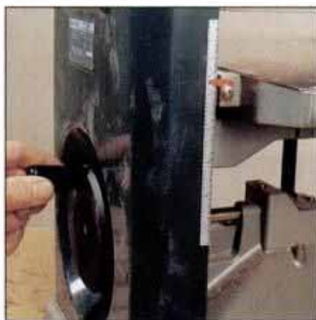
4 Planer thickness setting is adjusted with a wheel that controls table height. Pointer indicates thickness on a scale.
