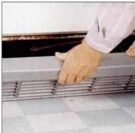
1 The grille is held to the refrigerator with clips. Snap out the grille to access the condenser coil.
