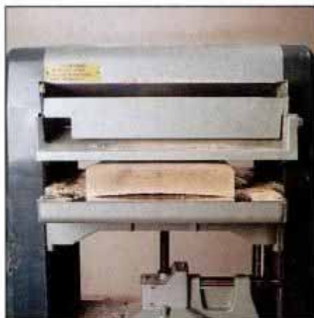
8 Heavy cupped lumber is often strong enough to resist feed-roller pressure. Always plane convex side first.
