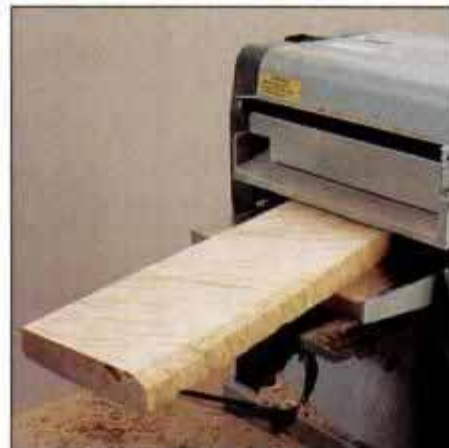
15 For wild or reversing grain, feed the work through diagonally for a smoother cut. Make shallow passes.
