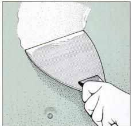
13 Use Dri Mix base compound for the first coat over the fasteners. Then, apply a second coat of joint compound.
