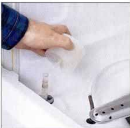
13 Lift off the water-level float and clean the tube the float rides on. Dirt can cause the float to malfunction.
