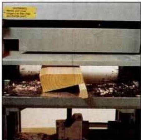
22 To plane shallow bevels, secure a shim along the edge. Take shallow passes so feed rollers don't flip up stock.
