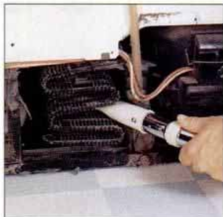
3 Also vacuum the evaporator coil and compressor. Often these are located at the back of the refrigerator.
