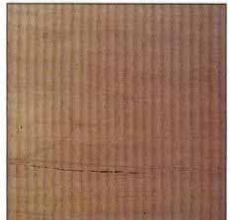
16 Washboarding, or ripples across the board, is caused by coarse knife cuts. Check that knives are at the same height.
