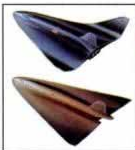
Original waverider wind-tunnel shape (below) has evolved to model two different configurations with realistic control surfaces.
