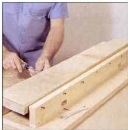
10 Adjustable jig holds twisted stock so it can be planed flat. Drywall screws placed in sidewalls hold work securely.
