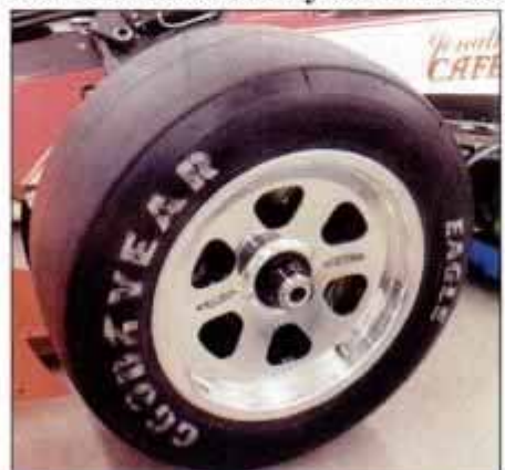
Flush-faced aerodynamic wheels are now banned in favor of open-faced alloys.
