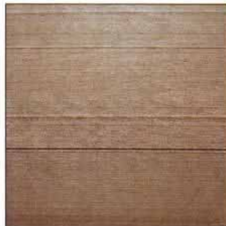
18 Ridges that run along the length of the work are caused by nicks in knives. Resharpen knives to eliminate problem.
