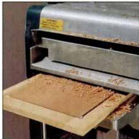
20 Plane thin stock by gluing it to a flat, parallel backer board. Apply the glue at the infeed end of the work only.
