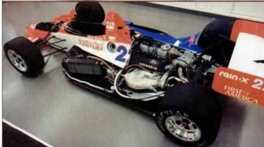
The POPULAR MECHANICS/Dick Simon Racing Lola driven by Scott Brayton is standard, state-of-the-art Indycar weaponry. Built to the '93 rules, the Lola chassis has a carefully contoured aero bottom tub (top right), plumbing work tucked under the side pods (center right) and massive outboard front disc brakes (bottom right).
