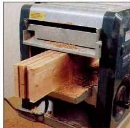
24 Trim several pieces to width by ganging them together and feeding them through the planer at the same time.
