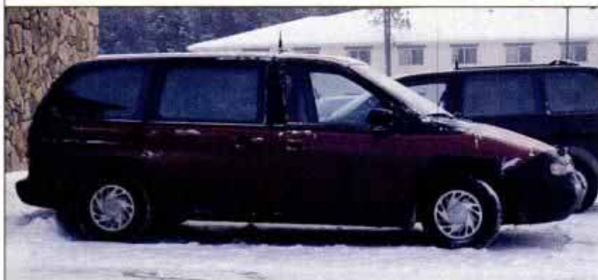
New front-wheel-drive Ford Windstar will use the Taurus drivetrain, eventually replacing the current rear-wheel-drive Aerostar minivan.
