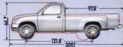
Expanding on a good idea: size relation shown between Toyota T100 2WD and Compact 2WD.
