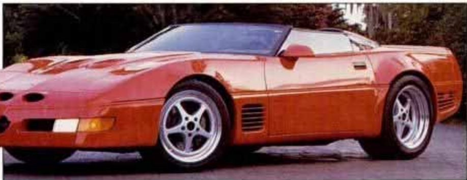
Callaway twin-turbo super Vette boosts ZR-1 V8 engine output to 750 horsepower.
