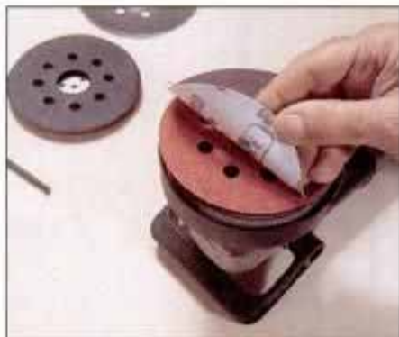
Sander comes with pressure-sensitive pad, but hook-and-loop pad is available. Disc holes are for dust collection.
