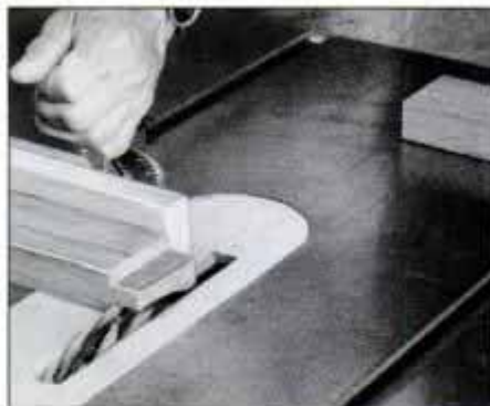
2 Clamp a stopblock to the saw table. Butt each workpiece that will have a tenon to the block and cut the tenon.
