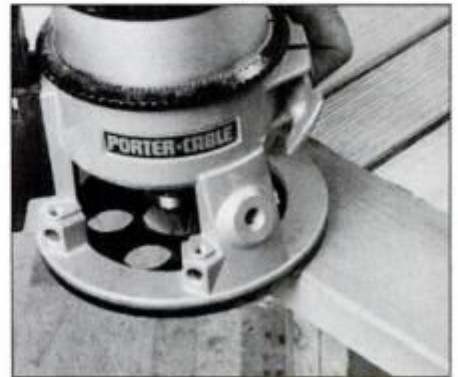
18 Use a rounding-over bit in the router to put a curved edge along the top and bottom edges of each top.
