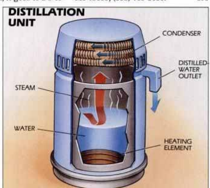
Distillation purifies water by first converting it to vapor, leaving impurities behind. Then, vapor is condensed for use. Countertop (above) and large-capacity units are available.
