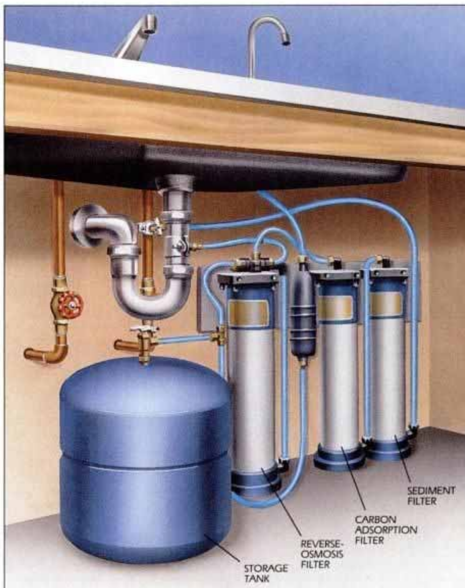
A complete point-of-use water treatment system may include several filters. This example shows an initial sediment filter to screen large particles. The water then passes through a carbon filter followed by reverse osmosis. Clean water is held in the storage tank.
