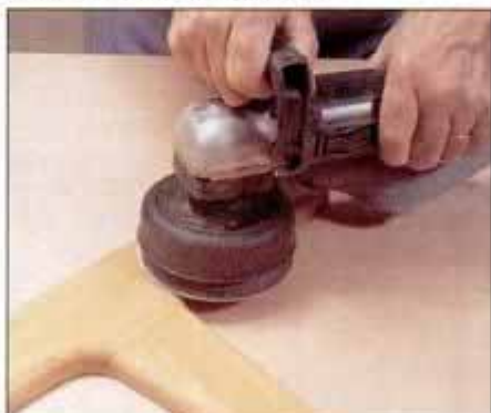
Skil sander produces swirl-free surfaces and is especially useful when sanding work that has different grain directions.
