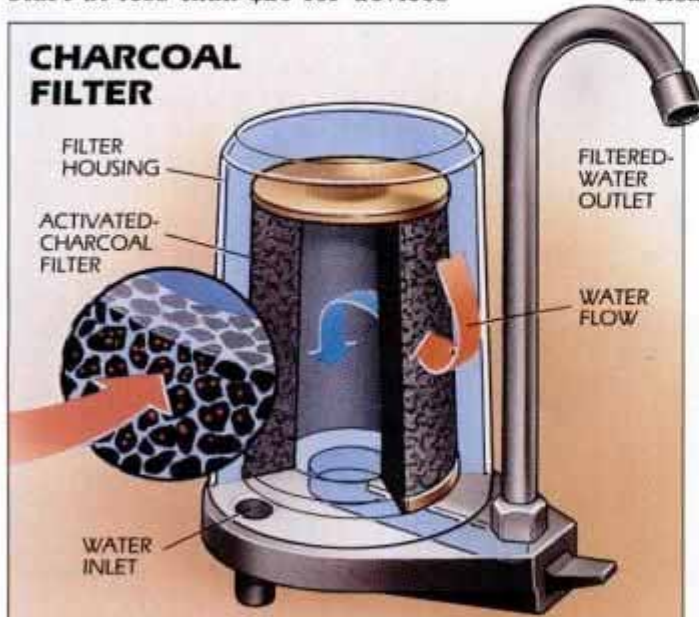
Carbon filters collect impurities through adsorption. They're used both in conjunction with other systems and alone on the countertop or mounted directly on the faucet.
