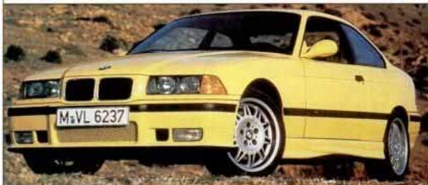
Limited to European markets so far, the new BMW M3 coupe offers supportive multi-adjustable bucket seats. M3's 3.0-liter dohc 16-valve Six produces 286 horsepower, 0-to-60 in less than 5 seconds.
