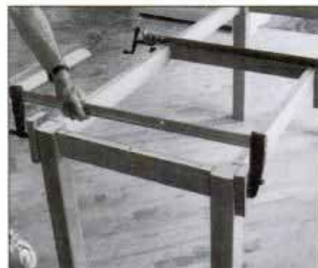
14 Glue and clamp together the leg-apron assemblies spanned by the short aprons and center support rails.
