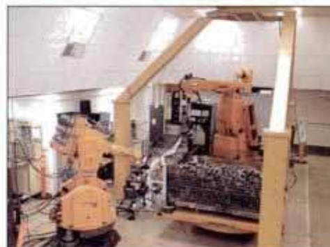
Laser camera illuminates jumble of exhaust manifolds, sending 3D image information to bin-picker robot.
