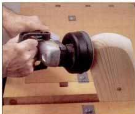
Coarse-grit disc makes fast work of heavy stock removal. The model No. 7484 is well balanced and easy to handle.
