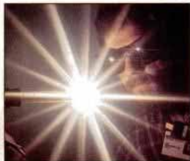
Tungsten-carbide filament heats methane and hydrogen in Oak Ridge diamond-making process.
