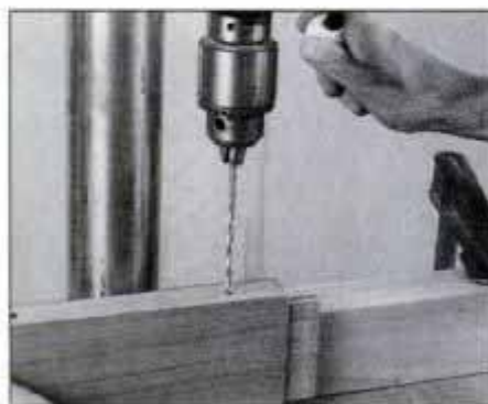
8 Bore the pilot holes through the width of the aprons using a long bit chucked into the drill press.
