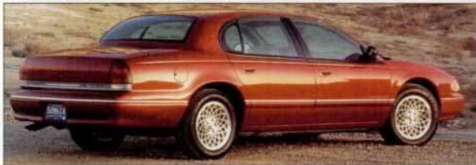
Chrysler's 214-hp dohc 24-valve 3.5-liter V6 and 4-speed automatic. Like the other LH sedans, dual airbags
