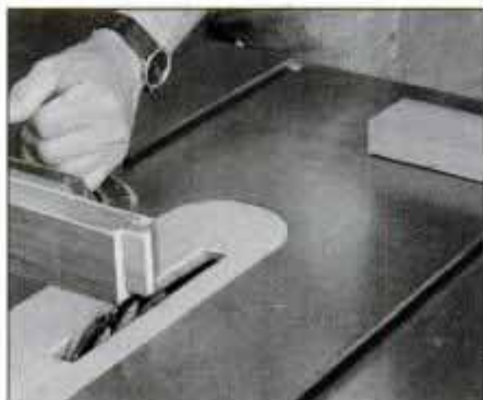
3 Tip the workpiece on edge, butt it to the stopblock and move the piece over the dado head to finish the tenon.
