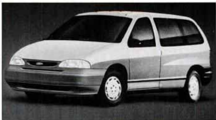
Front-drive Aerostar replacement is based on Taurus components.
