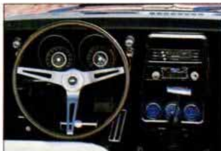
Optional wood-grain wheel and gauges make our Camaro top of the line. Modern B&M shifter hints at non-stock drivetrain.
