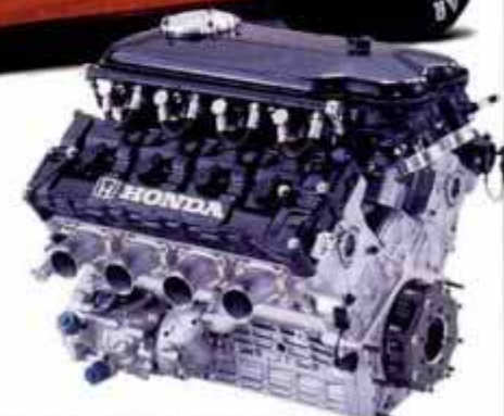
Honda's 1994 IndyCar campaign will be built around a new 2.65-liter dohc 32-valve turbocharged V8.
