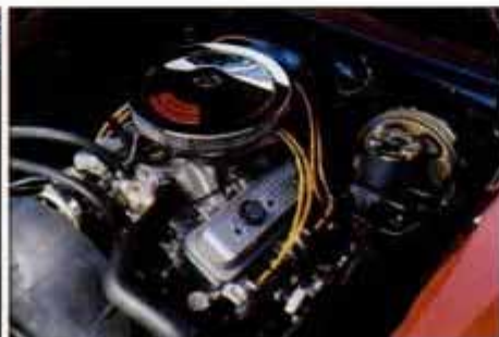
Surprise! Engine compartment is totally 1967, except for the '93 HO 350 V8 and TH700 4-speed overdrive transmission.
