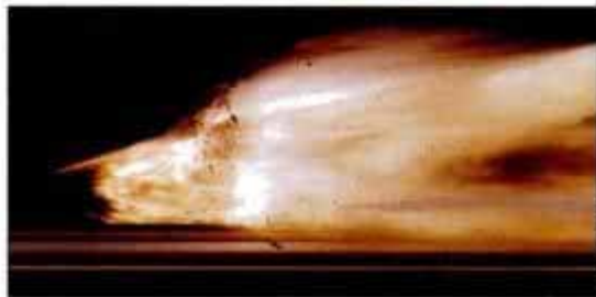
A kinetic-energy warhead explodes into a cloud of tungsten pellets traveling at a speed of Mach 4.25.
