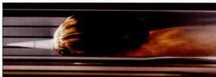
A kinetic-energy warhead explodes into a cloud of tungsten pellets traveling at a speed of Mach 4.25.
