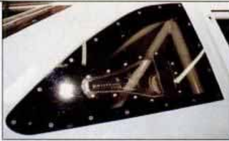
Outer body skin is sheetmetal. Front and rear sections are Kevlar and cover front- and rear-suspension components designed to deform in specific patterns on impact. Power comes from pushrod V8.
