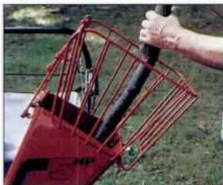
Large-capacity chipper has protective gate to keep hands clear of chute. When not in use, gate folds down over chute.
