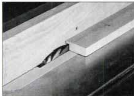
18 Use dado blades in the table saw to cut the rabbet on the inner edges of the upper door stiles and rails.
