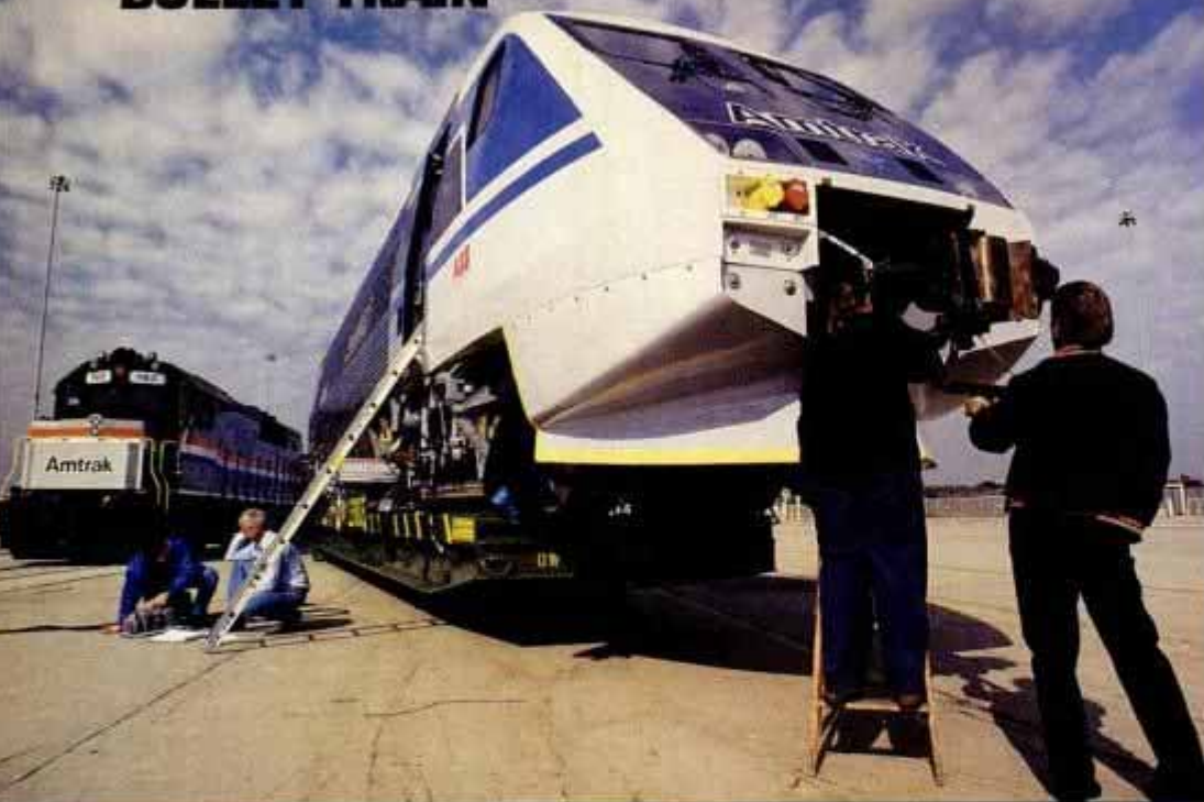
At Baltimore Harbor, diesel locomotive waits as Amtrak and ABB Traction personnel charge X2000's batteries and prep train for short haul to Northeast Corridor track.
