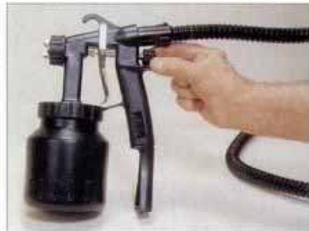
Finish flow rate is adjusted by turning a knob behind the handle. Spray pattern is adjusted by turning the air cap at front.
