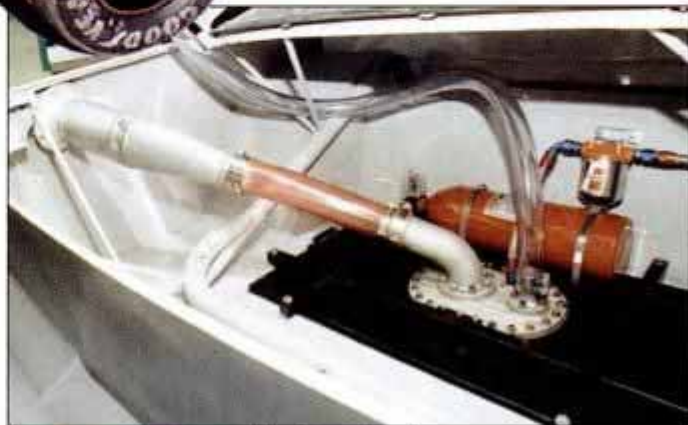
Nearly identical beneath the skin, all the cars have 3 x 4-in. frame rails and a safety cage of 1 1/4-in. tubing. Note fire extinguisher next to fuel tank.
