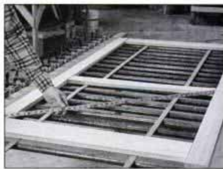
6 Clamp the face frame parts on a flat surface. Check diagonal measurements to be sure the face frame is square.
