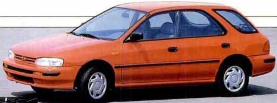
New Subaru Impreza uses 16-valve dohc version of 1.8-liter opposed Four.
