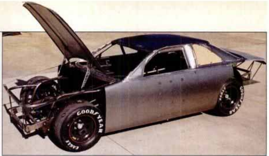
Outer body skin is sheetmetal. Front and rear sections are Kevlar and cover front- and rear-suspension components designed to deform in specific patterns on impact. Power comes from pushrod V8.
