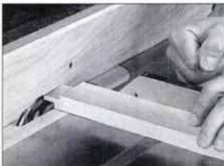
19 Use the miter gauge and the rip fence to cut tenons on the upper door rails. Make the cheek cuts first.
