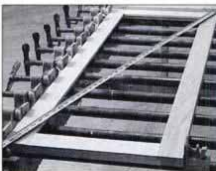
21 Glue and clamp the upper doors. Check the assembly for square by comparing diagonal measurements.
