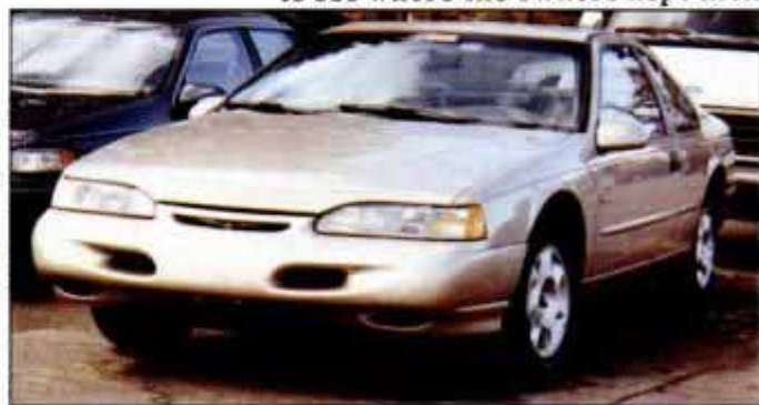
'94 T-Bird gets new grille, hood to fit 4.6-liter modular V8.
