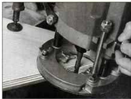
3 Clamp the shelf-blank template to the workbench. Use a flush trimming bit in the router to cut the blank to size.
