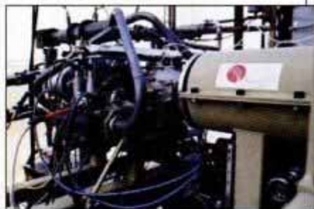
Extensively modified Rotax is the core of Perseus's Arion 1 powerplant.
