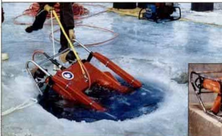
Super Phantom 2 robo-sub enters freezing lake during Antarctic field test of telepresence hardware.
