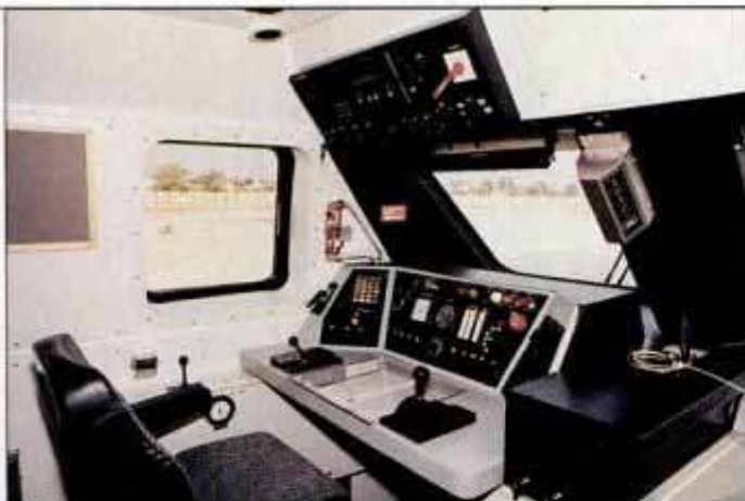
Although brake and throttle lie in reverse of American layout, X2000's cab puts controls within easy reach of the engineer.
