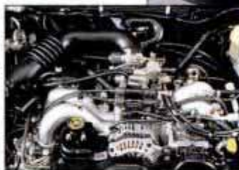
New Subaru Impreza uses 16-valve dohc version of 1.8-liter opposed Four.
