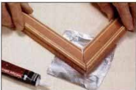
Super Strength Adhesive is clamp free. This miter joint needs only a few minutes of hand pressure for a good bond.
