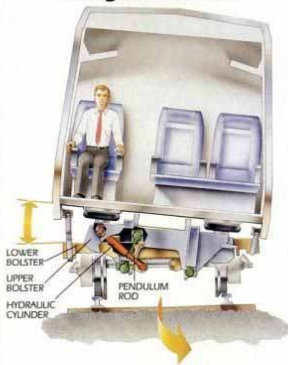
A hydraulic cylinder separates two structural bolsters, opening an angle between cabin and undercarriage.
