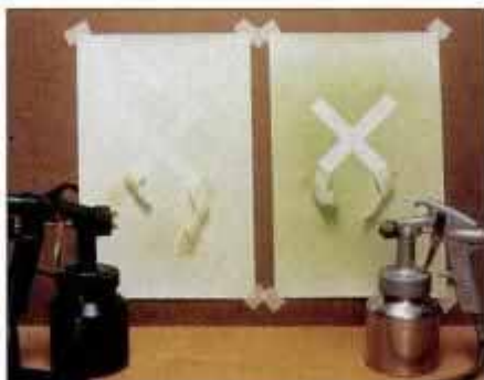
Backdrops behind test pieces show comparative overspray of HVLV system (left) and standard spray gun (right).
