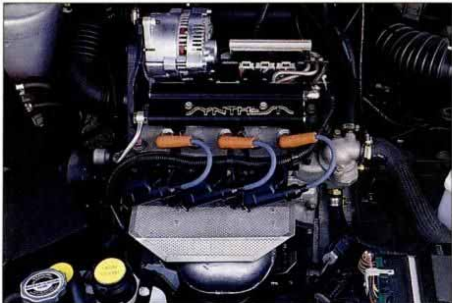
Orbital 1.2-liter 3-cylinder 80-hp 2-stroke engine sends power to the front wheels.
