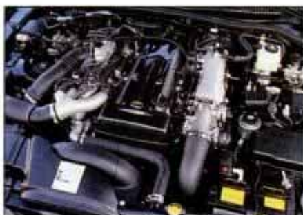
Sequential twin turbochargers boost 3.0-liter dohc 24-valve V6 output to heady 320 hp.
