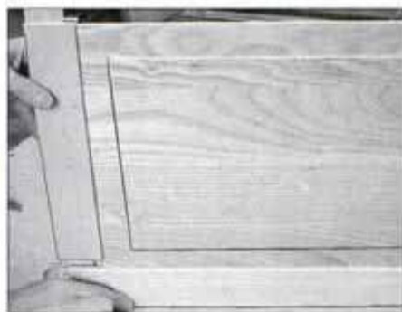
22 Slide the panel into the stile-rail assembly on a lower door. Then clamp the assembly with the remaining stile.
