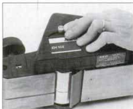
Retractable cutterhead guard on the AEG works like a circular-saw blade guard. Lever on the side retracts guard manually.
