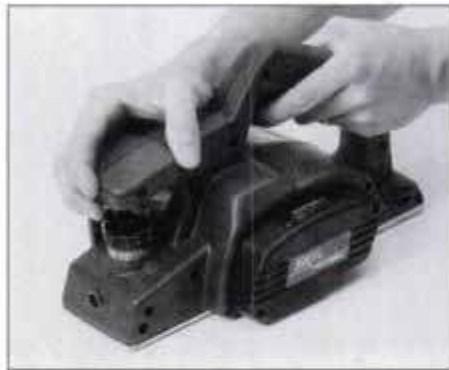
Skil and Sears tools have dedicated front handles. Depth knob on other models doubles as a front handle.
