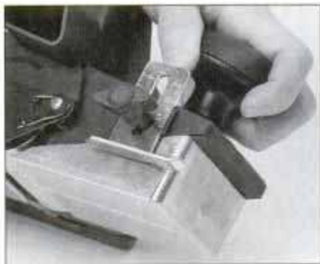
The depth stop controls rabbeting depth. Stop on Bosch power plane has scale in inches and millimeters.
