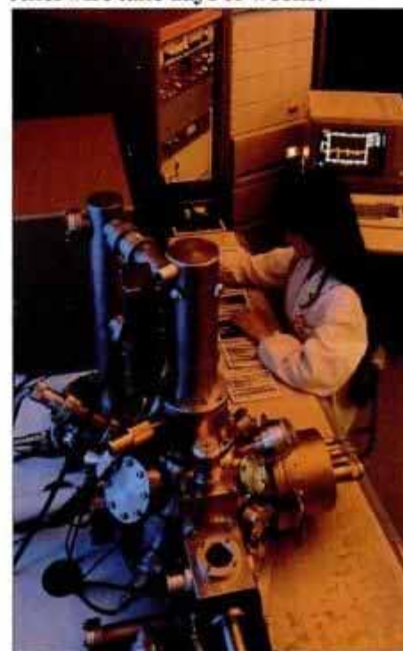
High-tech extends to electron microscope testing of tire-manufacturing materials.
