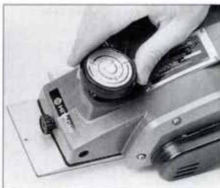
Hitachi, Makita and Ryobi depth knobs require several rotations for complete range. Spiral scale is difficult to read.
