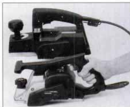
Extremes in handle angle are illustrated by Porter-Cable (top) and Sears. Hitachi and Makita handles are similar to Sears.
