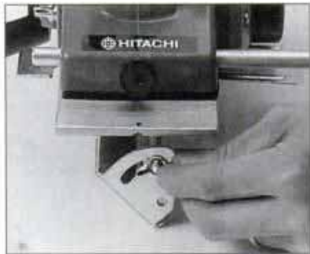
Hitachi fence is adjustable for planing bevels. Other tools have fixed 90° fences with optional beveling fences.
