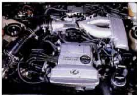
220-hp 3.0-liter dohc 24-valve inline Six drives rear wheels via 4-speed automatic.
