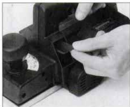
Chip ejection on the Porter-Cable 9367 can be switched from one side to the other by pivoting the chip gate.
