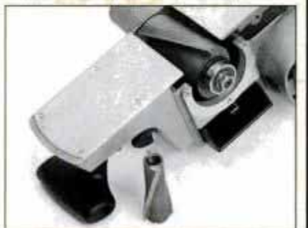
Helical power plane cutters create a smoother slicing action. Porter-Cable offers both carbide or high-speed steel.
