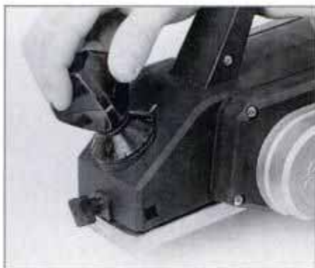
Cut depth is set with a knob that adjusts the height of the front shoe. Elu (shown) adjusts through its range in one rotation.
