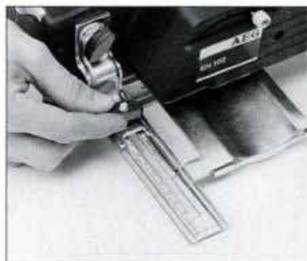
Fence on AEG, Bosch and P-C attaches to L bracket. Scale on AEG shows rabbet width in inches and millimeters.
