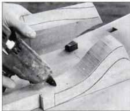
11 Tack the cutoff piece back on the leg blank with hot glue to provide a guide for cutting the side profile.
