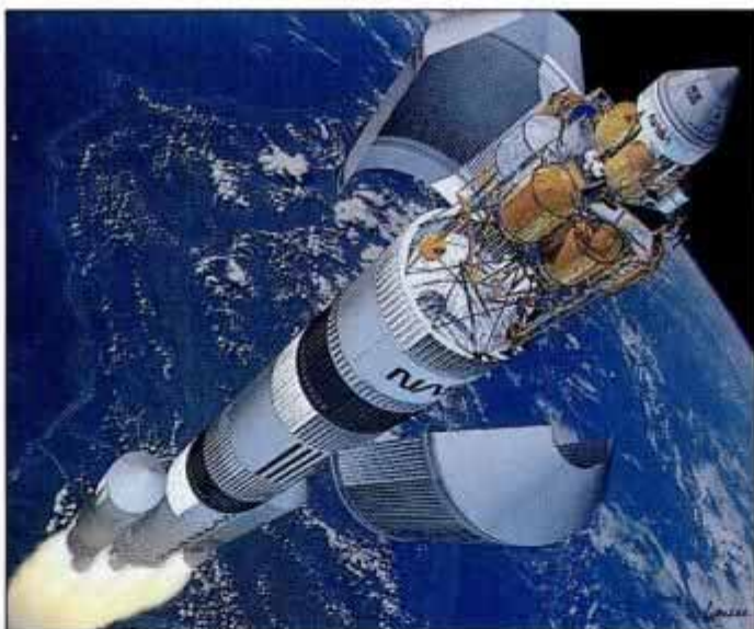
First Lunar Outpost would rely on monster booster, featuring Saturn V -derived engines, to fly nonstop from Earth to Moon.
