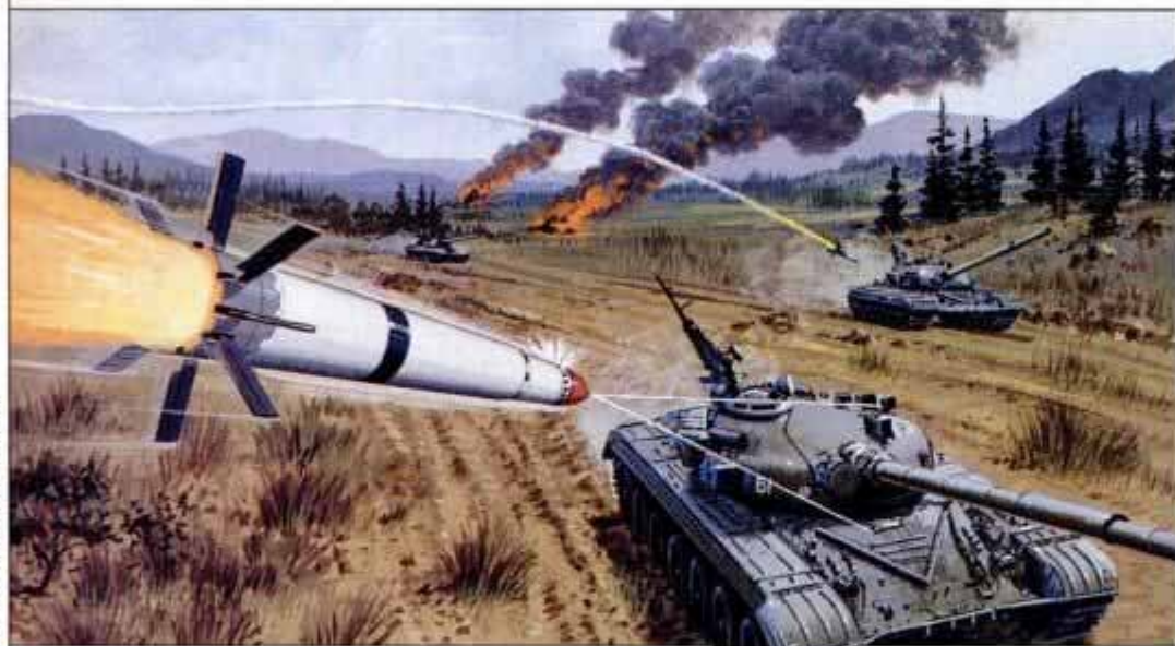
Rocket-powered X-Rod homes in on enemy armor with the aid of millimeter-wave radar.
