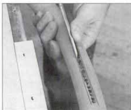
22 Pare the sides of the splat mortise flat and its ends square using a chisel. Work down to the knife line.
