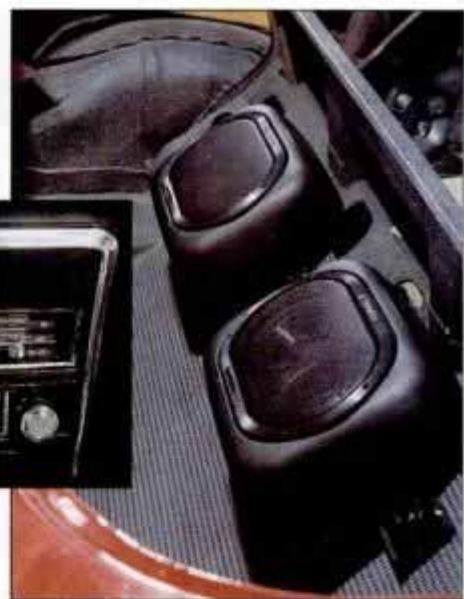
USA-04 '60s-style radio and Pioneer TS/TRX40 speaker systems came from Custom Autosound. The radio perfectly matches the dash. Trunk-mounted speakers are hidden by top well boot.
