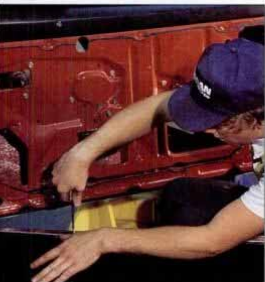
PM Contributing Editor Rich Taylor and buddy Ken Barnes tag-team staple the rear window to the top bow (above left). Ken installs new door weatherproofing panels and doorsills (above).
