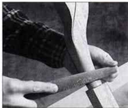
12 Clamp the front leg in a vise and shape the round section of the front legs using chisels and rasps.
