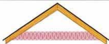
INSULATION BELOW VENTILATED ATTICS
