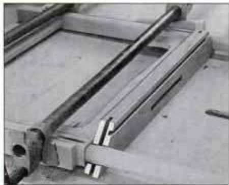
23 Glue and clamp the rear legs, seat frame, apron and stretcher. Follow the same procedure for the front legs.
