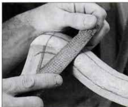
26 With the chair well supported on a padded surface, use gouges, chisels and rasps to shape the bow-leg joint.
