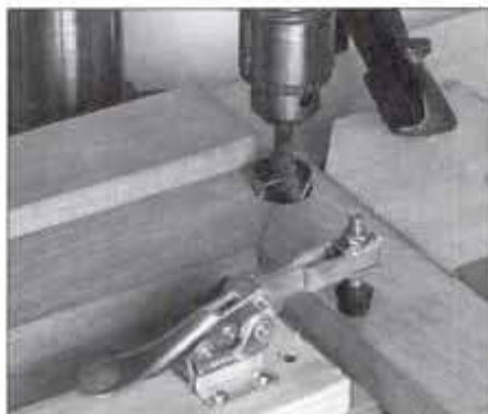
17 Clamp the seat frame pieces to the drill-press table, then bore 1\frac{1}{4} -in.-dia. holes through the miter.
