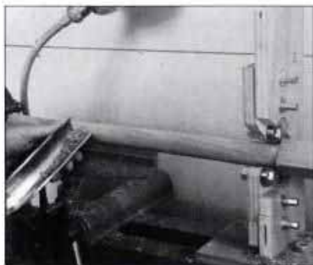
14 Turn the round section of the rear legs by first using a gouge. The legs can also be shaped with a spokeshave.
