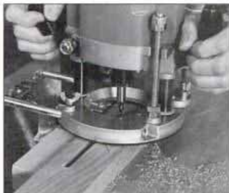
18 Hold a seat frame to the workbench and use the plunge router and a straight bit to cut the splat mortise.
