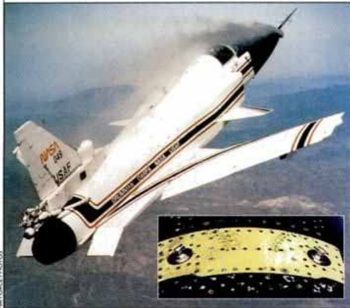
Smoke streams over forward fuselage of X-29 No. 2 to visualize vortex flow disrupted by gas nozzles (inset).
