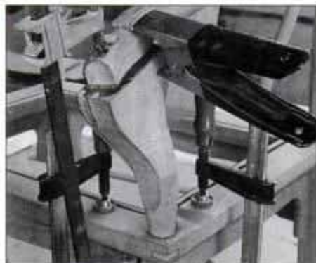
25 Apply epoxy where the bow front and legs meet and on the dowel. Clamp until the epoxy has cured.
