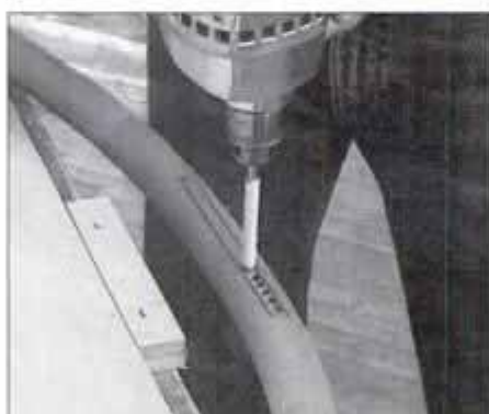
21 While the bow is still on the jig, bore a series of \frac{3}{8} -in.-dia. holes to remove the bulk of the splat mortise.
