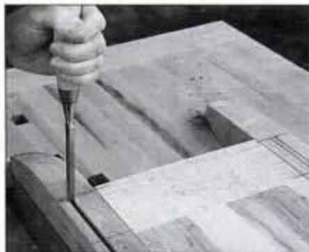
10 Use a sharp chisel to square the ends of the mortises. Butt the chisel to the pencil line and chop down.
