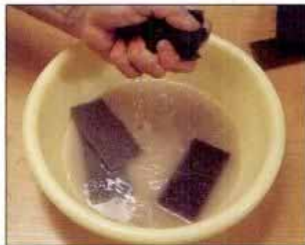
After use, the pads can be rinsed to a like-new condition. They're compatible with water- and solvent-based finishes.
