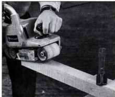
7 Clamp each leg to the workbench and use a belt sander or hand plane to remove saw marks and refine the curve.
