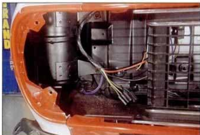
Ready for the headlight assembly, the grille and wiring harness are in place and underhood panels are painted correct semigloss black.
