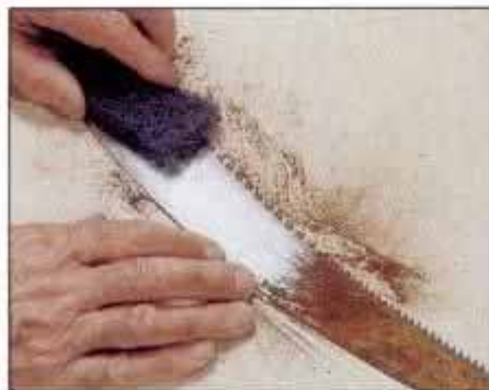
The coarse pad is best for removing heavy rust from metal. 3M claims that the synthetic pads last longer than steel wool.
