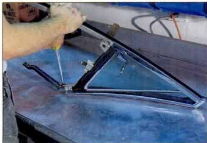
Tired vent window frames were stripped, straightened, filled and rechromed before reassembly with new glass and weatherstripping.
