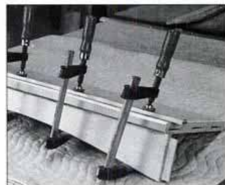
17 Assemble the bookshelf in stages. First, glue and clamp together the bottom shelf and the front rail.
