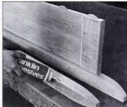
8 Cut matching joining plate slots in the legs and case sides. Apply glue as before then clamp the assembly together.
