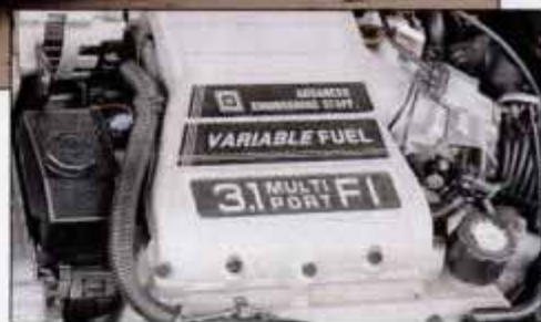
3.1-liter V6 has been graced with virtually no internal changes to support dual fuel usage.
