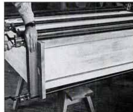
19 When base assembly is complete, glue and clamp the top to the assembly. Cauls spread the clamping pressure.
