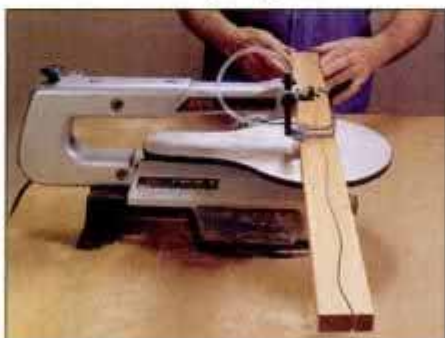
With the blade installed in side position, you can handle stock of unlimited length. The table measures 10 × 15 in.
