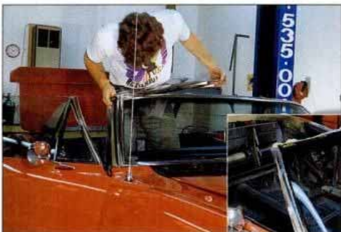
Ken Barnes (top) fits a new taillight assembly. Above, he's installing our rechromed windshield header.
