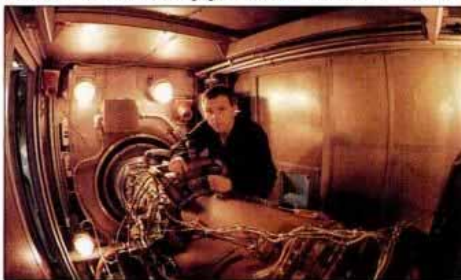
Gas-turbine powerplants are derived from DC-10 airliner engines.
