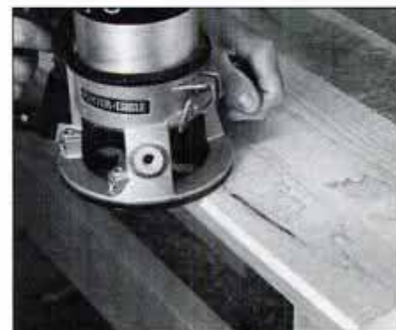
21 Hold each shelf to the workbench then cut a chamfer on the top and bottom edge on the front of each shelf.
