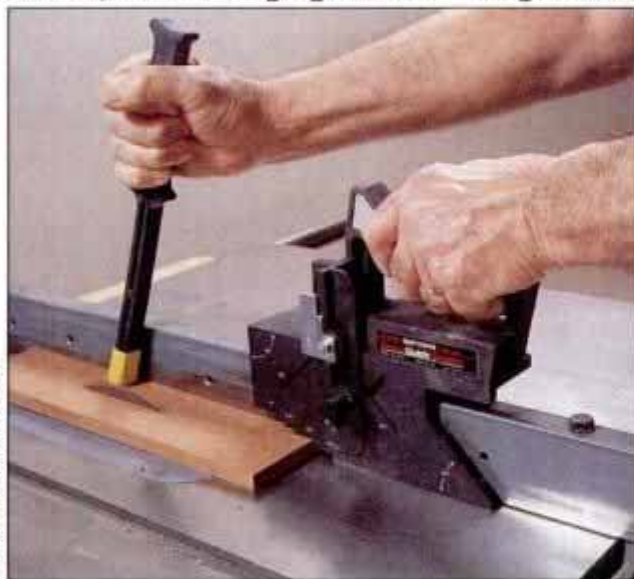
The Sears Fence Guide System slides along the table saw fence as it guides and holds stock. Holddown stick (included) keeps your hands away from blade. Jig also has provisions for setting blade height in 1/8-in. increments, and 45° and 90° blade angles.
