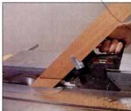
For tenons, open mortises and lap joints, stock is clamped to jig side. Mitered or 90° work can be handled.
