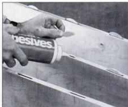
2 Apply glue to the slots and edges of the strips. Install the joining plates and clamp the pieces together.
