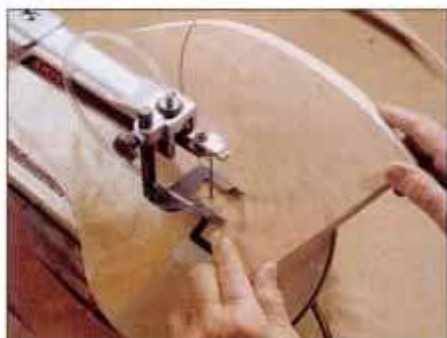
The table tilts to 45° for making bevel cuts. The holddown foot tilts to match the table and hold the work securely.
