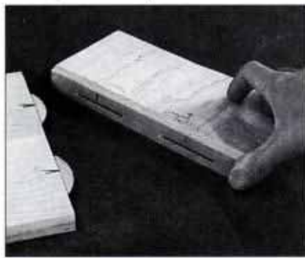
5 Cut joining plate slots in the side panel and false rail. Insert the plates then glue and clamp the two together.
