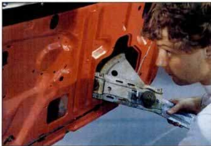
Pesky window winders must be inserted and adjusted through small holes in the door. Sore forearms are an occupational hazard.
