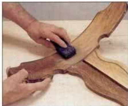
Working from coarse through fine grades, the synthetic pads completely stripped old, flaky varnish without chemicals.
