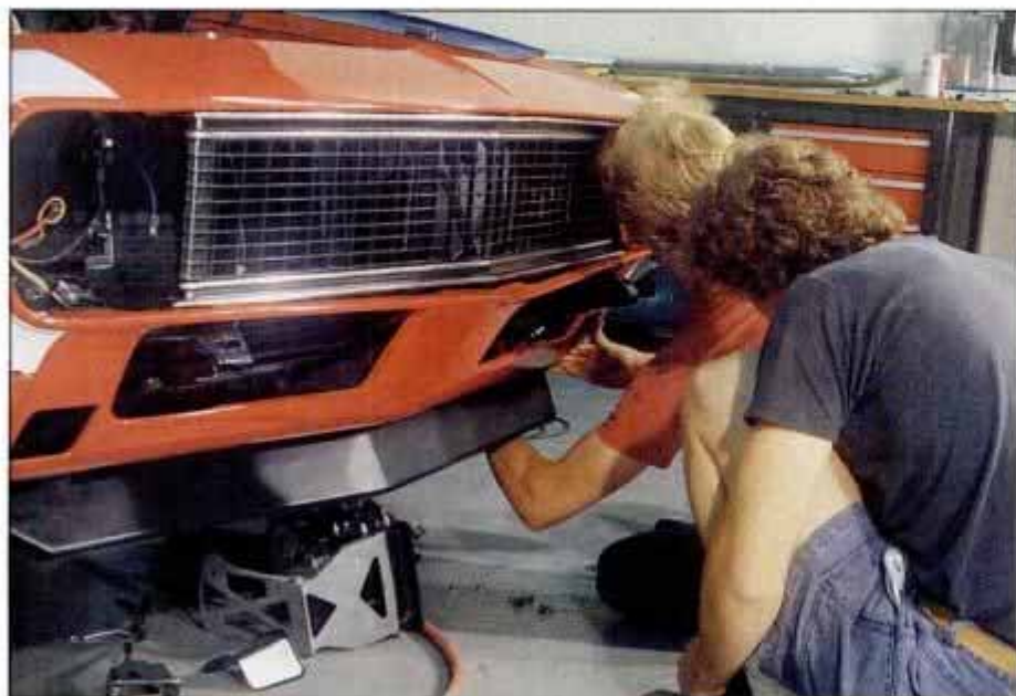
Grille, lower valence panel and spoiler took a lot of time and patience to align properly.
