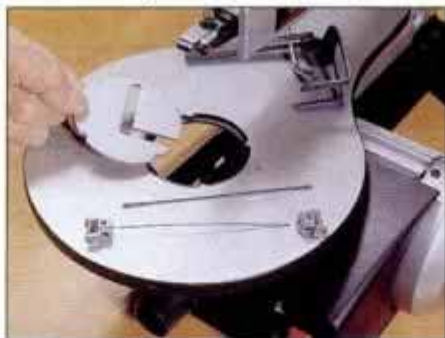
The Skil saw has a 2-position insert to handle both pin and plain-end blades. Narrow pin-less blades are held by adapters.
