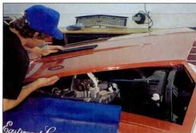
Ken carefully fits the SS vents to the newly painted hood. The finish is still quite soft at this point.
