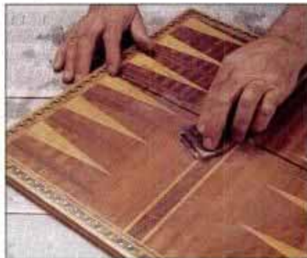
The extra-fine pad is ideal for obtaining a hand-rubbed, satin finish. Here the pad is used with oil and rubbing compound.
