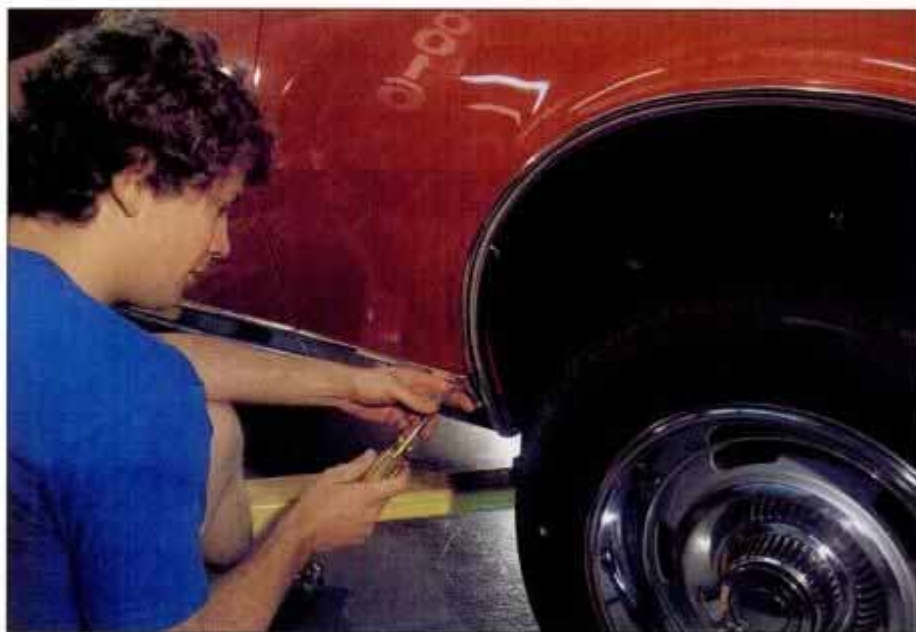
The trick here is getting the two pieces on the fenders to line up with the piece on the door.
