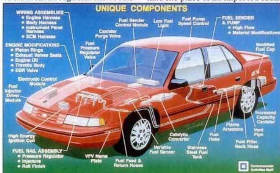
Fuel sender senses proportion of ethanol, high-capacity injectors, alcohol-tolerant plastic and metal parts.
