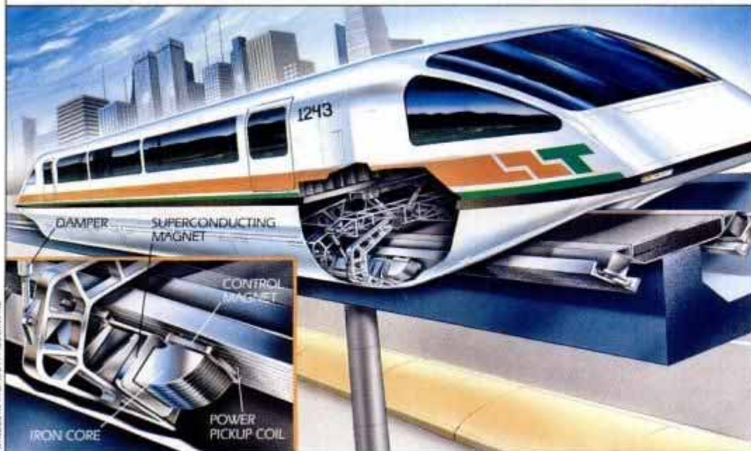
Grumman's maglev features hybrid magnet in attractive-levitation arrangement.
