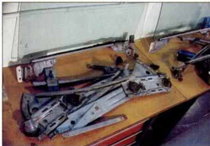
Completed subassemblies of window mechanisms and glass are ready to be installed.
