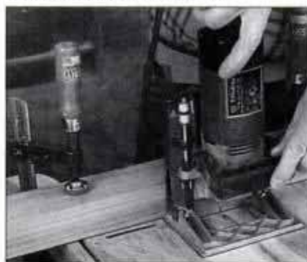
14 Clamp a straight piece of scrap across the case side. Butt the plate joiner to it and cut the plate slots.
