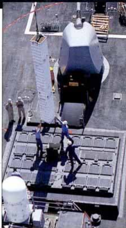
Missiles are lowered into VLS in canisters (above) and stay sealed until launch (top).
