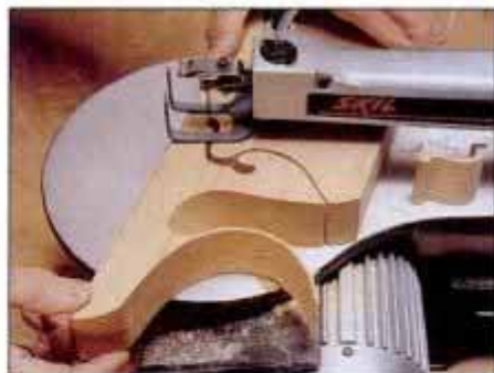
With a maximum capacity of 2 in. at 90°, this saw easily handles intricate cuts in thick hardwoods and softwoods.
