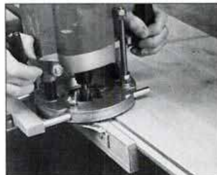
16 Cut the rabbets in the back panels using a router, straight bit and edge guide. Move the router slowly.
