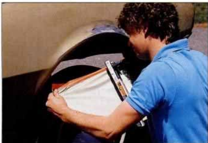
Ken masks wheel wells and chassis before putting on a protective coat of Dupont 1615 self-etching primer.
