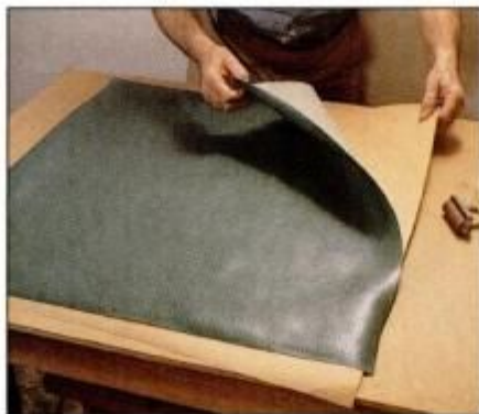
14 Carefully align the vinyl over the kraft paper, then lower it into place. Slip out the paper sheets one at a time.
