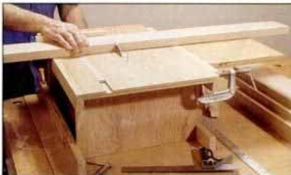
2 This shop-built table works well for crosscuts using a fixed-angle miter gauge and an extension table.
