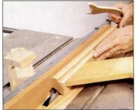
18 Cut crown with molding head in table saw. Use featherboard and pushstick to keep stock firmly against fence.
