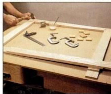
5 Assemble frame parts facedown. Apply glue, then drive two alignment brads through both pieces and clamp.
