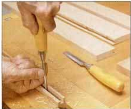
3 Clean out all mortises with sharp chisels. Make sure that mortise walls are pared smooth and square to edge.
