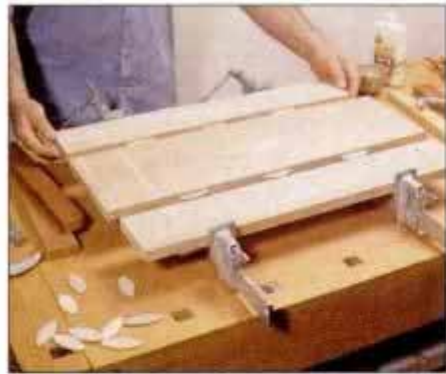
11 Use plates or dowels to join stock for door panels. Locate plates or dowels clear of area that will be beveled.
