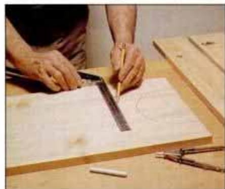
1 Align the stock for the sides, and lay out the circular cutout for the feet and the location of the joining plates.
