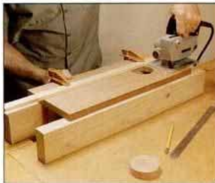
4 Cut the stock to width using a wood straightedge to guide the saw.
