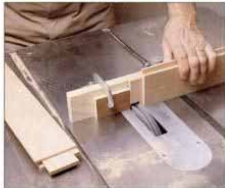
4 Cut rail tenons using dado blade on table saw. Wood fence and stopblock on miter gauge ensure identical repeat cuts.
