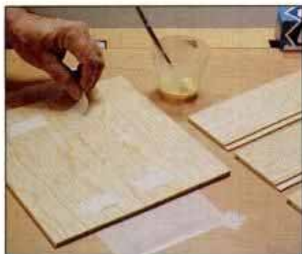
12 Join panels with glue and tape. Wax paper keeps assembly from sticking.
