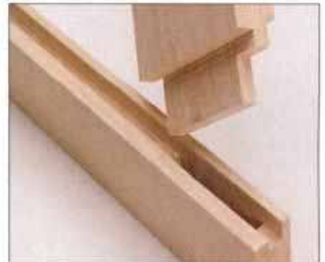
5 Closeup shows configuration of joint. Haunch on tenon is required to fill gap in groove above mortise.
