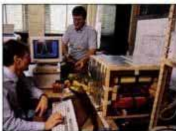
Ripeness sensor uses magnetic resonance to measure amount of sugar in produce.
