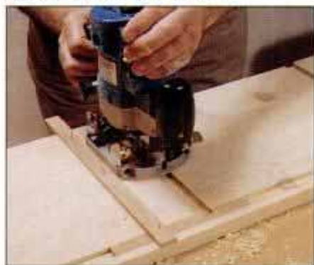
8 Cut shelf dados using an L-shaped guide. Place the short leg into the long dado and tack the other leg to the side.
