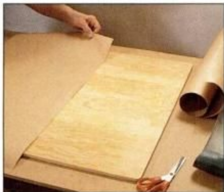
13 Cut the top plywood panel to size and shape. Then sand it smooth and cover it with two pieces of kraft paper.
