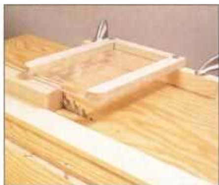
9 If you use our table to rip the legs, its shallow blade projection requires cutting in two passes, one on each side.
