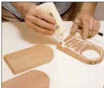
6 Apply glue evenly to mating surfaces, then install clamps until glue is dry.
