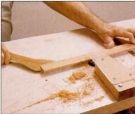
13 Use a router table, or a table saw with a molding cutter head, to cut the base and top moldings for the case.
