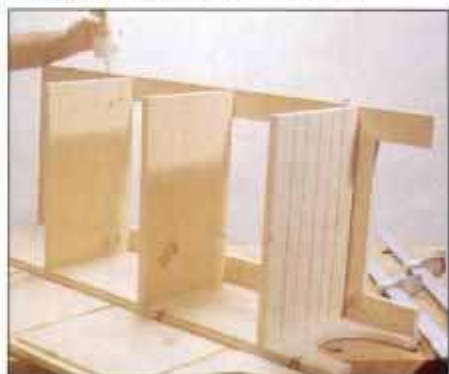
9 Assemble piece on its side. First glue the face frame and shelves to one side, then add second side and clamp.
