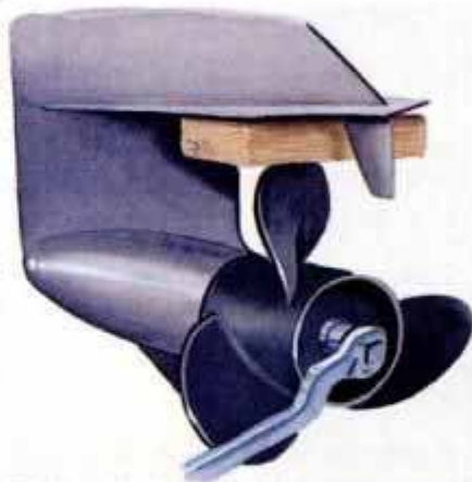
Wedge a block of wood between prop and anti-ventilation plate before loosening prop nut and inspecting hub and splines.
