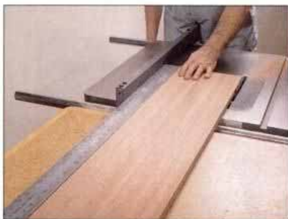
1 To straighten stock on table saw, tack-nail metal rule to one edge, then rip. Remove rule and rip other edge.
