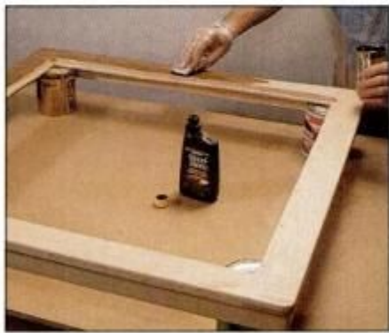
16 Check the top panel for fit. Then remove, finish sand the frame and apply the finish before installing the top.
