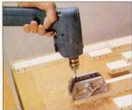
9 Lay out dowel locations in support frame members, then bore dowel holes using portable drill and doweling jig.
