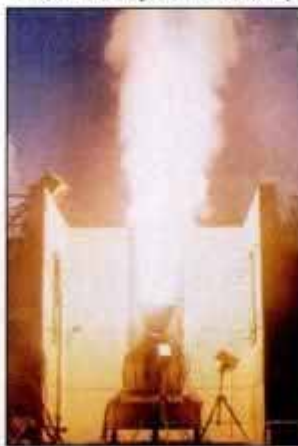
Star 48V upper stage, test-fired in June, will boost COMET and Westar payloads.
