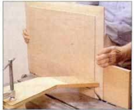
13 Cut panel bevels on table saw using high auxiliary fence and elevated featherboard as safety precautions.
