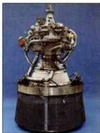
New Centaur rocket engine has extending nozzle cone coated with heat-resistant niobium. The cone is controlled by a system of three actuators.
