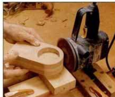
7 Use a bench-mounted sander to shape the top curve of the workpiece.
