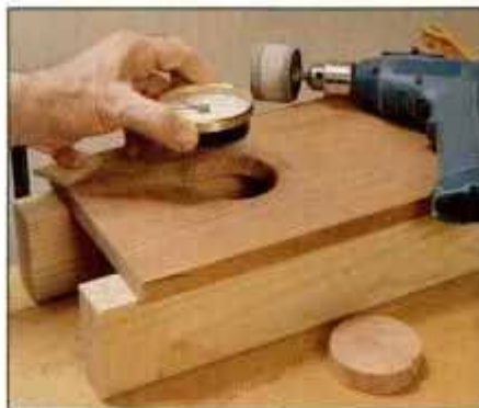
3 Use a sanding drum to smooth the wall of the cutout. Test fit the movement.
