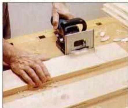
2 Using a plate joiner, cut the plate slots in the board edges. Work on a flat surface or the slots will not align.
