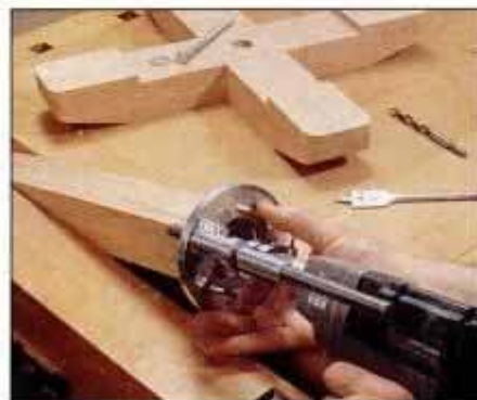
12 Bore a lag screw clearance hole in the base assembly. Then bore a pilot hole in the post using a drill guide.
