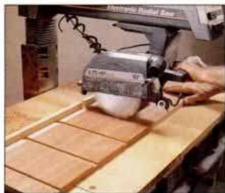
3 Adjust radial-arm saw for proper dado depth then test cut a scrap block. When satisfied, cut dados in both case sides.
