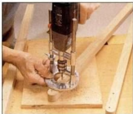
10 Lay out brace rivet holes in the legs. Then bore them using a drill with a guide to keep holes perpendicular.
