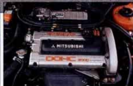
In awd tune, the Mitsubishi 2.0-liter dohc 16-valve turbo Four generates 195 hp.
