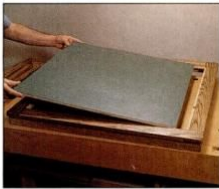
17 Attach the legs to the frame assembly and slide the top panel into place. Attach the panel with screws from below.
