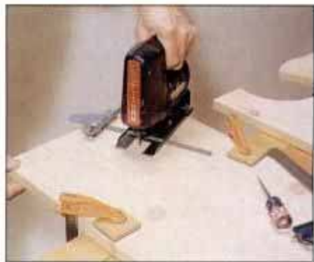
6 Use a sabre saw with a pivot guide, or work freehand, to cut the legs to shape. Cut from the back side of the panel.
