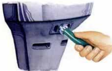
Flushing out raw water is easy using a built-in garden hose port. Special attachments are needed for older engines.
