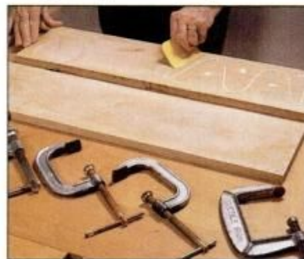
8 Obtain the stock for the legs by gluing up two ¾ boards. Spread the glue evenly and clamp boards securely.
