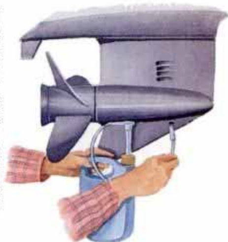
After draining the old gear-case lube and examining it for signs of wear, slowly refill until lube appears at the upper port.
