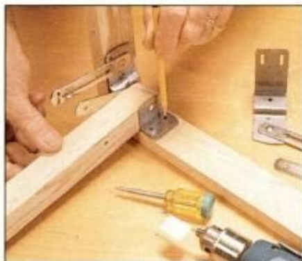
11 Temporarily place all the folding hardware on the legs and aprons. Then mark all the bracket screwholes.
