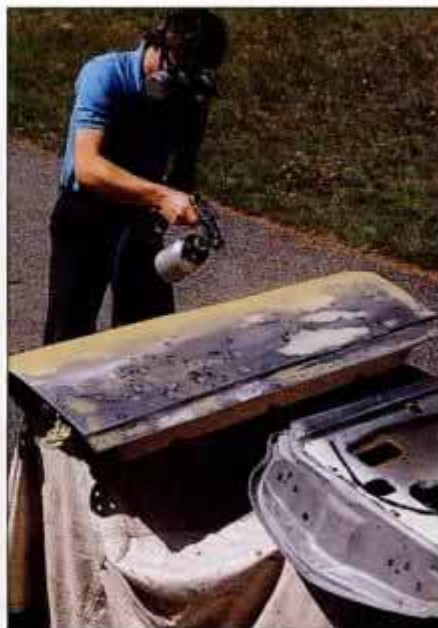
Wearing a respirator, Ken sprays "yellow death" onto finished doors using our TP-77.
