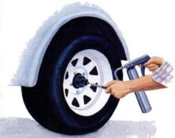
A squeeze from the lube gun does the trick on the bearings.
