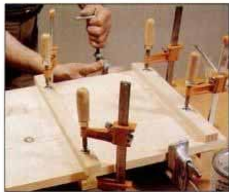
4 Join the boards with bar or pipe clamps first. Then clamp wood cauls across the surface to keep the panel flat.
