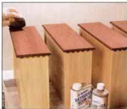
19 Apply stain to drawer fronts with clean, soft cloth. Retarder is added to stain to keep lap marks from showing.
