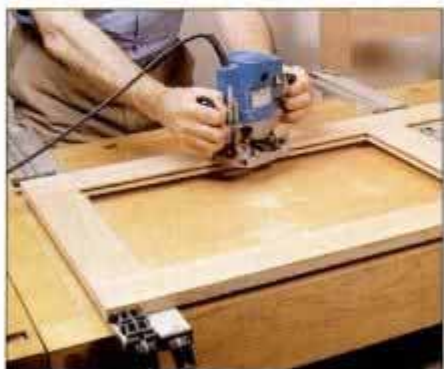
6 Temporarily dry assemble side frame, making sure parts are square. Then round over inside edges with router and bit.
