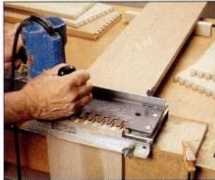
17 Cut drawer stock to size then lay out and cut dovetails using router and jig. Code mating pieces to avoid mismatches.
