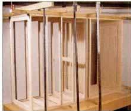
10 Glue and clamp case together. Clamps can bear directly on case, or be attached to cauls and workbench as shown.
