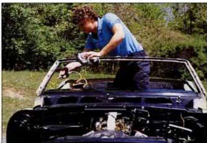
It's not enough to clean areas to be painted, you must also clean areas where dust can blow onto fresh paint.
