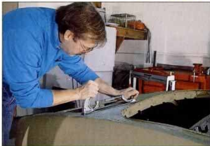
Rich uses an English file to shape body filler on the rear deck. This is a tricky area where many different body surfaces meet.
