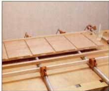
5 Apply glue to frame mortises and tenons, then clamp securely. Check for square and readjust clamps if necessary.
