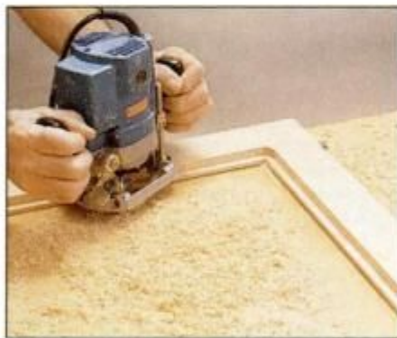
6 Use a router and a rabbet bit to make the recess cut in the top frame for the top panel. Make cut in several passes.
