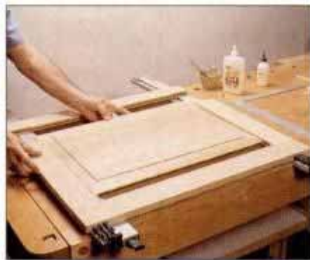
15 Attach bead to frame members, then glue and clamp frame together. Do not glue panel into groove—it should float.
