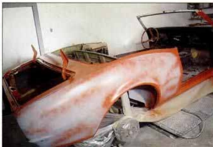
Edges painted! Matador Red overspray on primer helps locate imperfections and will be sanded off before finish coat is applied.
