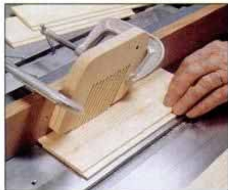
11 Cut lattice stock to size for door panels. Then cut rabbets on mating edges.
