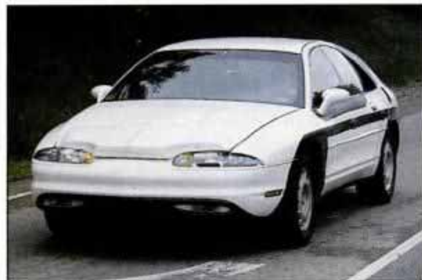
1994 Olds Toronado-replacement Troféo will receive 4.1-liter version of Cadillac Northstar V8 engine.
