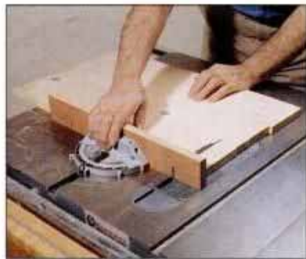
5 Glue and clamp together boards for the top panel. Once the glue has dried, cut the panel to size on the table saw.
