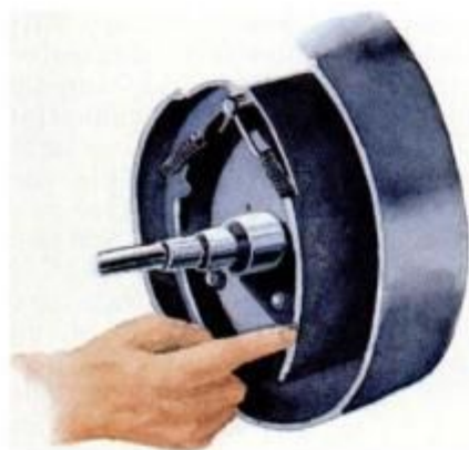
With the wheel and hub removed, clean and inspect the brake lining for wear.
