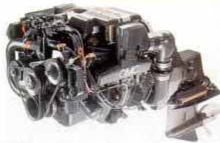
OMC's new EFI stern drives are based on 5.0-liter and 5.8-liter Ford engines.
