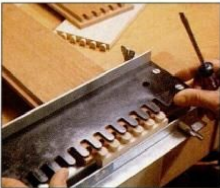
16 Cut dovetails by hand. Or use router template. Just align template, according to maker's directions, and rout.
