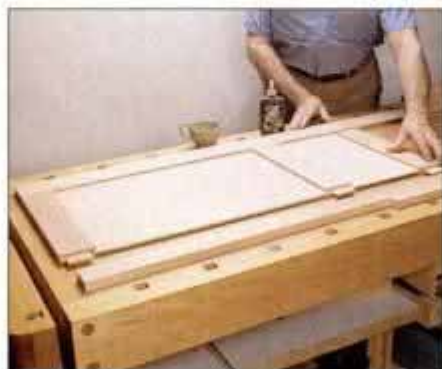
7 Assemble frame and panels using slow-setting hide glue. Add second stile only after all other parts are joined.
