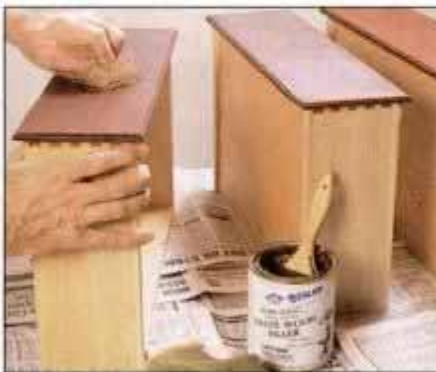
20 Apply filler to stained surfaces. When filler reflection begins to dull, wipe off across the grain with a coarse cloth.
