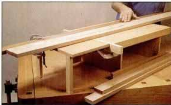
1 Rip post stock to width on a table saw or a table-mounted circular saw with extension table.
