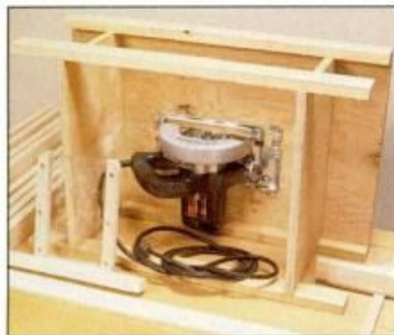
1 A shopmade table for your circular saw will yield easier, more accurate cuts. See drawing for building directions.
