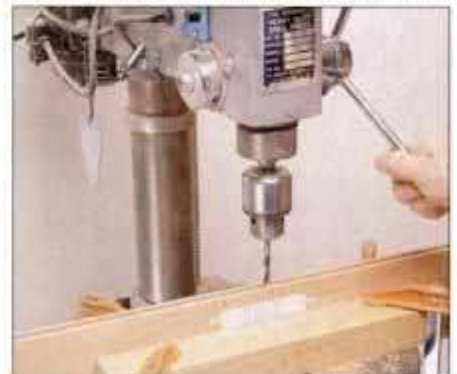
2 Cut joint mortises in stiles by boring overlapping holes on drill press. Marked tape on surface guides spacing.
