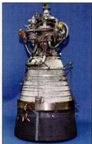
New Centaur rocket engine has extending nozzle cone coated with heat-resistant niobium. The cone is controlled by a system of three actuators.
