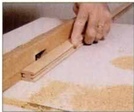
14 Cut bead molding on router table with two different bits: a bullnose bit first, followed by a slotting bit.
