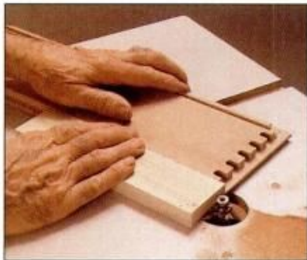
17 Cut outside bead on drawer front with router table. Hold backup board against workpiece to prevent tearout.
