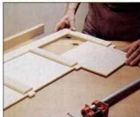
14 Join door parts by gluing rails to stiles. Do not glue door panels in place.
