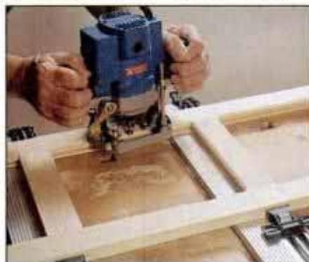
13 Dry assemble doorframe. Then make bead cuts on inside edges.
