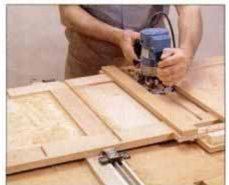
8 Cut shelf dados using a router and simple jig made of scrap lumber. Block at end of jig stops router travel.
