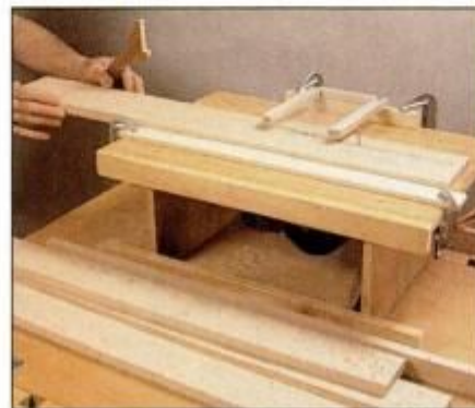
2 Using shop-built table, rip top frame members to width. Clamp blade guard in place and use pushstick for safety.
