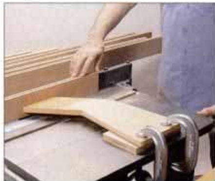
1 Cut stock to size. Then cut panel grooves in cabinet and door rails and stiles using dado blade in table saw.
