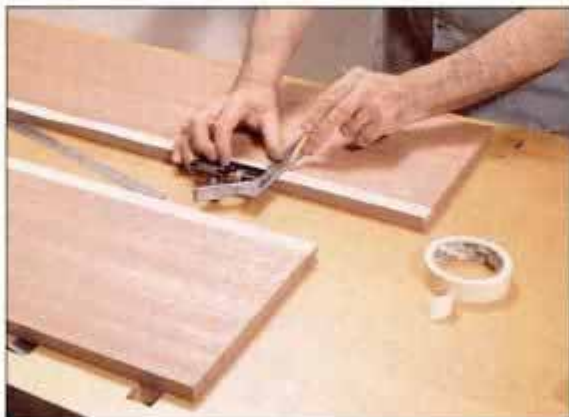
2 Because pencil marks are hard to see on darker woods, apply tape to edge then lay out frame dados.
