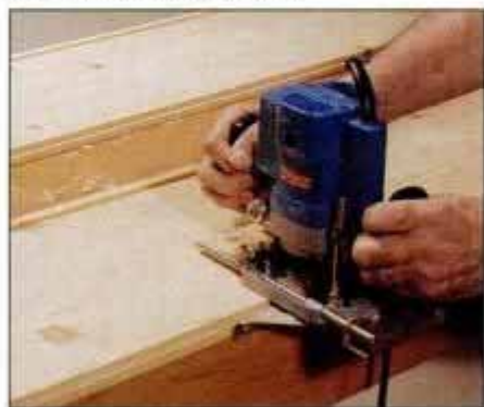
7 Cut a stopped rabbet for the back panel in the case sides, using a router with an edge guide and a straight cutting bit.
