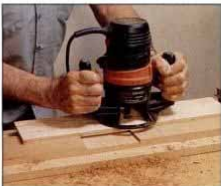
5 Attach an oversize base to a router and rout the middle board to thickness.
