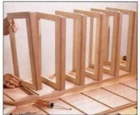
12 Join frames to sides with hide glue. Apply glue to front third of joint. Back is held with screws in slotted holes.
