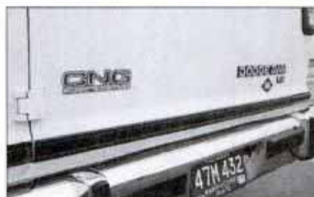
The badge on the tailgate and lack of exhaust odor identify this as one of 900 Dodge CNG-powered full-size vans. Gaseous-fuel engine uses 3000-psi tanks and lines—so refueling must be done at specialized facilities.
