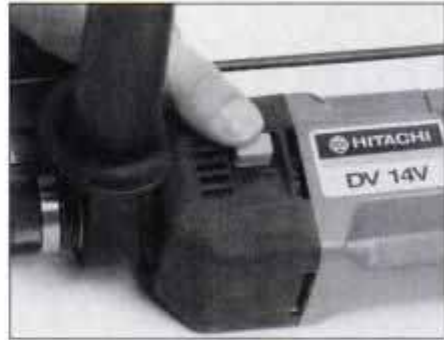
Hitachi hammer drill has convenient button to switch drilling modes. Most other drills of this type have a top-mounted dial.
