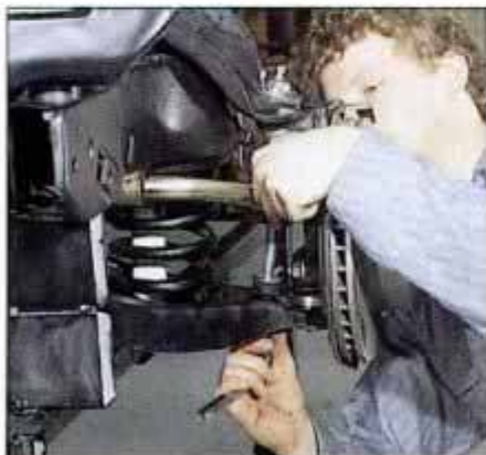
Ken tightens the antiroll bar mounting. This PST bar is considerably heftier than stock.
