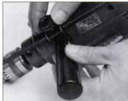
Round depth-stop rod on Makita HP 1030W is held with locking screw. This tends to loosen when hammer drilling.
