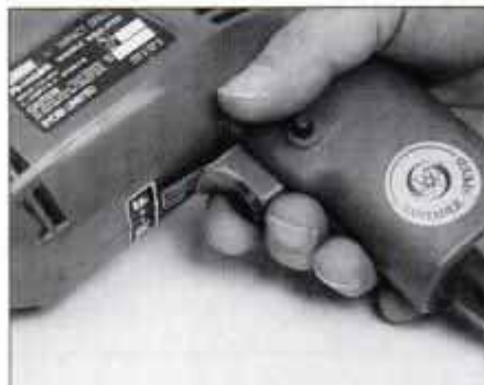
On Ryobi, Makita, Skil, Sears and Hitachi, dial on trigger controls lock-on speed. Other drills lock on at maximum speed.
