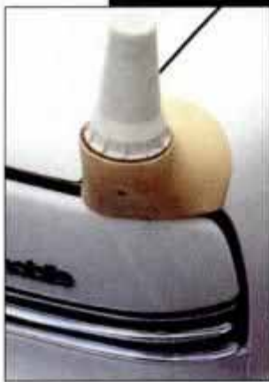
TravTek uses wheel sensors tied to a computer. A backup satellite link uses a special antenna (left).
