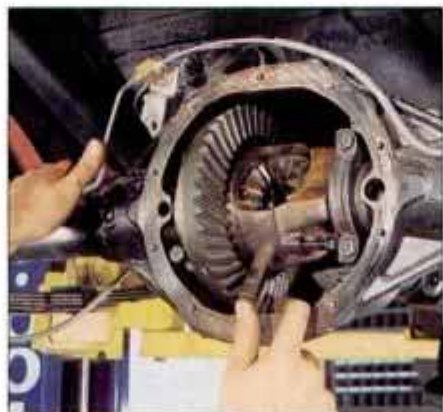
The new 3.70 ring and pinion should give our Camaro good snap off the line.
