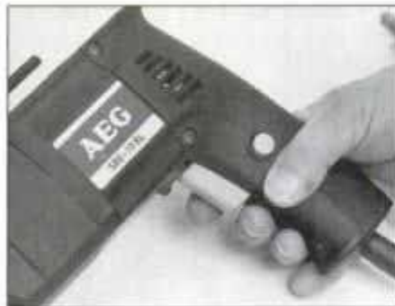
AEG, Bosch, DeWalt, Milwaukee, P-C and Skil have the reverse lever above trigger. Thumb controls trigger-lock button on most.
