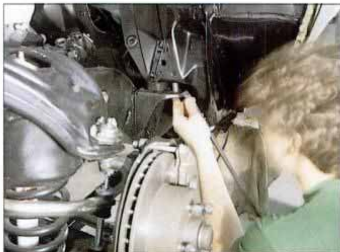
With the completed front subframe on its rack, Ken lowers the unibody until the locating pegs line up, then bolts them together.
