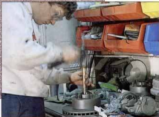
Ken Barnes taps a seal into our new front disc brakes. The new brake callipers are on the table in front of him.
