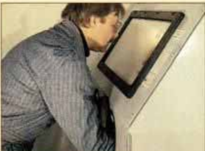
Blasting cabinet has a light and high-volume vacuum to keep down the dust.
