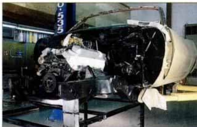
Our Camaro, back on its wheels and ready for bodywork and paint (top). Trial fitting of the front subframe (above).
