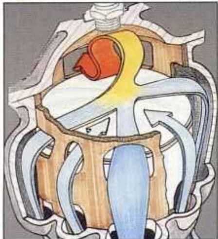
Two finger-size ports fine-tune induction on OMC's new Ocean-series outboards.
