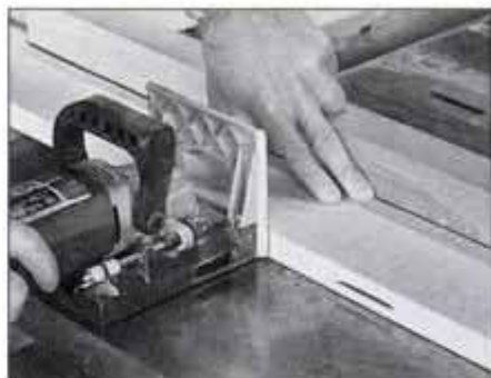
2 Cut the joining plate slots in the edge of each board. Work on the table saw or another clean, flat surface.
