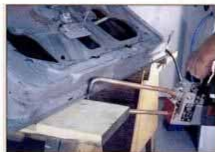
Eastwood's resistance spotwelder has long tips that reproduce factory spotwelds.
