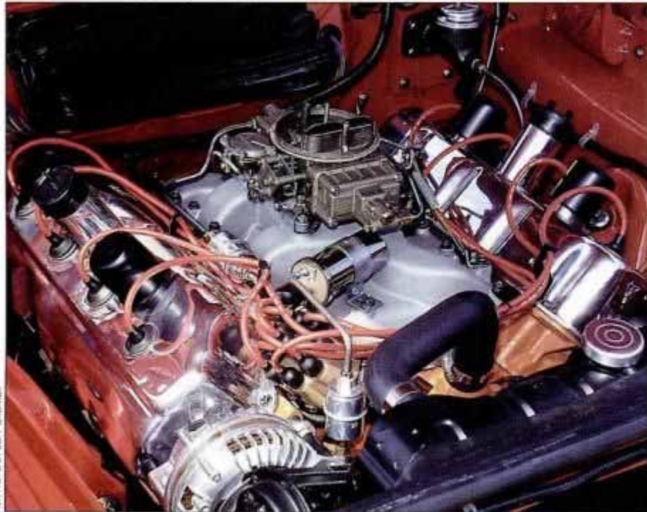
Chrysler 426 hemi for NASCAR used one 4-barrel carb. Street versions used two.
