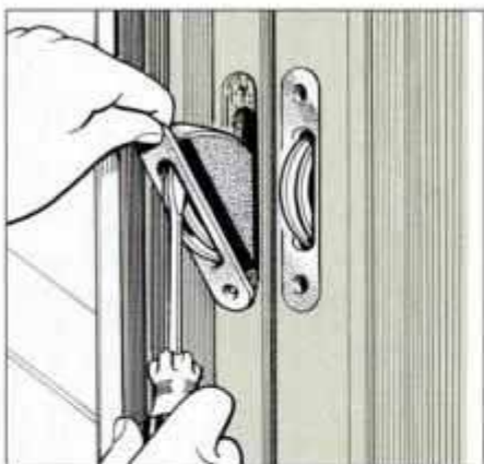
5 Remove the screws that hold the sash-weight pulleys, and pry the pulleys from the jamb using a screwdriver.
