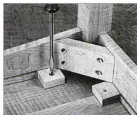
18 Invert the leg-apron assembly on the top with equal spacing all around. Screw the buttons into the top.
