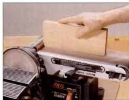
The belt sander has a stop at one end to hold small pieces in place. For longer work, stop and belt end cover must be removed.
