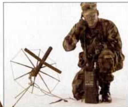
LST-5C satellite radio folds down into a compact, 12-pound unit, but can reach any spot on the globe.
