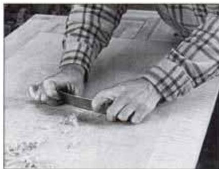
4 Before sanding the top, use a cabinet scraper to remove small areas of tearout from the hand plane.
