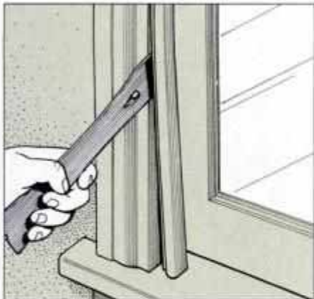
1 Remove the inside sash by prying off the inside window stop. To prevent breaking the stop, pry where it is nailed.
