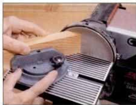
Miter gauge and tilting die-cast aluminum table enable accurate sanding of bevels, miters, compound miters and chamfers.
