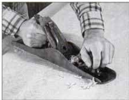
3 After glue-up, use a razor-sharp plane to remove irregularities in the top. Work diagonally or across the top.
