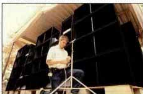
Sonic-boom simulator features servovalve speaker (right) for super-subwoofer.
