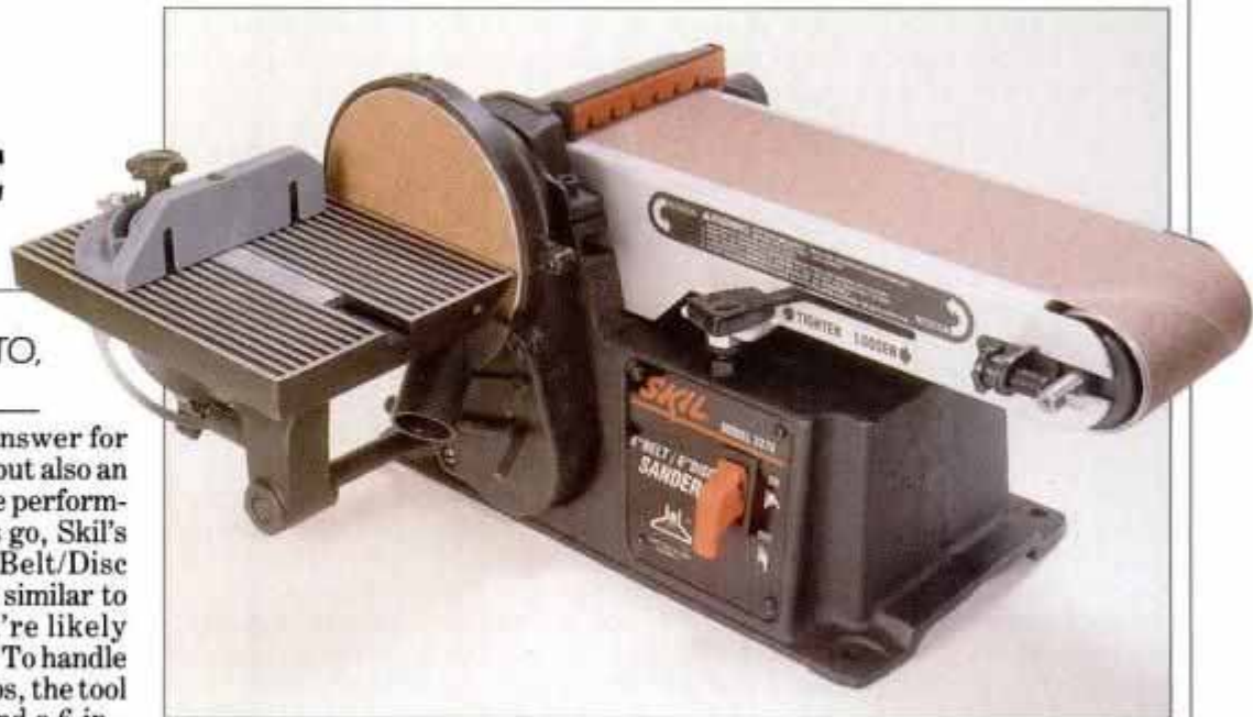
The Skil model 3370 Sander has a 4-in. belt and 6-in. disc. It features a tilting table that can be used with the belt or disc, and the belt can be positioned horizontally or vertically.
