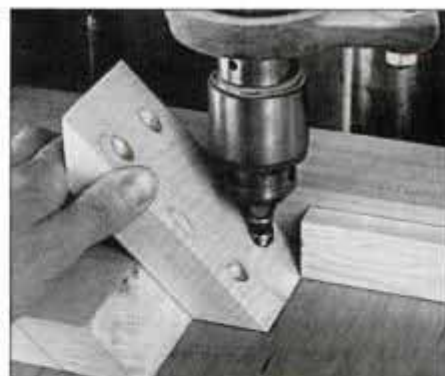
16 Clamp a stopblock and backrest to the drill press. Bore, then counterbore, the pilot holes in the corner blocks.
