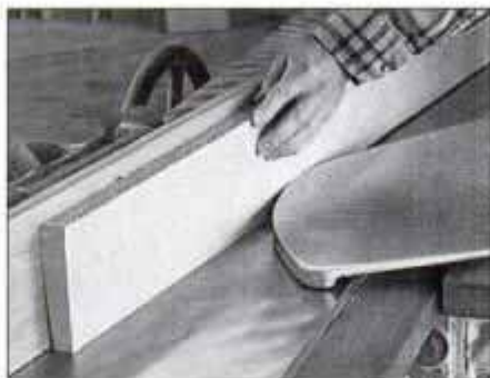
1 Joint one edge of each board used in the top. Rip the board slightly over width, then joint the sawn edge smooth and straight.
