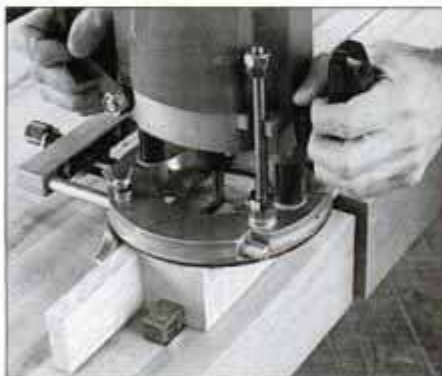
11 Cut the mortises with a plunge router and fence. Place a scrap piece next to the leg blank to support the router.
