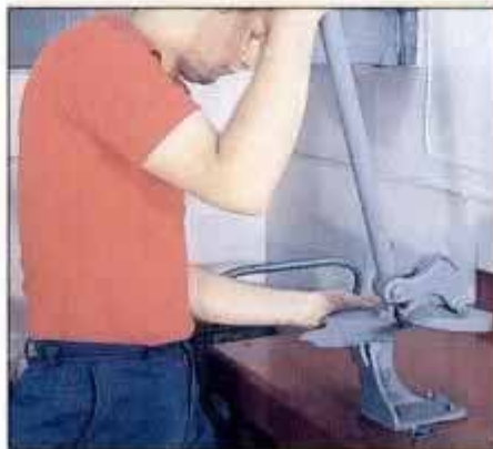
Ken Barnes cuts a sheetmetal patch with our throatless Beverly Shear, then bends it to fit.
