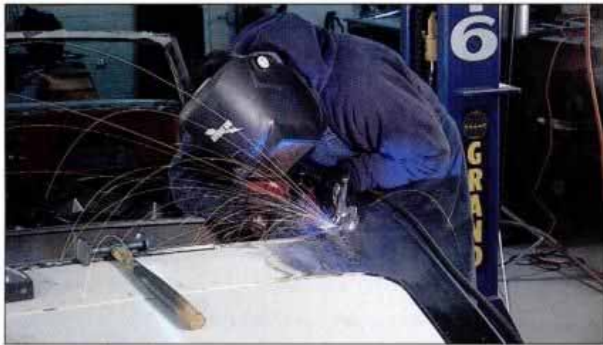
Our Camaro convertible is resplendent in all-new unibody panels and primed with "Yellow Death" (top). Don Breslauer grinds welds on a quarter-panel filler (above).
