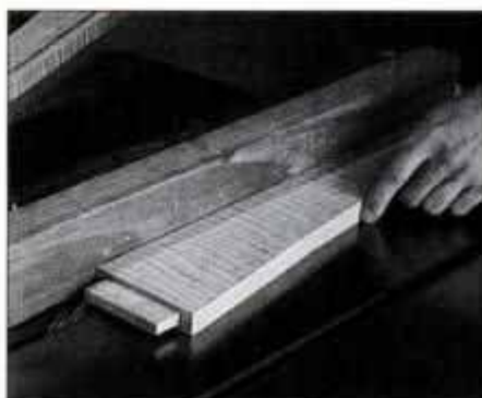
10 Cut the groove in the aprons with dado blades in the table saw. The small lip on each button fits the groove.
