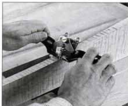
9 Remove the saw marks and smooth the apron's curve with a sharp spokeshave, or use a sanding drum on a drill press.
