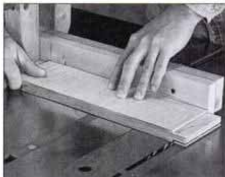
6 Saw the tenon shoulders with a miter gauge and extension fence. Note the parallel jaw clamp that acts as a stop.
