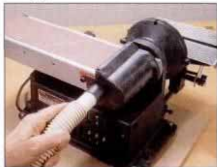
Dust collection is facilitated by vacuum hose ports—one at the belt cover and the other at the disc cover under the table.
