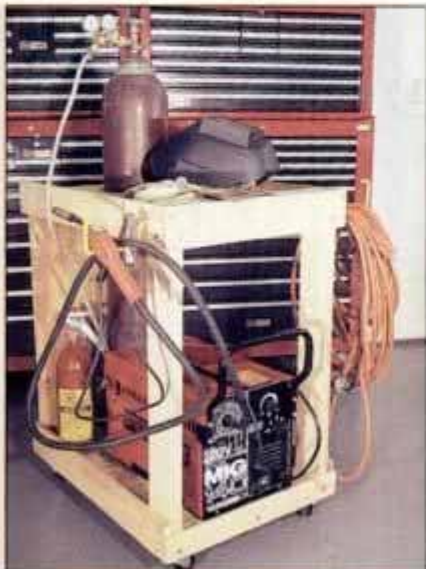
Our homemade cart carries the Daytona Mig welder and all supplies.
