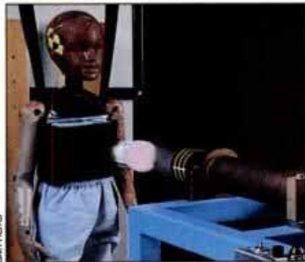
Pitching machine fires fastballs at child-size dummy to test protective gear.
