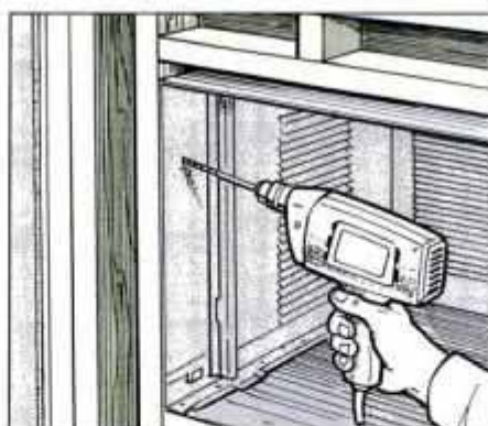
19 Position and shim the sleeve in the frame with flashing tucked under the siding. Drill holes to attach the sleeve.
