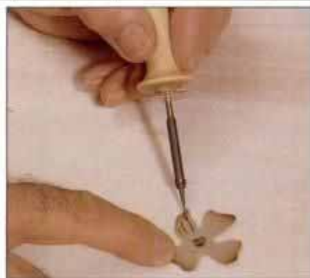
19 Use a woodburning pen to add linear details, such as petal striations and veining in leaves. Hot nail scorches dark center.
