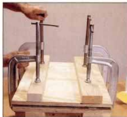
22 Sandwich assembly between wax paper and 3/4-in. plywood. Use newsprint as a cushion and apply clamps to crossbearers.
