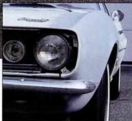
Cheap replacement fender was part of a 10-year-old "restoration"—note the poor fit.
