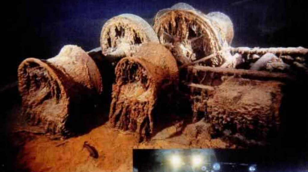
Massive, steam-driven windlass (above) was used to hoist cargo, and now dissolves into rust on the forecastle. Mir photographs Mir (right) near the bronze steering telemotor that held the ship's wheel inside the now-demolished wheelhouse. A rattfish (below) glides over broken champagne bottles and White Star Line china.
