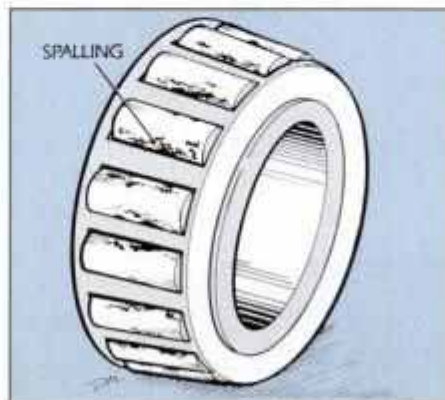
A bearing that shows chips, spalling or deep scratches must be replaced.
