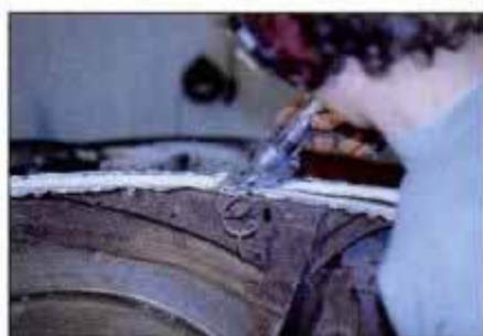
Air-powered shear makes a clean cut as to the jagged edge left by the air hammer.
