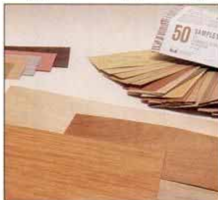
2 Veneers used in marquetry are available in a wide range of natural and dyed colors. A veneer sample kit is a good way to start.
