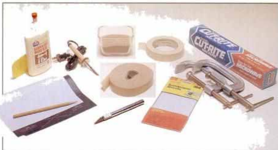
1 Tools and materials used in marquetry include a razor knife, tracing paper, carbon paper, 4H pencil, gummed veneer tape, masking tape, white or yellow carpenter's glue, wax paper, woodburning pen, shading sand, sandpaper and clamps.
