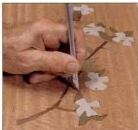
15 The leaf cutout on the background acts as a template for the actual leaf piece. Hold the knife vertically for scoring.
