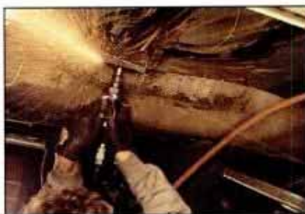
Air shear makes a neat job of sectioning floor pan at seat tubs.
