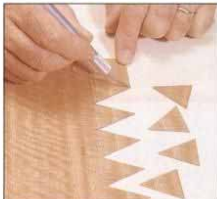
4 Make practice cuts to become familiar with using the knife. Always cut away from the corners to avoid splits and tears.
