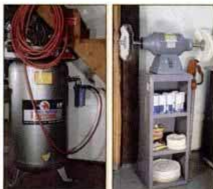
Our 5-hp, 80-gallon compressor and 3/4-hp buffer get used every day.
