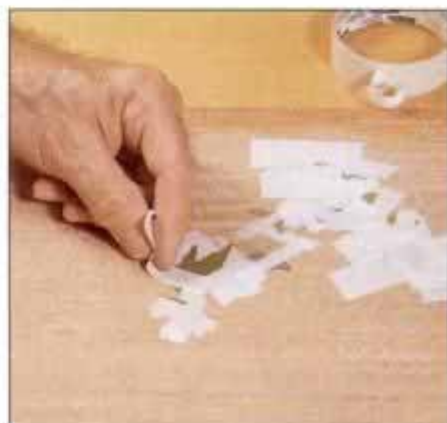
17 Masking tape can build up on the underside. Remove small pieces and use fewer long pieces to even out assembly.
