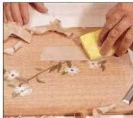
23 After the glue is dry, use a damp sponge to soften the veneer tape adhesive. Avoid wetting surrounding area.
