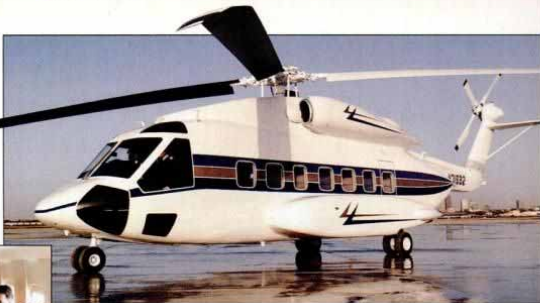
Sikorsky S-92 has 54-ft. fuselage with enough interior space to carry 19 passengers.
