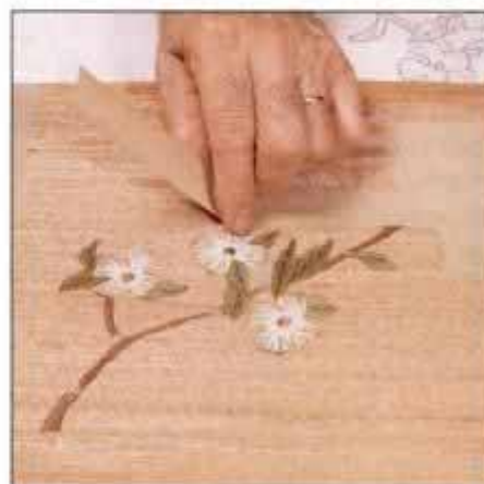
20 Remove masking tape and replace it with parallel strips of gummed veneer tape. This side will be the finished side.
