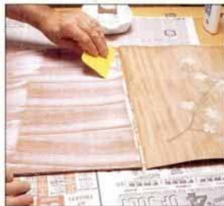
21 Apply glue to ground, not to veneer, and use backing veneer to balance assembly. Plastic applicator spreads glue.
