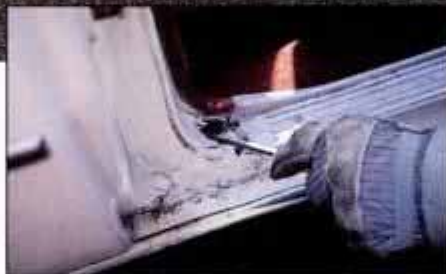
Rust-through in doorjamb is typical of older unibody cars.
