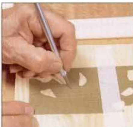
16 Use masking tape to hold the veneer on a cutting board for better control. Use solid wood or plywood for cutting board.
