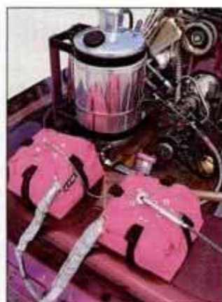
Clockwise from top right: Twin Dietz parachutes and a 4-plus-gallon fuel tank are features on the Blown Alcohol Hydro Money For Nothin' ; an anodized housing guards the split shaft of the Casale V-drive; and an Enderle fuel-injector hat and Mooneyham supercharger sit atop an aluminum Aries-built intake manifold, heads and block.
