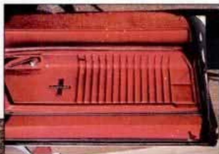
Stock door panels were cracked from age and had been cut up for speakers.
