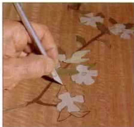
14 Follow the procedure for each piece to be cut and fitted. Here, leaf shapes in our floral pattern are cut from the background.
