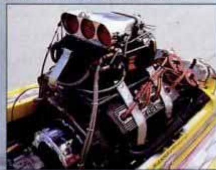
The hull of QuarterFlash (far left) features the classic twin-sponson, 3-point-hydro design. Beneath the canopy (left), is a tight but well laid-out cockpit. Note the safety restraints on the supercharger on the boat's massive tower of power (below). Top Fuel Hydro Spirit of America (opposite page) attacking a sub-6-second run.
