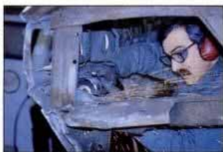
The rusty unibody must be cut apart very carefully, like peeling an onion.
