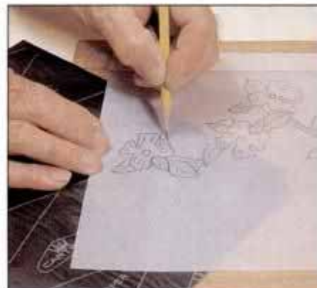
5 To transfer pattern to veneer, hinge tracing paper to veneer and place carbon paper in between. Then trace outline.
