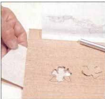
7 After the window is cut, place the selected fill veneer under the opening and tape in place to prevent shifting.
