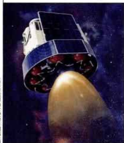
Apogee-boost rocket can wait 12 days before placing DSCS-III.
