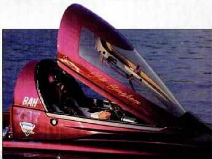
Top Fuel Hydros like Caught N the Act (left), which is equipped with an experimental tail fin for stability, scream through the liquid quarter-mile at speeds beyond 200 mph. The protective canopy (above) is the top part of a Kevlar-reinforced safety capsule that greatly improves Money For Nothin' driver Cliff Bingham's chances of walking away from a violent crash.
