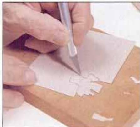
9 Then, remove the veneer and lay it on the cutting board. Cut out the shape by making light passes with the razor knife.
