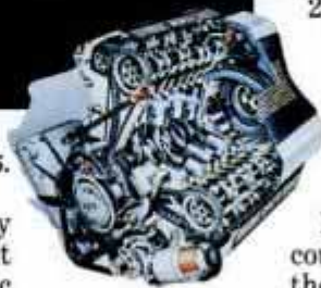
BMW's 7-series sedans will get V8 power for '93. The new dohc 32-valve aluminum engines will be BMW's first production V8s since 1965.
