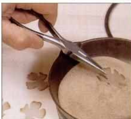
18 Heat shading sand in pan on hotplate and insert veneers to create gradated tone. Test process with scraps first.
