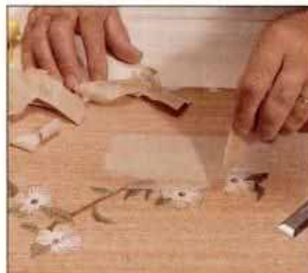
24 Use a chisel to start lifting the veneer tape at one end. Then, peel away tape. If glue still holds, remoisten tape.
