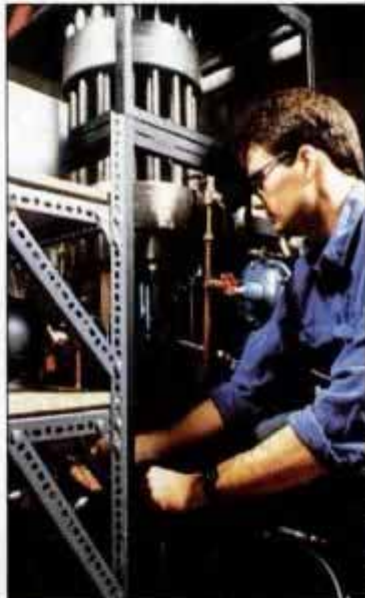
Hot triaxial compactor applies shear stress to metal powders, yielding new microstructures.
