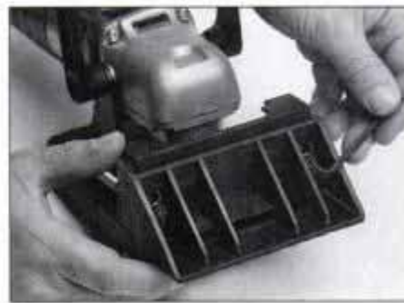
6 Allen screws on Skil must be removed to reverse fence or to shift fence from one of two fence-location ranges.
