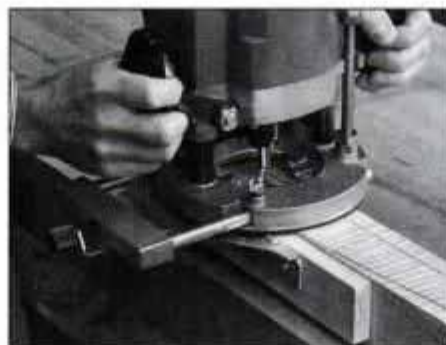
5 Lay out the mortise locations and the leg profiles on the front leg blanks. Cut the mortises with a plunge router.
