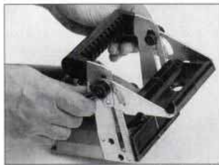
5 Ryobi fence is locked with side levers. It pivots forward and backward, and slides up and down through 2½-in. range.
