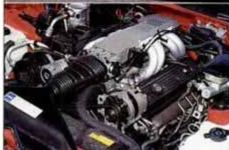
350-cu.-in. tuned-port fuel-injected V8 engine delivers 245 horsepower and 345 ft.-lb. of torque. Cornering is flat. Instrumentation is very readable.
