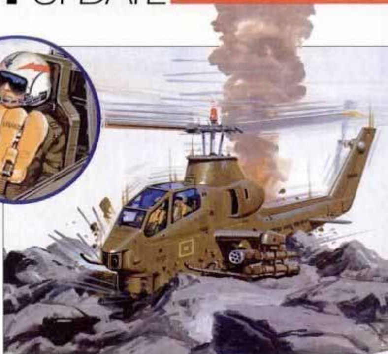
In crash landings, AH-1 Cobra attack chopper drivers will benefit from airbag system that borrows automotive technology.
