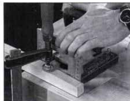
14 Cut the matching plate slots in the rear legs. Note that the plate joiner is shimmed with sheetmetal to the correct angle.
