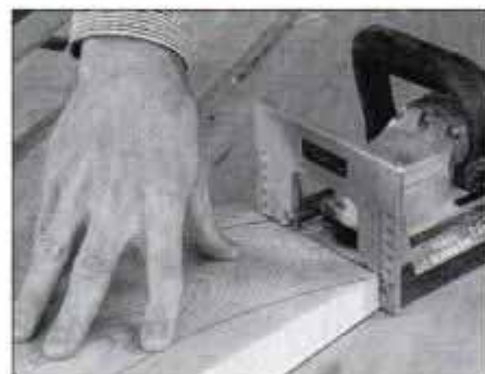
13 Lay the flat face (the front) of the top rail on the bench, and cut the slot for the joining plate that joins rail with legs.
