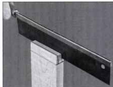
10 To cut the tenon cheeks, hold the rail upright in a vise and saw just to the waste side of the line. Clean up with chisel.
