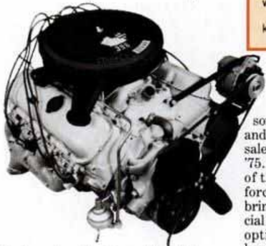
Most popular of the Camaro big blocks was the 325-horsepower version of the 396.
