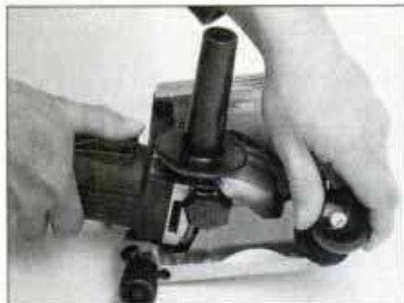
1 Elu joiner is pivoted into stock when making a slot. This design allows the tool to serve as a trim saw and grooving tool.
