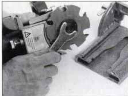
3 Blade change on Lamello Top 10 is simplest of all plate joiners tested. Spindle lock, also found on Ryobi, speeds removal.
