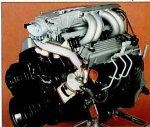
Tuned-port fuel injection came on-stream in '85. The 350-cu.-in. Corvette engine became available two years later.
