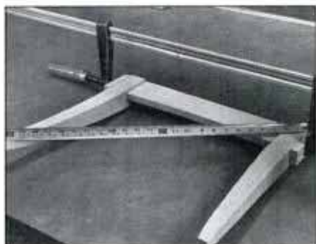
17 Glue and clamp the front legs to the front rail. Measure the diagonals to check for square and adjust if necessary.
