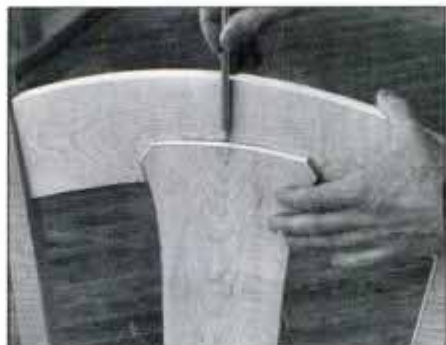
15 Saw the rail's front curve and smooth it. Dry assemble the chair and copy the curve on the back of the splat.
