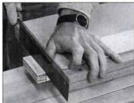
9 Cut the angled tenons on the side rails with dovetail or back saw. To cut the shoulders, clamp the rail in a bench hook.
