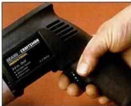
Trigger on ¾-in. drill has a speed dial so any point in the speed range can be locked on. Reversing switch is above the trigger.
