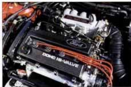
Mazda-built 1.8-liter dohc 16-valve Four is available only in GT and LX-E models.
