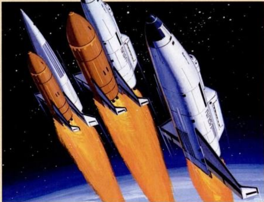
AMLS rocket-powered options include (left to right): advanced 2-stager with cargo held internally, near-term 2-stager with external payload bay and advanced single-stager.
