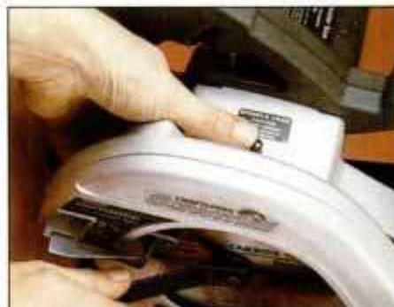
A convenient spindle lock on the Sawmill makes blade changing fast and easy. Blade wrench stores in stamped-steel base.
