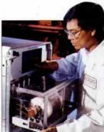
Rotating bioreactor frees cells from gravity, allowing complex tissue growth.
