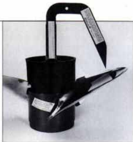
The inexpensive Propeller Pitch Gauge dials in the difficult-to-measure prop blade angle.
