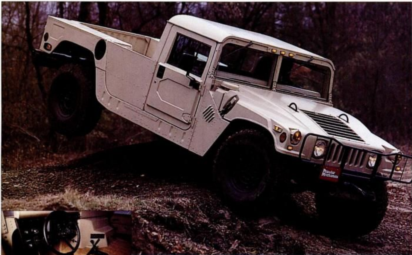
A General Motors 6.2-liter diesel Turbo 400 automatic transmission and Torsen differentials pull the Civilian Hummer into (and out of) some pretty heavy sledding.
