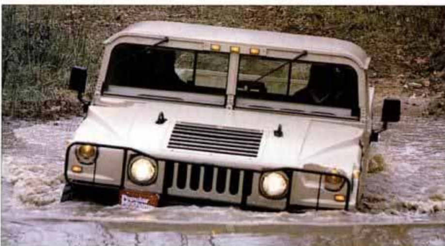
Hummer's capabilities include traversing 40% slopes and fording 30-in.-deep streams. Its chassis can take a pounding that leaves other 4x4s dead on the trail.
