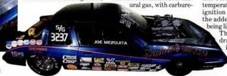
Joe Mezquita's 700-hp "super gas" racer is the only drag car on the circuit fueled by natural gas.
