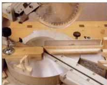
14 Cut opposing ends by reversing block and miter angle from right to left. Flat stock can be handled from one side.
