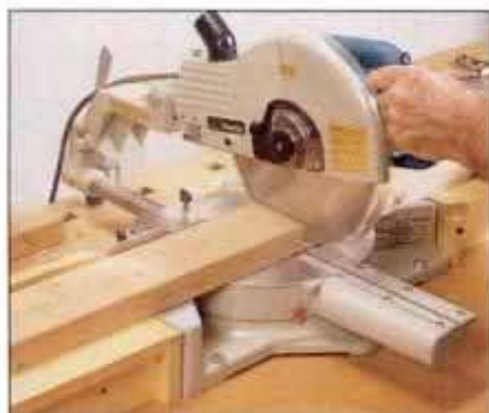
2 A press cut is made by gently lowering blade into stock. Carriage is locked at fence position on sliding compound miter saws.
