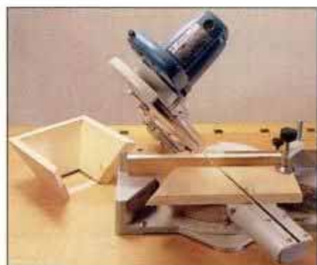
17 Use compound cutting to make tapered boxes and frames. Kerf cut in wood fence ensures stock alignment with blade.
