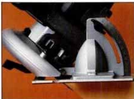
A maximum 50° bevel setting is 5° more than typical 7¼-in. saws. Large knob and smooth action make adjustments easy.
