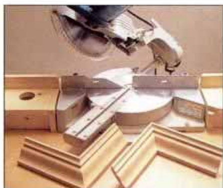
16 To cut inside or outside miters on crown molding, miter and bevel adjustments are made to produce compound cut.
