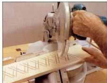
20 Make a decorative pattern by locking the blade depth and making angled press cuts at regular intervals along a board.
