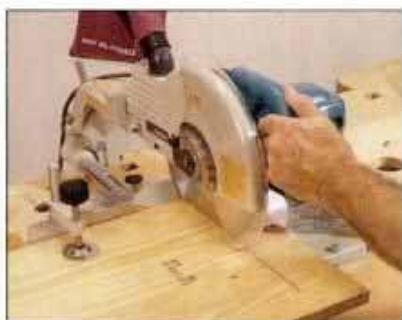
6 Cut stock that's wider than saw capacity by first cutting in from one side. Clamp work to table for maximum stability.
