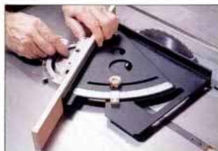
3 The tool makes for extremely precise setup. Here, it's butted between the table saw blade and the miter gauge fence.
