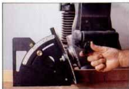
2 Both of the tool's working surfaces are wide flanges. This makes it easy to stand the tool and tilt a blade against it.
