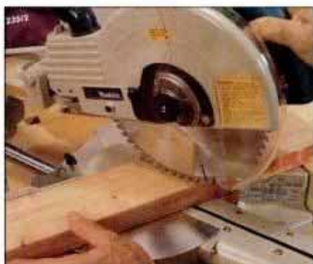
3 To make a cut precisely on a marked line, first lower the blade with the power off so it's slightly to the waste side of the line.
