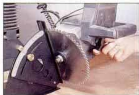
1 AngleWright's flanged surface is 11 in. long, more than enough to span even large-diameter saw blades.
