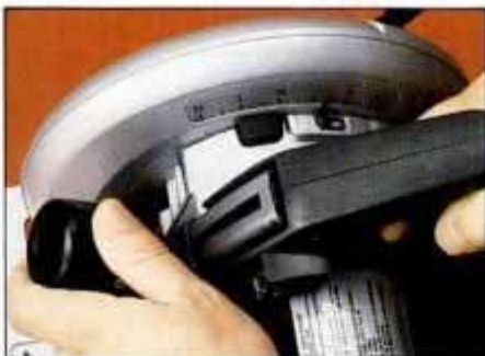
Front knob locks or loosens modified pivot-foot blade-depth adjustment. Scale on blade guard indicates depth of cut.
