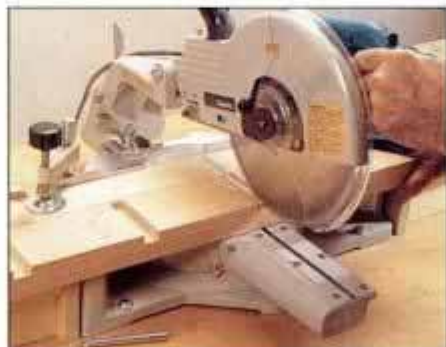
19 Lock blade depth for partial kerf, and make slide cuts to cut dado. Spacer behind work ensures uniform cutting depth.
