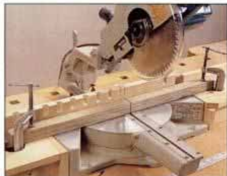
18 To make dentil molding, position and lock carriage so partial cut is made. Kerf in guide strip helps in aligning stock.
