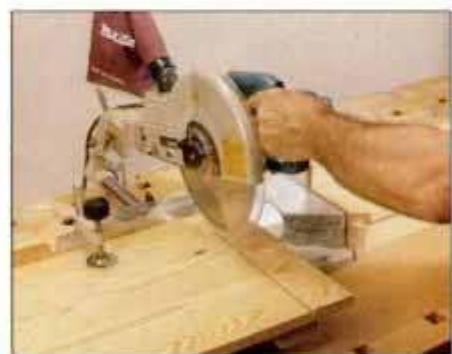
7 Finish the cut by flipping over the workpiece. Use partial kerf and blade to align stock accurately, and clamp work to table.
