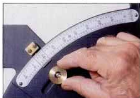
4 Set AngleWright by loosening its knurled thumbscrew and positioning the red line at the desired angle.
