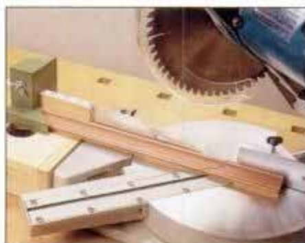
11 To cut frame miters, first cut one miter on each piece. Set the miter stopblock for frame length and miter opposite ends.
