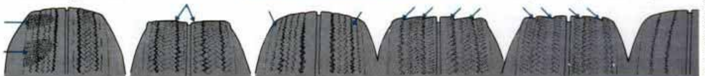
Tire tread wear indicates (from left to right) worn suspension, overinflation, underinflation, toe and camber problems.
