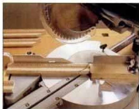
13 Next, clamp scrap stopblock to table so the blade intersects the corner of the work. Cut similar end of each piece.
