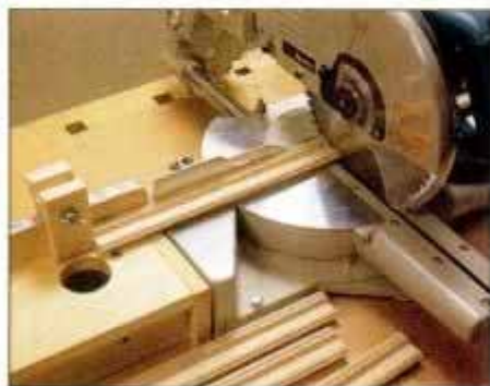
12 To cut accurate mitered frames with a straight stopblock, first cut each frame member squarely to exact finished length.
