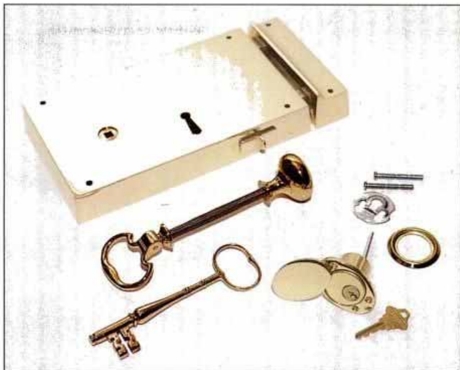
This rim lock has a built-in deadbolt. The brass box mounts inside the door and the key cylinder mounts outside. The knob spindle mounts through square hole in the box.
