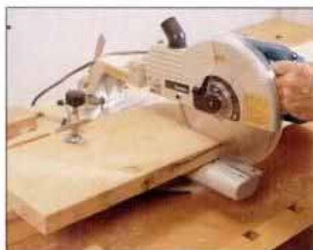
5 To make a slide cut, move carriage to its extended position. Then, start motor and push the blade through the workpiece.
