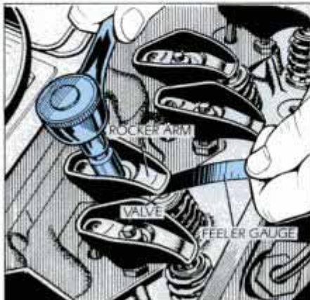
Tighten the locknut until the feeler gauge drags between valve stem and rocker.
