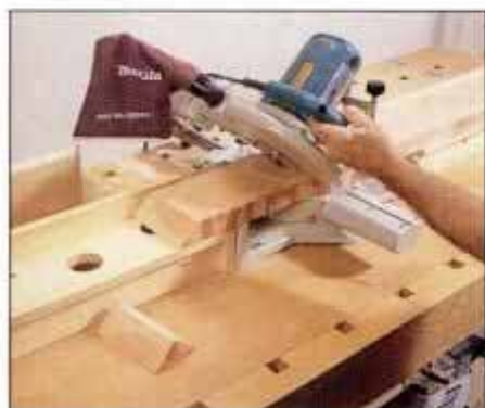
15 Compound miter saws only tilt to one side, so the opposing bevels shown are made by reversing the workpiece ends.
