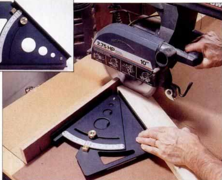
AngleWright is a 0° to 45° pivoting triangle used to set blade angles or to position stock for making cuts like face miters with a radial-arm saw.
