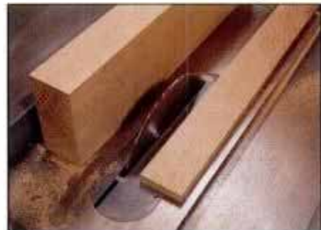
3 A piece of red oak is resawn with the Mach 1 to demonstrate glue-quality surface left by saw blade.
