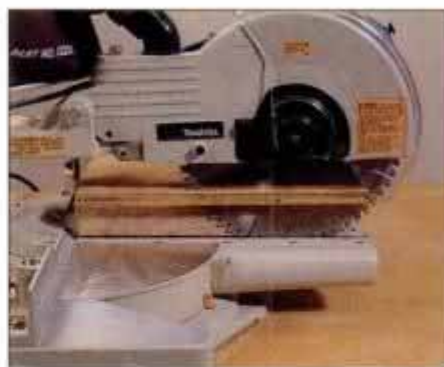
8 To increase crosscutting capacity slightly, place a spacer under the work so it is contacted by a larger section of the blade.
