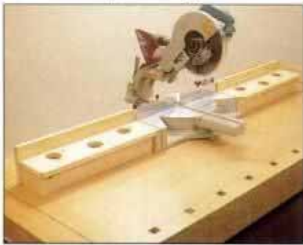
1 These easy-to-make extension tables provide 72 in. of work support. Holes allow clamp access for securing workpiece.
