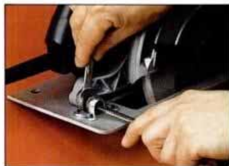
Alignment between blade and aluminum base edge is adjusted at pivot joint. Parallel alignment ensures smooth and accurate cuts.
