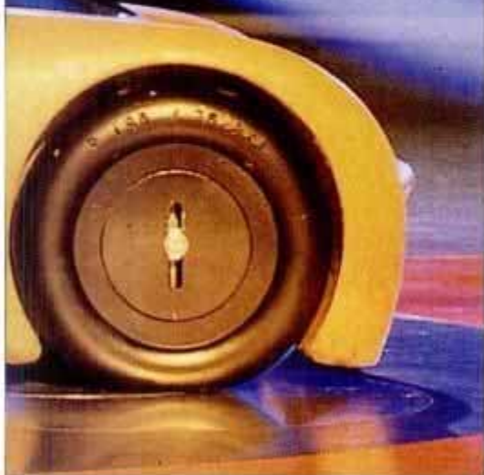
Carbon-fiber body shell consists of six sections and weighs only 420 pounds.
