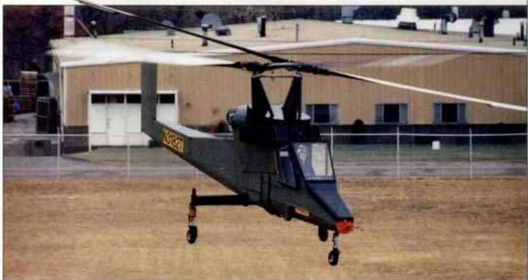
Kaman intermeshing-rotor technology demonstrator lifts off during early tests.
