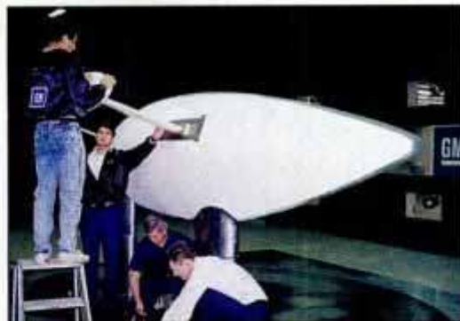
Engineers prepare a one-third-scale model of Stars & Stripes for testing in the GM wind tunnel.
