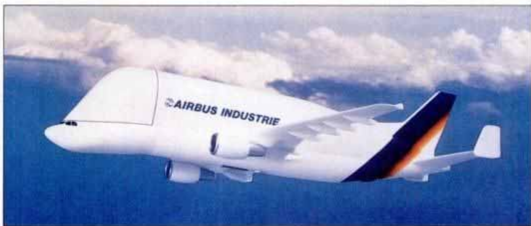
Airbus Super Transporter features cockpit below floor level to allow fast front-end loading.
