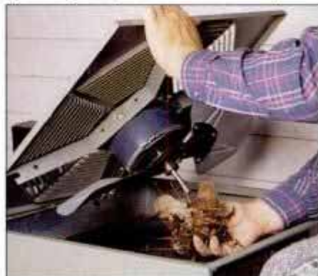
3 Carefully lift up the top panel and remove, by hand, any debris from inside the condenser coil or the area below the fan.
