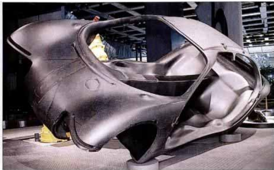
Carbon-fiber body shell consists of six sections and weighs only 420 pounds.
