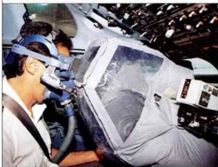
Emergency Vision Assurance System inflates during smoke emergency to give pilot clear view of instruments and flight path.
