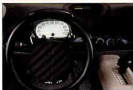
Speedometer uses electroluminescence lighting.
